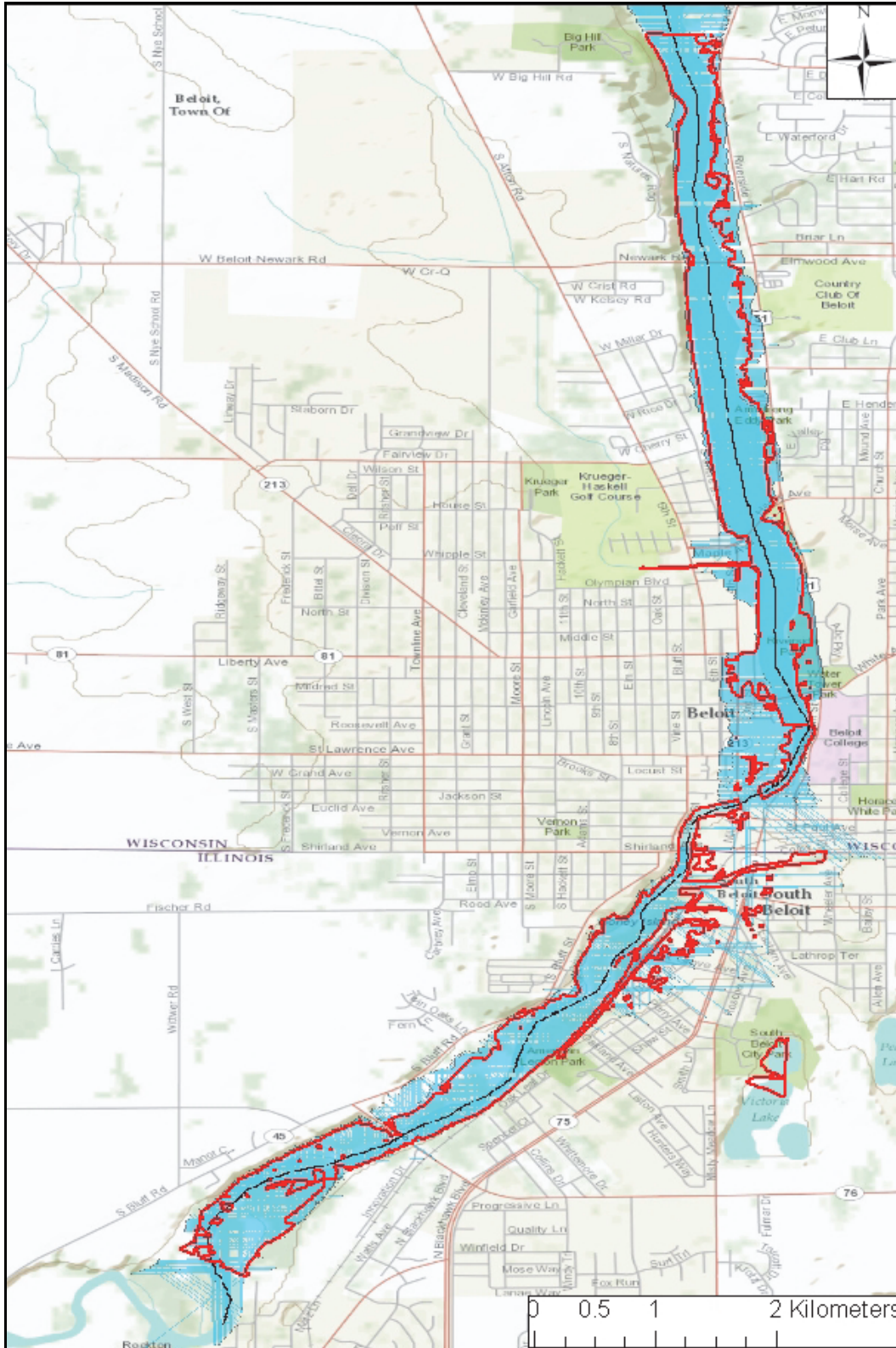
Figure 8. June 2008 Flood of Beloit, WI/IL, 10-m DEM, peak flow = 368 m 3 /s
