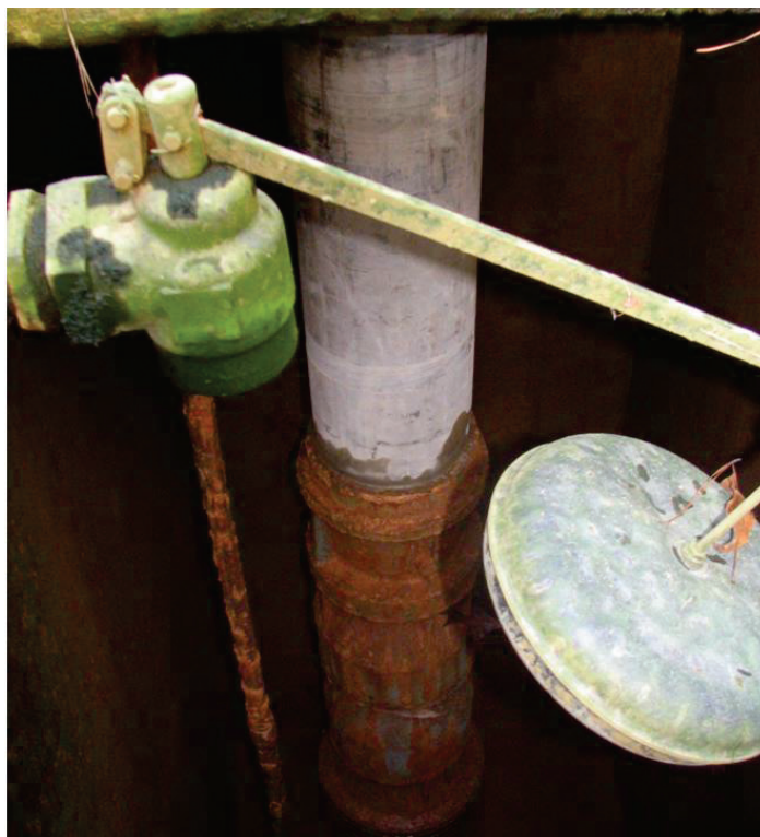
Figure 28. Pump 5 (316 Stainless Steel), 12 months exposure.
