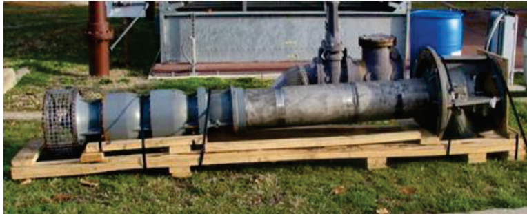
Figure 12. New pump 5 incorporating 316 stainless steel housing.
