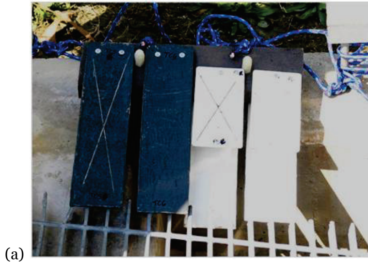
Figure 25. Macropoxy primer-topcoat and primer-only panels for pump 3 exposures at 3 months (a), 6 months (b), 9 months (c), 12 months (d), and 30 months (e).
