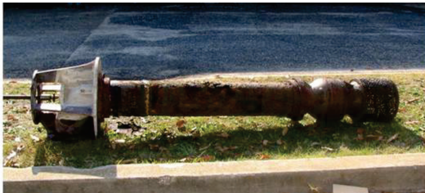
Figure 7. Condition of pump housing 4, after removal from sump.
