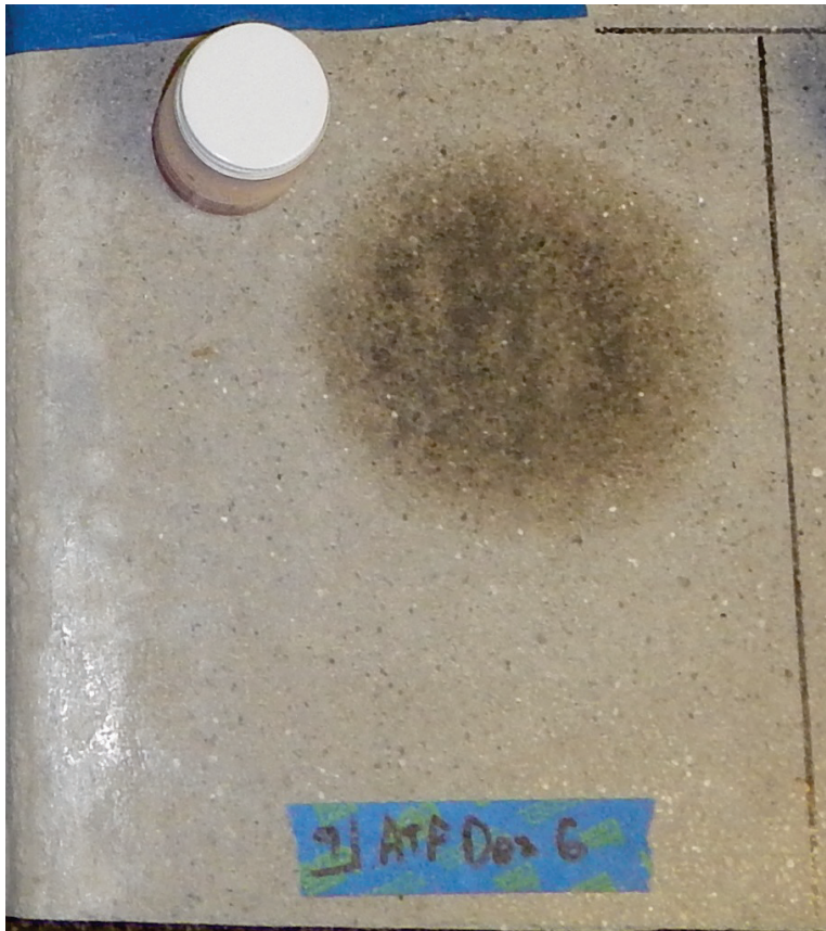
Figure D23. Test 9-Hydraulic Fluid ATF Dextron 6.
