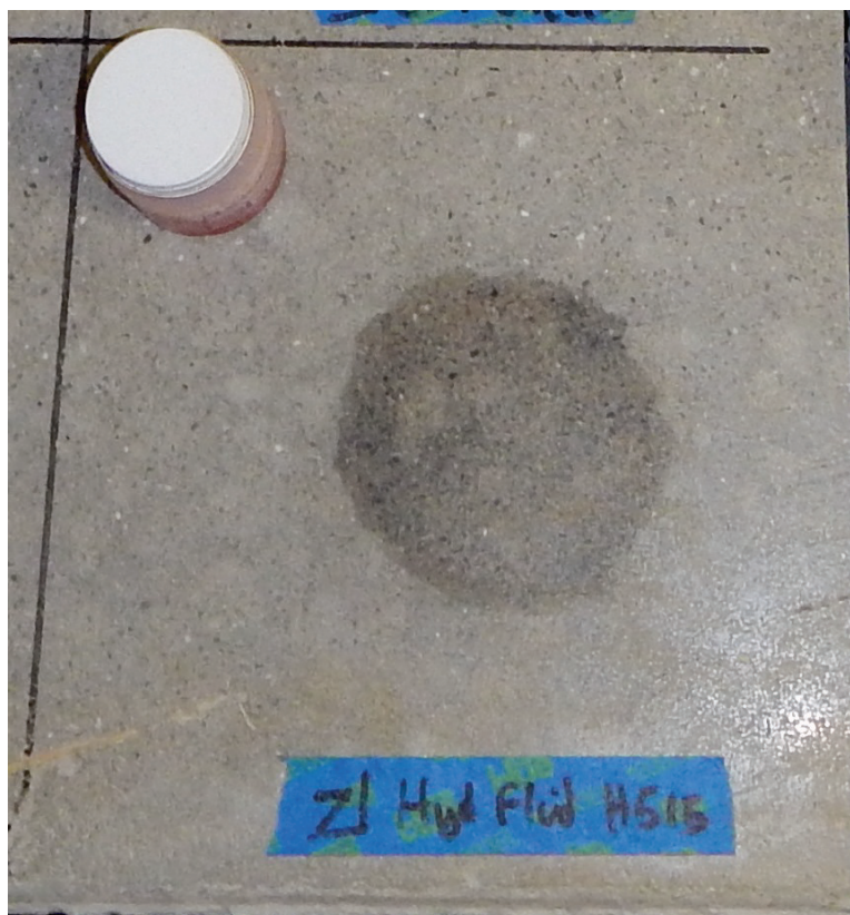
Figure D21. Test 7–MIL-PRF-5606H hydraulic fluid.
