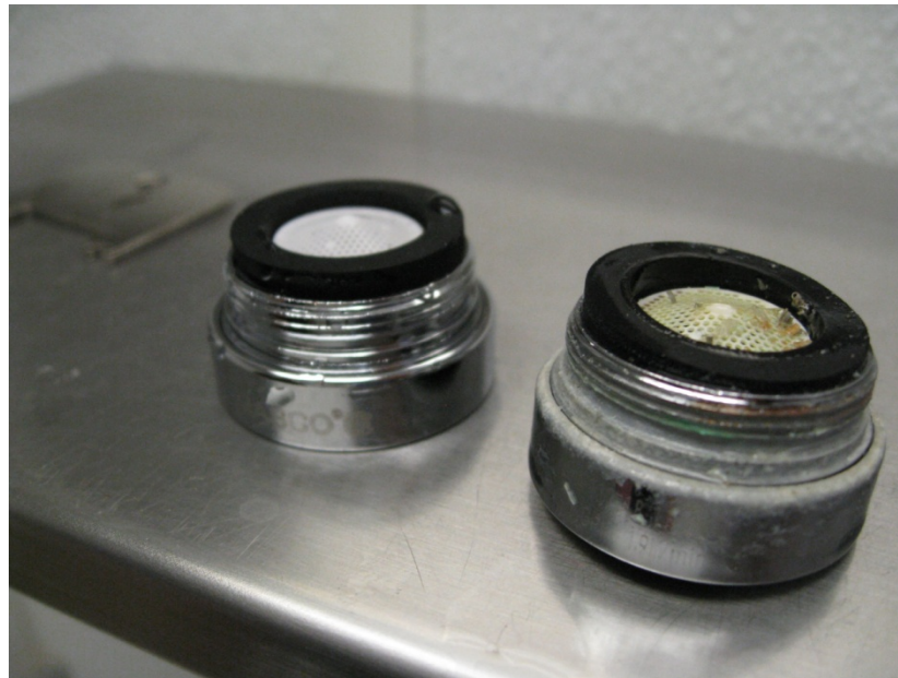
Figure 35. New 0.35 gpm and old 0.5 gpm faucet aerators.
