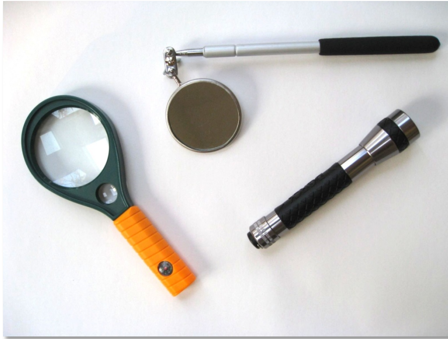
Figure 12. Fixture inspection mirror, magnifying glass, and flashlight.
