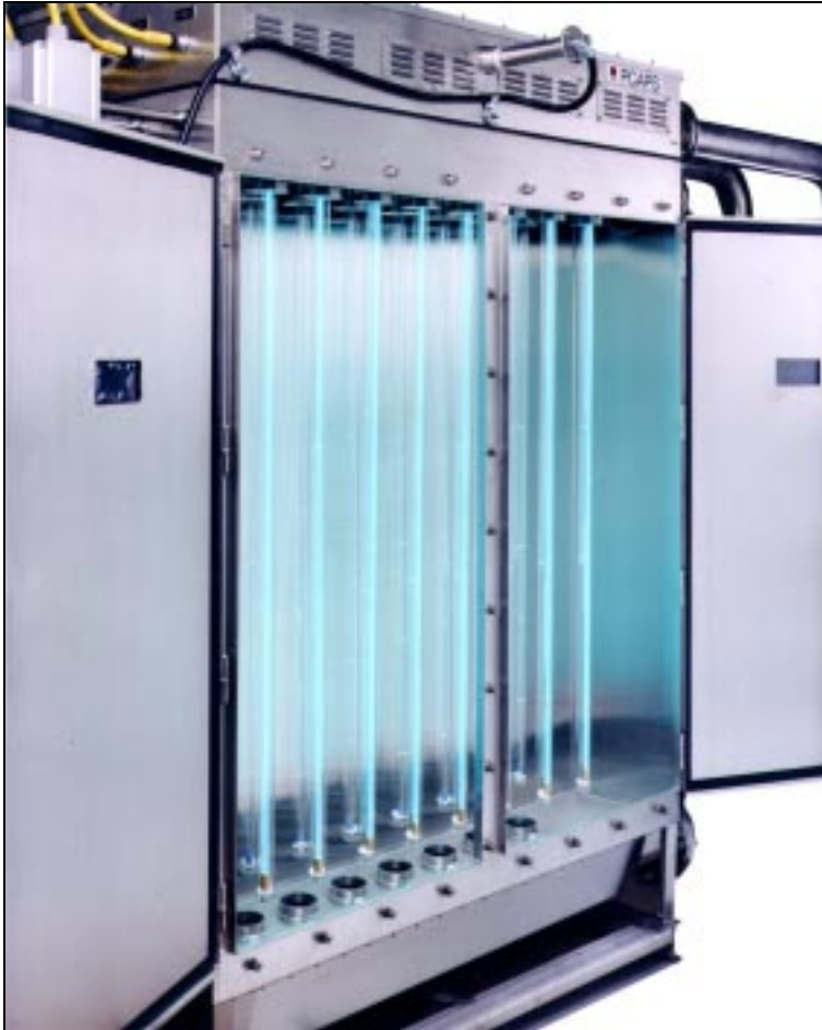
Figure 16. Interior of a 650 SCFM PPCU module.
