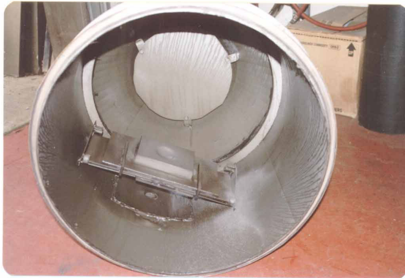
Photograph 4 Interior of Abrasive Breakdown (impaction) Chamber with Impactation Plate Mounted
