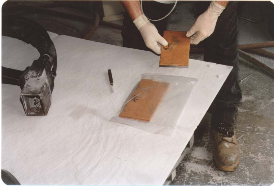
Photograph 1 Removal of Protective Coverings Prior to Metallizing
