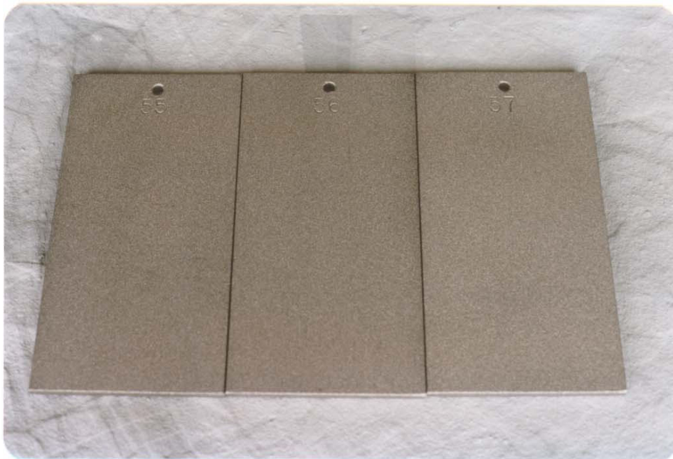
Photograph 2 Representative Condition of Test Panels Prior to Metallizing
