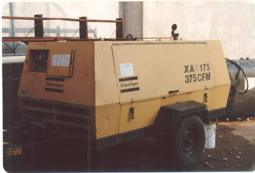
Photograph 1 Atlas Copco 375 CFM Air Compressor used to Maintain 95 psi Blast Nozzle Pressure
