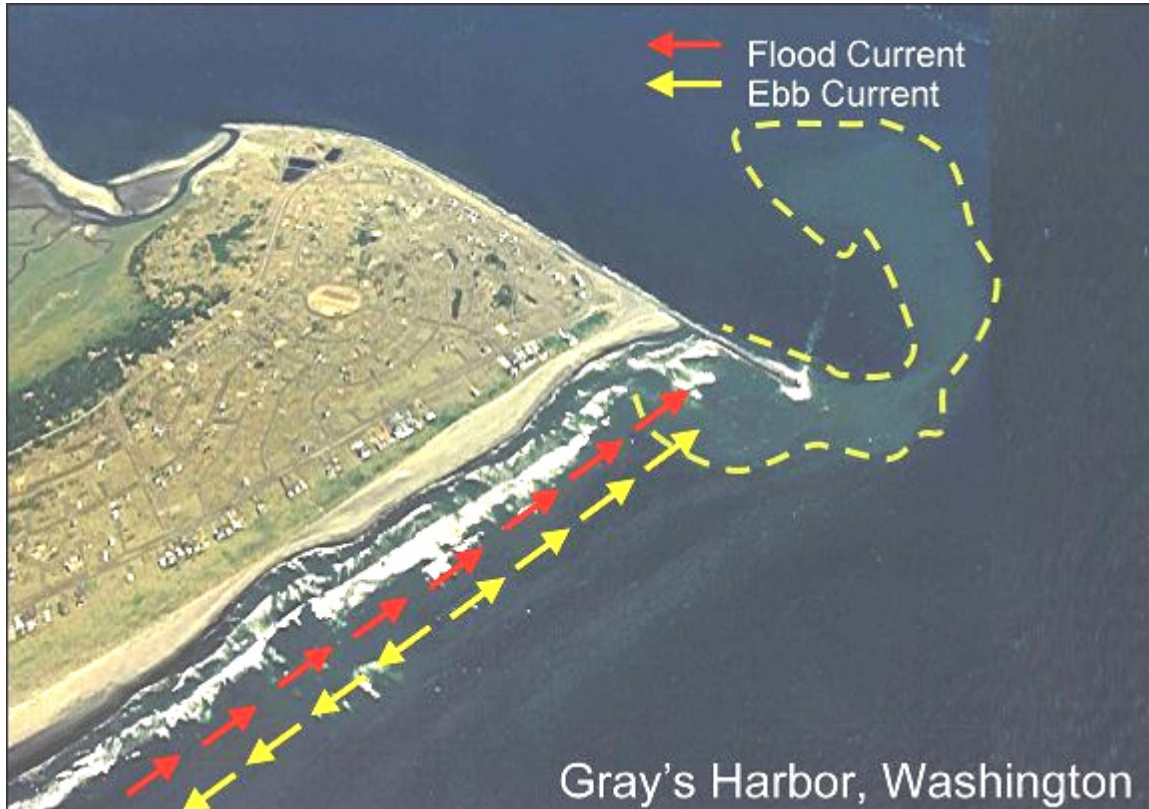
Figure 3. Sediment-laden longshore currents moving around Gray's Harbor north jetty
