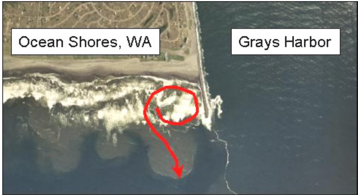
Figure 7. Bathymetric control of waves creating counterclockwise circulation near Grays Harbor north jetty
