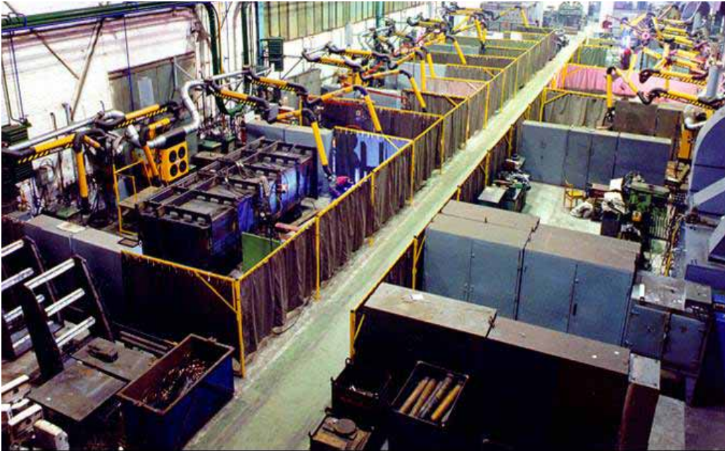
Figure 14. Articulated fume extraction arms with a built-in damper and a task light.
