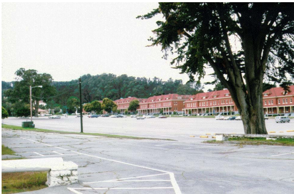
Figure 6. Impervious surfaces of large parking areas located close to buildings can give rise to “heat island effects” (source, R. Young).
