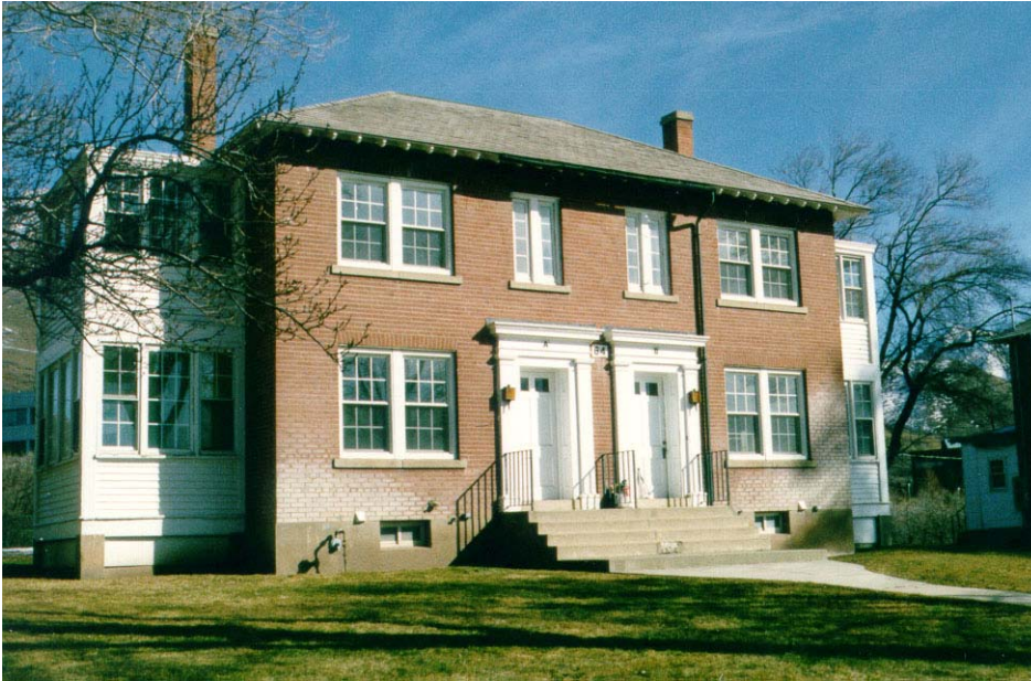
Figure 10. Passive solar orientation with east/west shade trees is a good use of renewable energy (source, R. Young).
