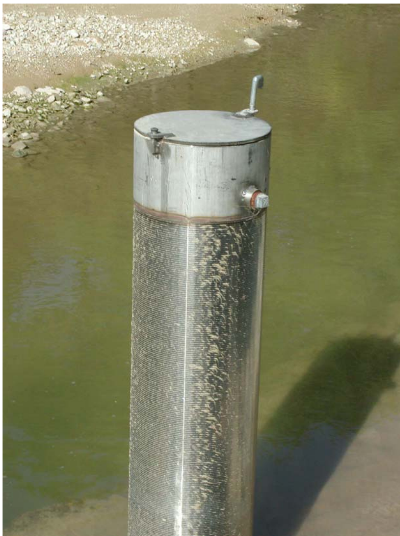
Figure 5. Enclosure for stream sensors.
