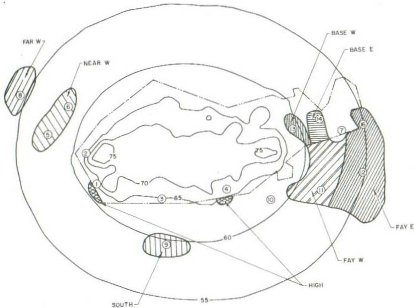
Figure 2. Final 1-year blast noise contours.
