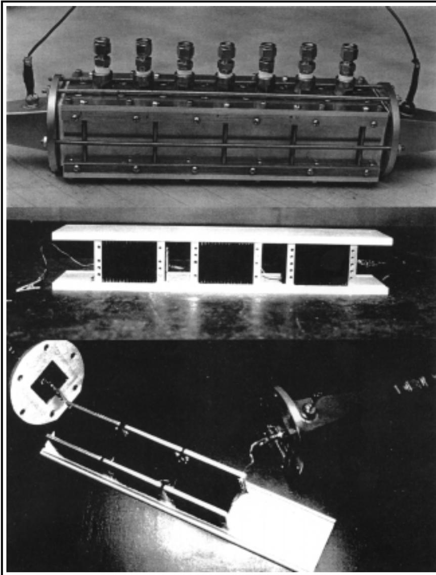
Figure 3. ACFC fixed-bed, fully and partially assembled.
