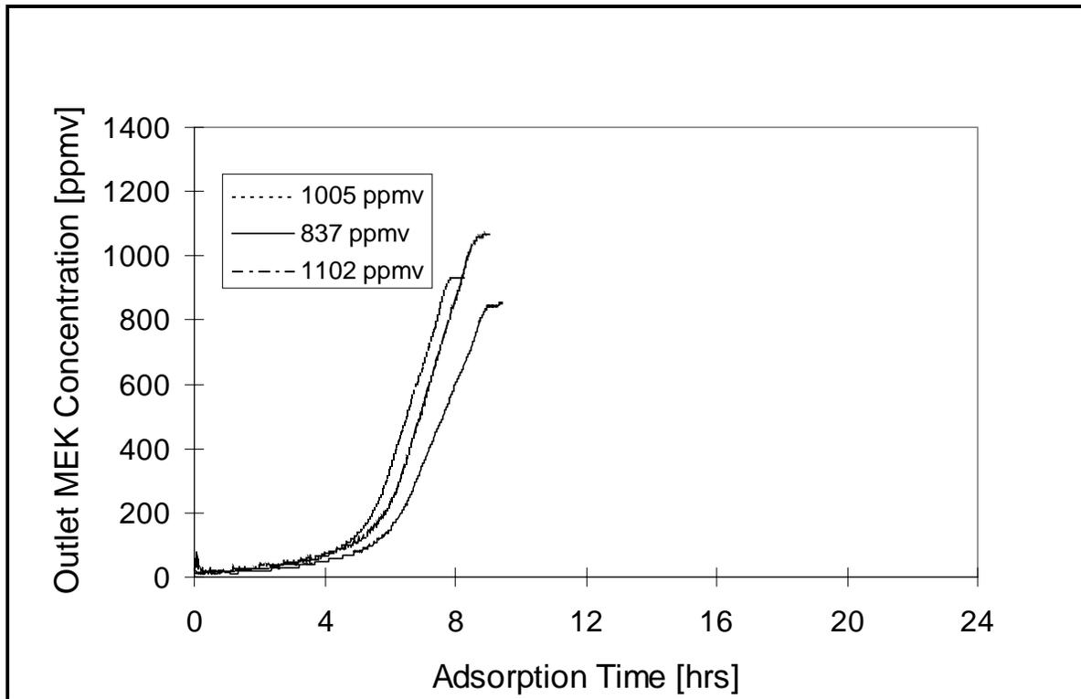
Figure 11. Adsorption breakthrough results for MEK in humid air.
