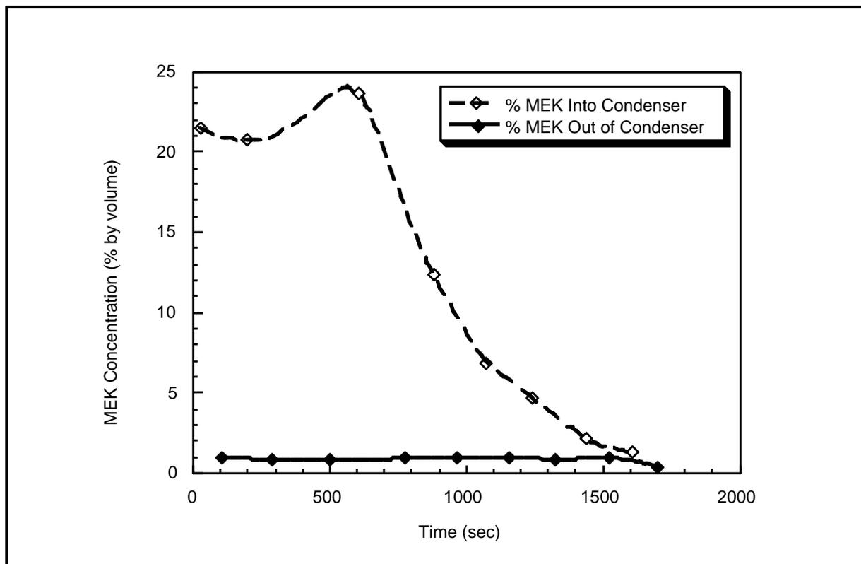
Figure 25. Condenser inlet and outlet MEK concentrations.
