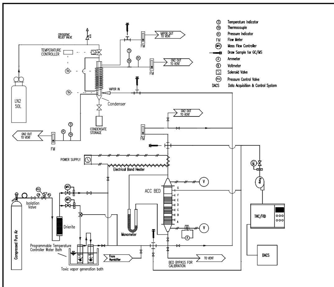
Figure 1. Laboratory-scale ACFC adsorption-cryogenic recovery system.
