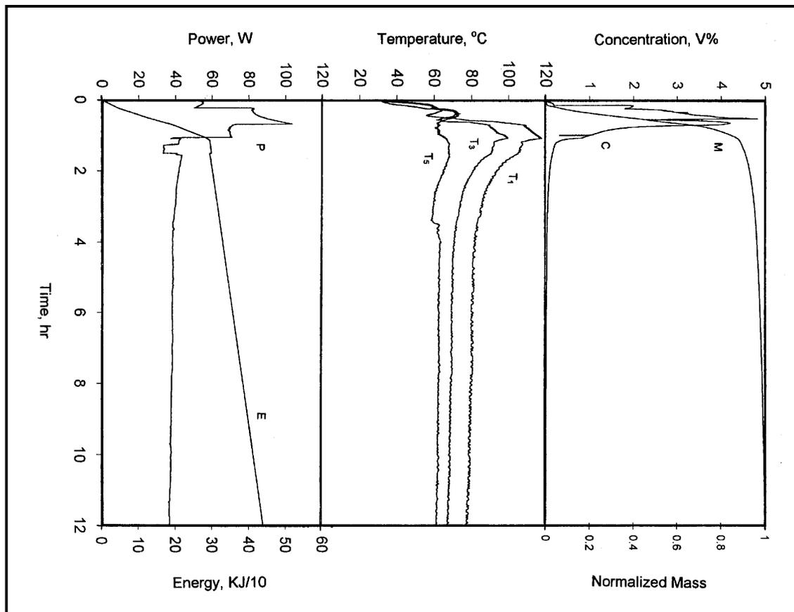
Figure 18. Results for MEK desorption from H<sub>2</sub>O/toluene adsorbed condition.
