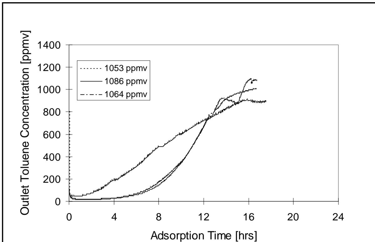
Figure 15. Adsorption breakthrough results for toluene in humid air.
