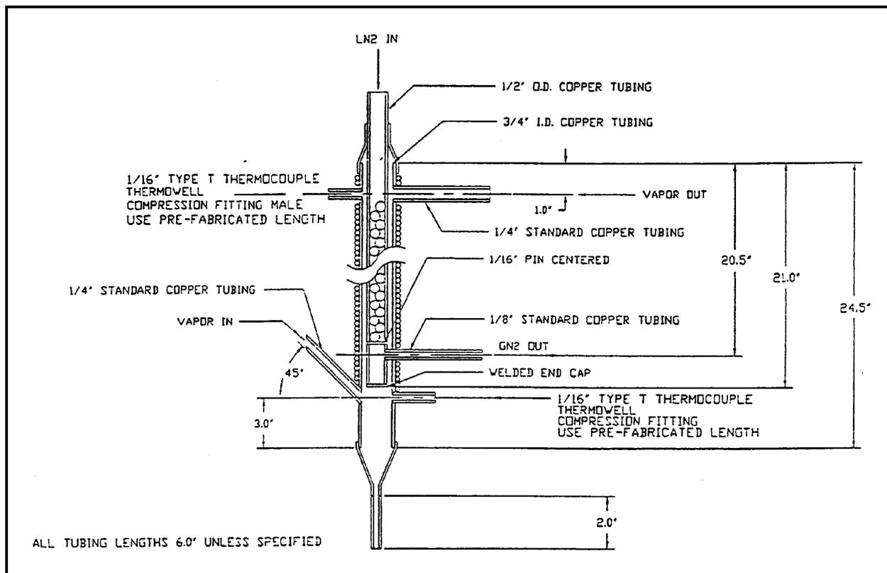
Figure 5. Cross-sectional view of cryogenic condenser.
