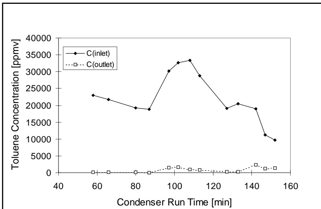
Figure 27. Condenser inlet and outlet toluene concentrations.
