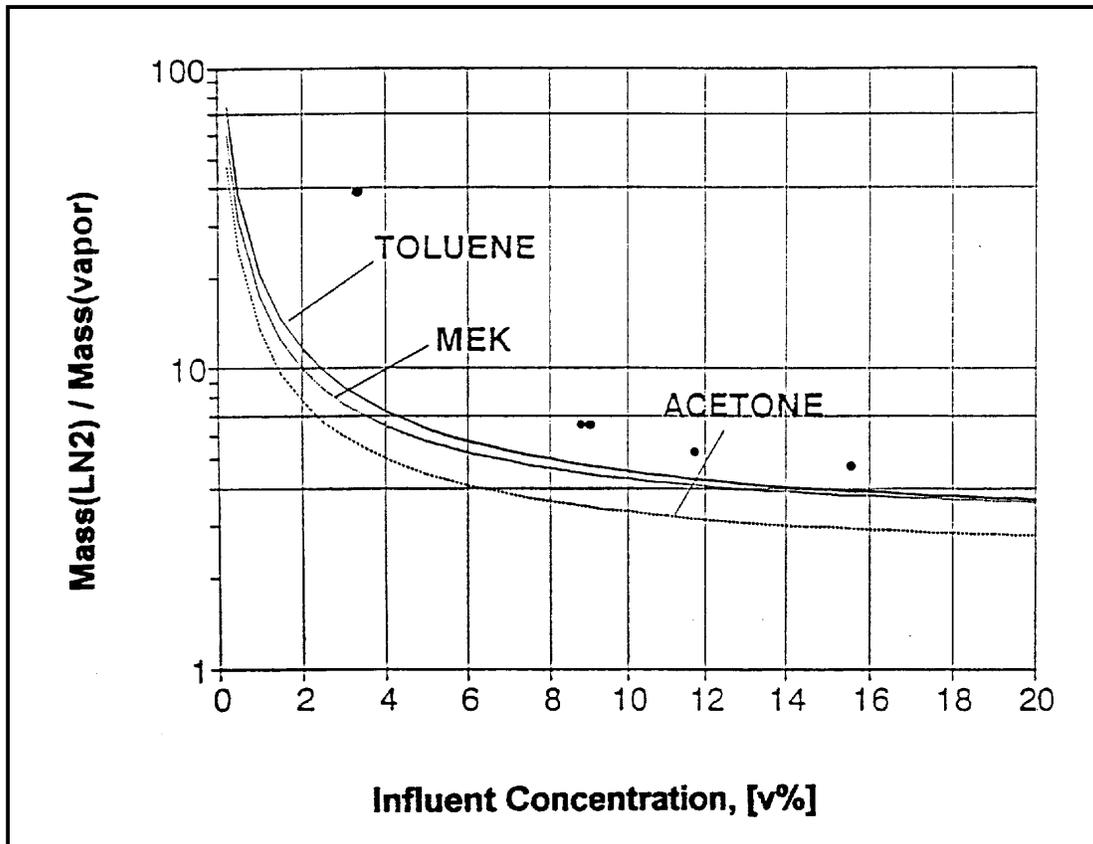
Figure 21. Condenser LN<sub>2</sub> consumption vs. TVOC concentration.
