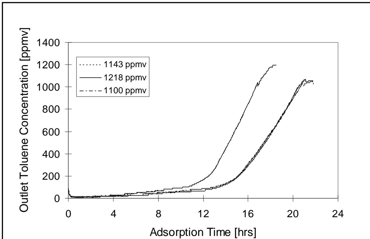
Figure 13. Adsorption breakthrough results for toluene in dry air.
