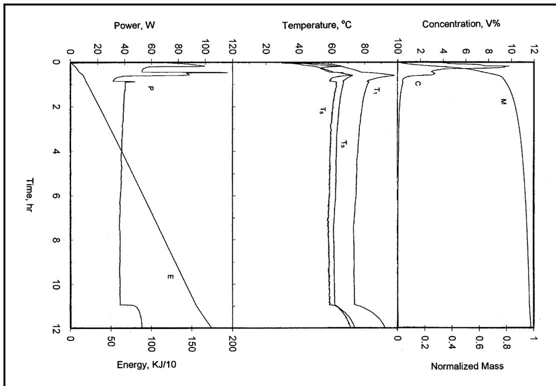
Figure 17. Desorption results for single component MEK.
