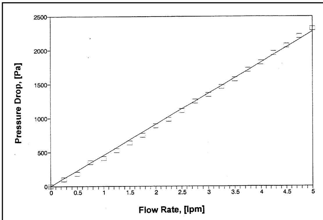
Figure 9. Pressure drop through the ACFC fixed-bed vs. flow rate.
