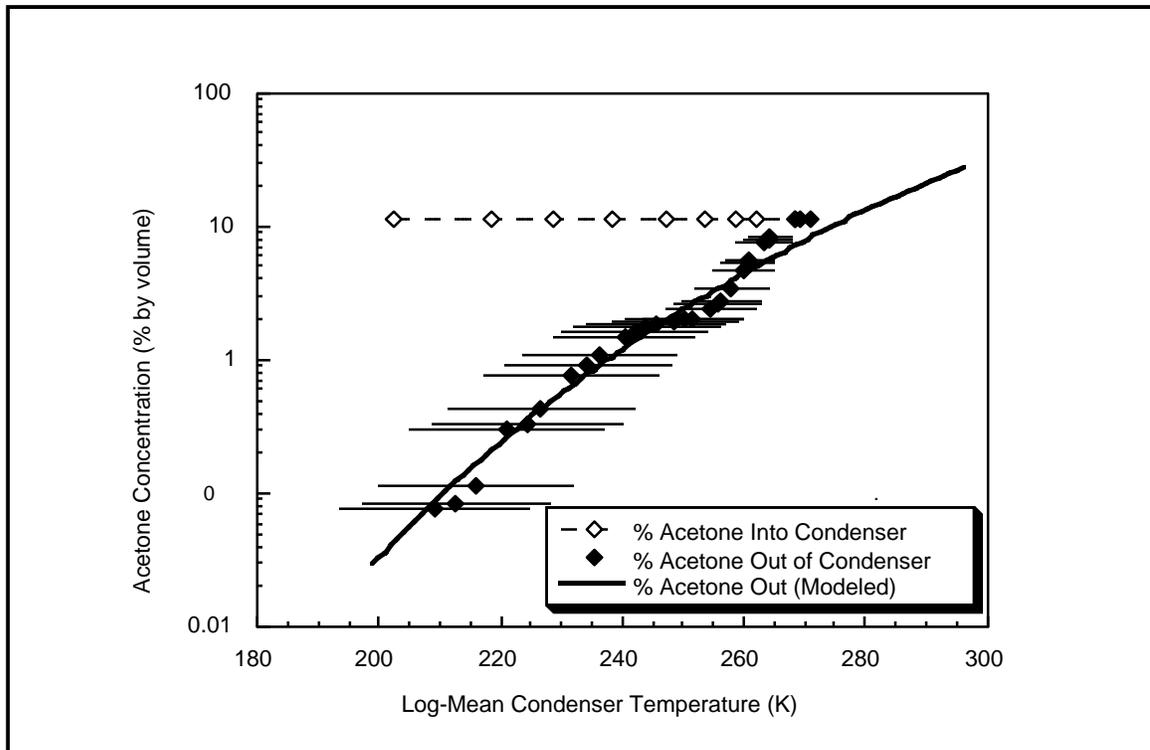
Figure 23. Inlet and outlet acetone concentrations vs. condenser temperature.
