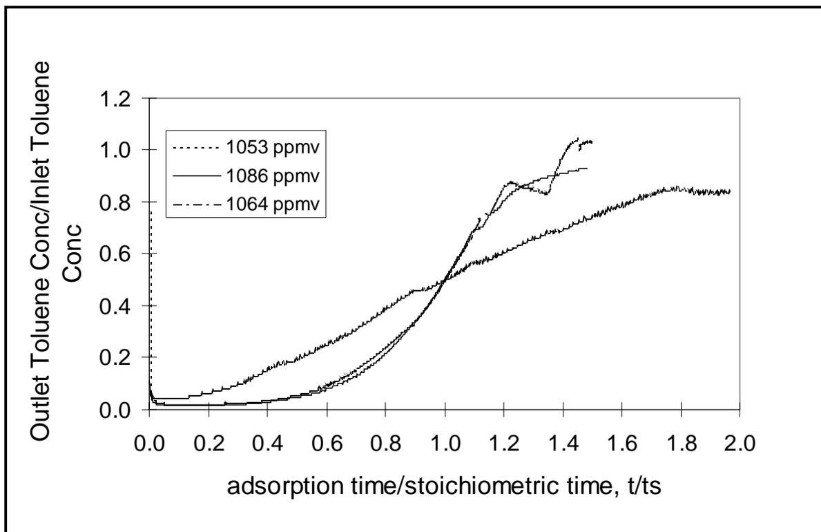
Figure 16. Normalized breakthrough results for toluene in humid air.
