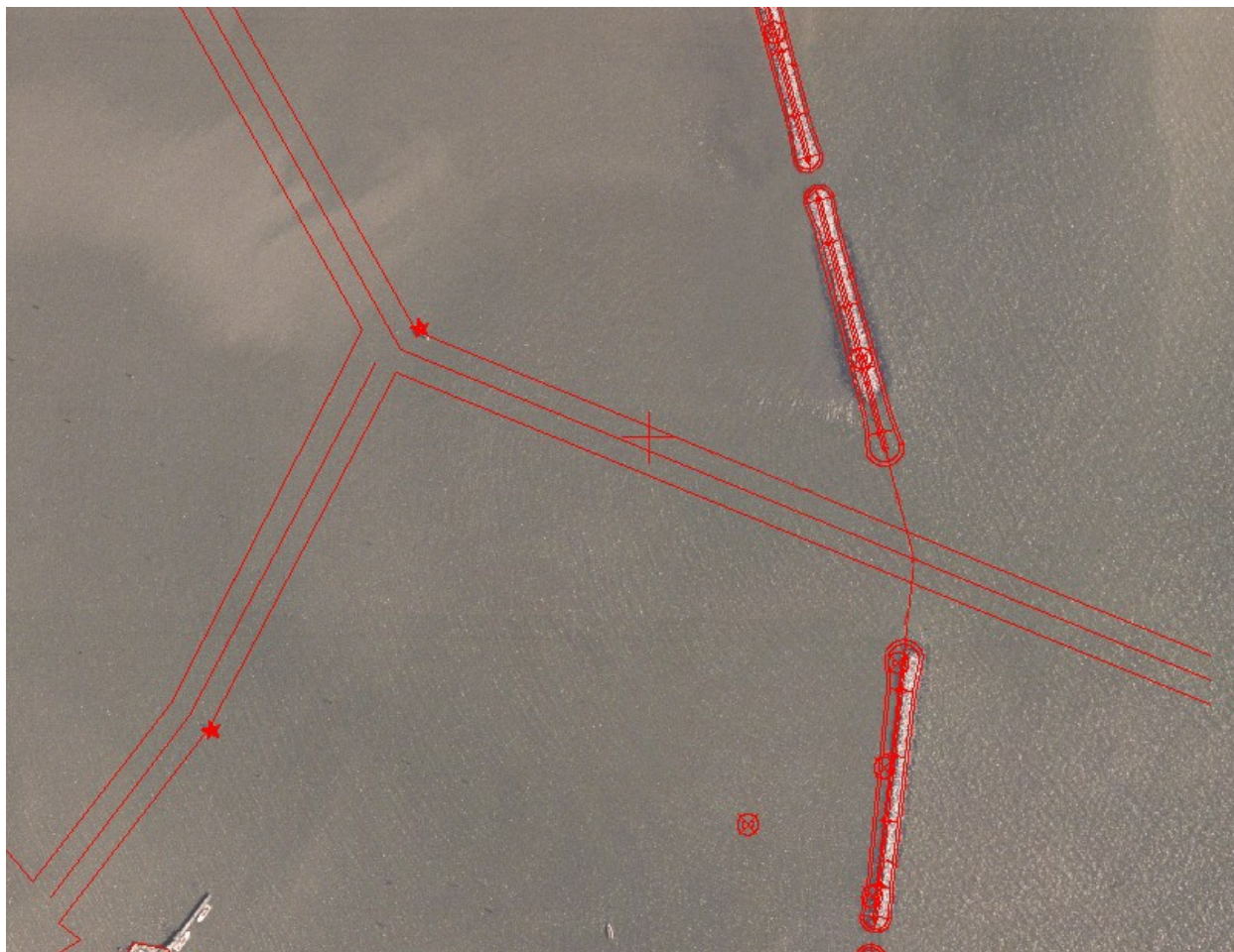
Figure 11. Schematic of existing breakwater configuration (121.9-m (400-ft) gap) versus red outline of authorized breakwater alignment (91.4-m (300-ft) gap) with respect to channel outline
