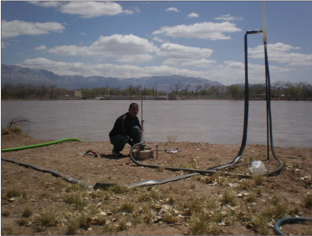
Figure 1. Photograph of submerged jet apparatus being used near San Juan Chama Drinking Water Project diversion dam. Submergence tank is in middle of photograph with standpipe used to generate constant head to right.
