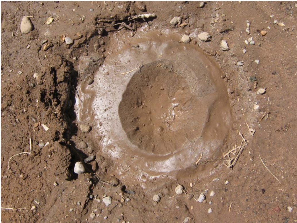
Figure 2. Observed scour at conclusion of test using submerged jet erosion apparatus.
