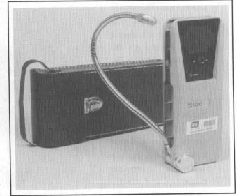
film. If halogen gas is present, it is absorbed onto the film and an electrical current passes through the film. A semipermeable membrane, wrapped around an electrode, accepts only halogen ions to the negative pole cathode. The conductance created is an indication of the halogen gas present.
