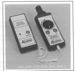
created. Because ultrasound comprises any sound above 20 kHz, it cannot be heard by the human ear. The Amprobe ULD-100 converts this ultrasound into an audible frequency.
