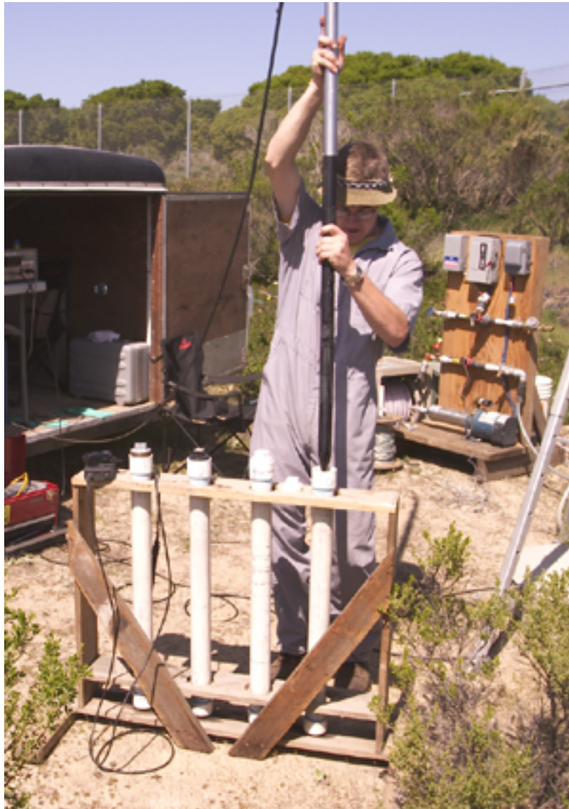
Figure 5. Calibration of the Hydrophysical logging tool with standardized salt solutions.
