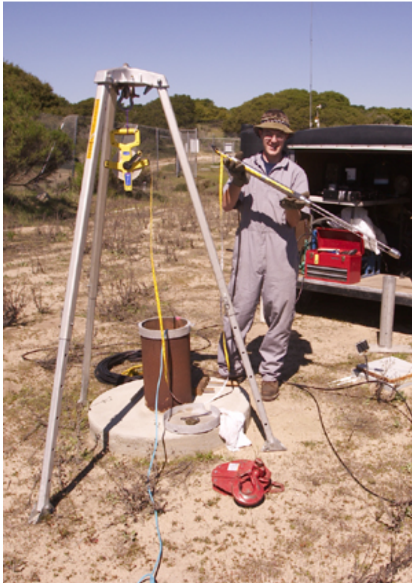
Figure 6. Preparing for installation of the LLNL Scanning Colloidal Borescope Flow Meter.
