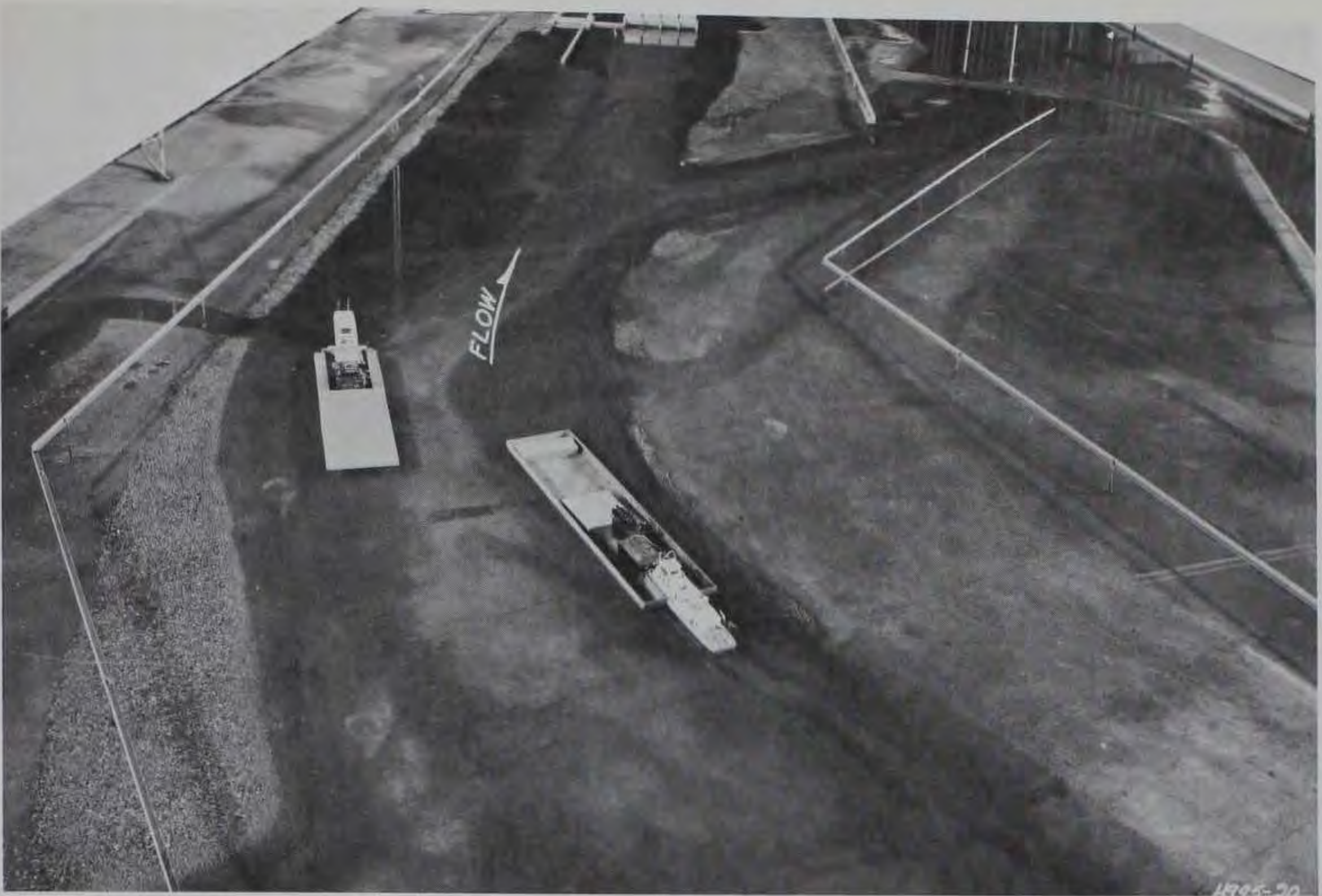
Photo 1. Plan D, 53,000-cfs flow. Relative positions of upbound and downbound tows passing near the upper end of the lock approach channel
