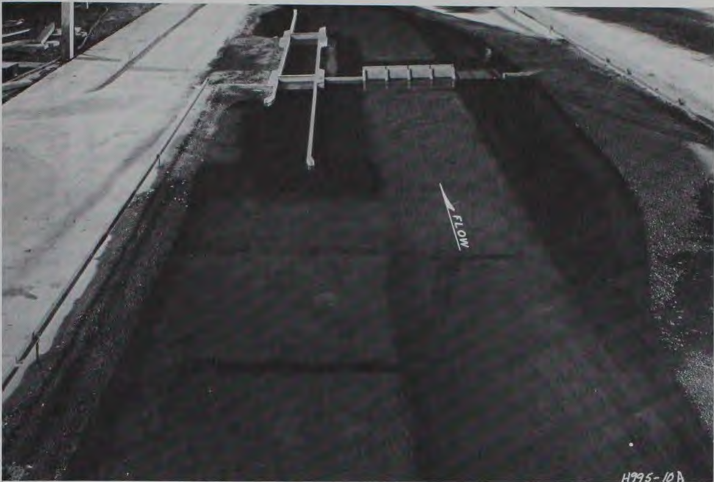
Figure 3. View of the model showing the arrangement of the lock and dam with the original plan
