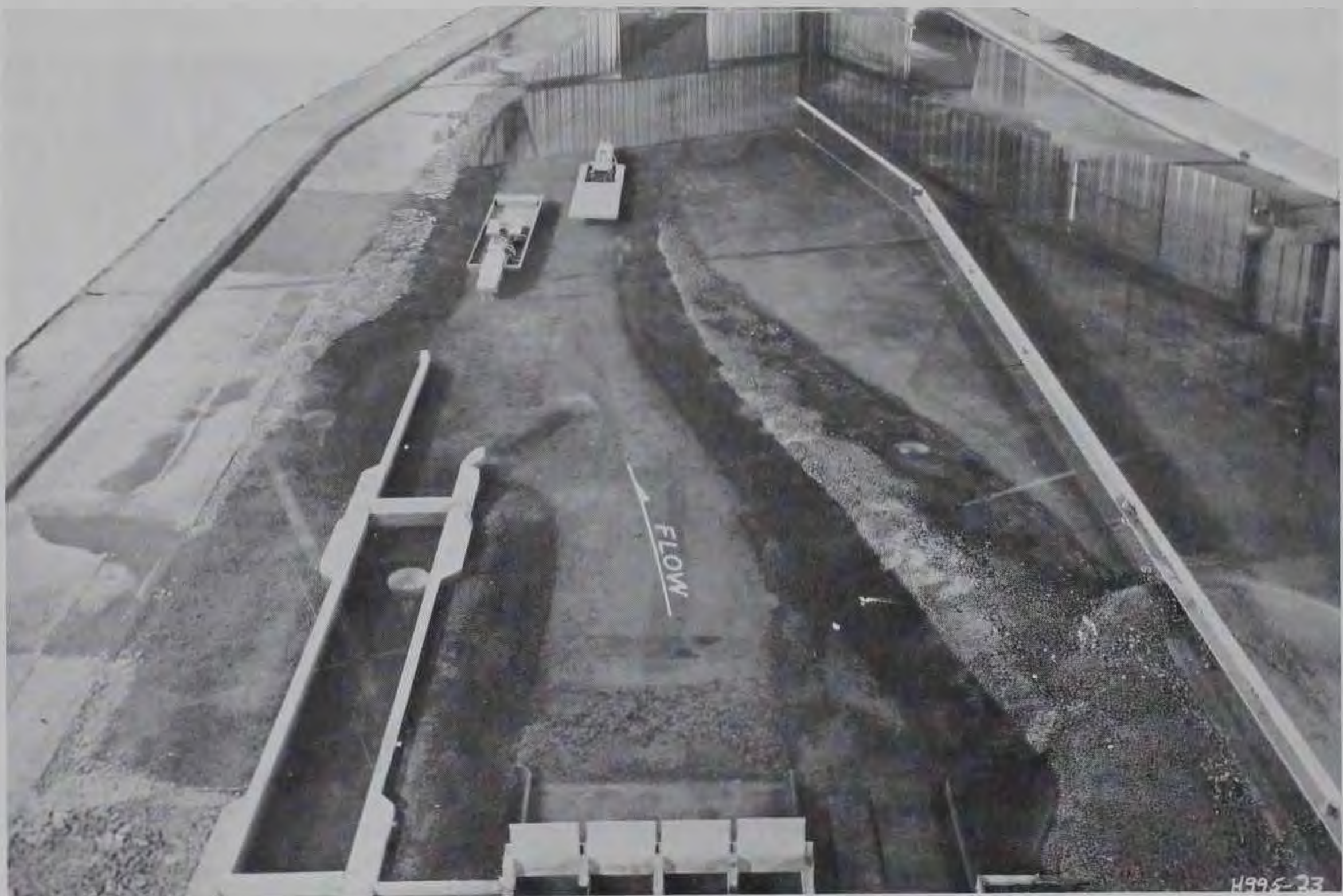
Photo 2. Plan D, 53,000-cfs flow. Relative positions of upbound and downbound tows passing within the lower lock approach
