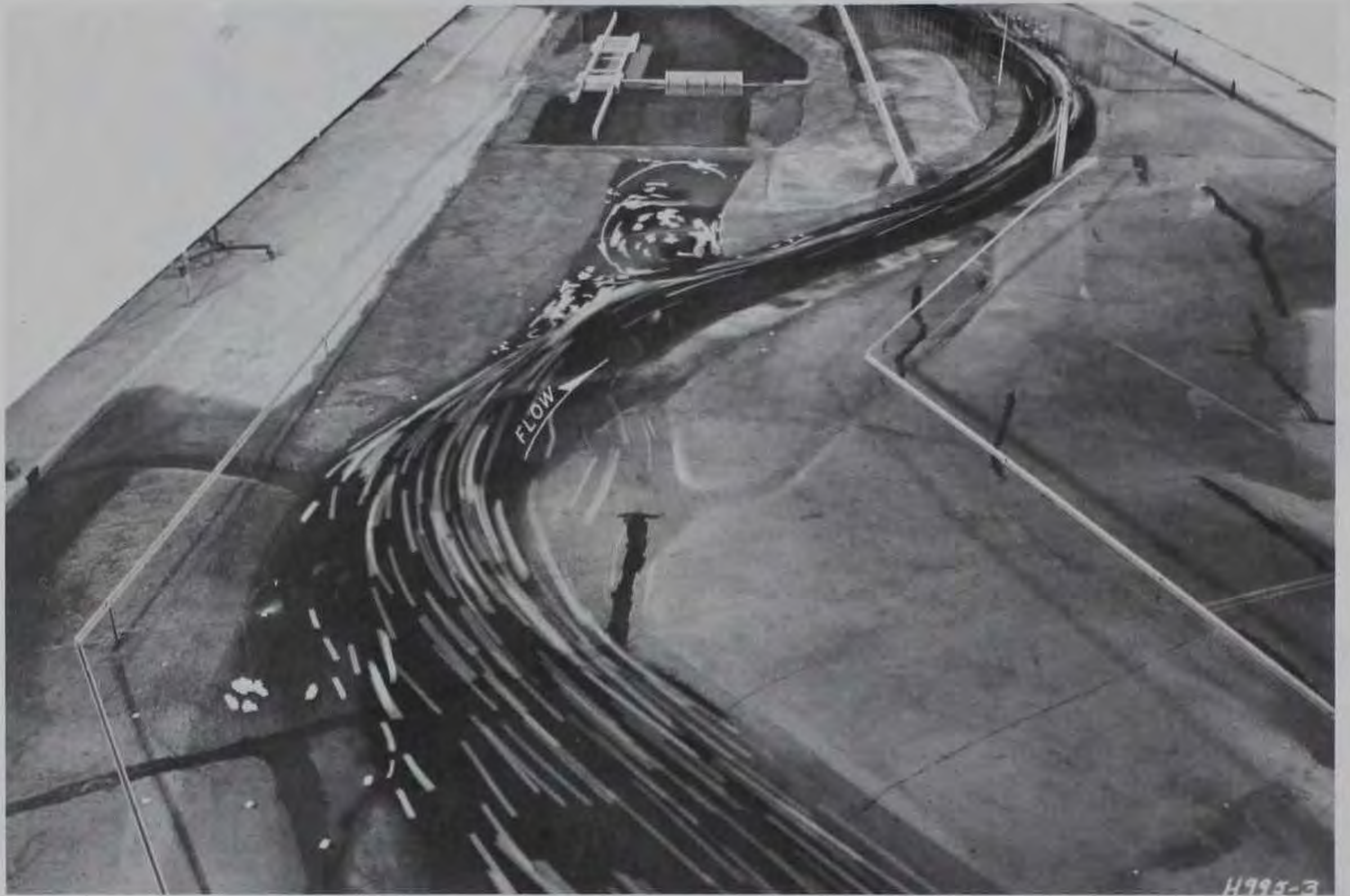
Photo 5. Construction plan, 30,000-cfs flow. Surface currents near the entrance and just downstream of the diversion canal during construction of lock and dam. Note concentration of surface currents along the left bank near the upper end of diversion canal
