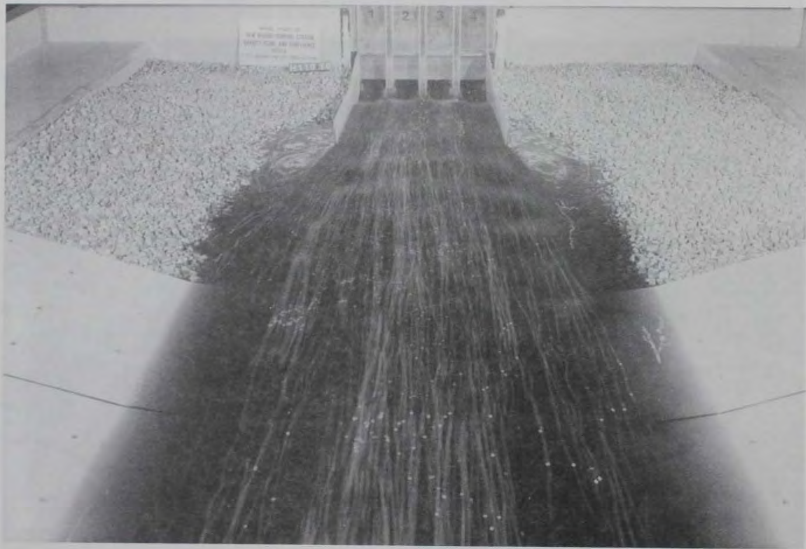
Photo 8. Surface flow pattern, gravity flow stilling basin, discharge 5,000 cfs, tailwater el 267.4
