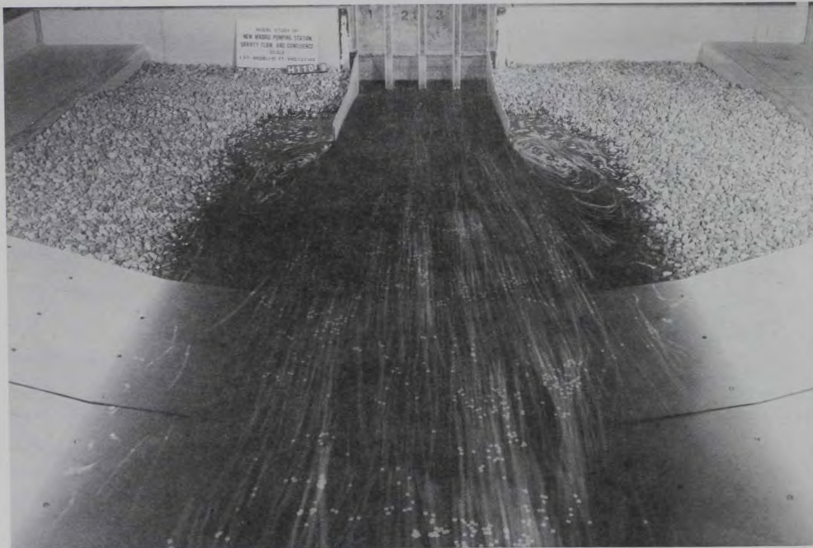
Photo 7. Surface flow pattern, gravity flow stilling basin, discharge 5,000 cfs, tailwater el 270.3
