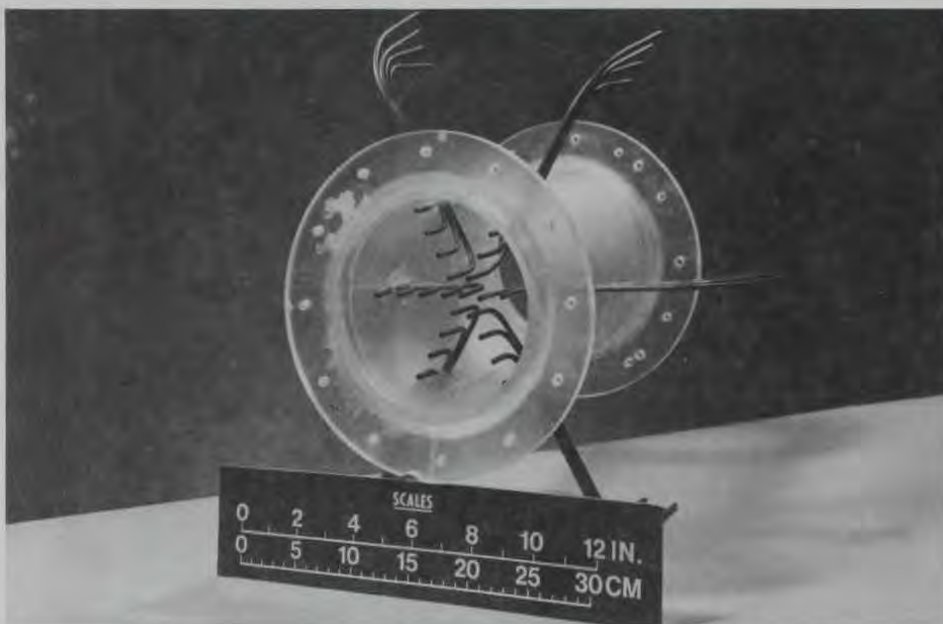
Figure 9. Replacement section of model pump column with impact tubes and static pressure ports
