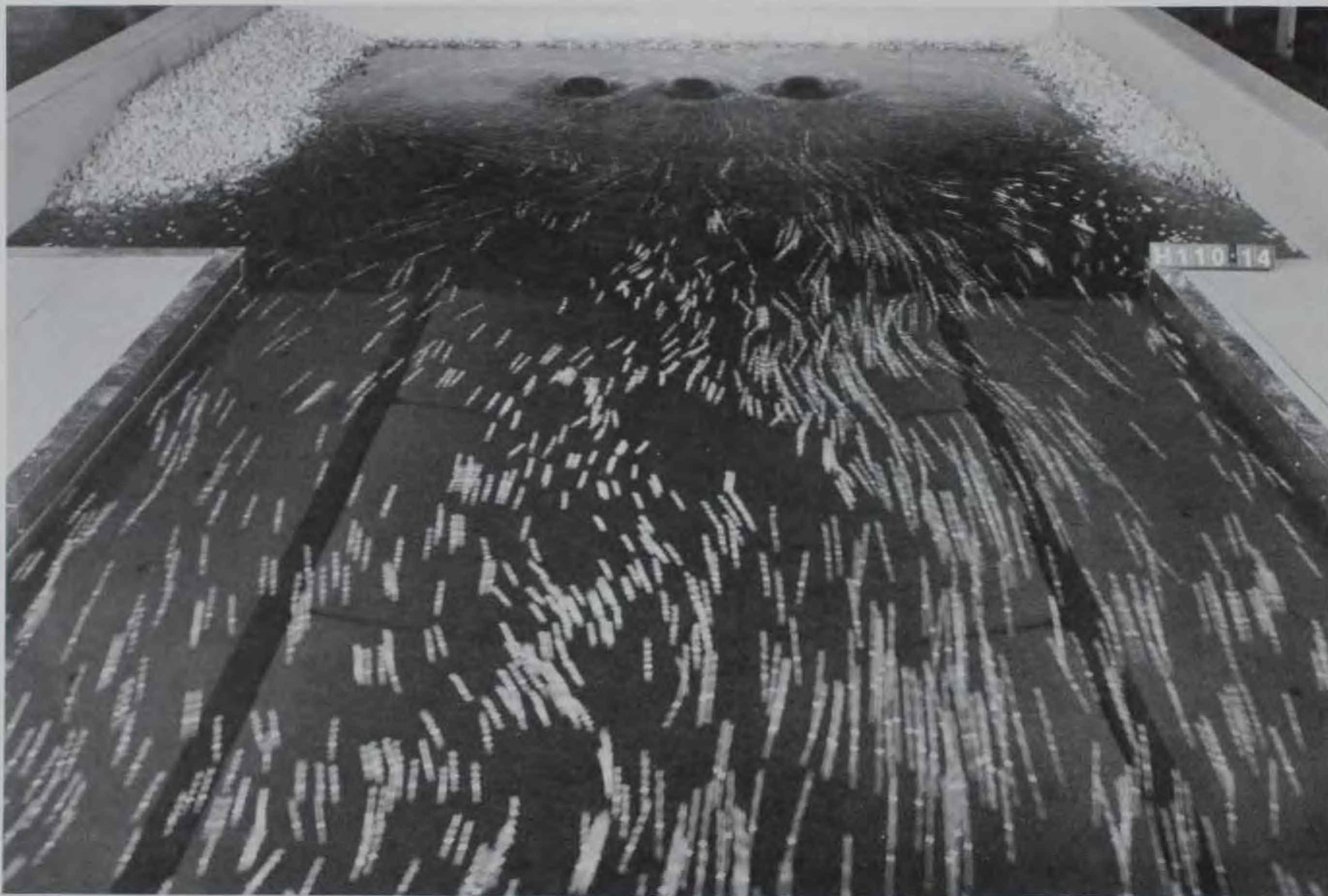
Photo 14. Plume and surface patterns, saxophone outlet operating, discharge per pump 333 cfs, tailwater el 290.0
