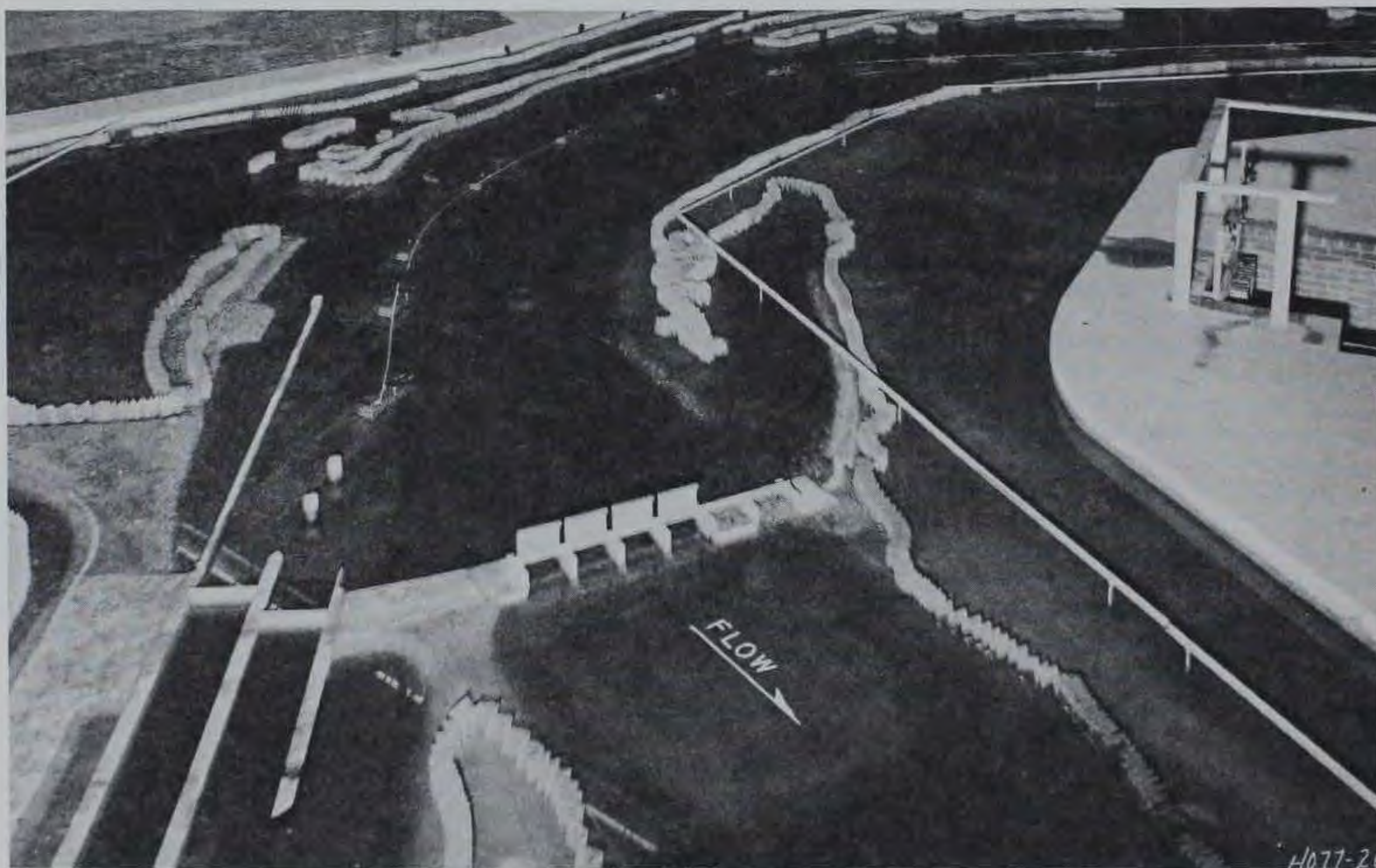
b. Path of downbound 600-ft tow approaching extended guide wall at a slight angle to wall. Note tendency for tow to be rotated clockwise
