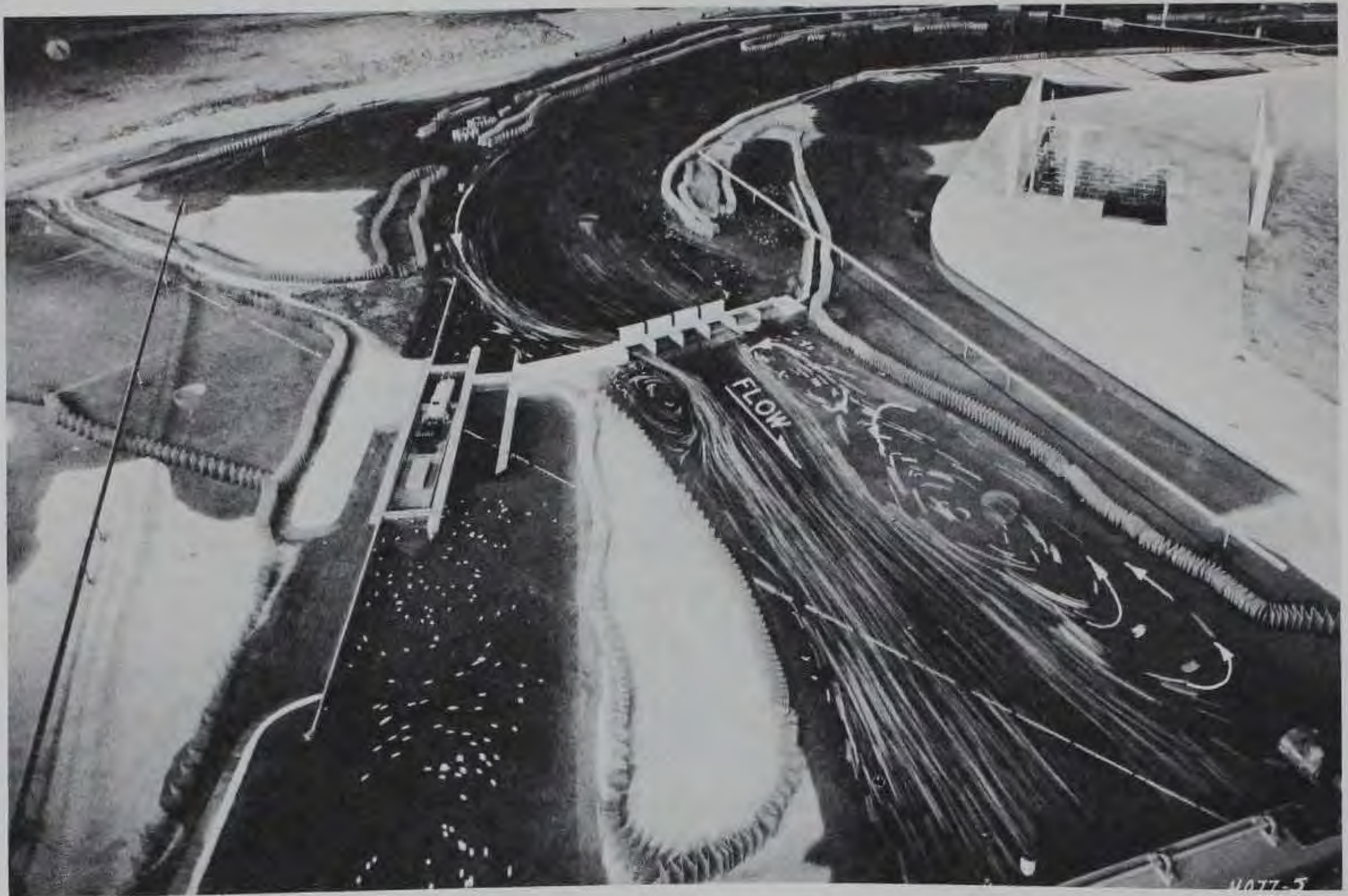
a. Surface currents in lock approach and in approach to gated dam
