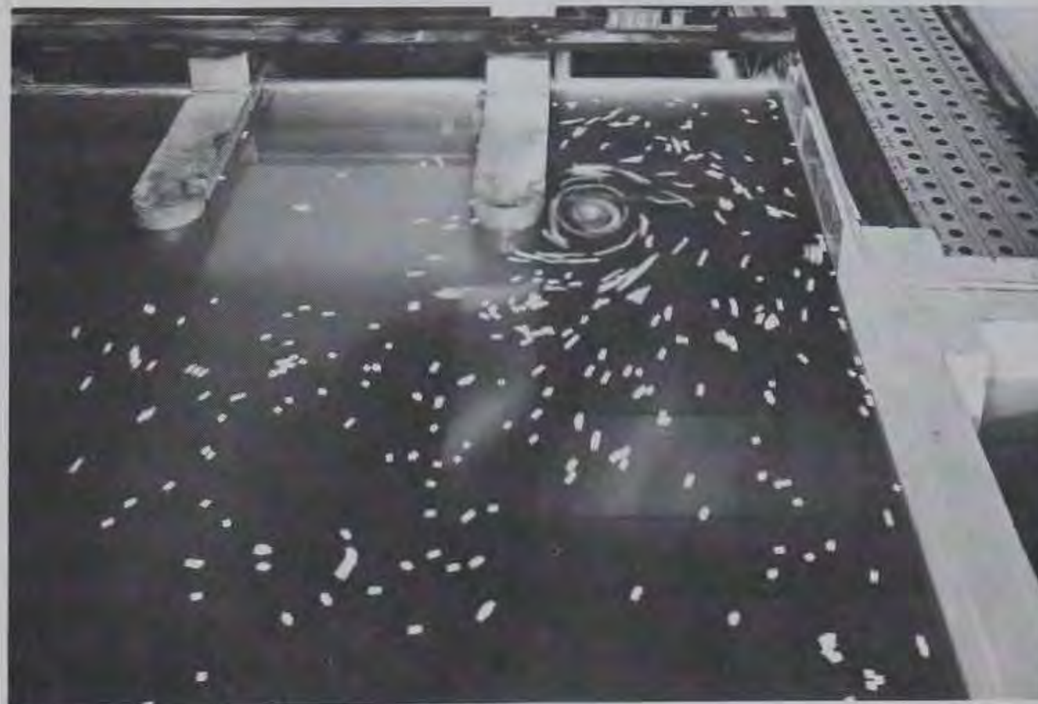
Photo 2. Surface currents during steady-flow peak discharge conditions at type 1 (original) intake, time exposure 5 sec, culvert valve fully open; upper pool el 750.0, lock chamber el 732.0
