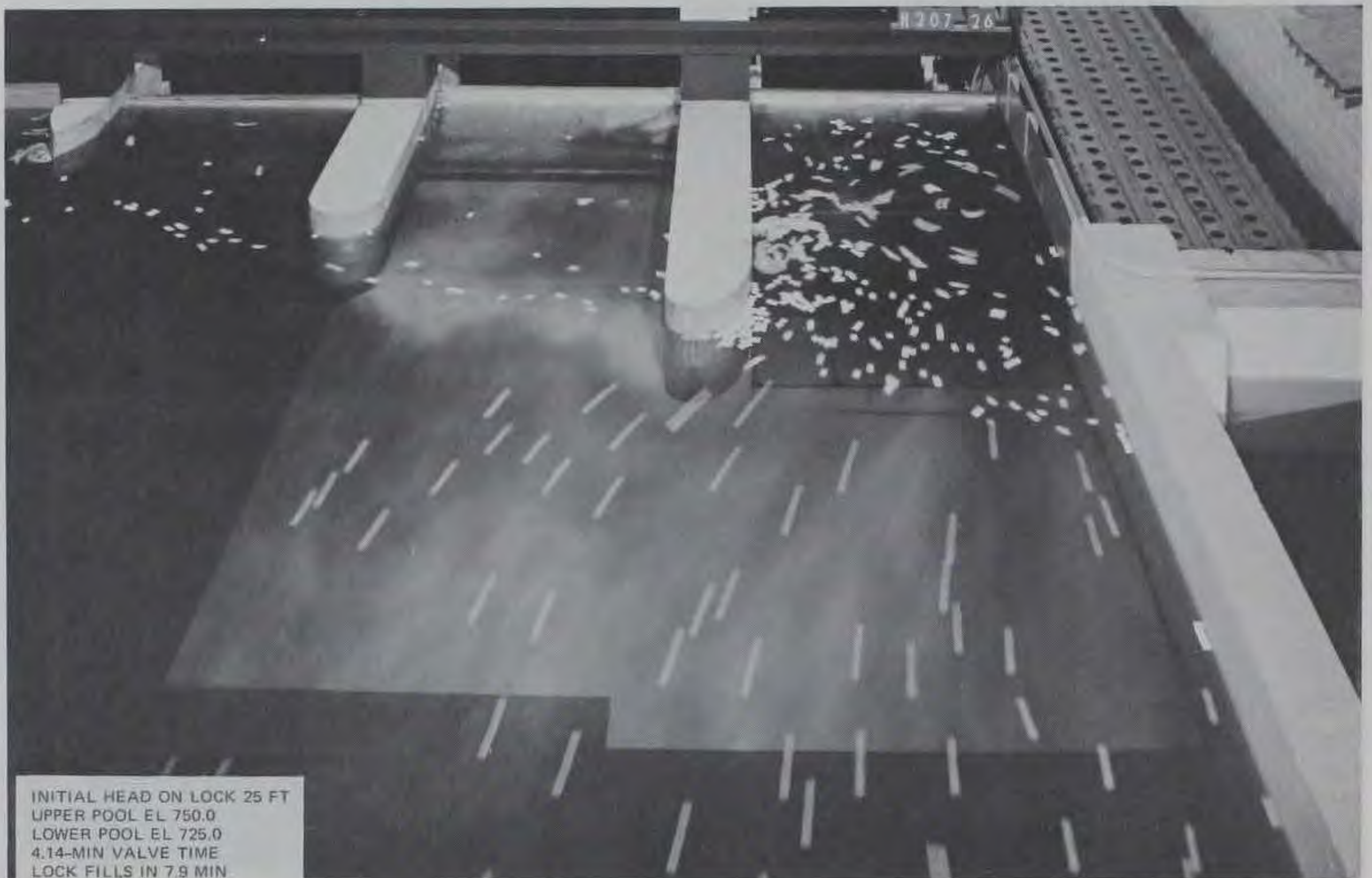
Photo 8. Type 5 (recommended) design, steady-flow peak discharge conditions through intake, time exposure 5 sec, culvert valve fully open; river discharge 5,000 cfs, discharge exceeded 47 percent of time; dam gates 1 and 2 open 1.5 ft, auxiliary lock gate closed
