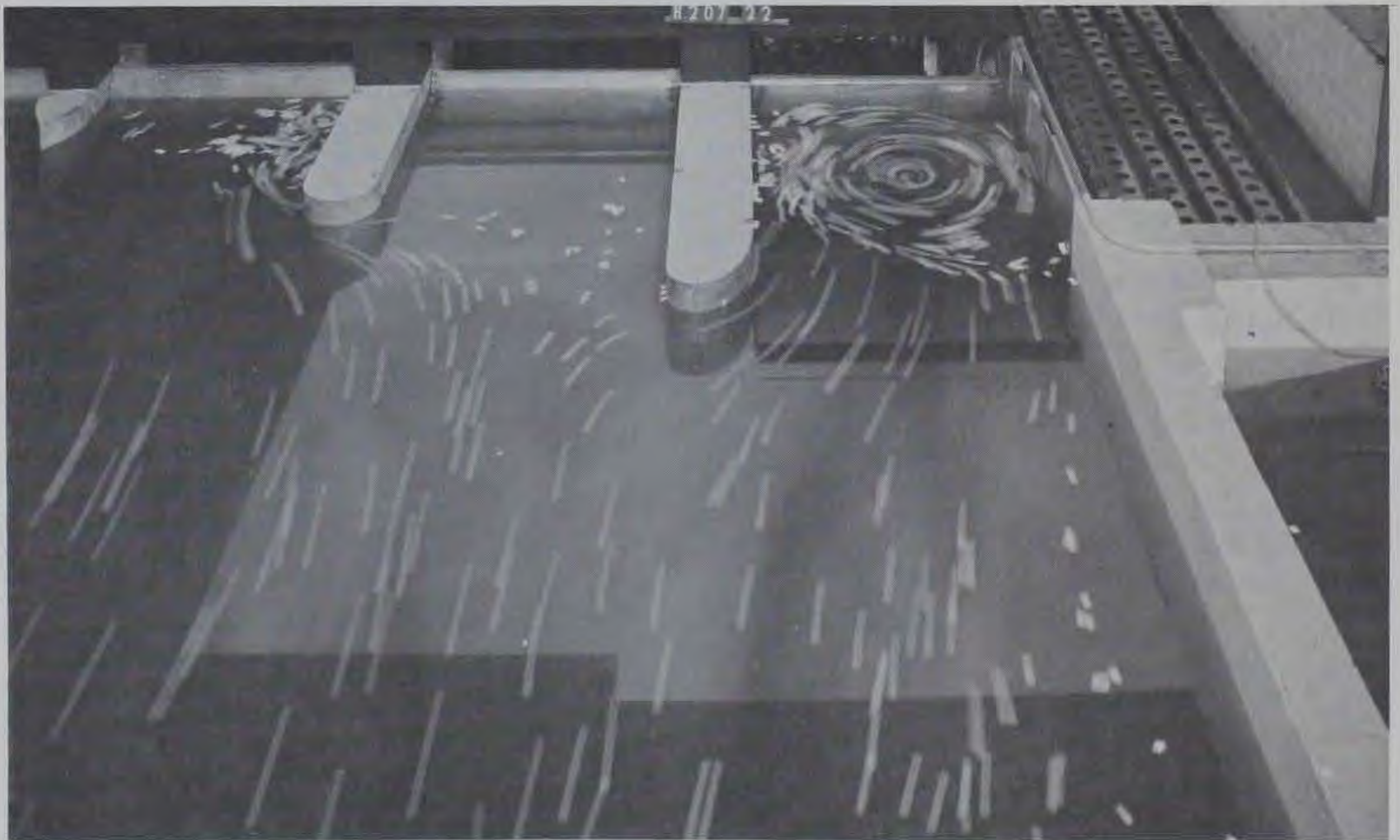
Photo 5. Surface currents during steady-flow peak discharge conditions through intake, type 3 design, culvert valve fully open; upper pool el 750.0, lock chamber el 732.0, auxiliary lock gate closed. Dam gates 1 and 2 open 3 ft, each gate passing 4,920-cfs discharge; dam gate 3 open 3.2 ft, passing 5,230-cfs discharge. Tailgate downstream of dam el 727.0; total discharge through dam approximately 15,070 cfs
