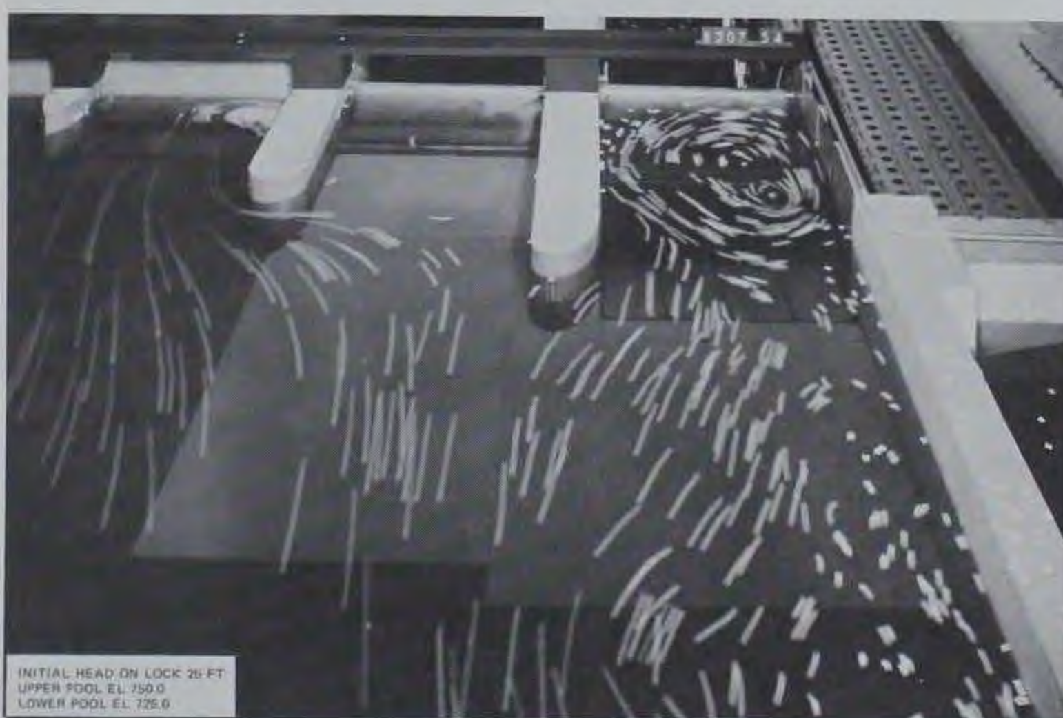
Photo 18. Surface currents during filling operation, type 5 (recommended) design, time exposure 5 sec; river discharge 24,000 cfs, discharge exceeded 4 percent of time, 6.21-min valve time; dam gates 1, 2, and 3 open 5.1 ft, auxiliary lock gate closed (sheet 1 of 2)
