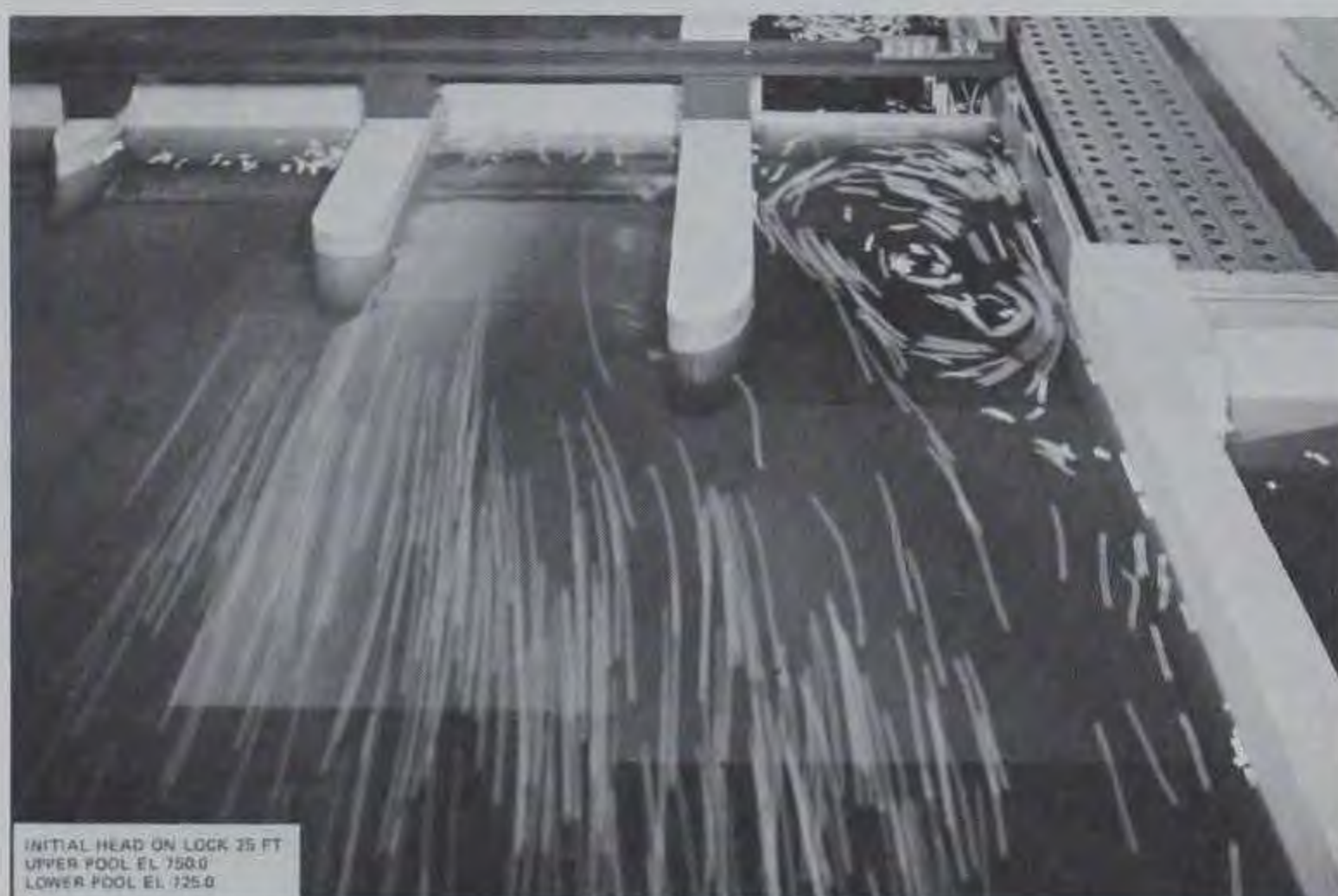
Photo 19. Surface currents during filling operation, type 5 (recommended) design, time exposure 5 sec; river discharge 32,000 cfs, discharge exceeded 1.2 percent of time, 6.21-min valve time; dam gates 1, 2, and 3 open 5.1 ft, auxiliary lock gate open 7.7 ft (sheet 1 of 2)
