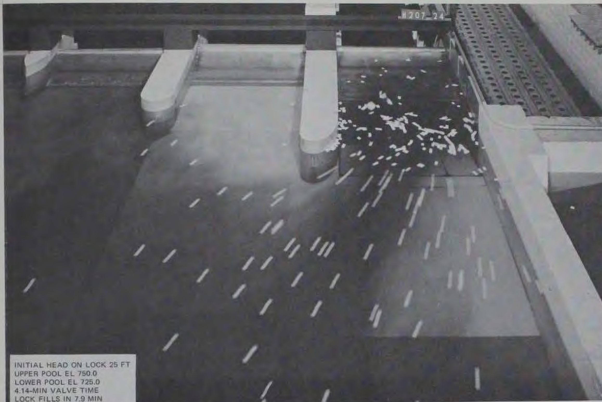
Photo 6. Type 5 (recommended) design, steady-flow peak discharge conditions through intake, time exposure 5 sec, culvert valve fully open; river discharge 0 cfs, discharge exceeded 100 percent of time
