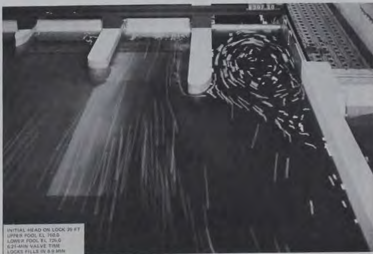
Photo 12. Type 5 (recommended) design, steady-flow peak discharge conditions through intake, time exposure 5 sec, culvert valve fully open; river discharge 32,000 cfs, discharge exceeded 1.2 percent of time; dam gates 1, 2, and 3 open 5.1 ft, auxiliary lock gate open 7.7 ft
