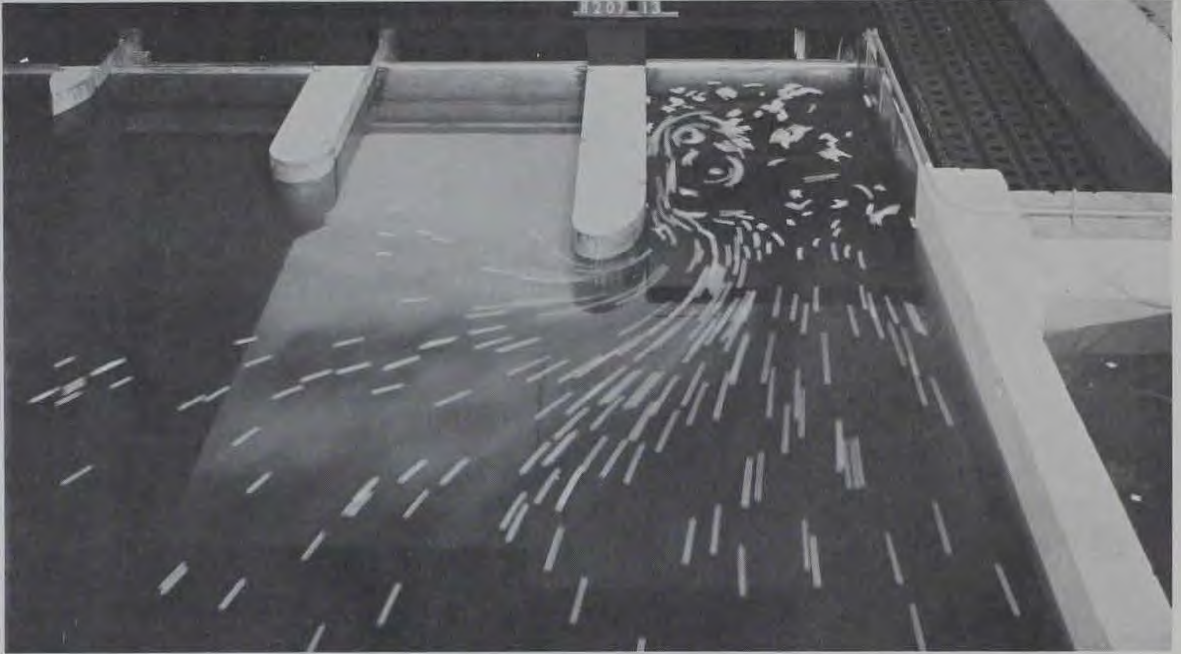
Photo 4. Surface currents during steady-flow peak discharge conditions, type 3 design, time exposure 5 sec; upper pool el 750.0, lock chamber el 732.0, culvert valve fully open
