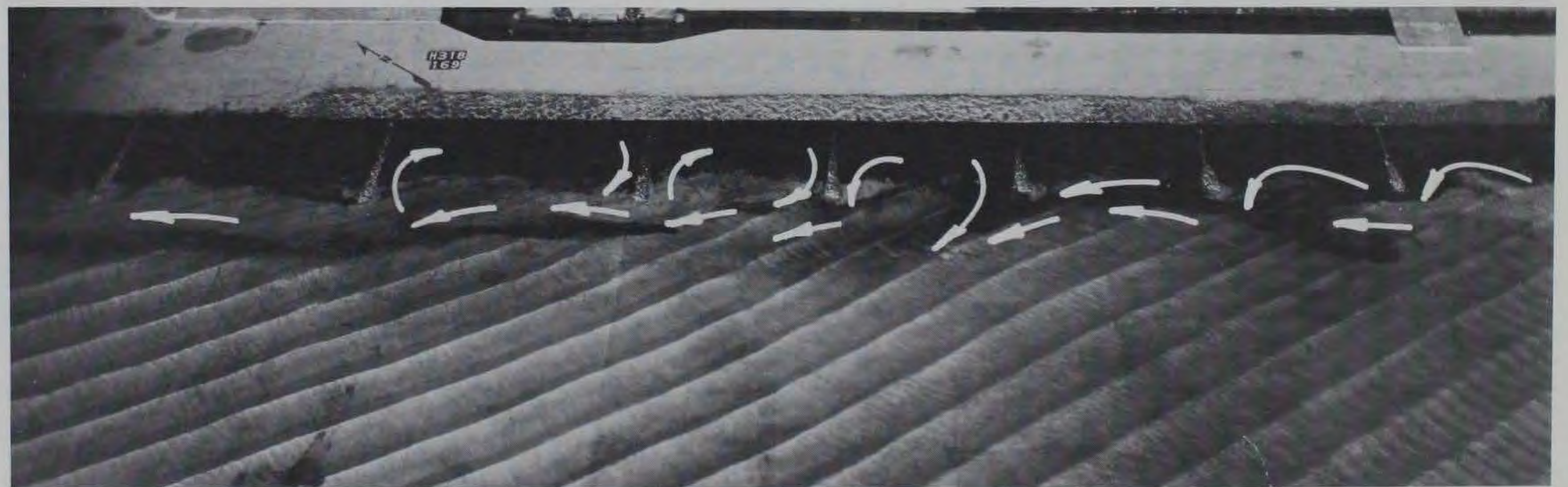
Photo 67. Semimovable-bed tracer deposits for Plan 12 resulting from 9-sec, 10-ft waves from south at mllw
