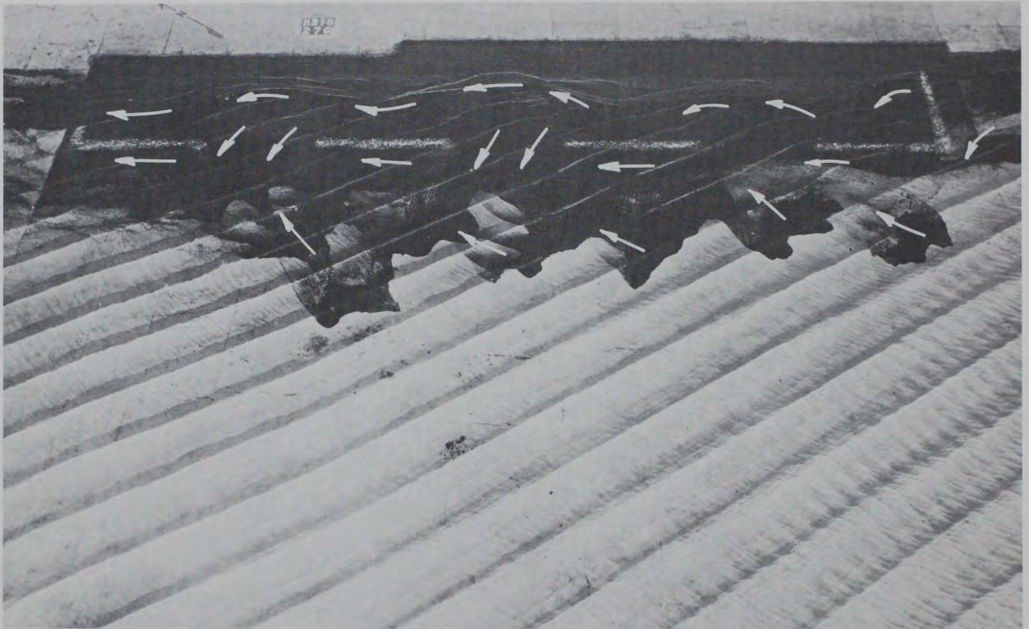
Photo 80. Movable-bed tracer deposits for Plan 15 resulting from 9-sec, 10-ft waves from south at mllw (with coal feed)
