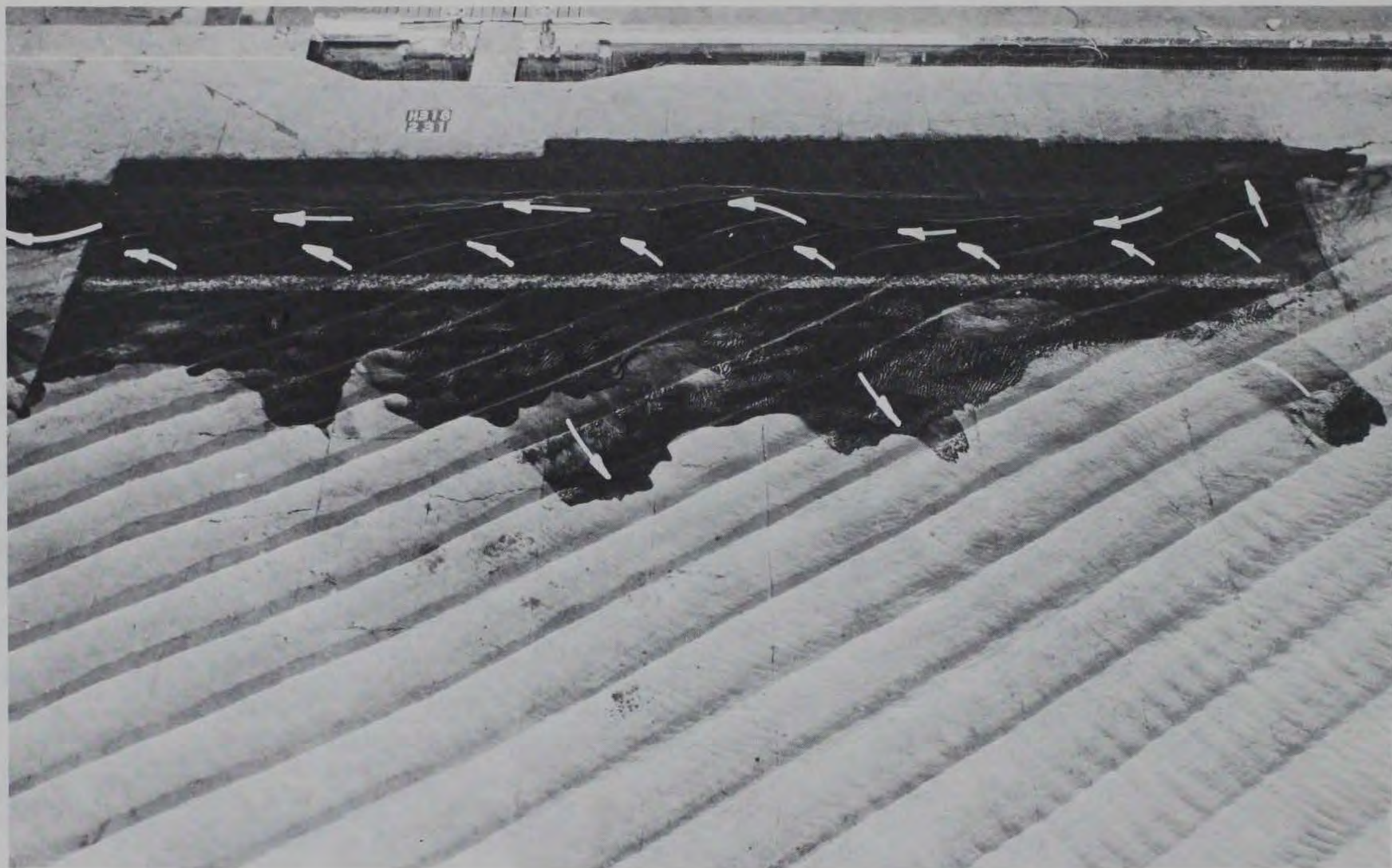
Photo 75. Movable-bed tracer deposits for Plan 13 resulting from 9-sec, 10-ft waves from south at mllw (without coal feed)
