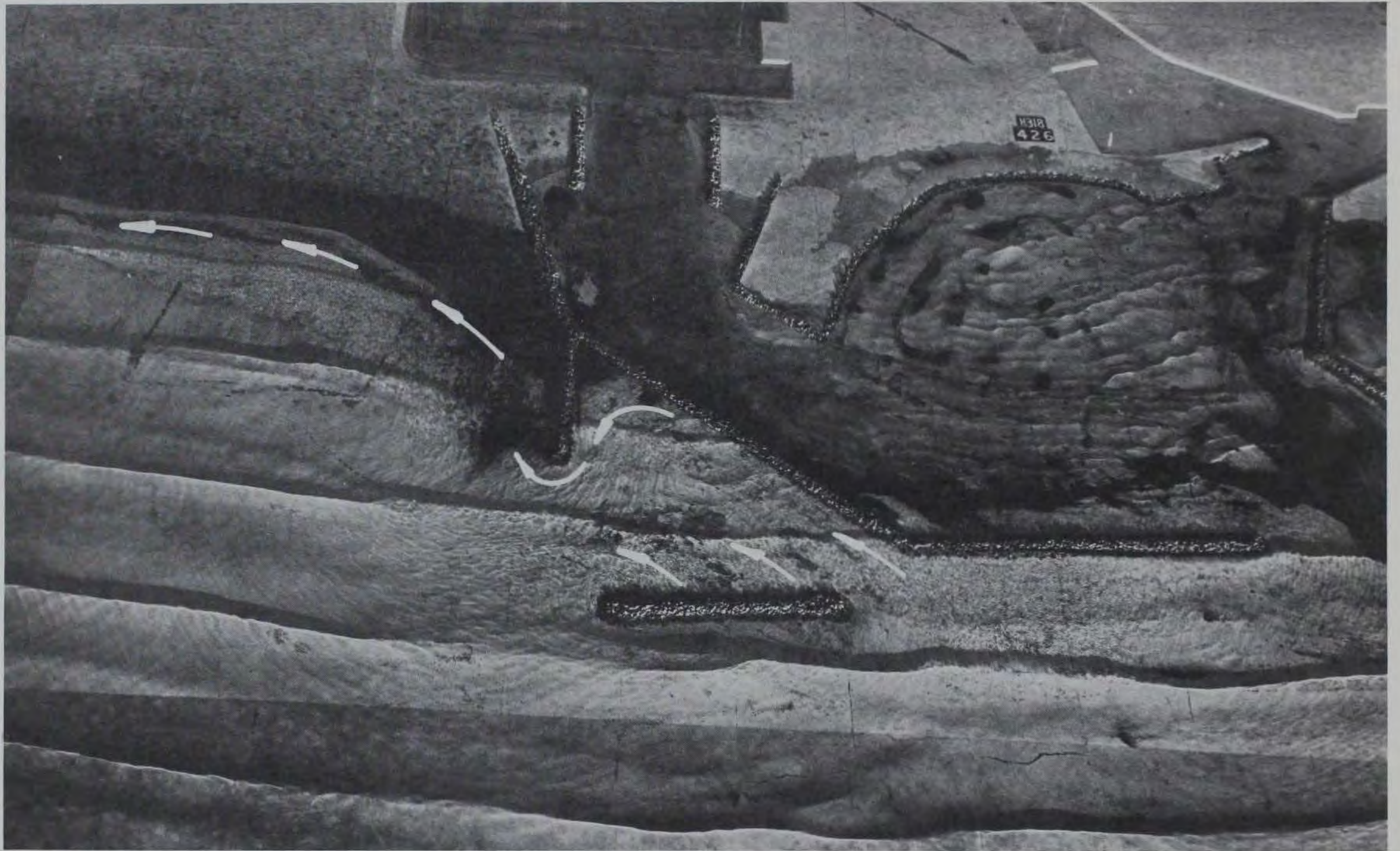
Photo 48. Typical tracer movement for Plan 38C resulting from 17-sec, 10-ft waves from southwest at mhhw (with waves)
