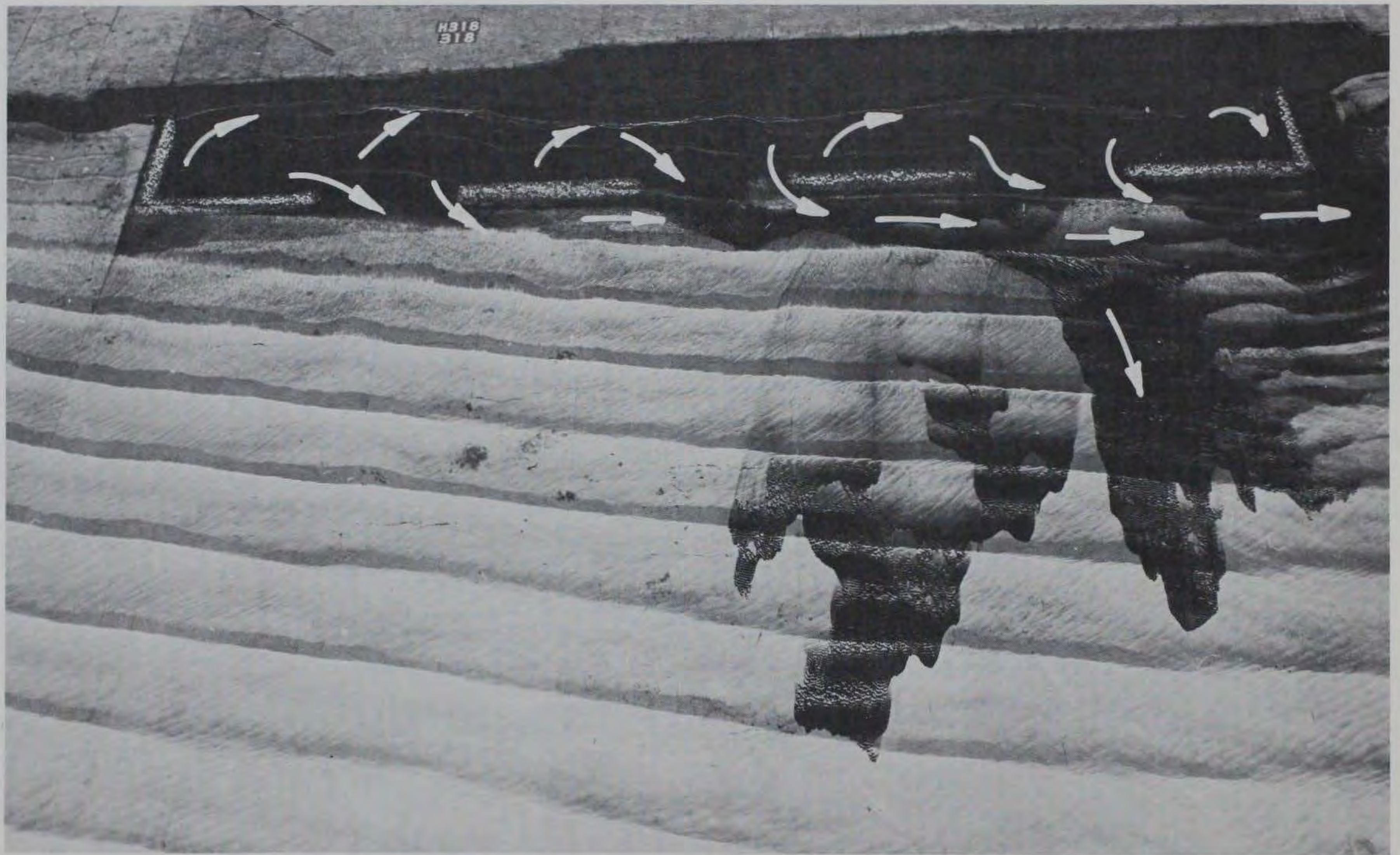
Photo 96. Movable-bed tracer deposits for Plan 17 resulting from 11-sec, 10-ft waves from west at mllw (extended test wave duration)
