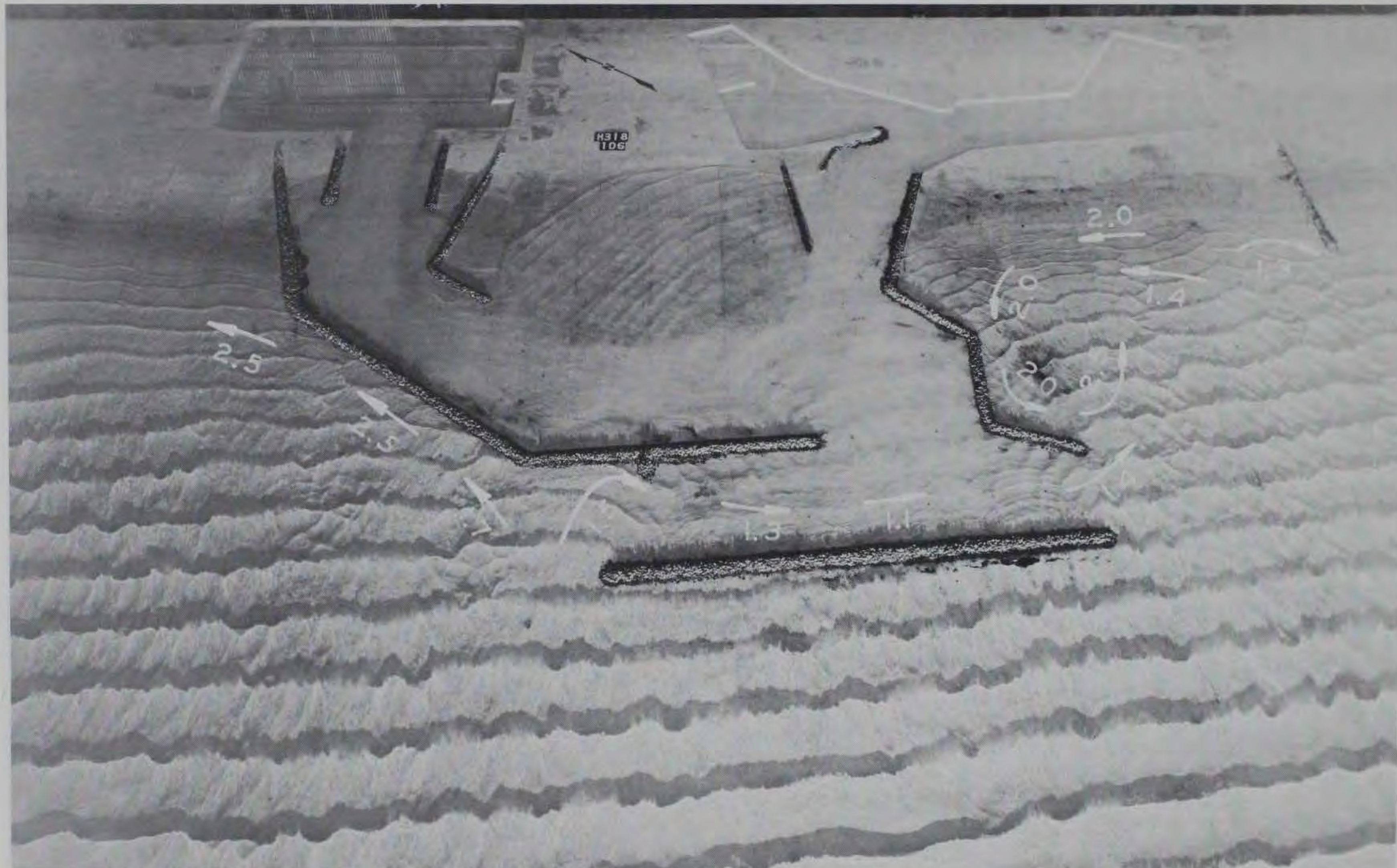
Photo 13. Typical wave and current patterns and current magnitudes (prototype feet per second) for Plan 4; 9-sec, 16-ft waves from southwest at mllw
