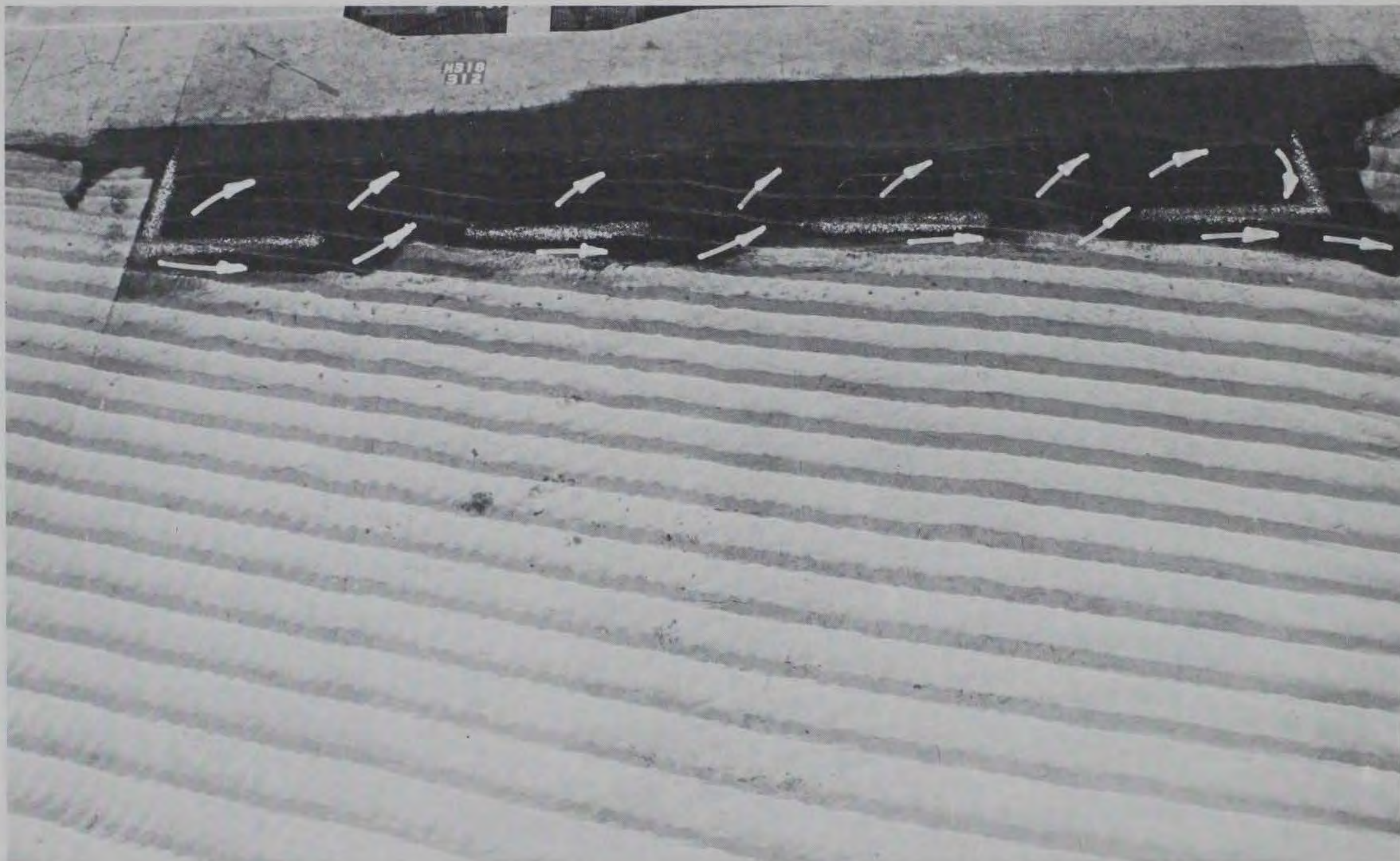
Photo 91. Movable-bed tracer deposits for Plan 17 resulting from 7-sec, 10-ft waves from west at mhw (extended test wave duration)
