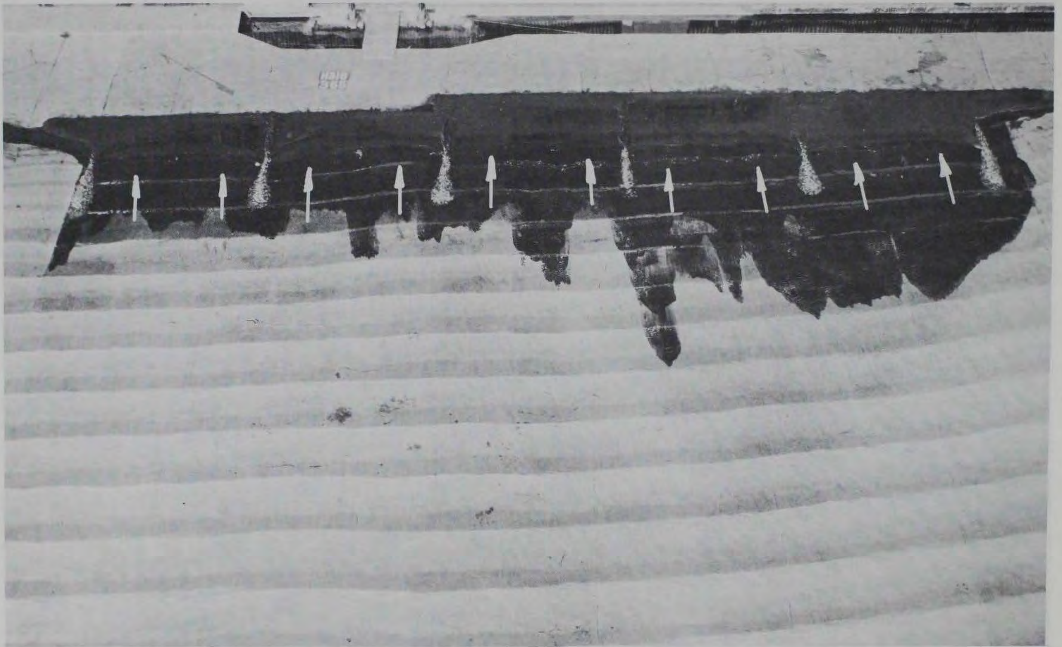
Photo 121. Movable-bed tracer deposits for Plan 9 (with revised beach slope) resulting from 9-sec, 10-ft waves from S55°W at mhhw
