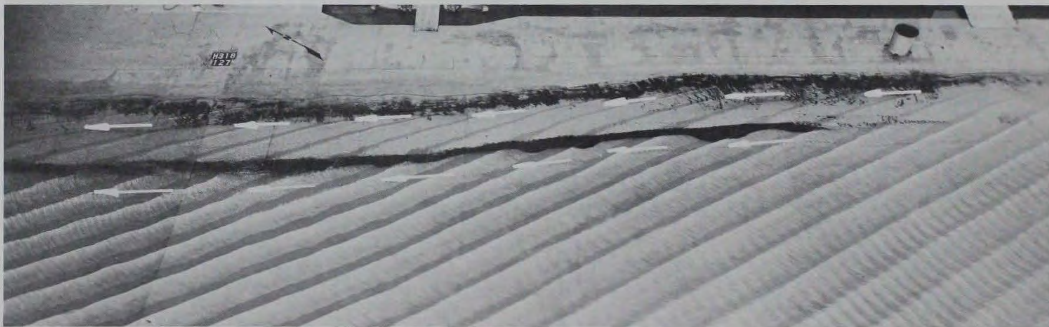
Photo 60. Typical tracer movements for existing conditions resulting from 9-sec, 10-ft waves from south at mllw
