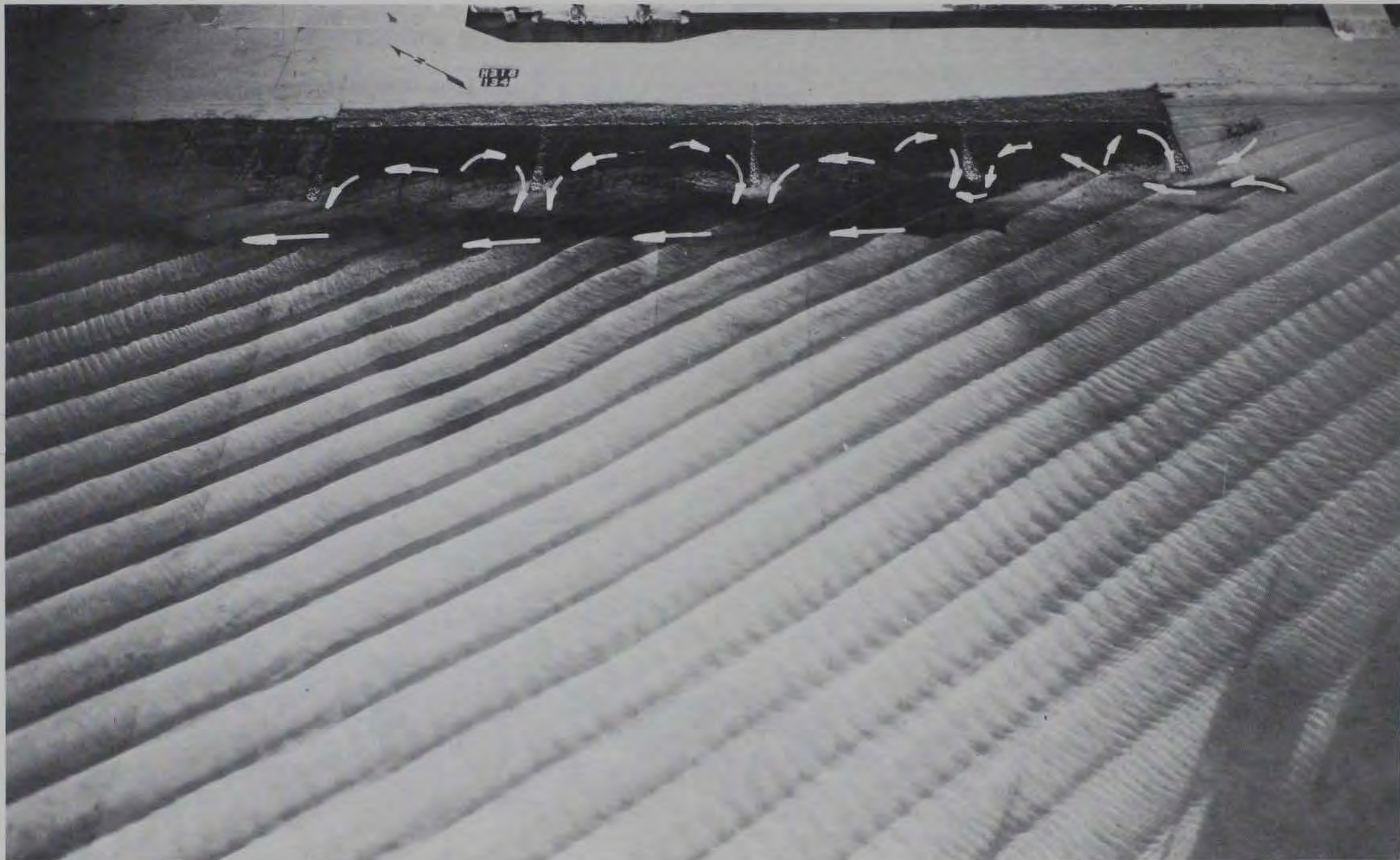
Photo 61. Semimovable-bed tracer deposits for Plan 6 resulting from 9-sec, 10-ft waves from south at mllw
