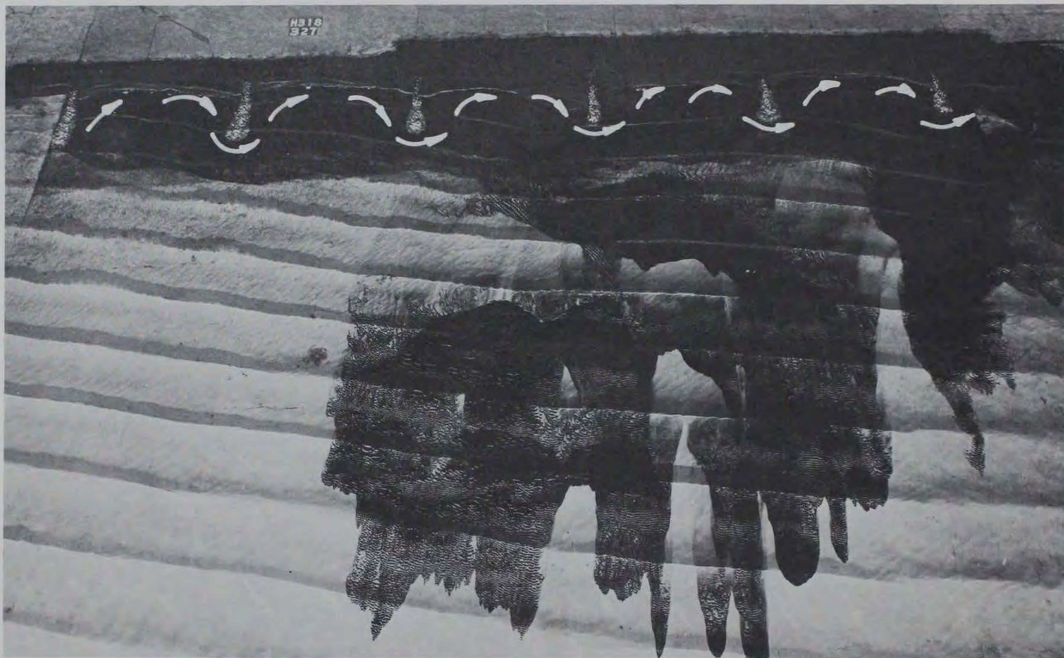
Photo 104. Movable-bed tracer deposits for Plan 18 resulting from 11-sec, 10-ft waves from west at mllw (extended test wave duration)
