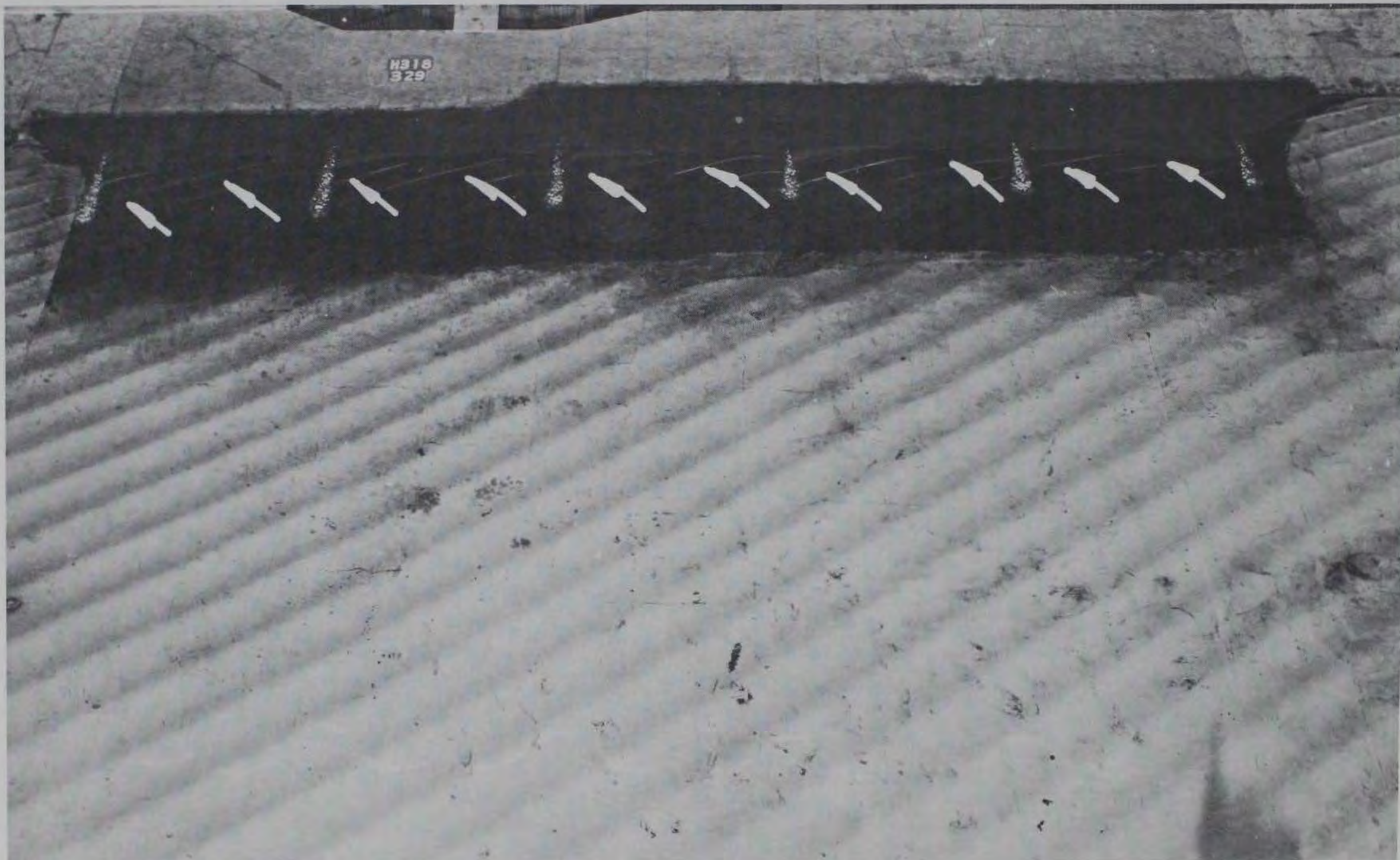
Photo 105. Movable-bed tracer deposits for Plan 18 resulting from 7-sec, 4-ft waves from south at mhw (extended test wave duration)
