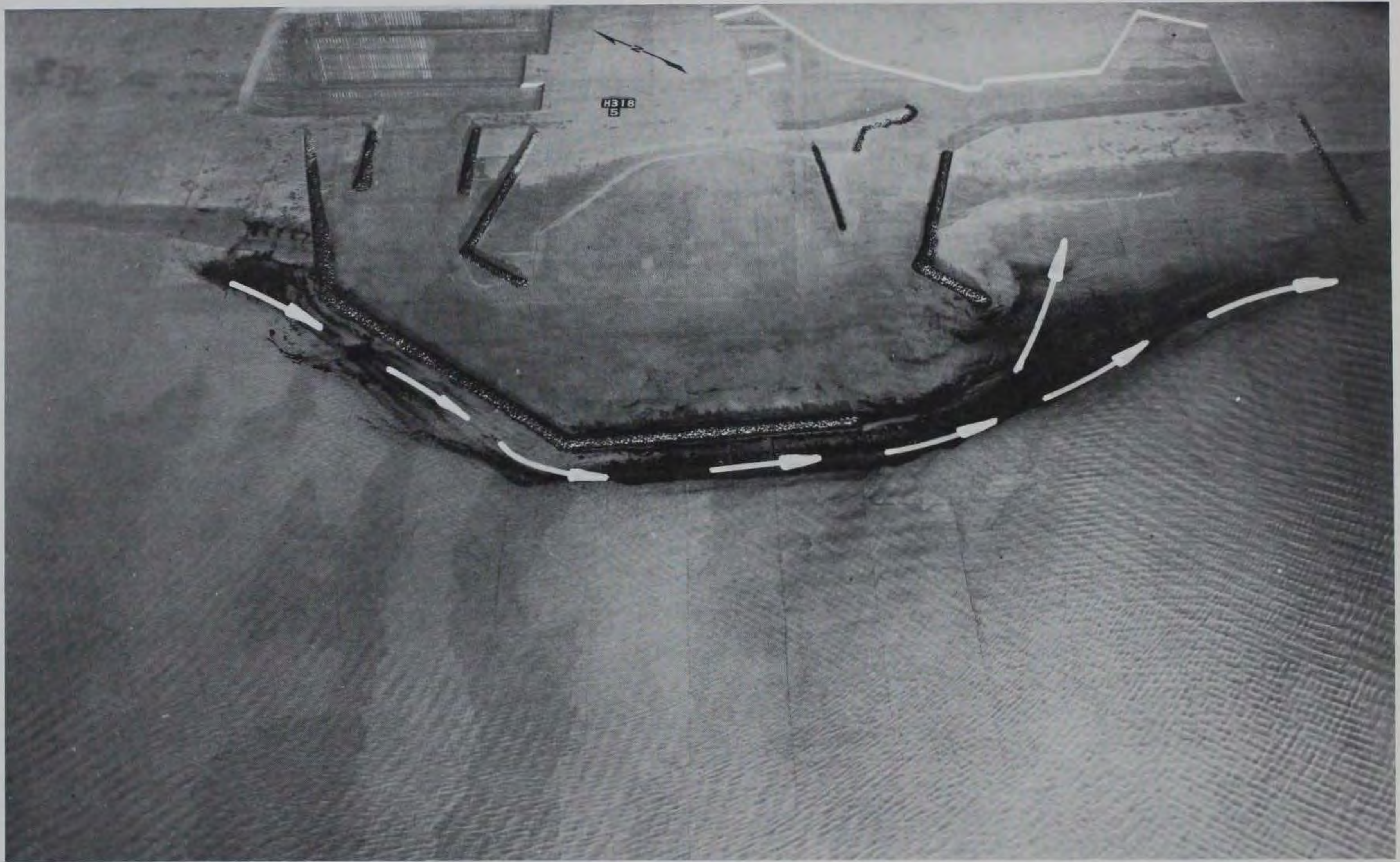
Photo 6. Typical tracer movement for existing conditions resulting from 7-sec, 10-ft waves from northwest at mllw
