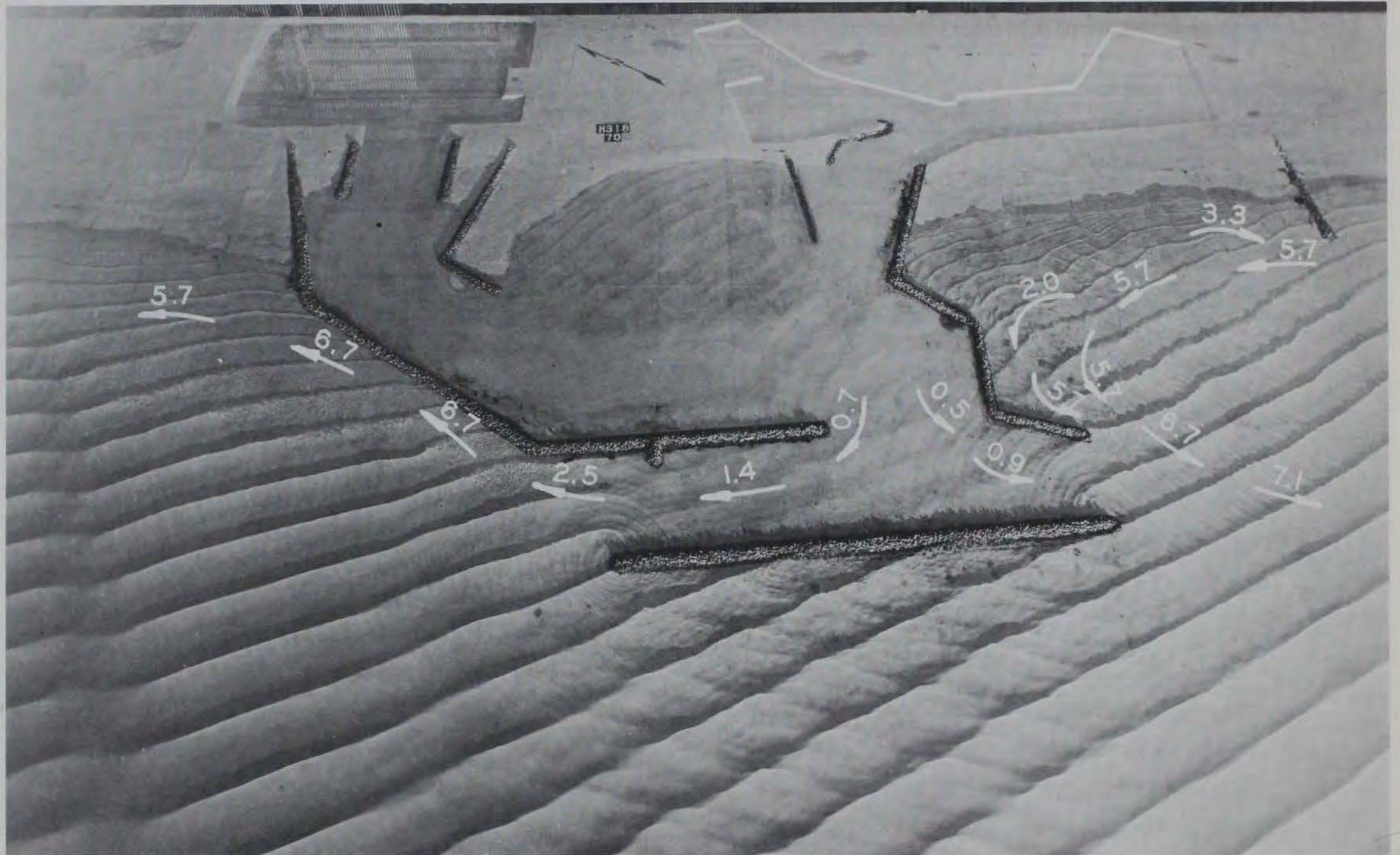
Photo 14. Typical wave and current patterns and current magnitudes (prototype feet per second) for Plan 4; 9-sec, 10-ft waves from south at mllw
