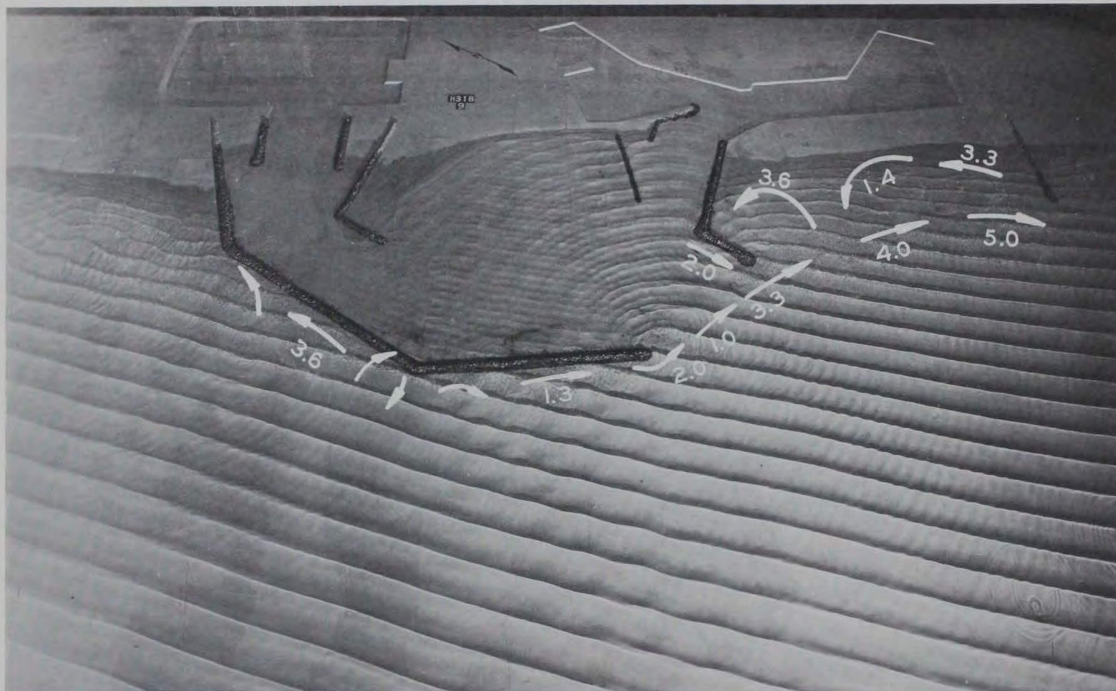
Photo 2. Typical wave and current patterns and current magnitudes (prototype feet per second) for existing conditions; 7-sec, 10-ft waves from west at mhw
