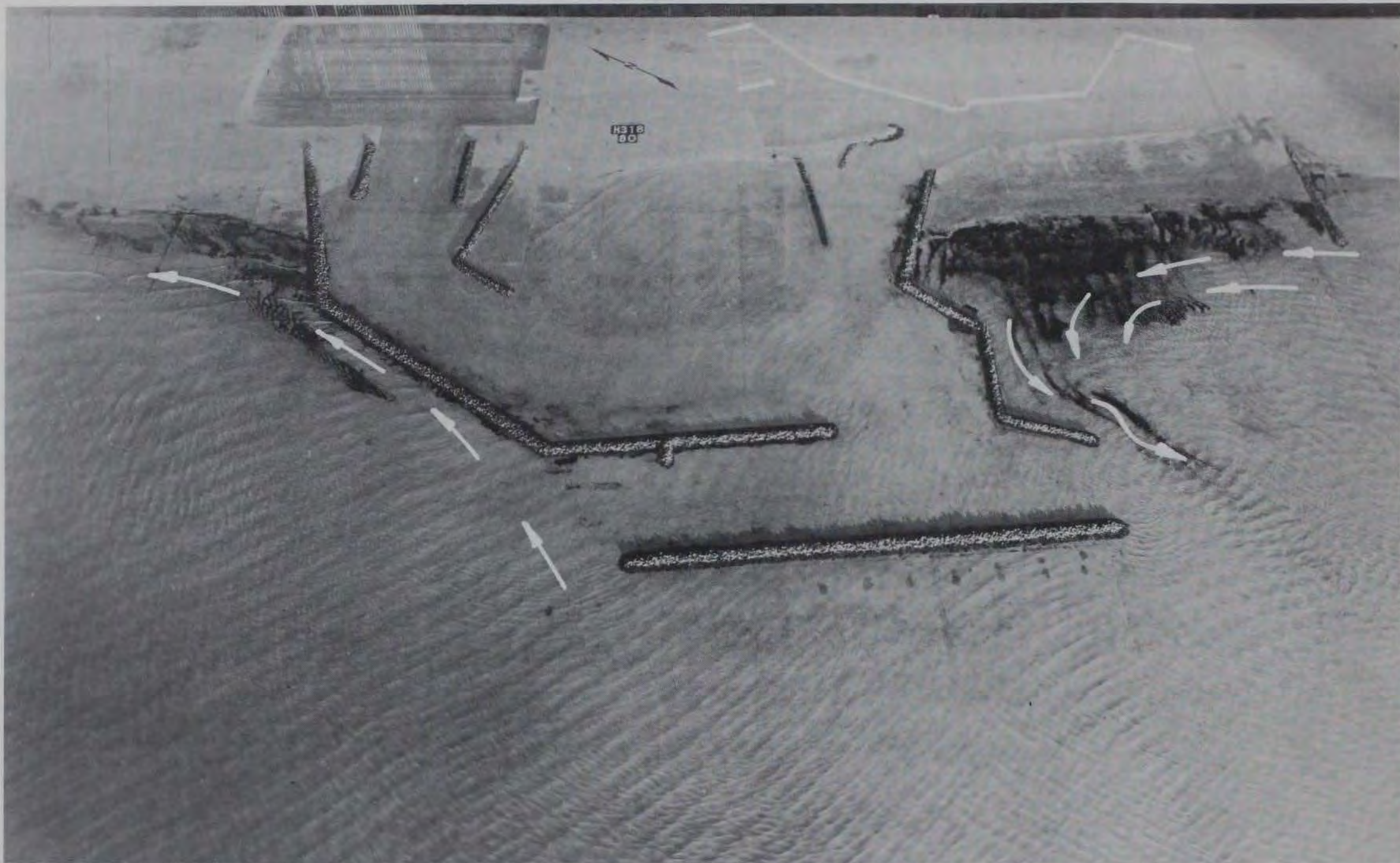
Photo 18. Typical tracer movement for Plan 4 resulting from 9-sec, 10-ft waves from south at mllw
