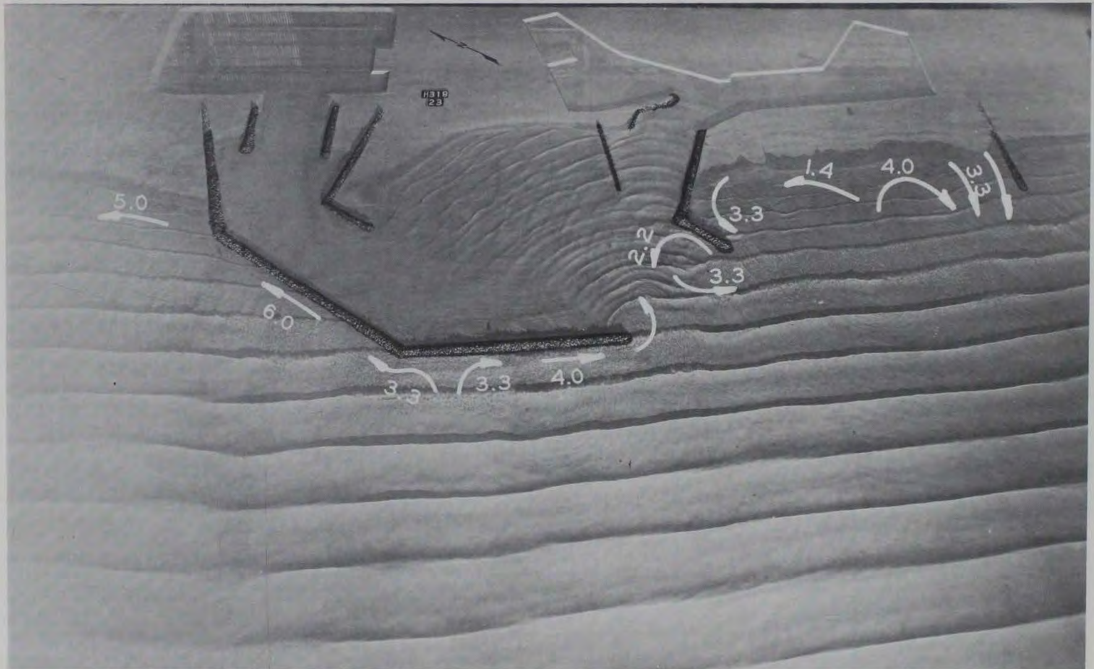
Photo 3. Typical wave and current patterns and current magnitudes (prototype feet per second) for existing conditions; 11-sec, 8-ft waves from southwest at mllw
