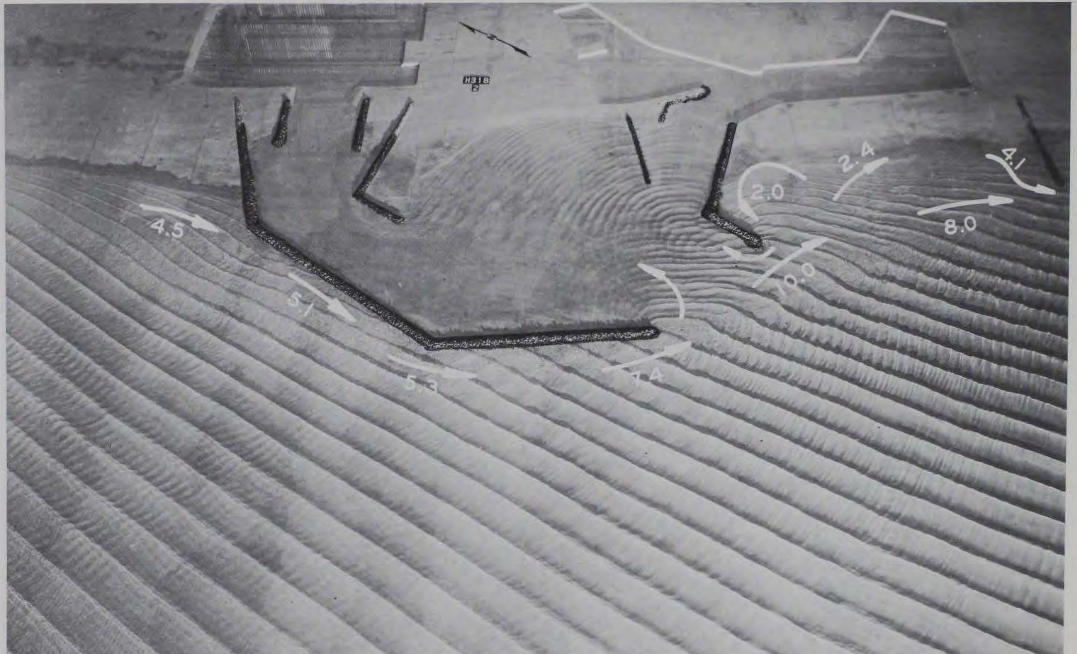
Photo 1. Typical wave and current patterns and current magnitudes (prototype feet per second) for existing conditions; 7-sec, 10-ft waves from northwest at mllw
