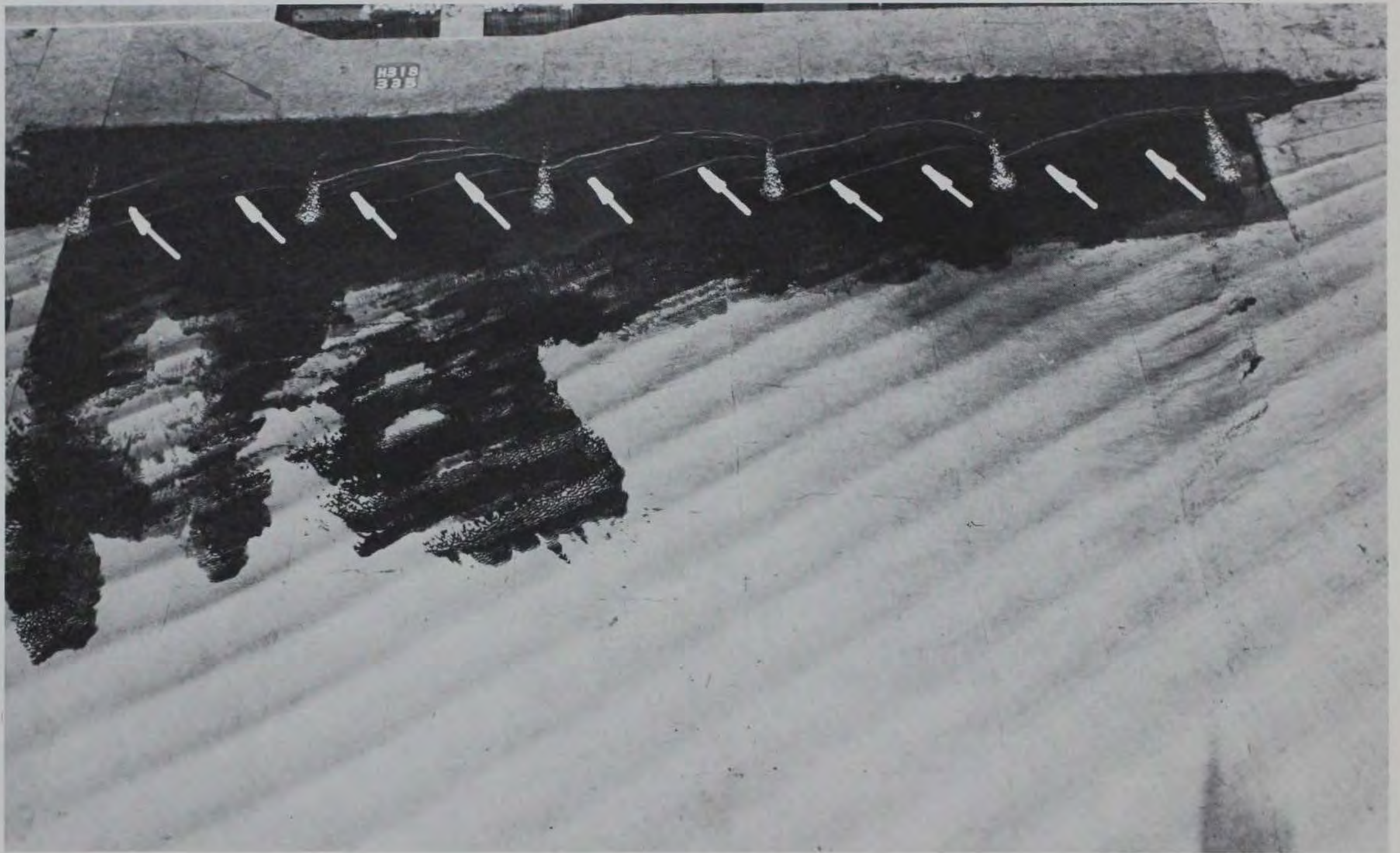
Photo 110. Movable-bed tracer deposits for Plan 18 resulting from 9-sec, 4-ft waves from south at mllw (extended test wave duration)
