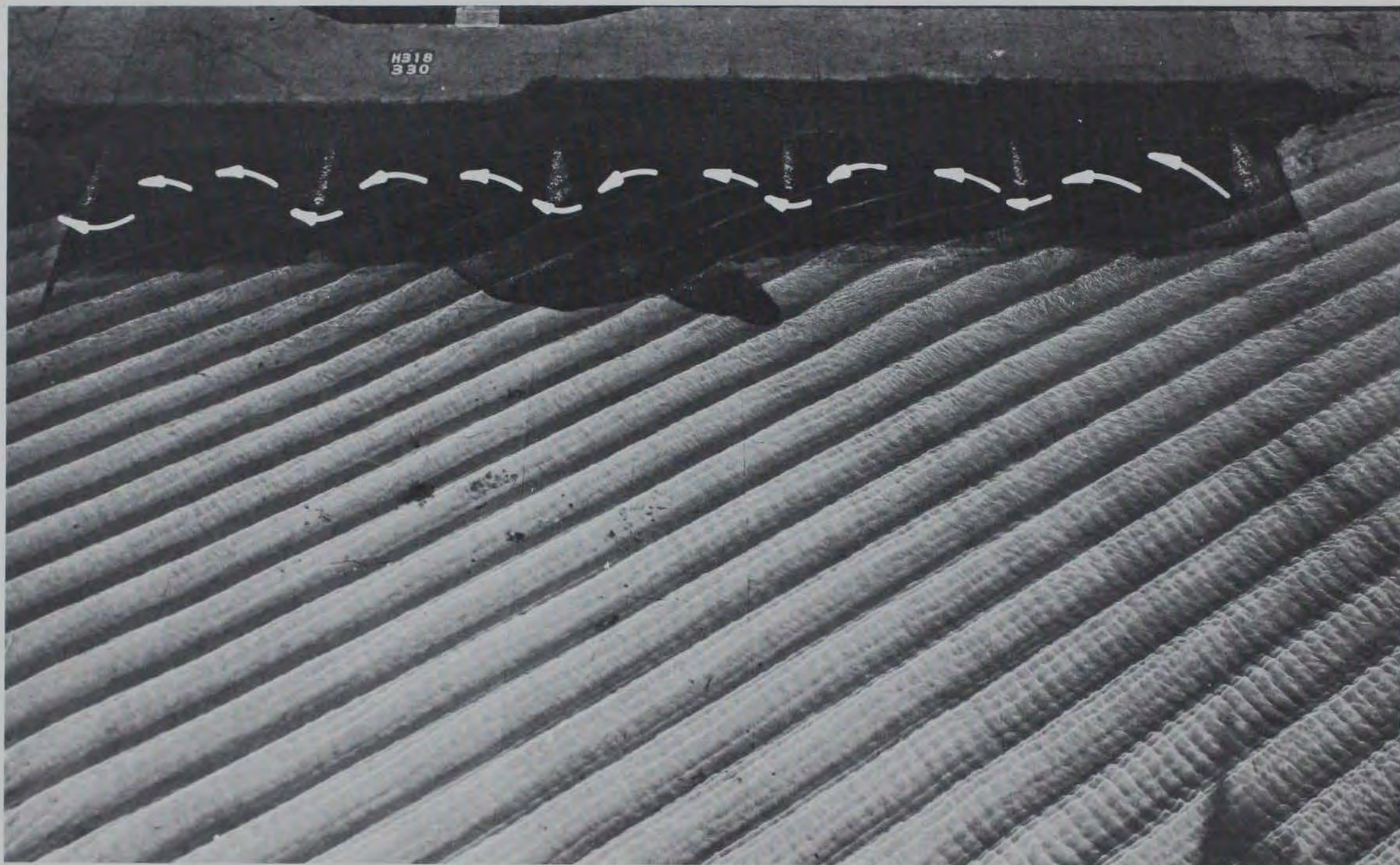
Photo 106. Movable-bed tracer deposits for Plan 18 resulting from 7-sec, 10-ft waves from south at mhw (extended test wave duration)
