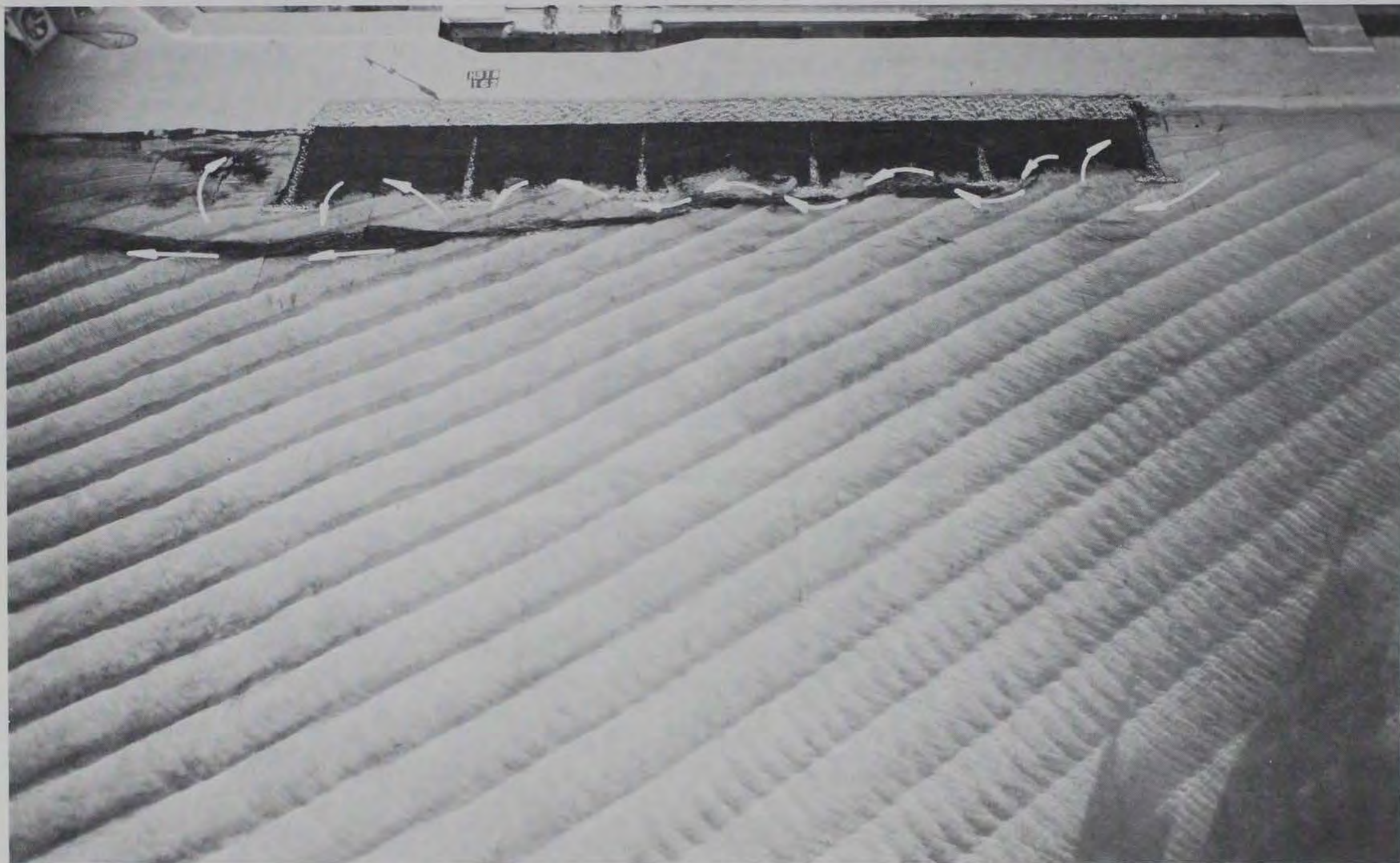
Photo 65. Semimovable-bed tracer deposits for Plan 10 resulting from 9-sec, 10-ft waves from south at mllw
