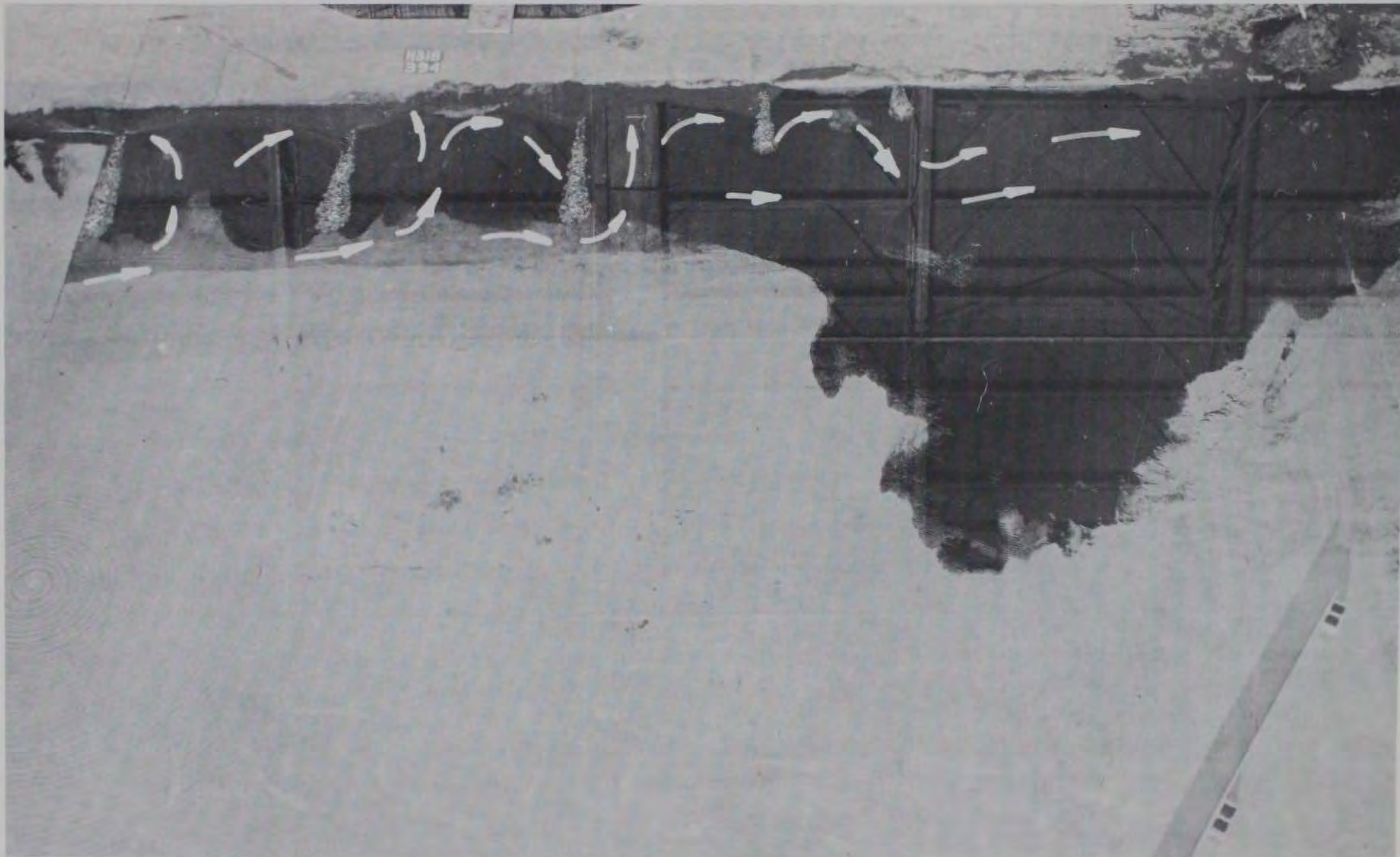
Photo 123. Movable-bed tracer deposits for Plan 9A (and adjacent south beach) resulting from 9-sec, 10-ft waves from northwest (after 4 hr)
