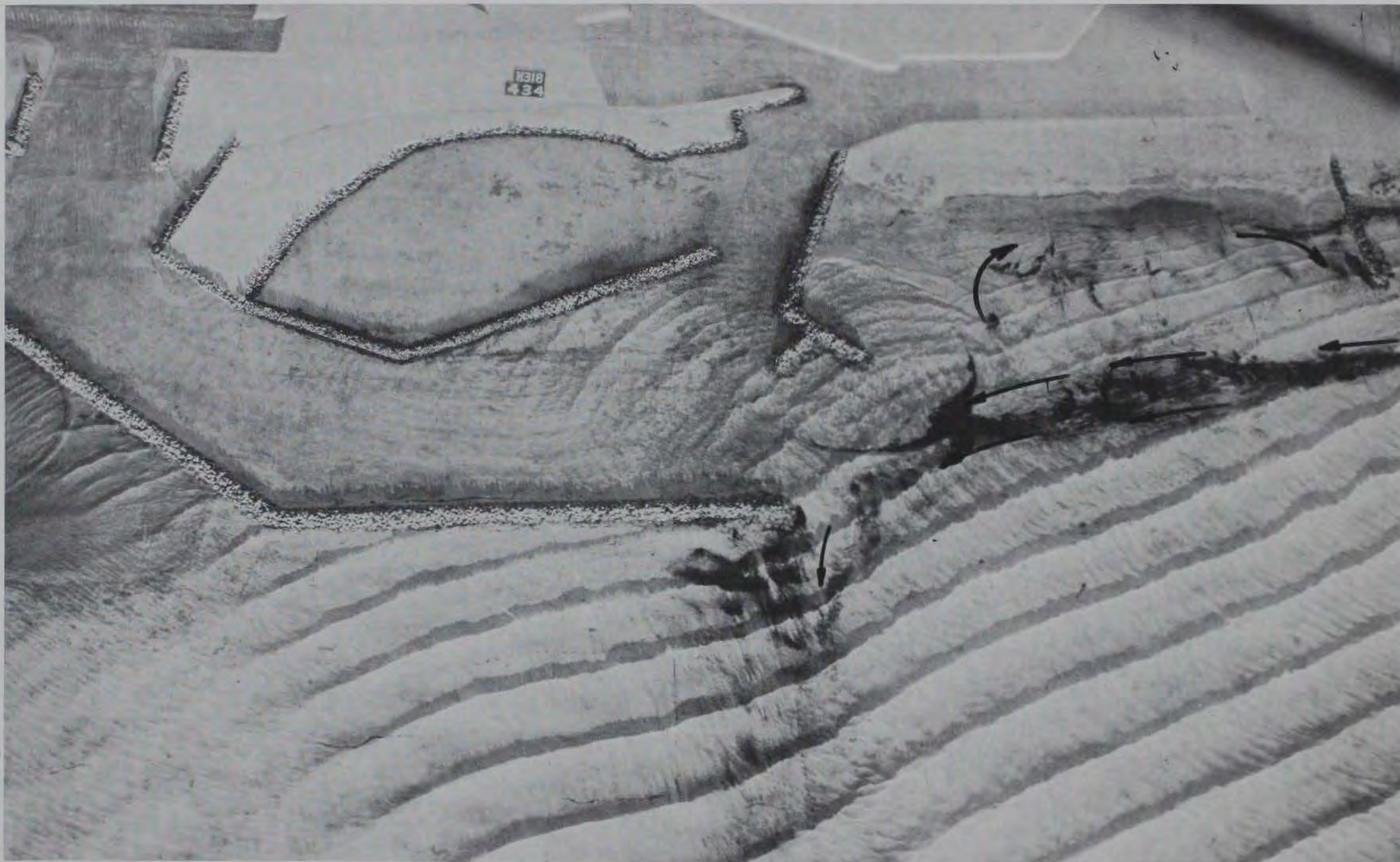
Photo 54. Typical tracer movement for Plan 61 resulting from 9-sec, 10-ft waves from south at mllw
