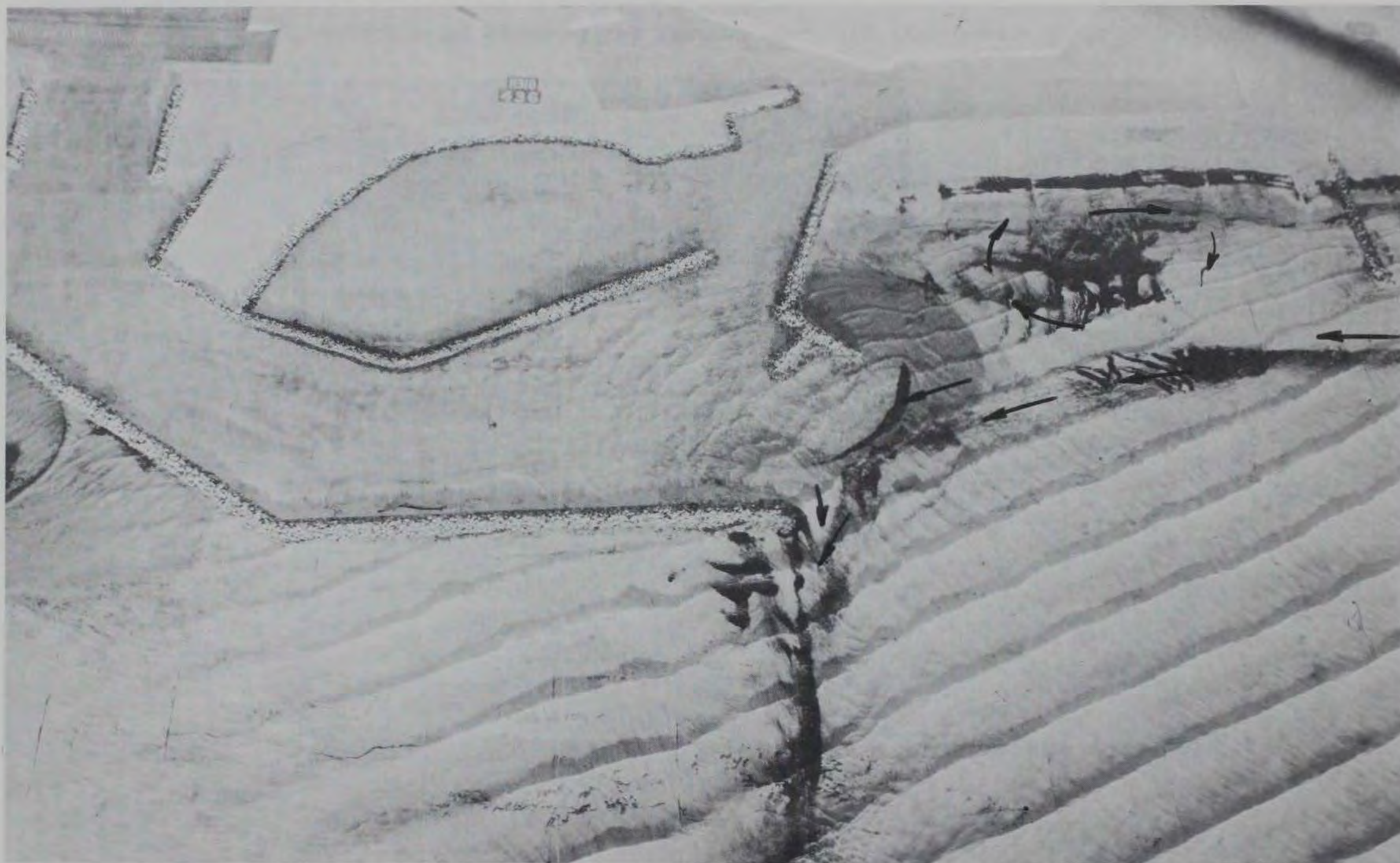
Photo 56. Typical tracer movement for Plan 62 resulting from 9-sec, 10-ft waves from south at mllw
