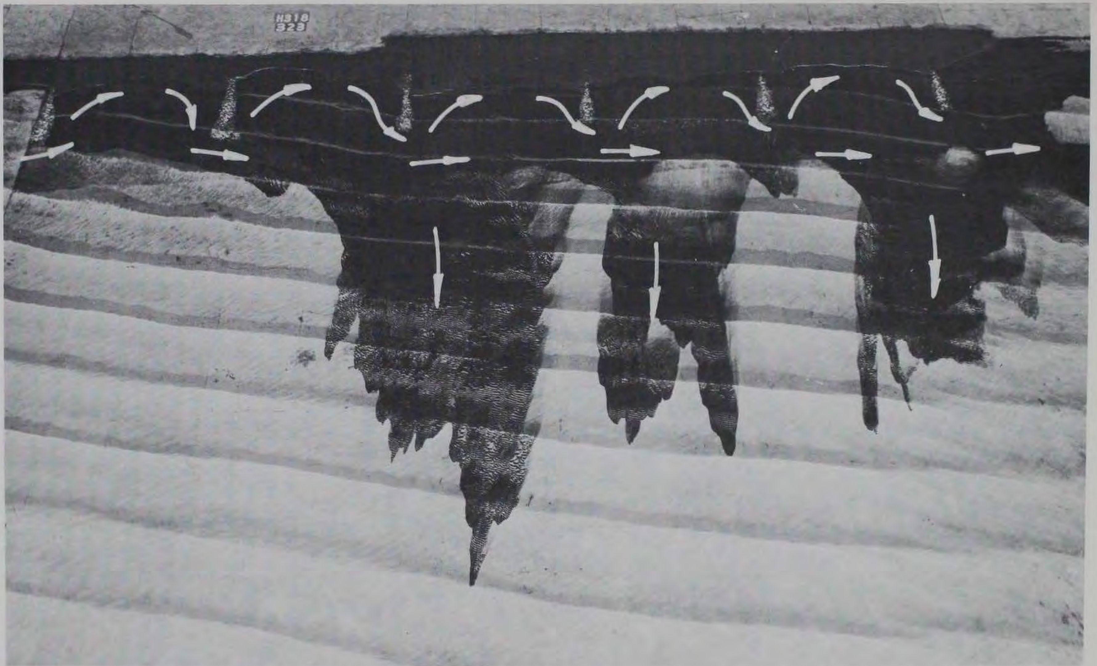
Photo 101. Movable-bed tracer deposits for Plan 18 resulting from 11-sec, 10-ft waves from west at mhw (extended test wave duration)
