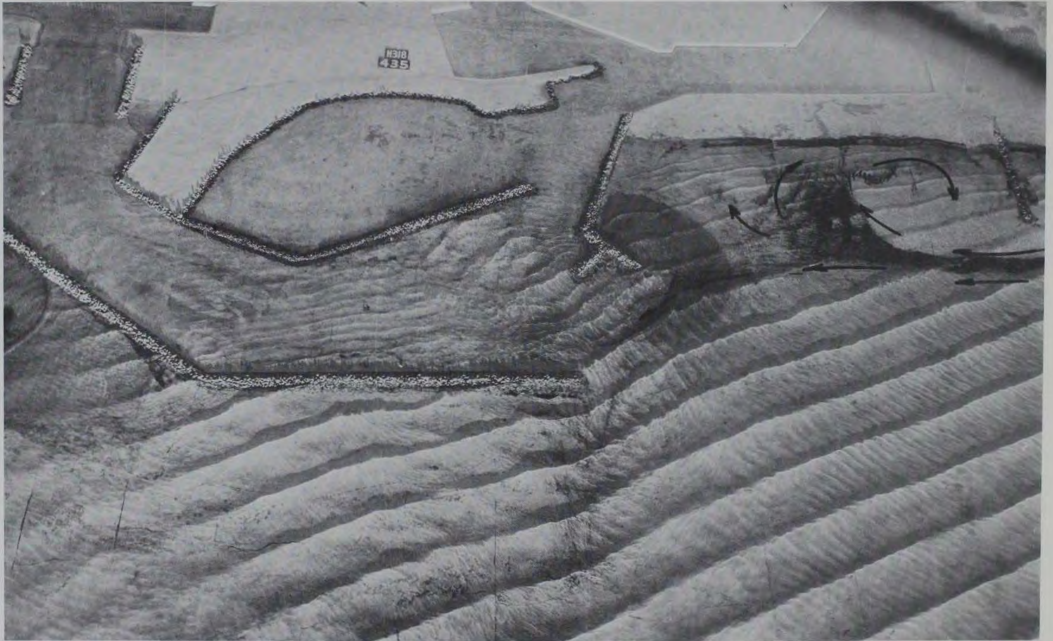
Photo 55. Typical tracer movement for Plan 62 resulting from 9-sec, 10-ft waves from south at mhhw
