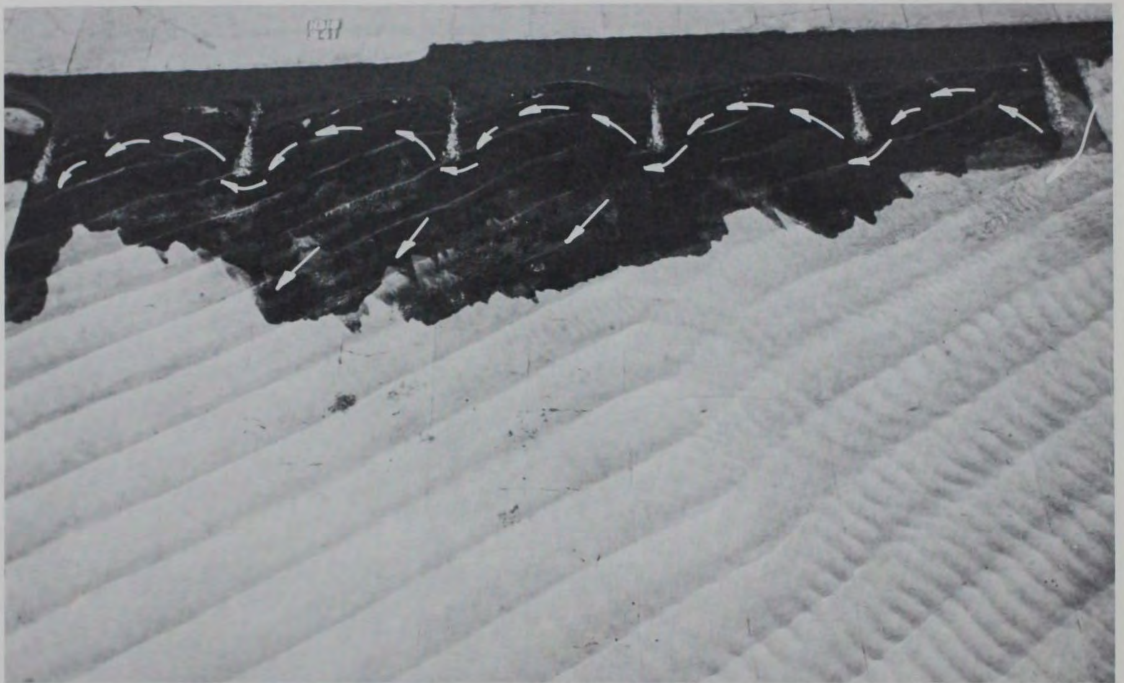
Photo 116. Movable-bed tracer deposits for Plan 9 resulting from 9-sec, 10-ft waves from south at mhw (extended test wave duration)
