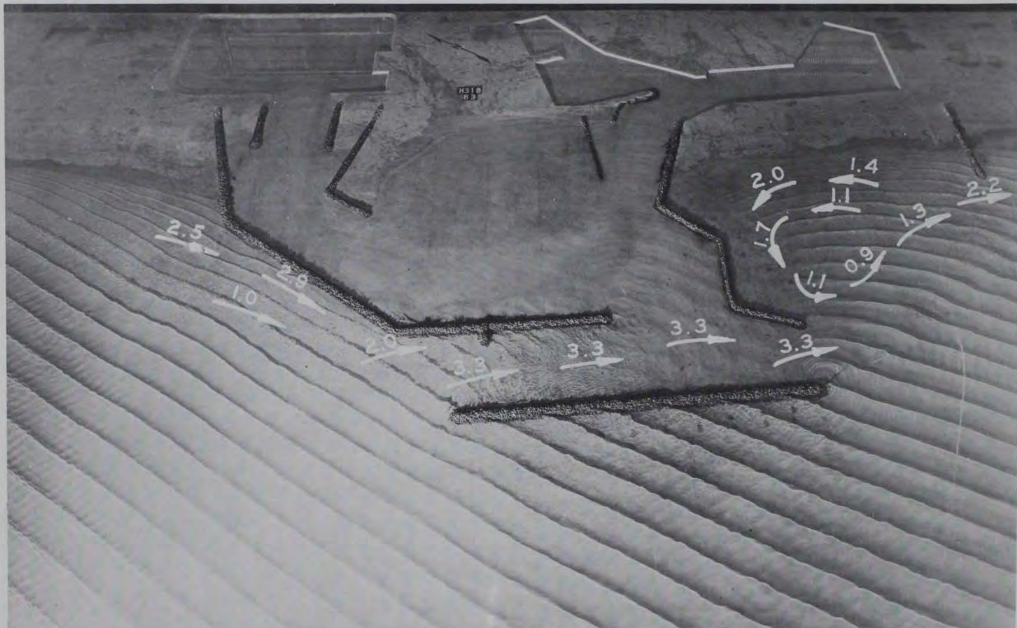
Photo 11. Typical wave and current patterns and current magnitudes (prototype feet per second) for Plan 4; 7-sec, 10-ft waves from northwest at mllw
