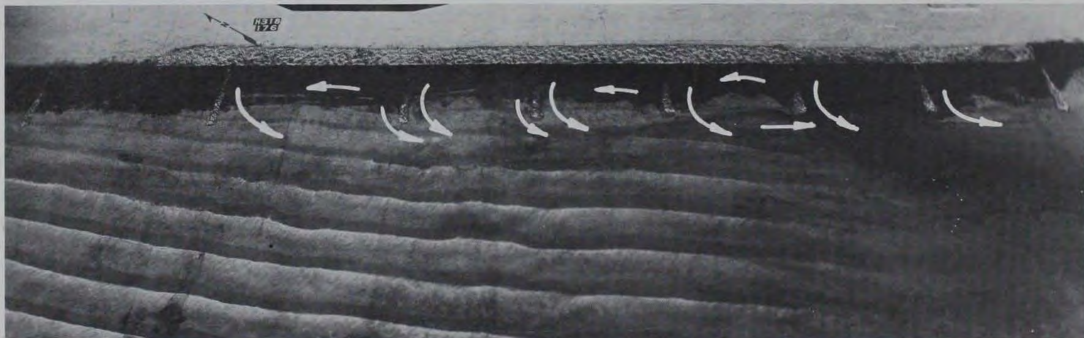
Photo 68. Semimovable-bed tracer deposits for Plan 12 resulting from 11-sec, 10-ft waves from west at mllw (tested with final beach of previous test)
