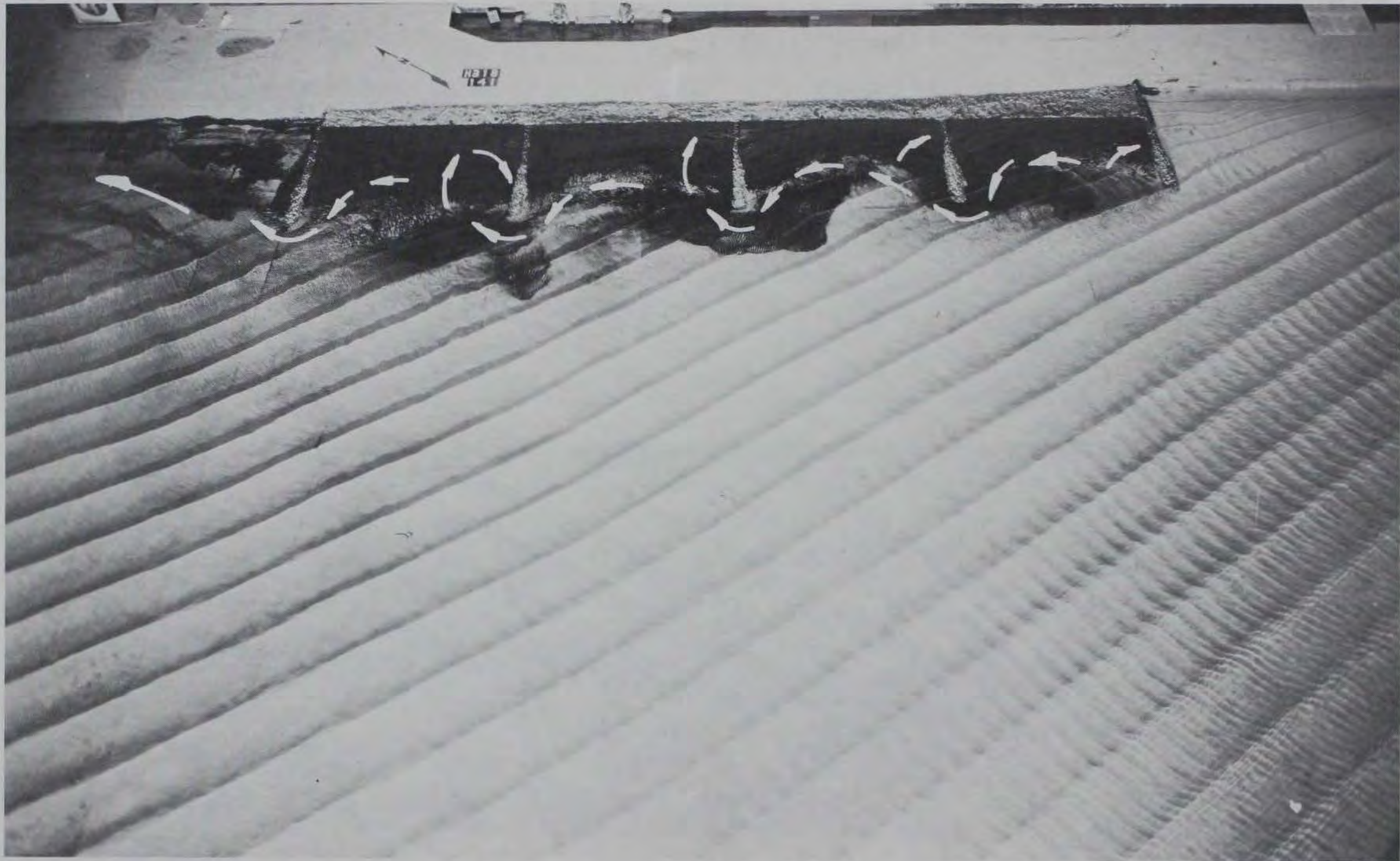
Photo 62. Semimovable-bed tracer deposits for Plan 7 resulting from 9-sec, 10-ft waves from south at mllw
