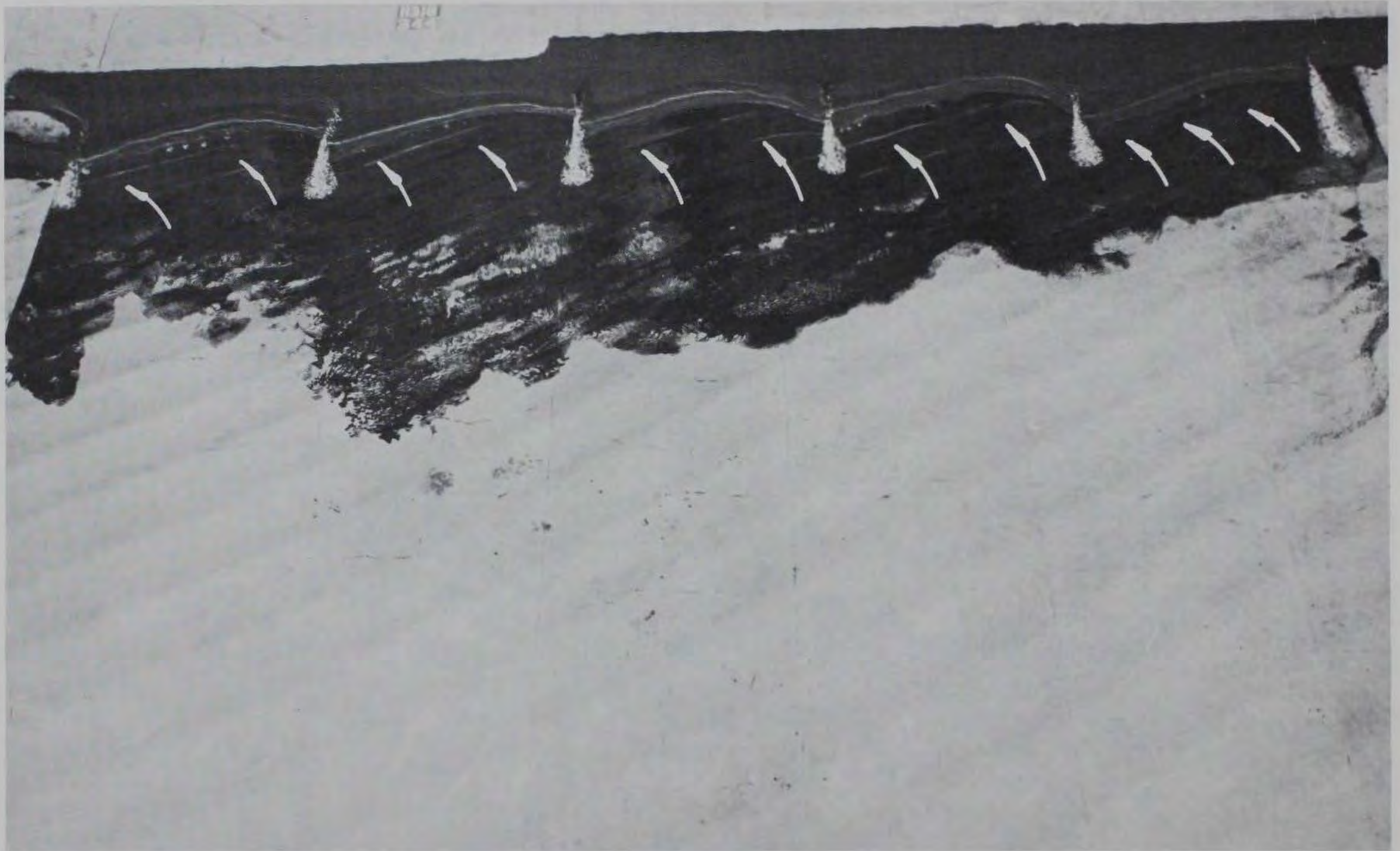
Photo 118. Movable-bed tracer deposits for Plan 9 resulting from 9-sec, 4-ft waves from south at mllw (extended test wave duration)
