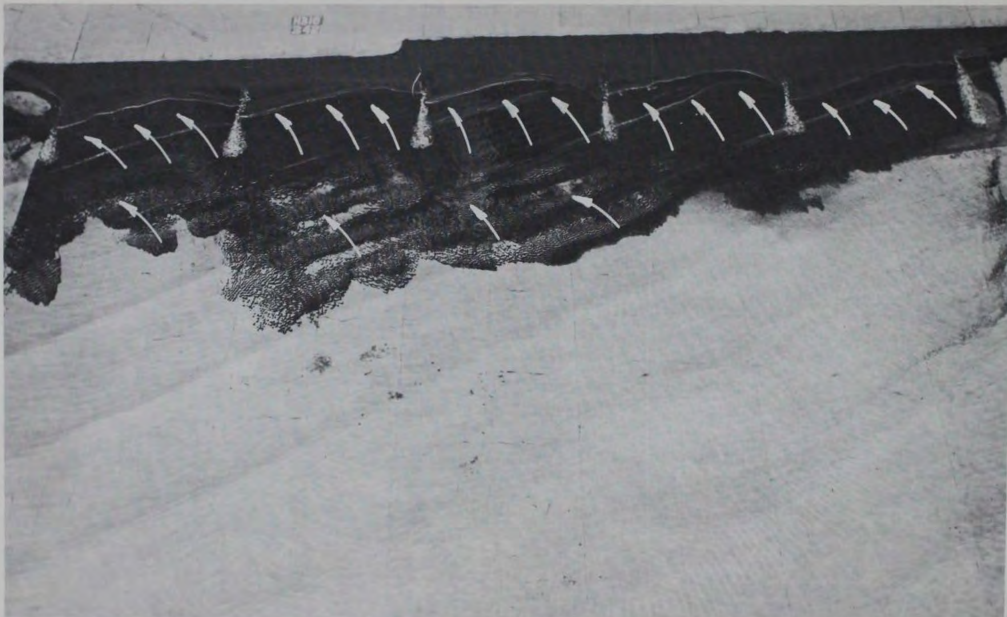
Photo 117. Movable-bed tracer deposits for Plan 9 resulting from 17-sec, 6-ft waves from south at mhhw (extended test wave duration)
