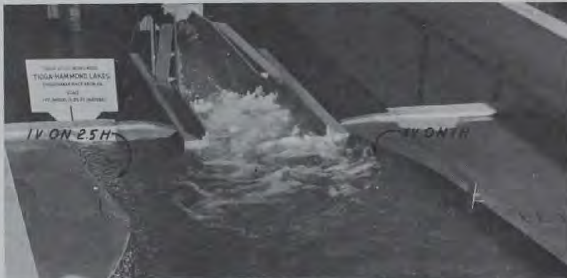
Figure 5. Abrupt walls with satisfactory wave action at design flow
