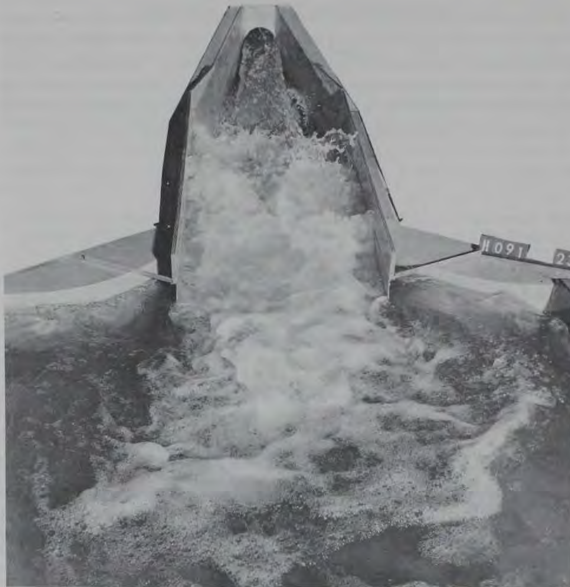
Figure 4. Original basin with walls raised 8 ft to el 1051
