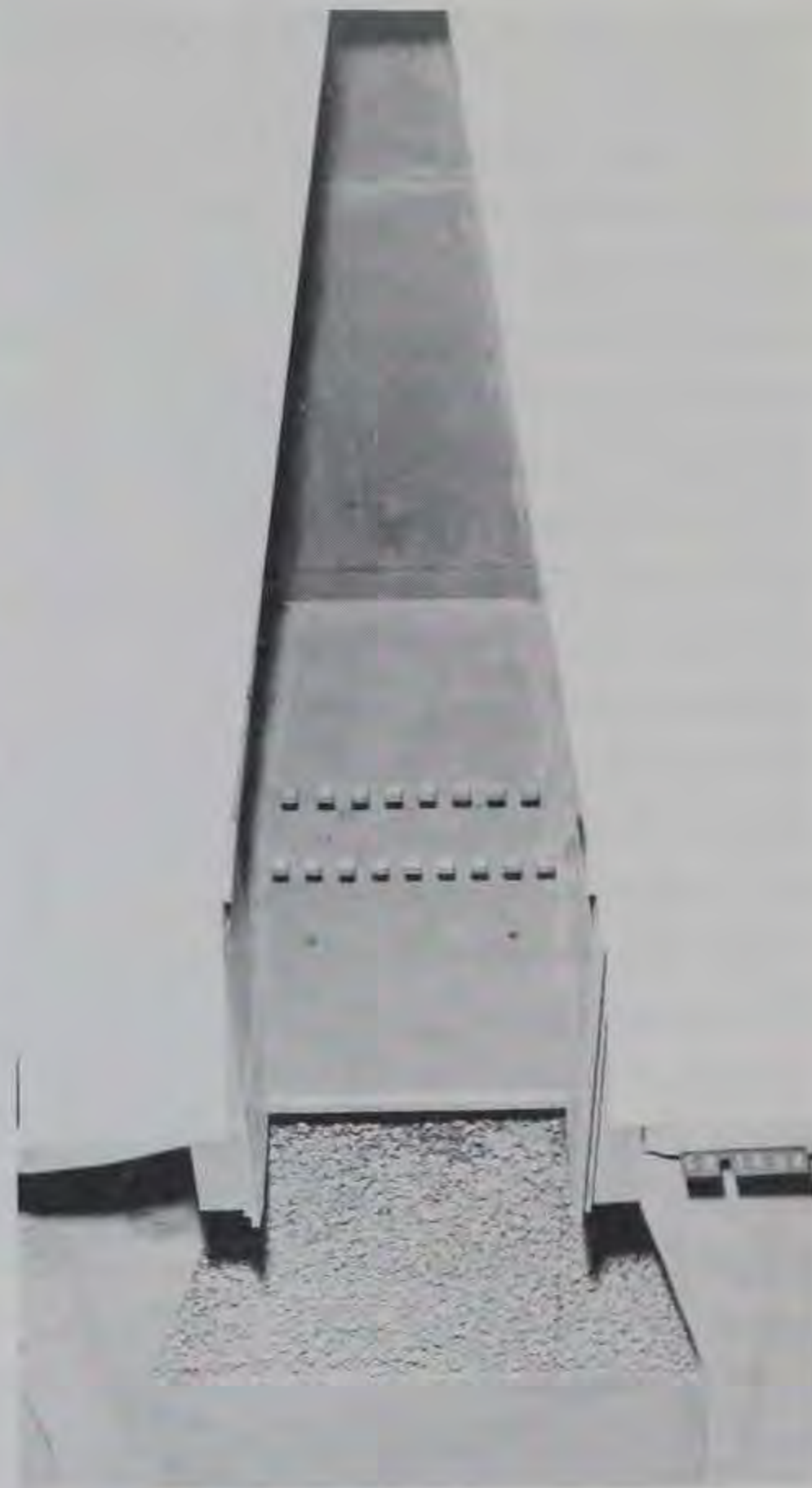
Figure 6. Recommended stilling basin, design 15
