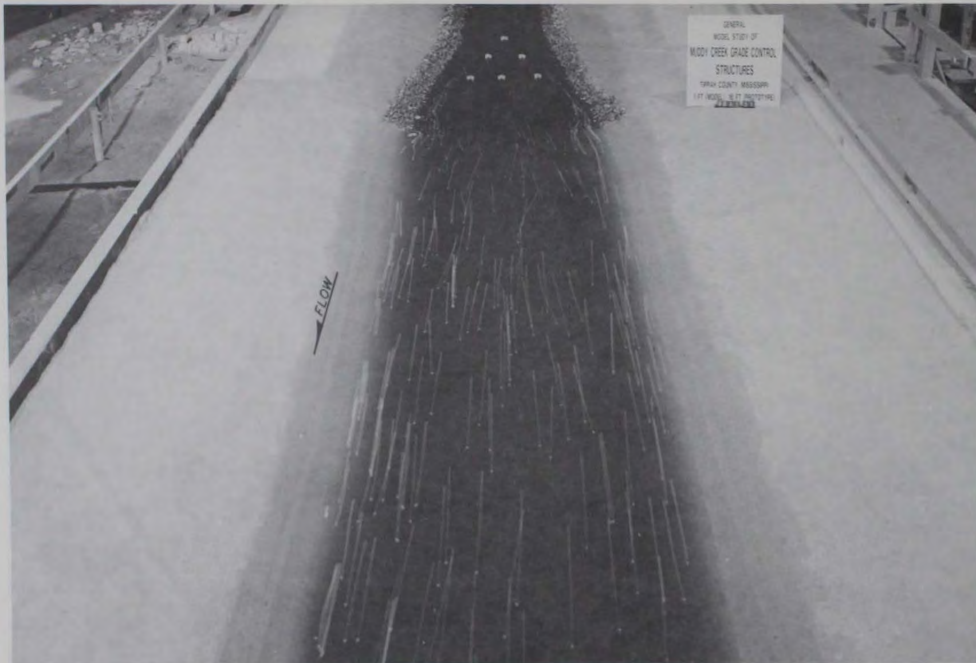
Photo 6. Type 3C exit transition (6.2-ft tall baffles) at 1,000-cfs flow
