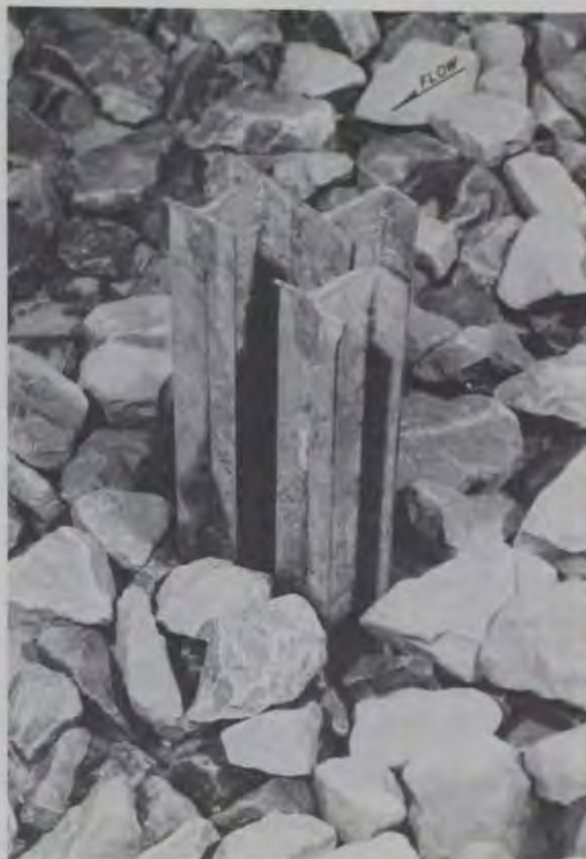
Figure 5. Type 3C baffle
