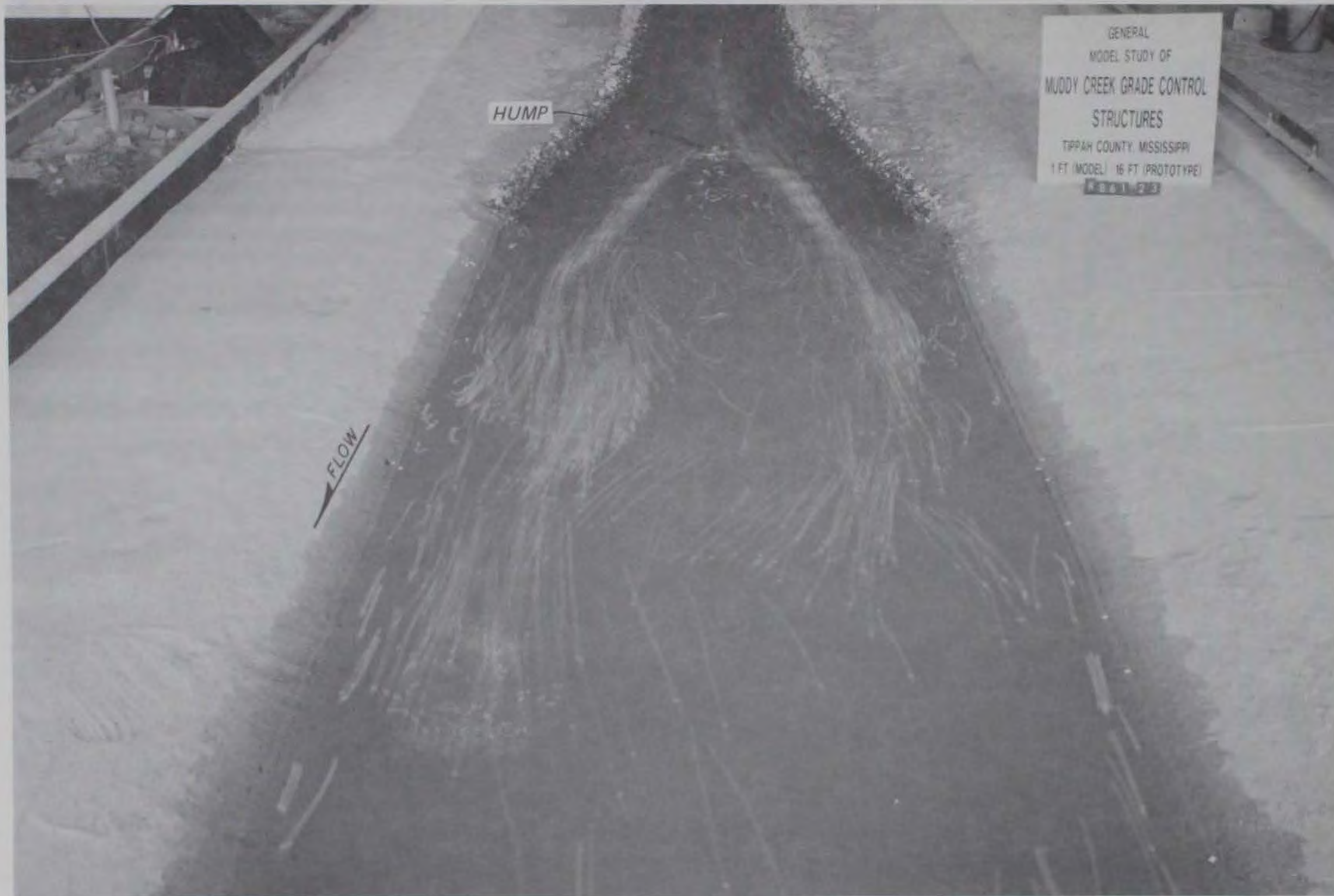
Photo 4. Type 2 exit transition at 2,000-cfs flow
