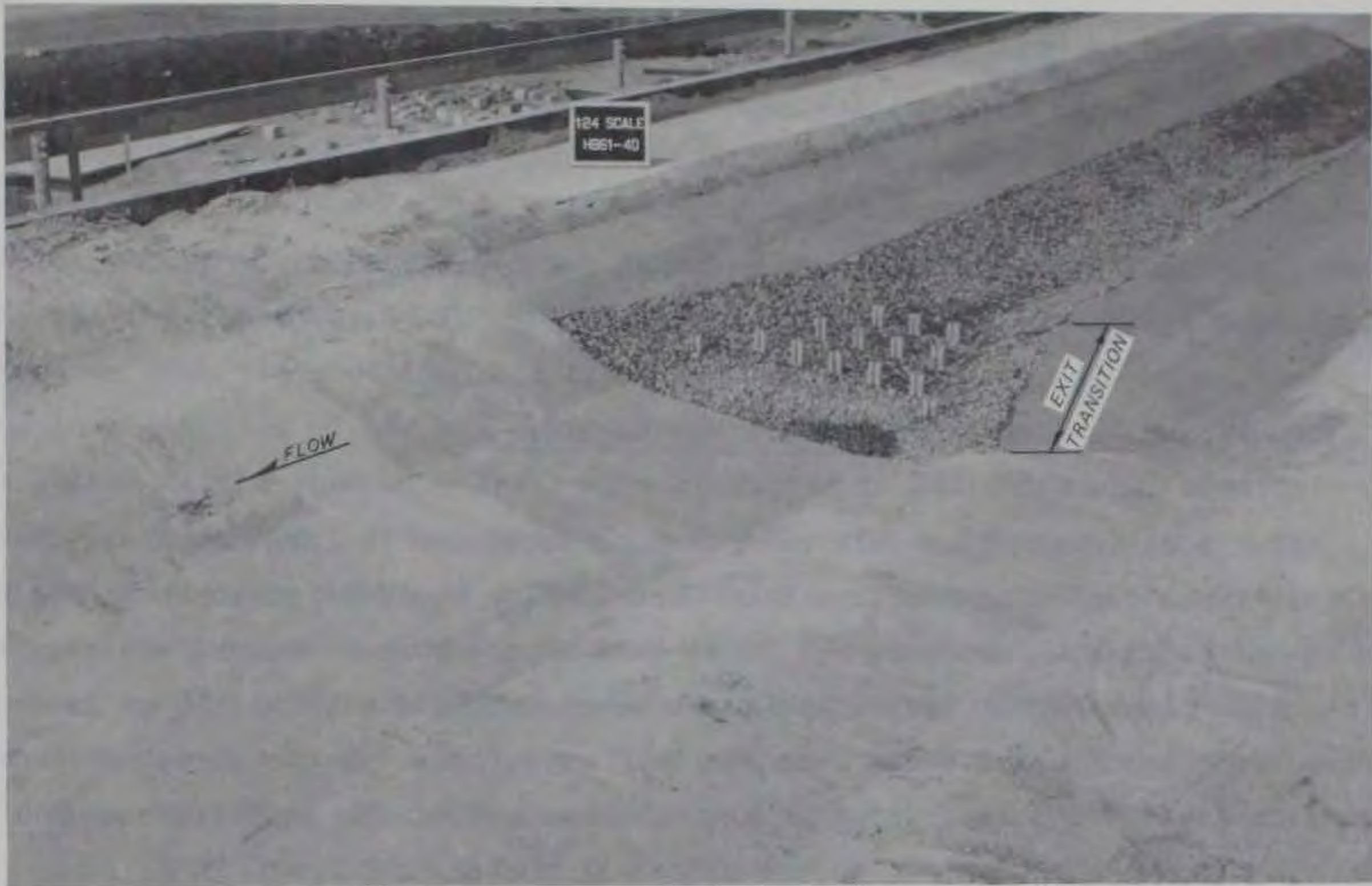
Figure 6. Type 7 exit transition
