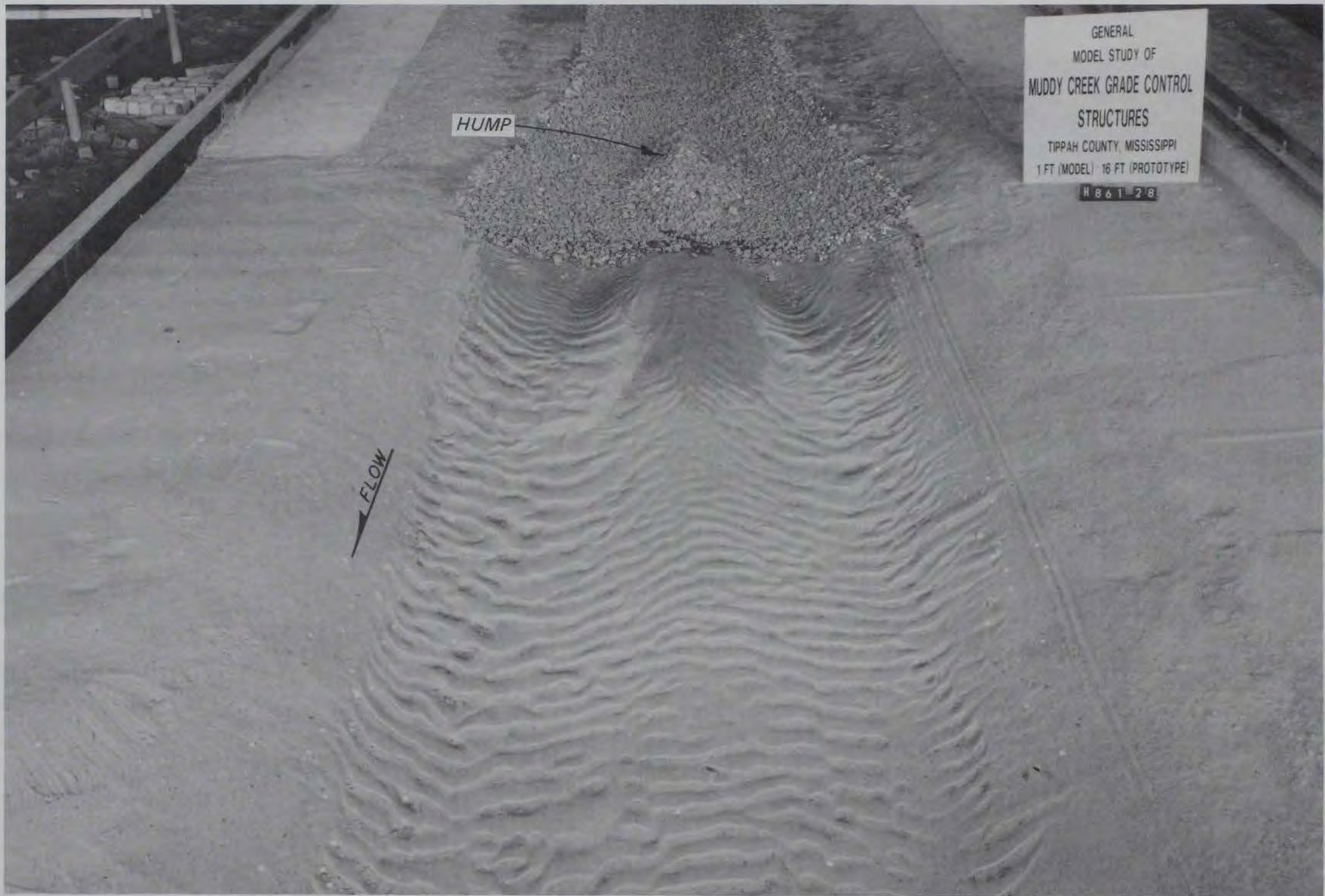
Photo 5. Scour resulting from the synthetic hydrograph, type 2 exit transition design
