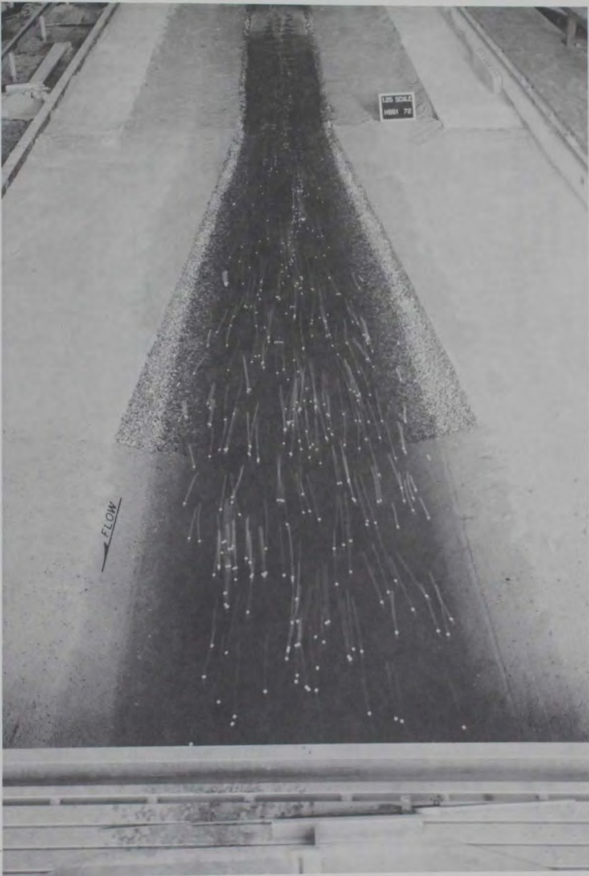
Photo 16. 1:16 flare exit transition at design flow
