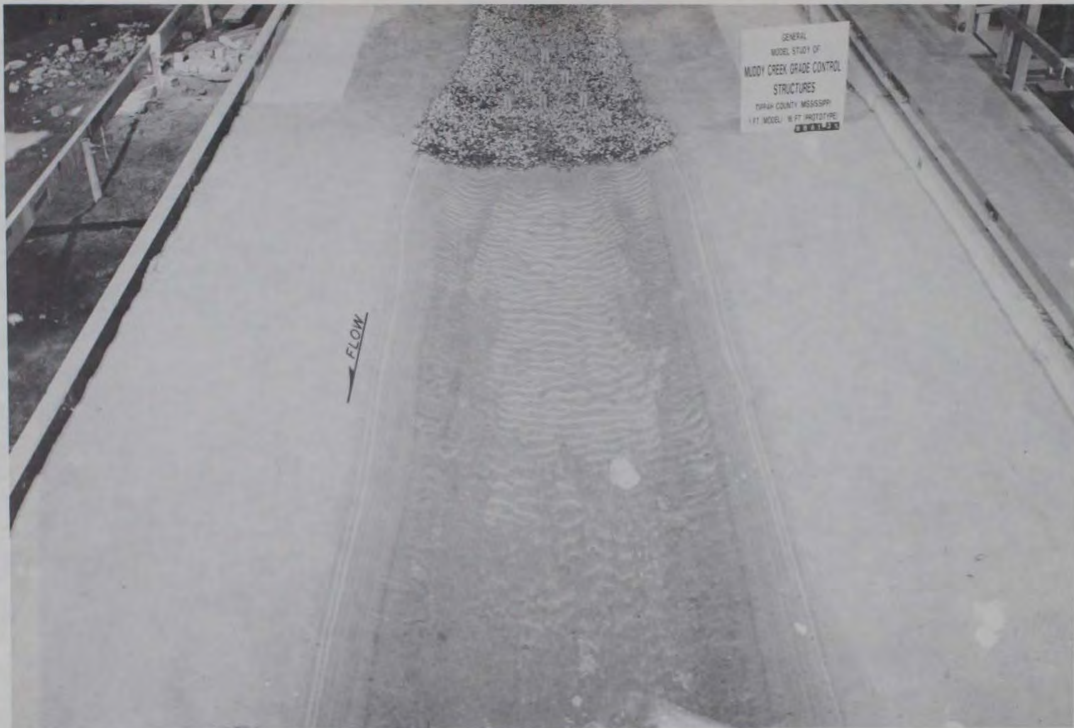
Photo 8. Scour resulting from the synthetic hydrograph, type 3C exit transition (6.2-ft-tall baffles)
