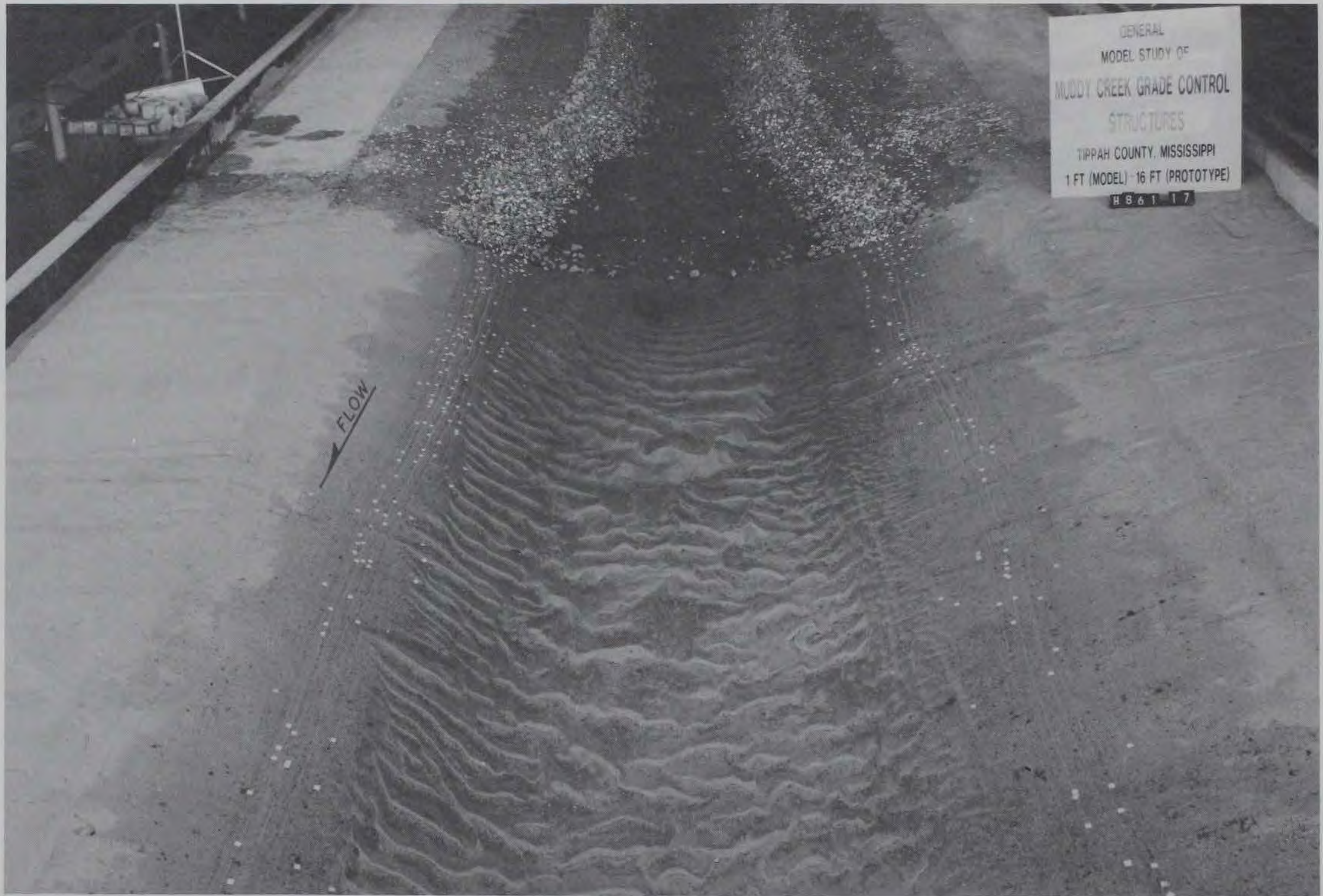
Photo 3. Scour resulting from the synthetic hydrograph, original design
