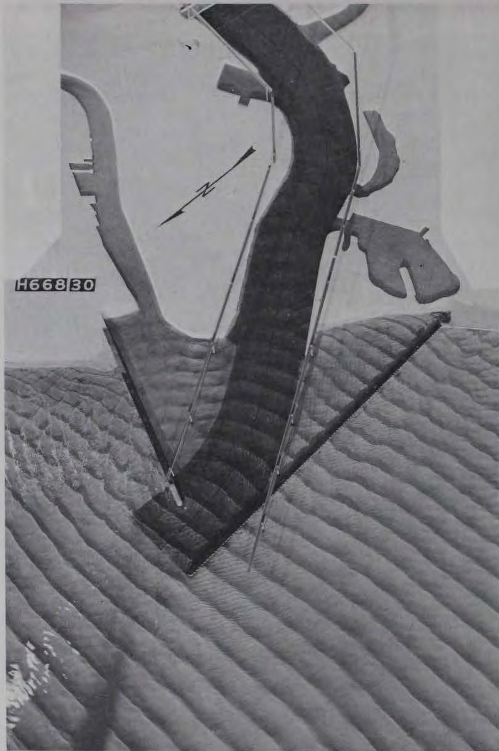
Photograph 4. Plan 2; 5-sec, 5-ft waves from north 06^{\circ} east
