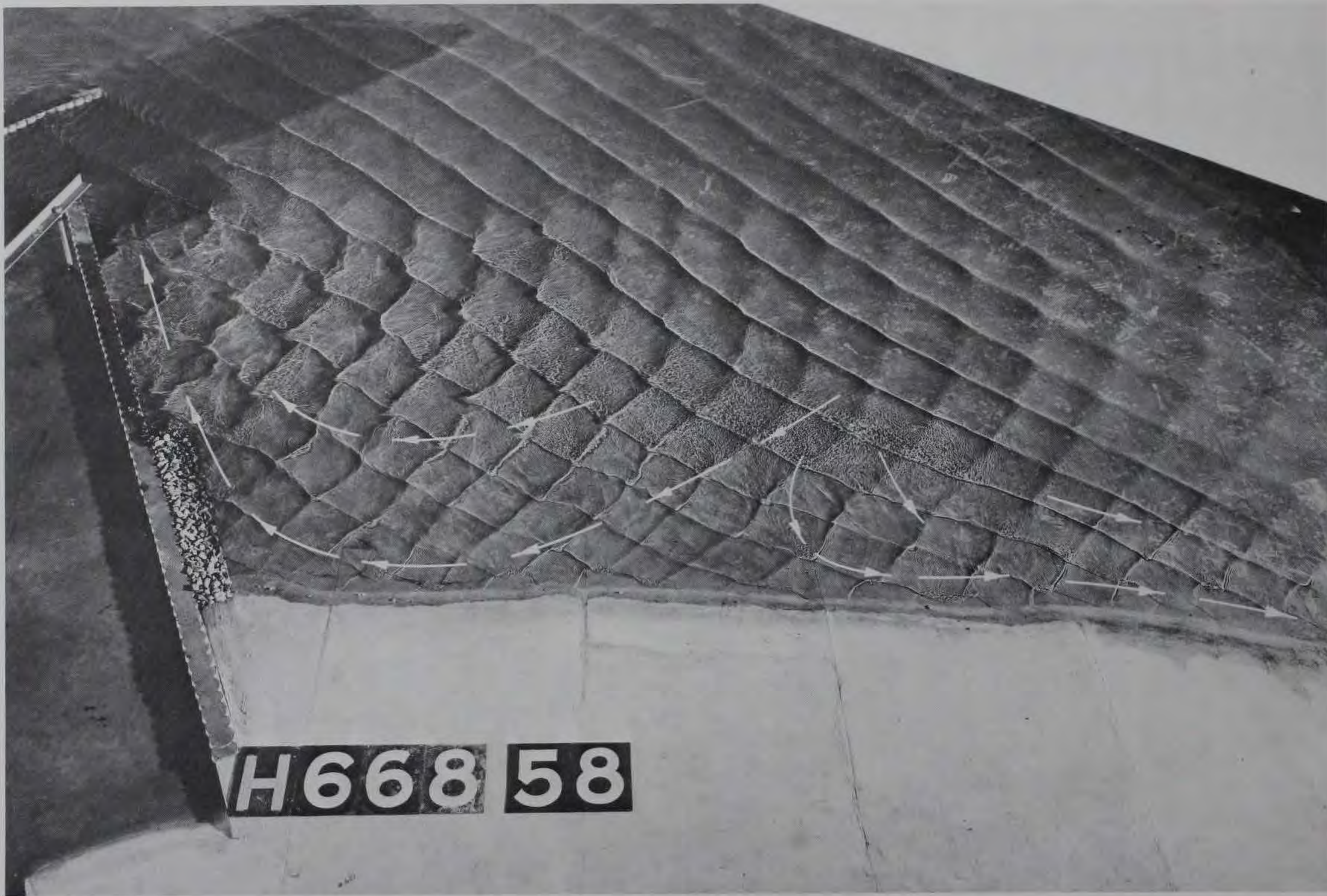
Photograph 17. Plan 6D; 5-sec, 5-ft waves from north 06^{\circ} east
