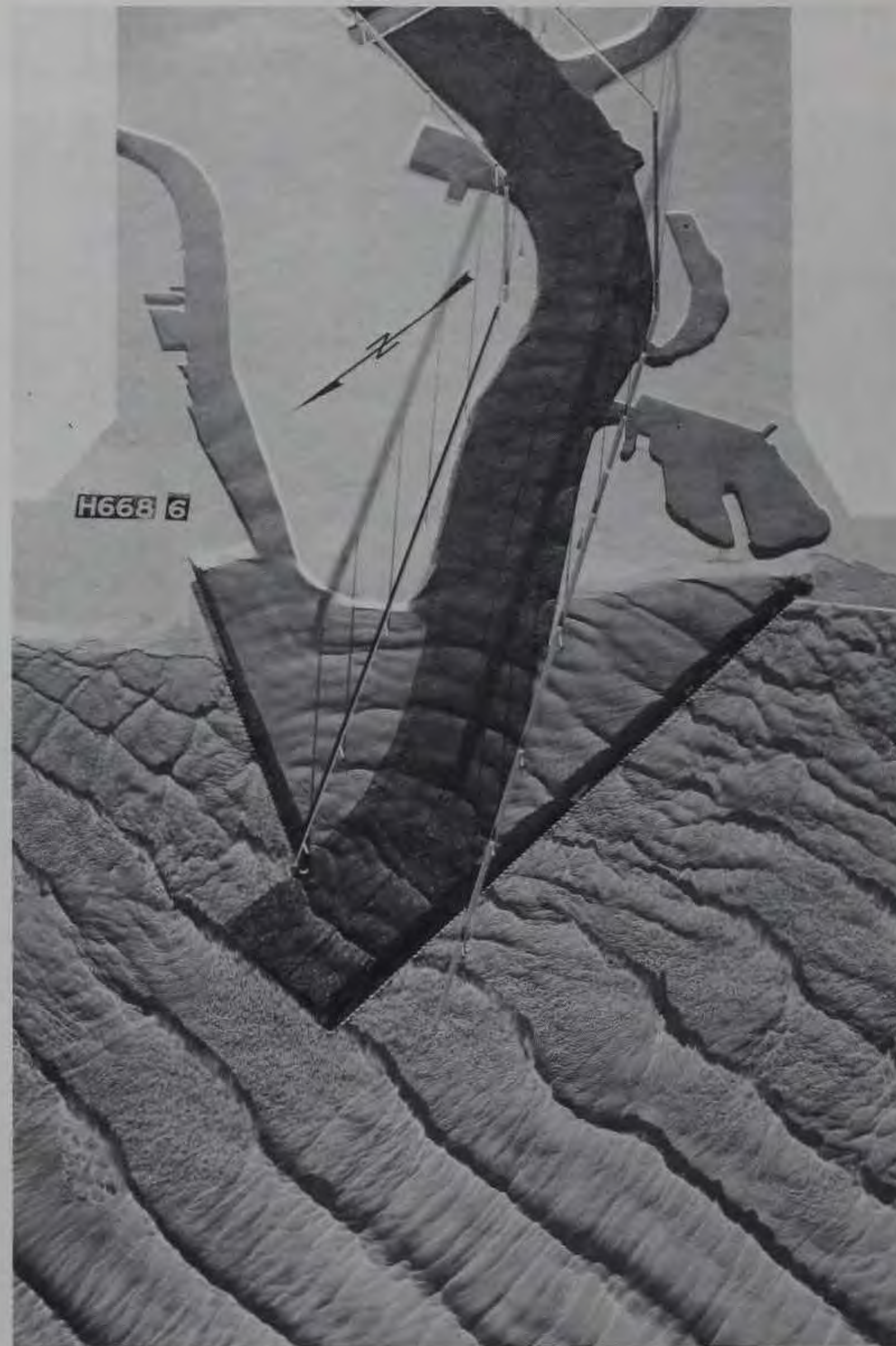
Photograph 3. Plan 1; 9-sec, 10-ft waves from north 06^{\circ} east
