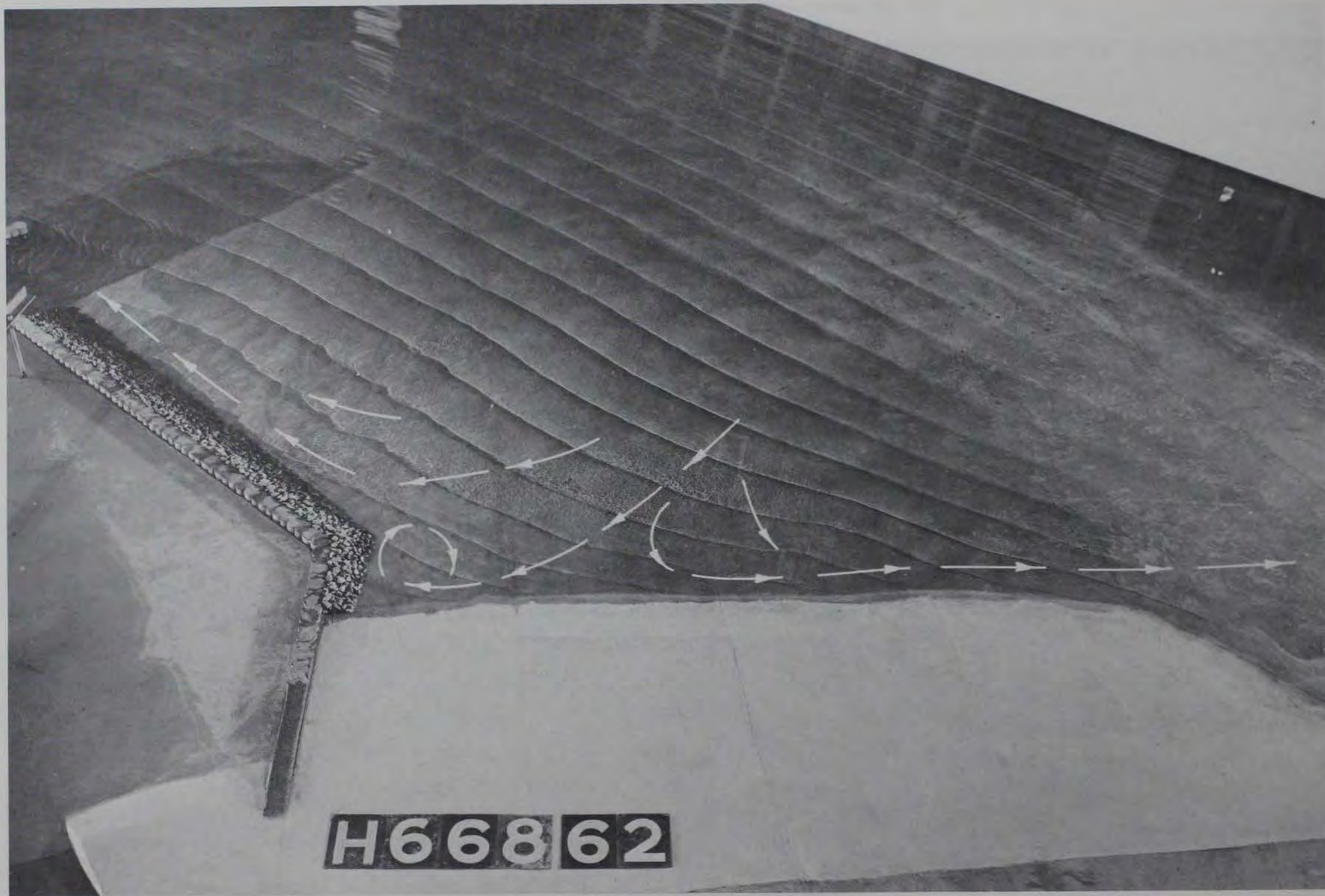
Photograph 23. Plan 7A; 5-sec, 5-ft waves from north 06° east
