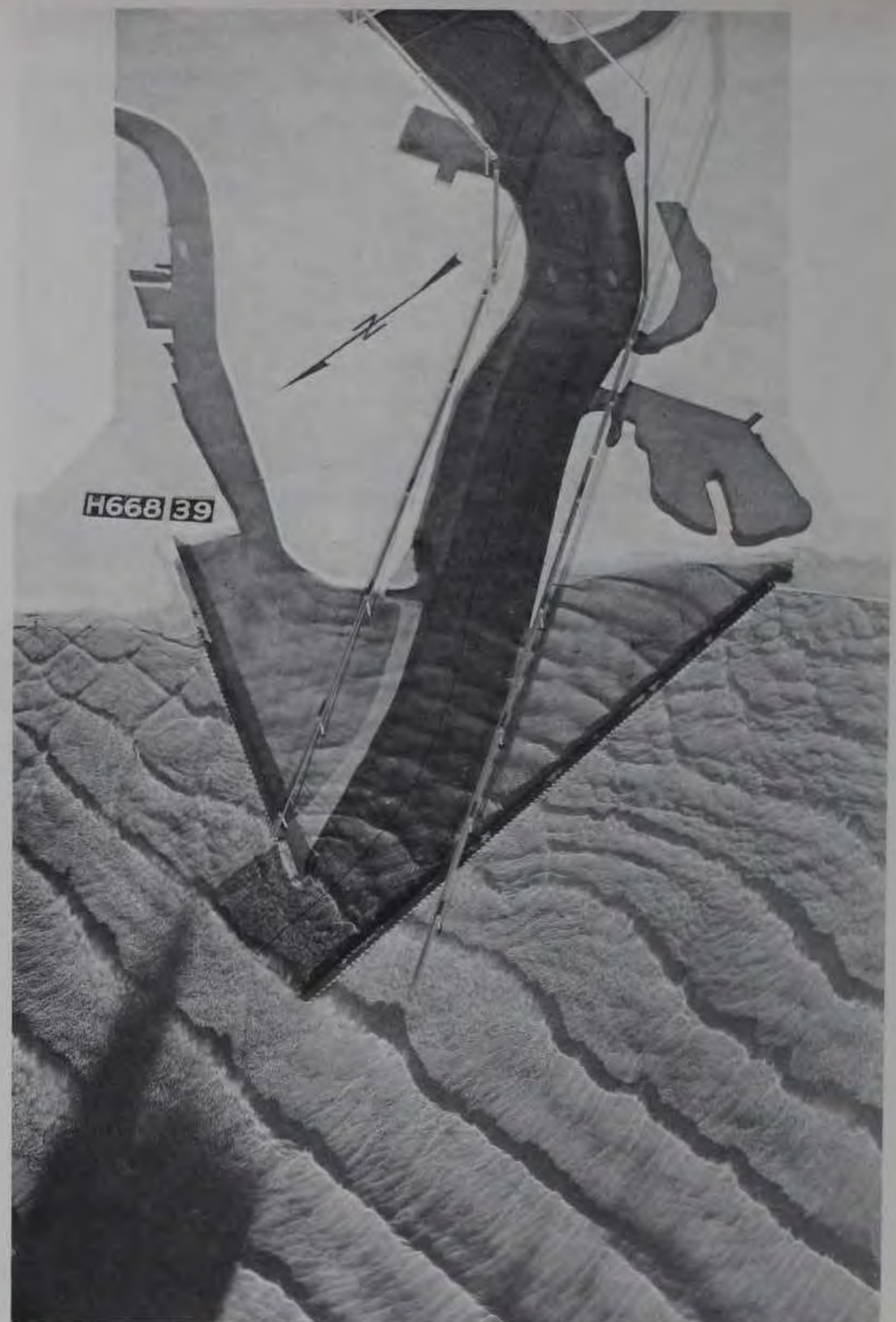
Photograph 9. Plan 4; 9-sec, 10-ft waves from north 06^{\circ} east
