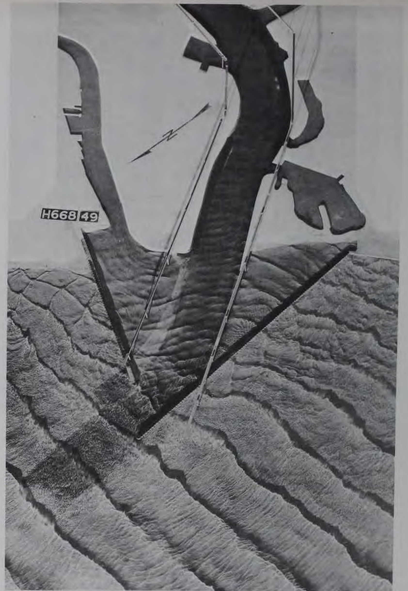
Photograph 13. Plan 6; 9-sec, 10-ft waves from north 06^{\circ} east
