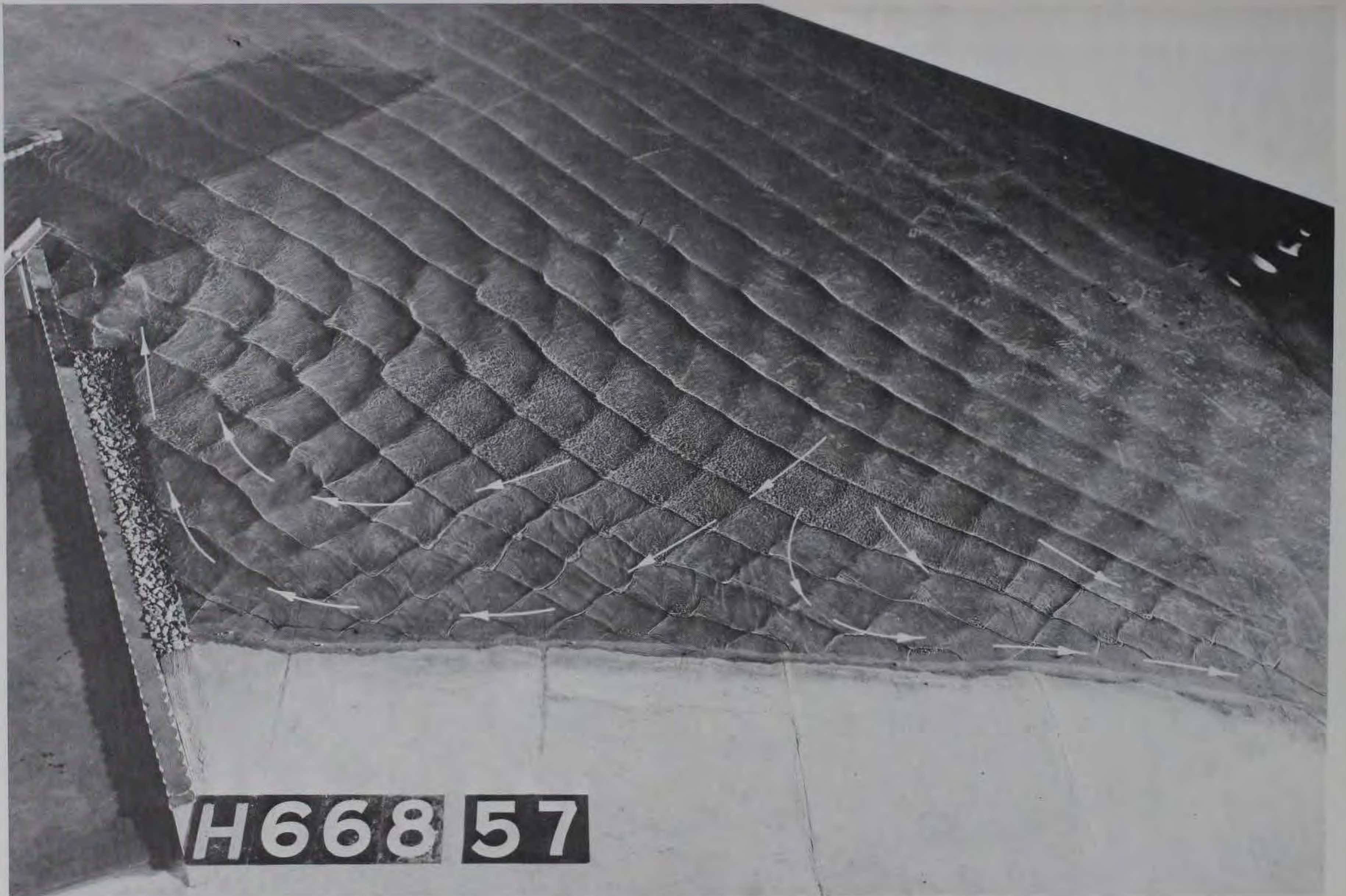
Photograph 18. Plan 6E; 5-sec, 5-ft waves from north 06^{\circ} east
