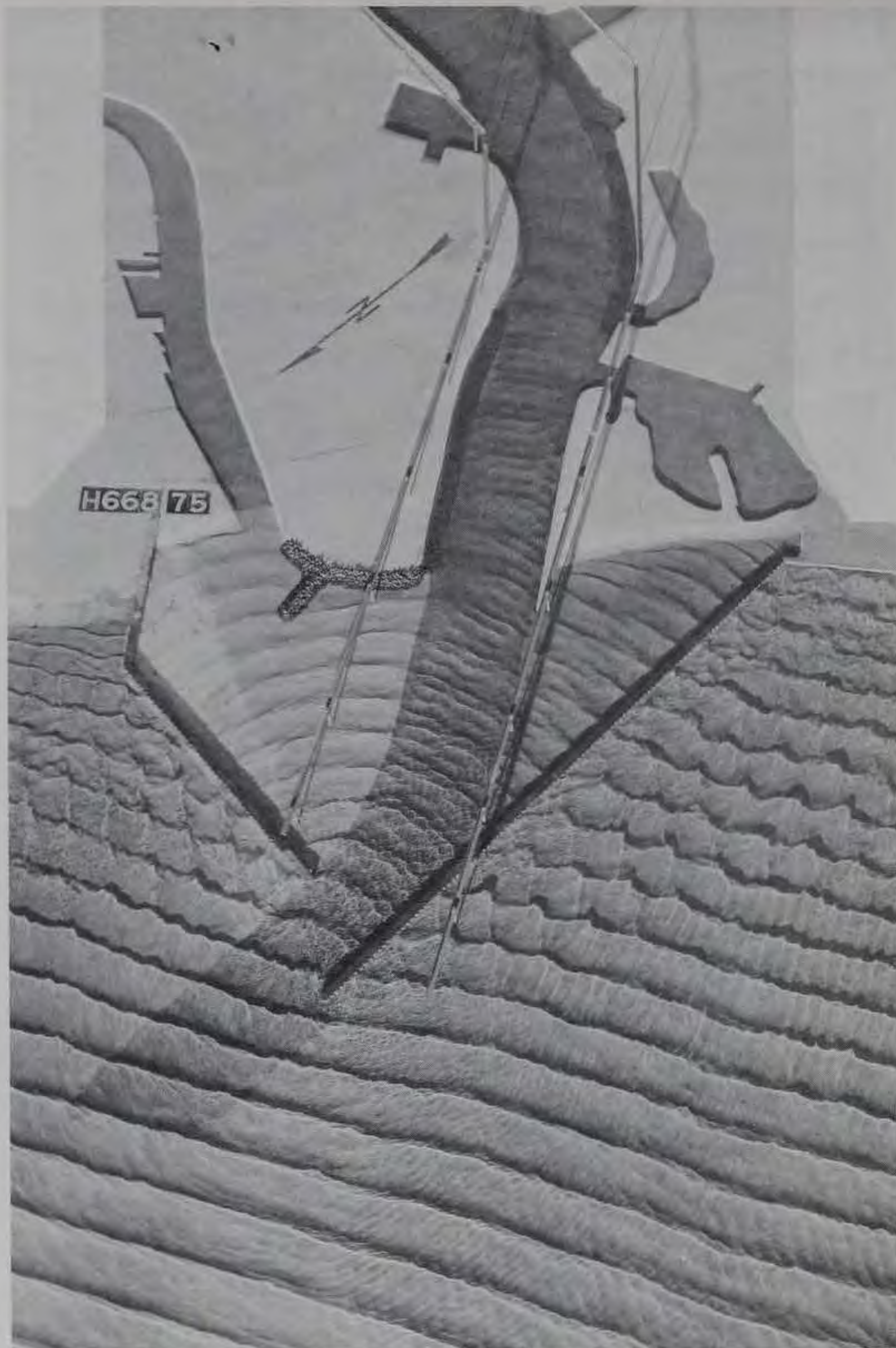
Photograph 30. Plan 7; 5-sec, 7-ft waves from north 25^{\circ} west
