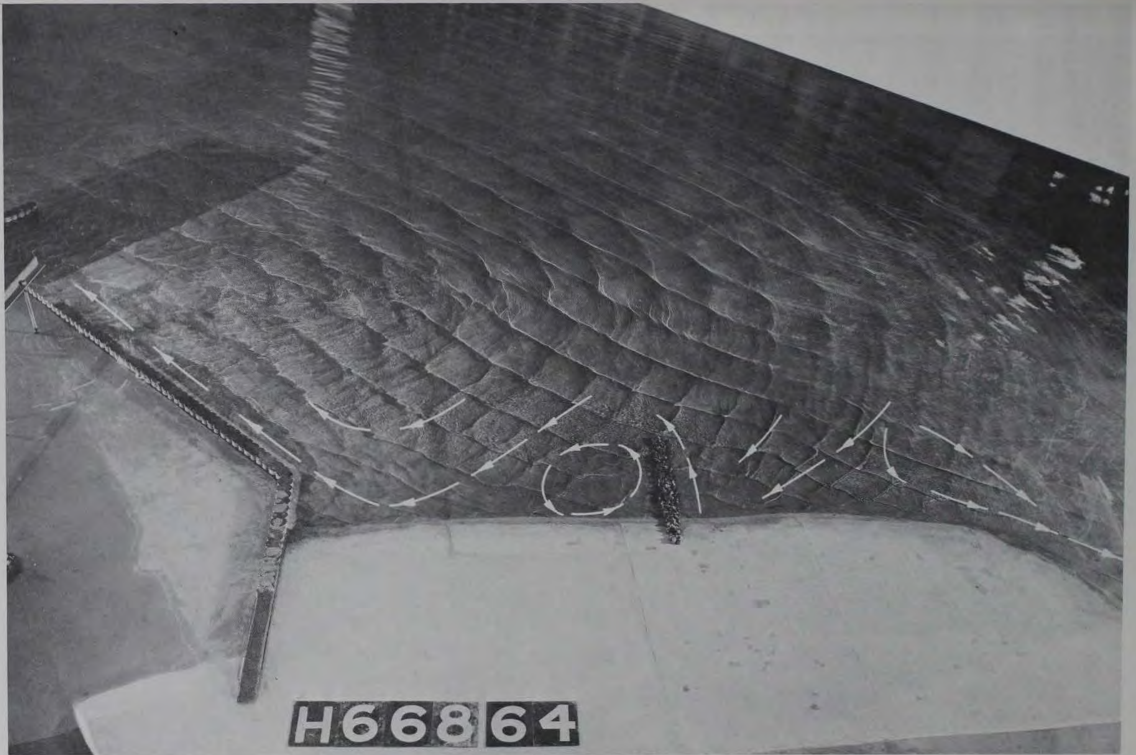
Photograph 24. Plan 7B; 5-sec, 5-ft waves from north 06^{\circ} east
