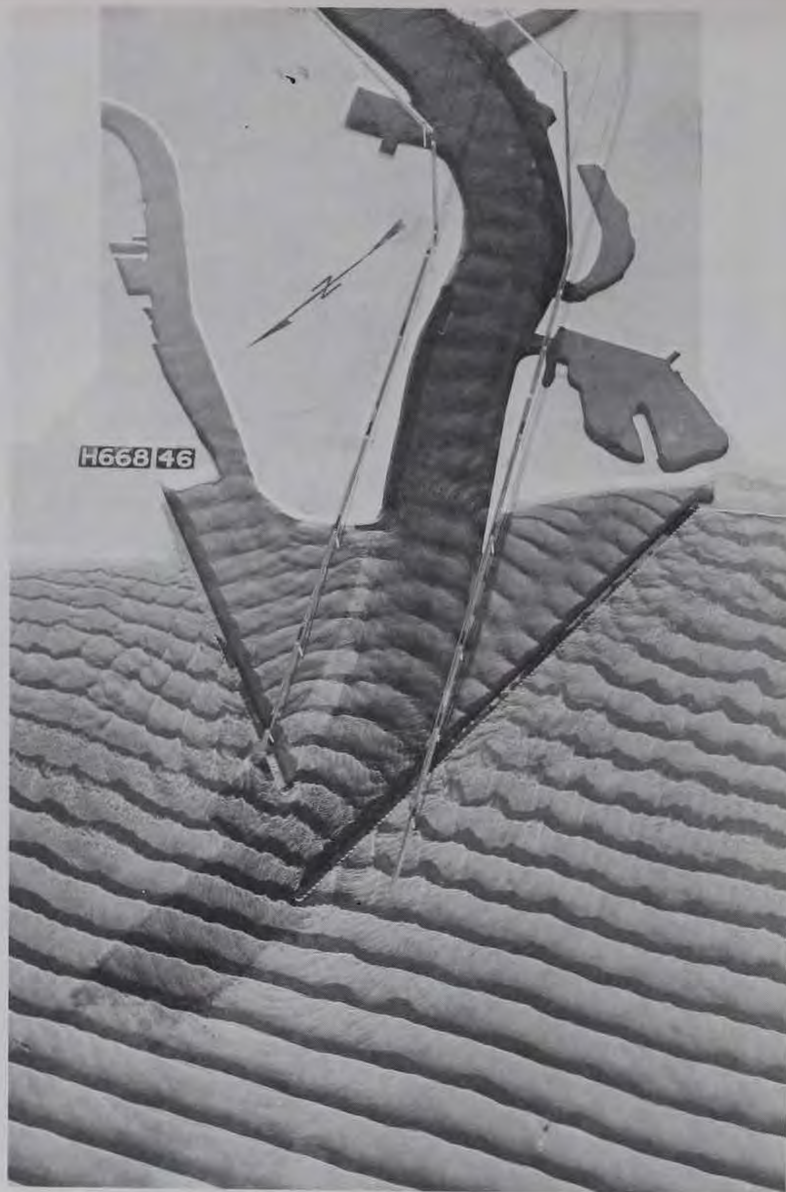
Photograph 12. Plan 6; 5-sec, 7-ft waves from north 25^{\circ} west
