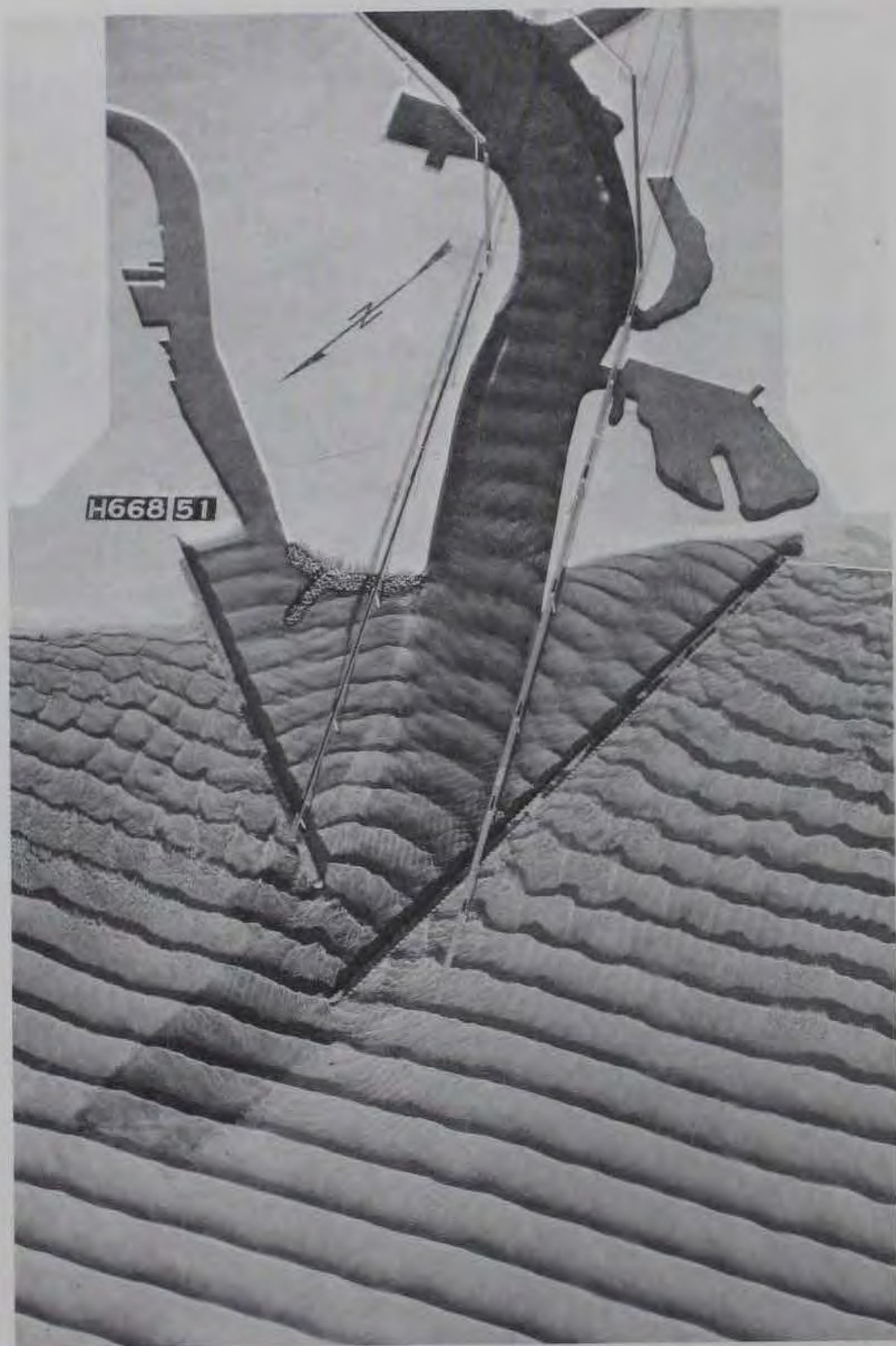
Photograph 14. Plan 6B; 5-sec, 7-ft waves from north 25^{\circ} west
