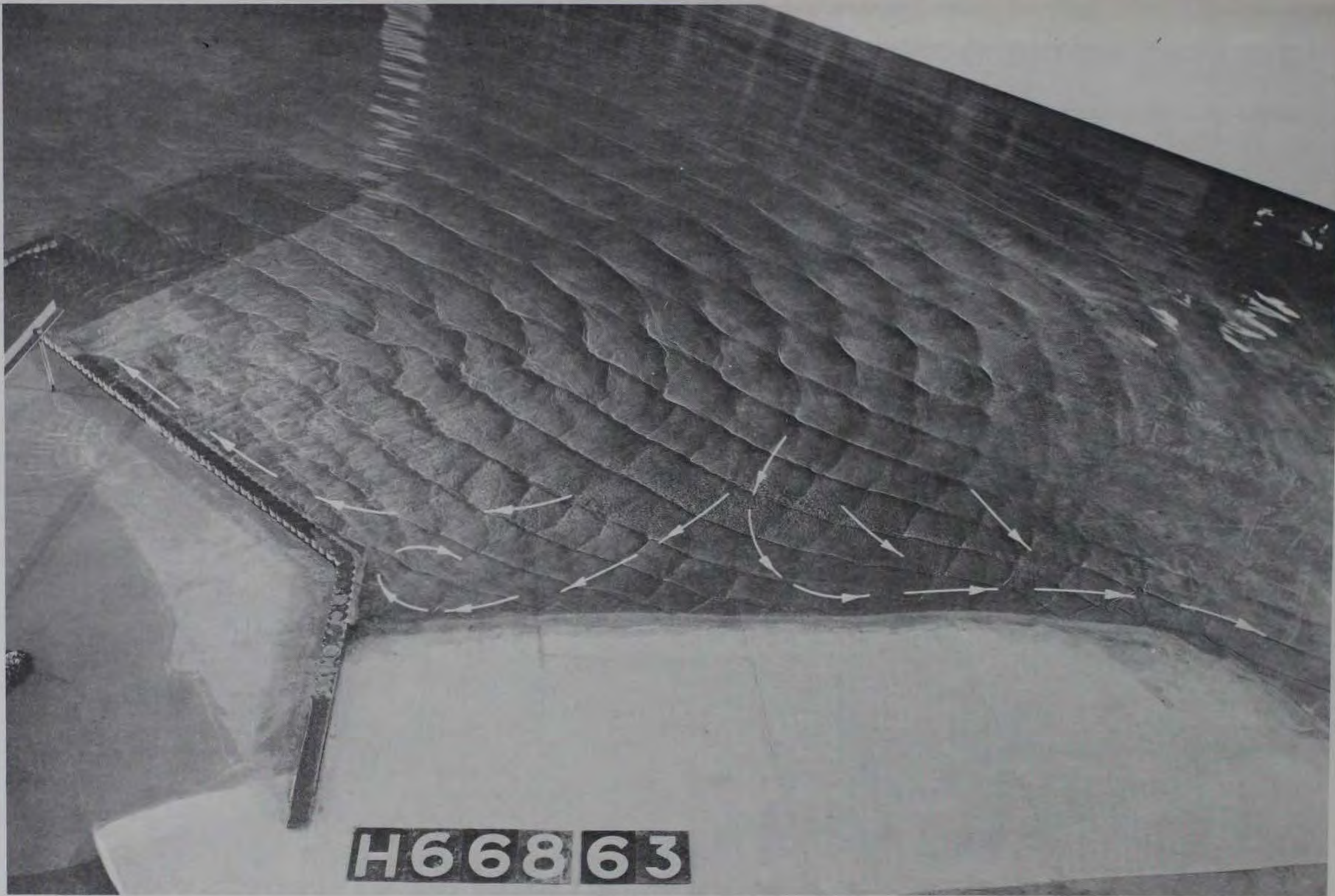
Photograph 22. Plan 7; 5-sec, 5-ft waves from north 06^{\circ} east
