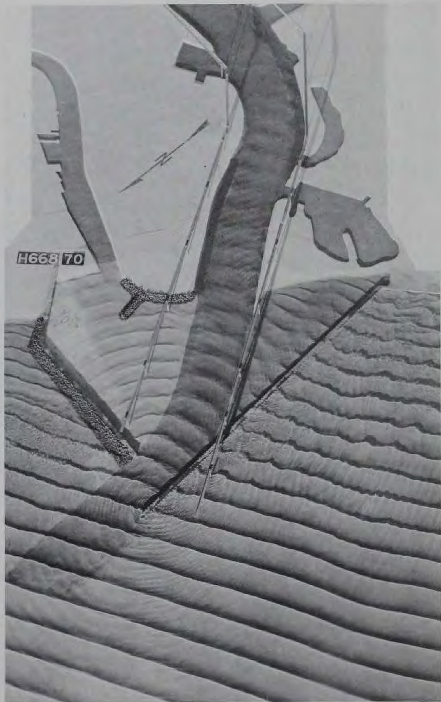
Photograph 32. Plan 7A; 5-sec, 7-ft waves from north 25^{\circ} west
