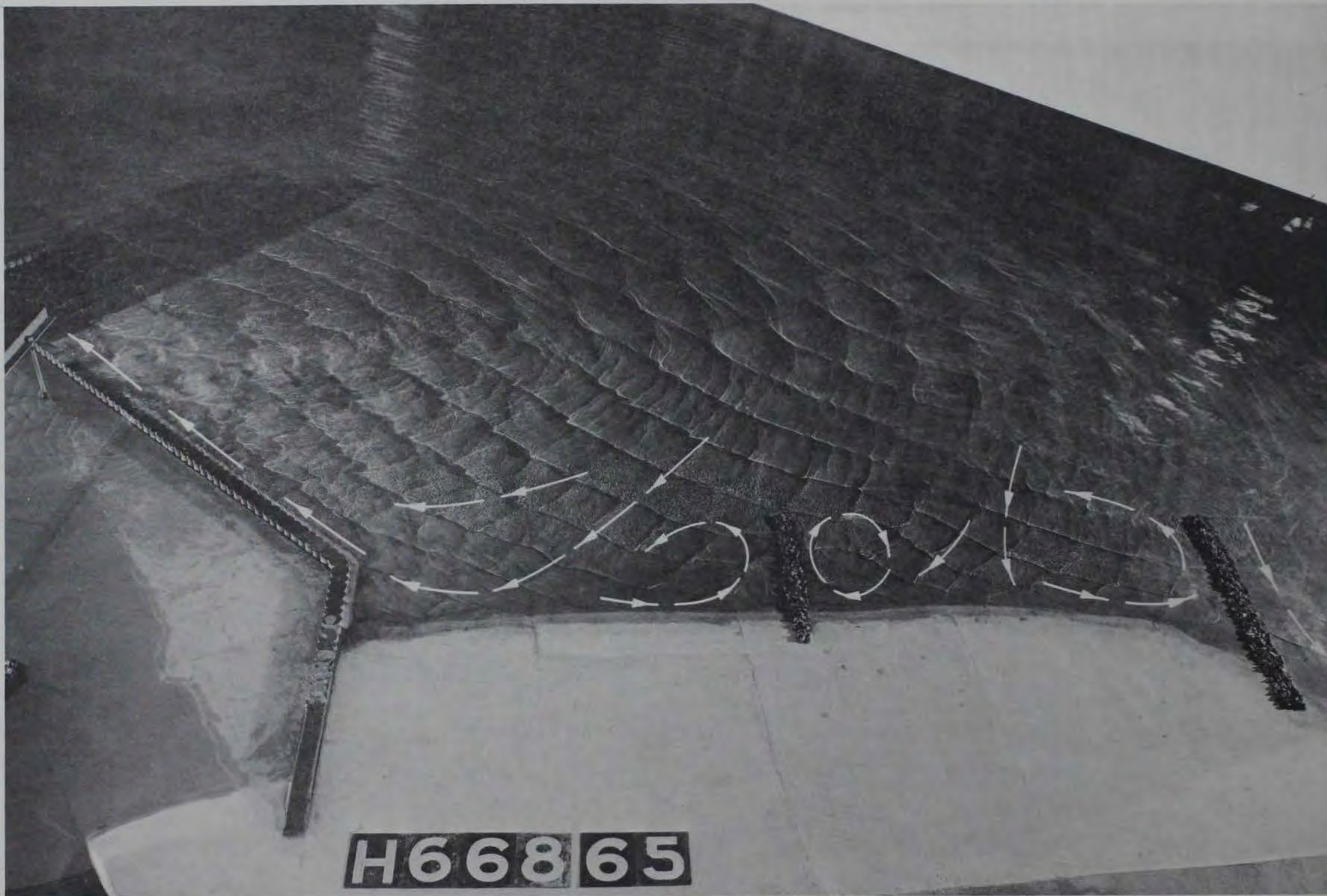
Photograph 25. Plan 7C; 5-sec, 5-ft waves from north 06^{\circ} east
