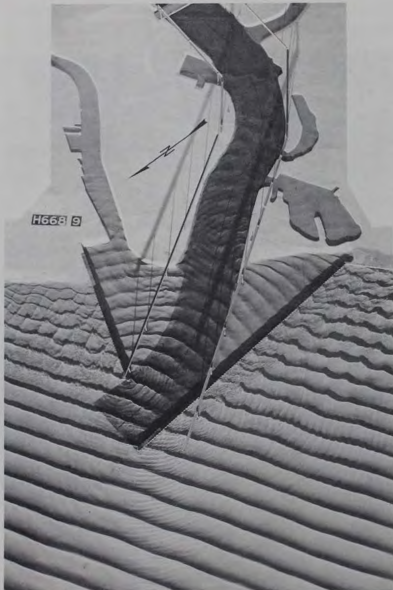
Photograph 2. Plan 1; 5-sec, 7-ft waves from north 25^{\circ} west
