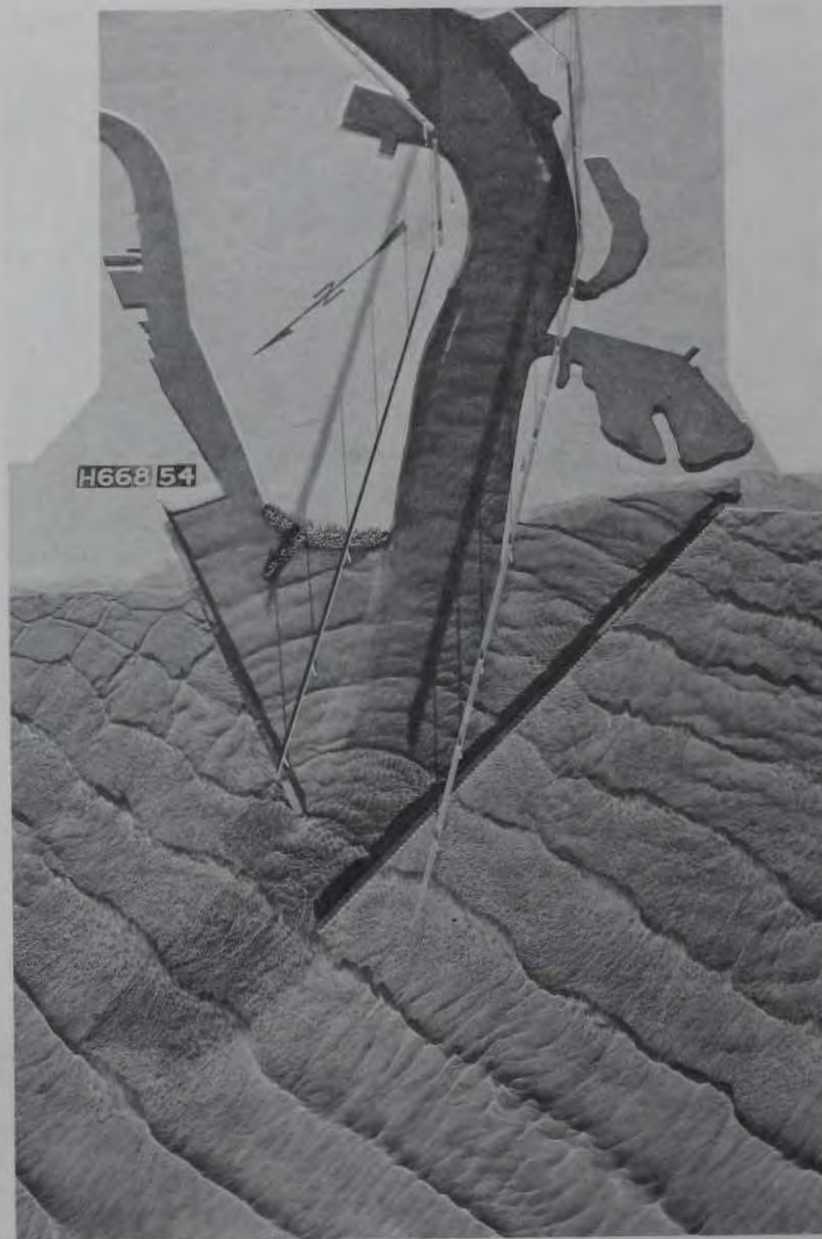
Photograph 15. Plan 6B; 9-sec, 10-ft waves from north 06^{\circ} east
