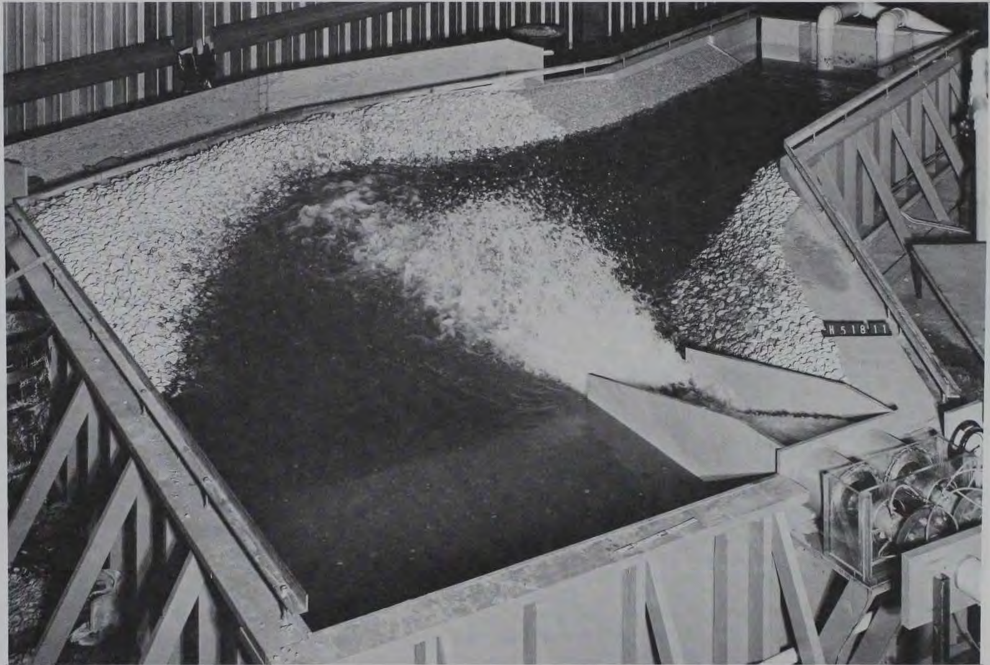
Photo 3. Plunge pool design, impingement pad removed, hood deflector and baffle blocks added; pool el 804, 32.4-in. sleeve travel, minimum tailwater
