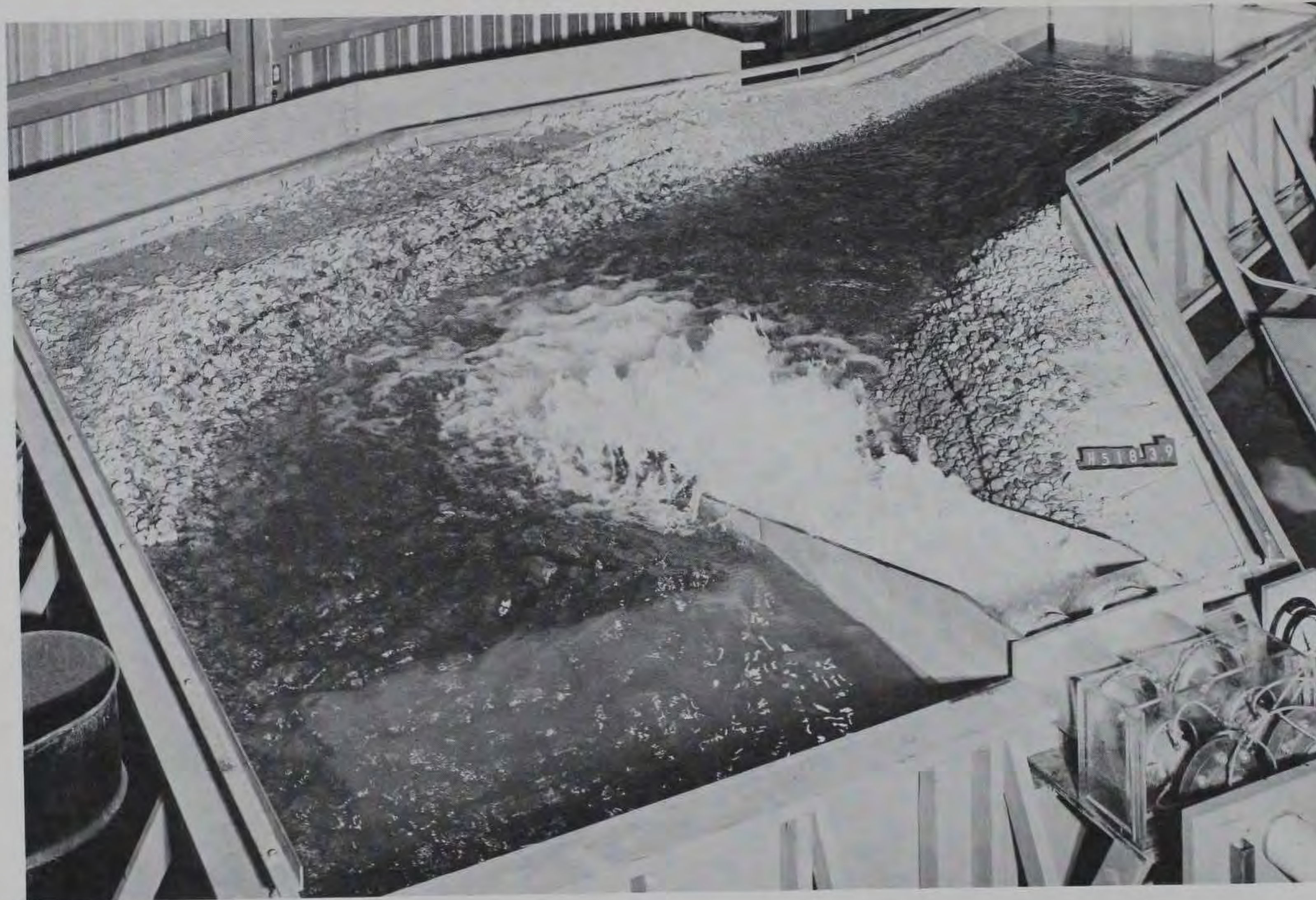
Photo 9. Recommended deflector plate design. Same flow as in Photo 9, showing attack on opposite bank
