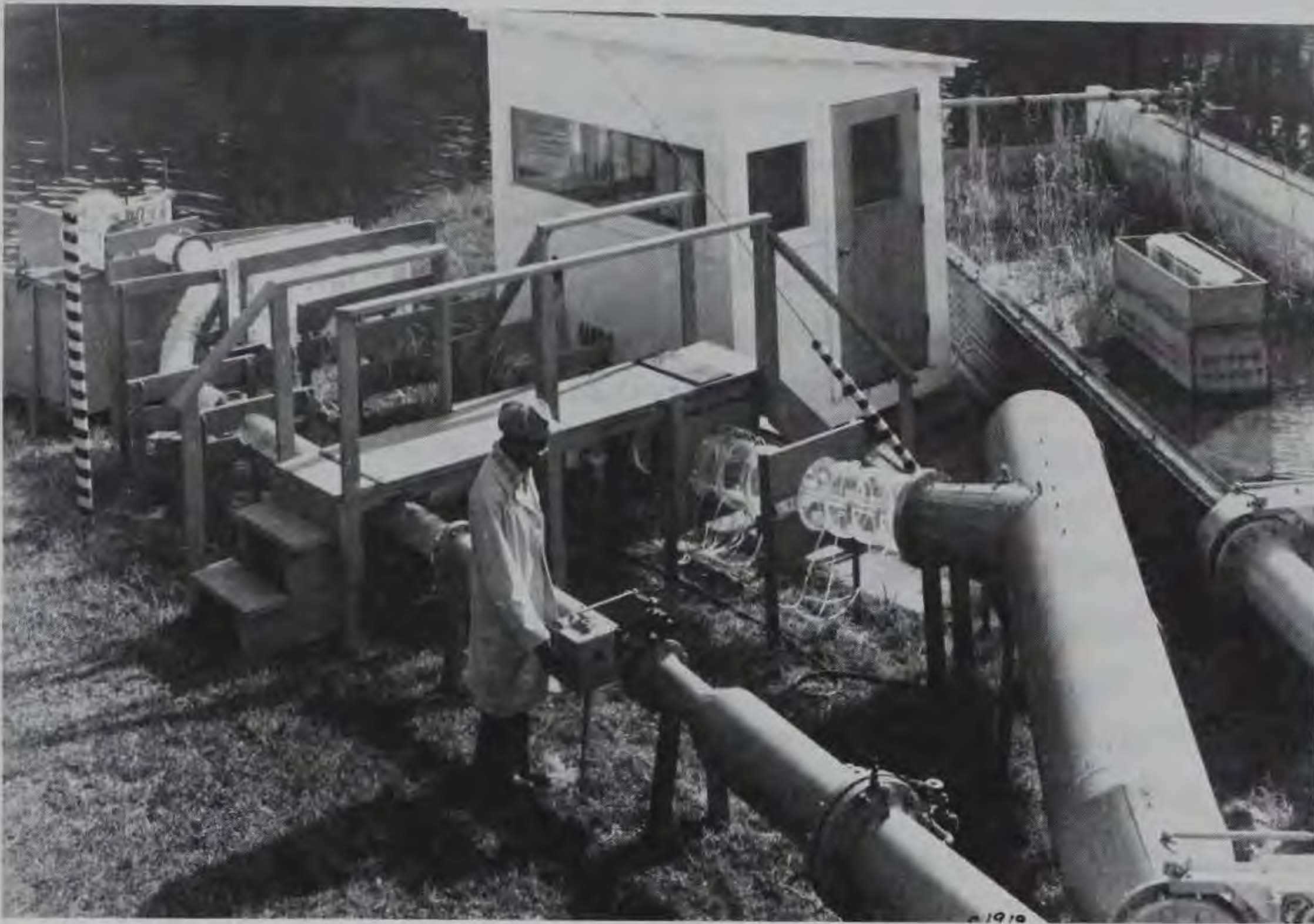
Figure 8. 1:12-scale model of New Melones fixed-cone valve
