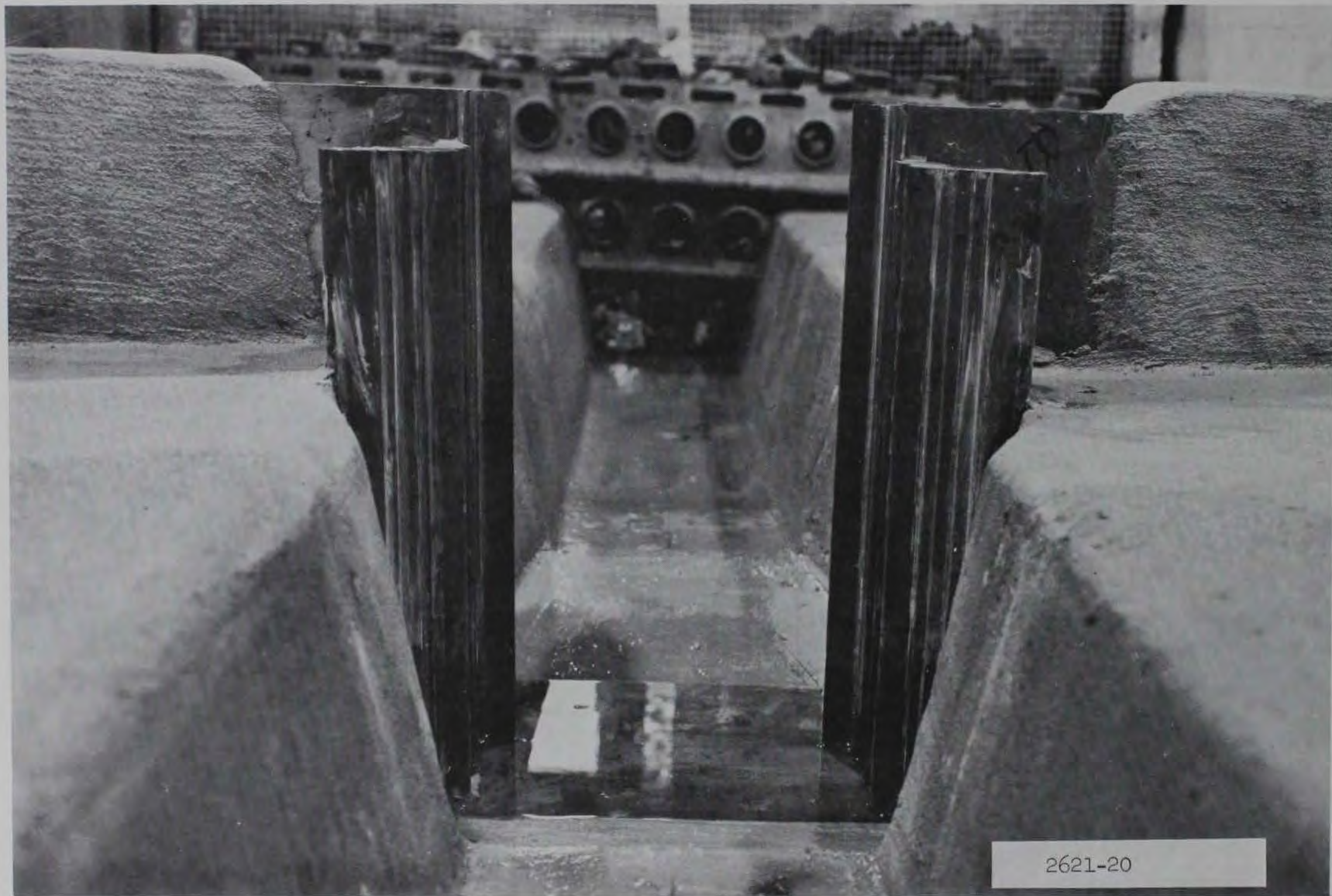
Photo B9. Gamma plan, distorted-scale model of the navigation structure, water-level view
