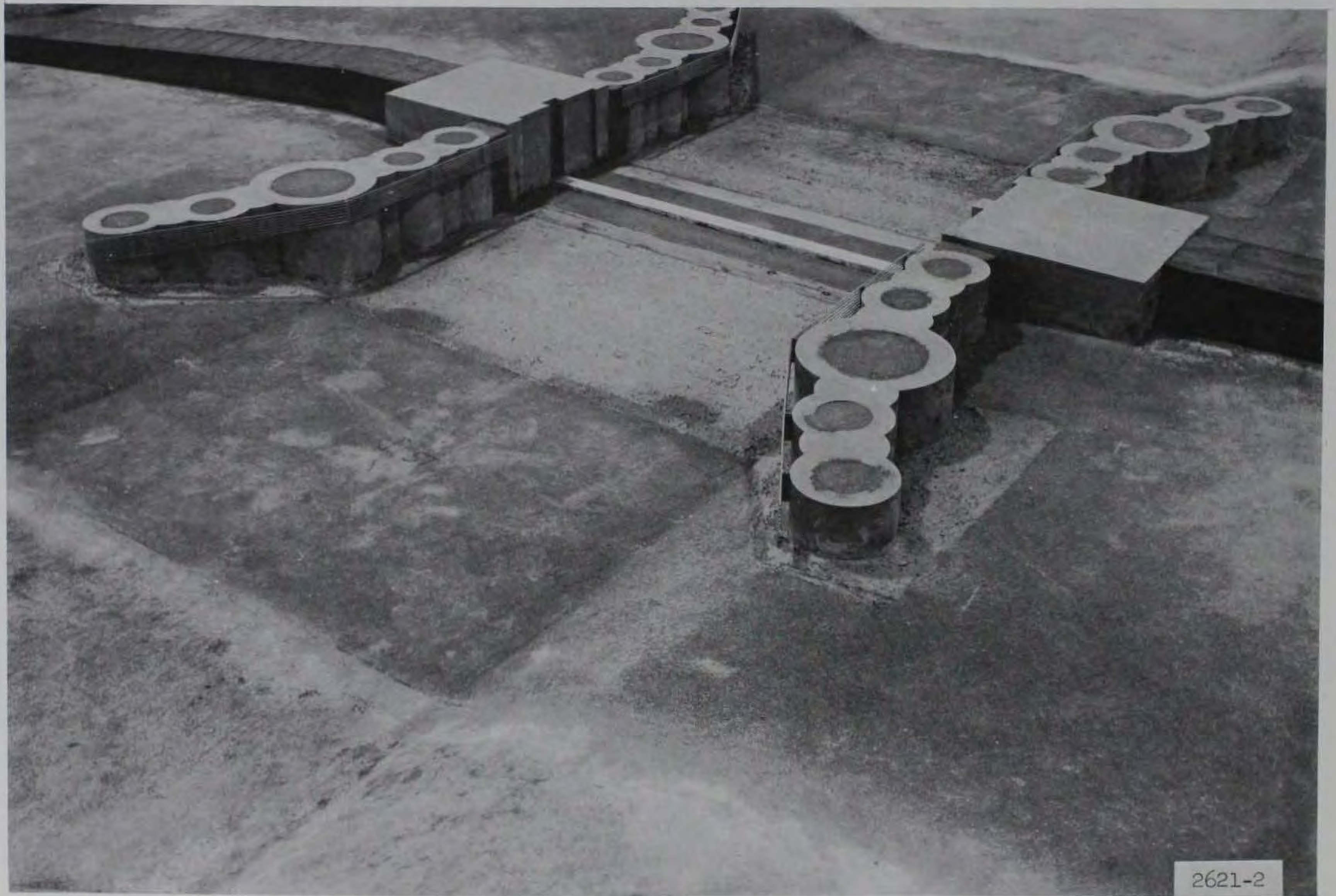
Photo B5. Gamma plan, undistorted-scale model of the navigation structure
