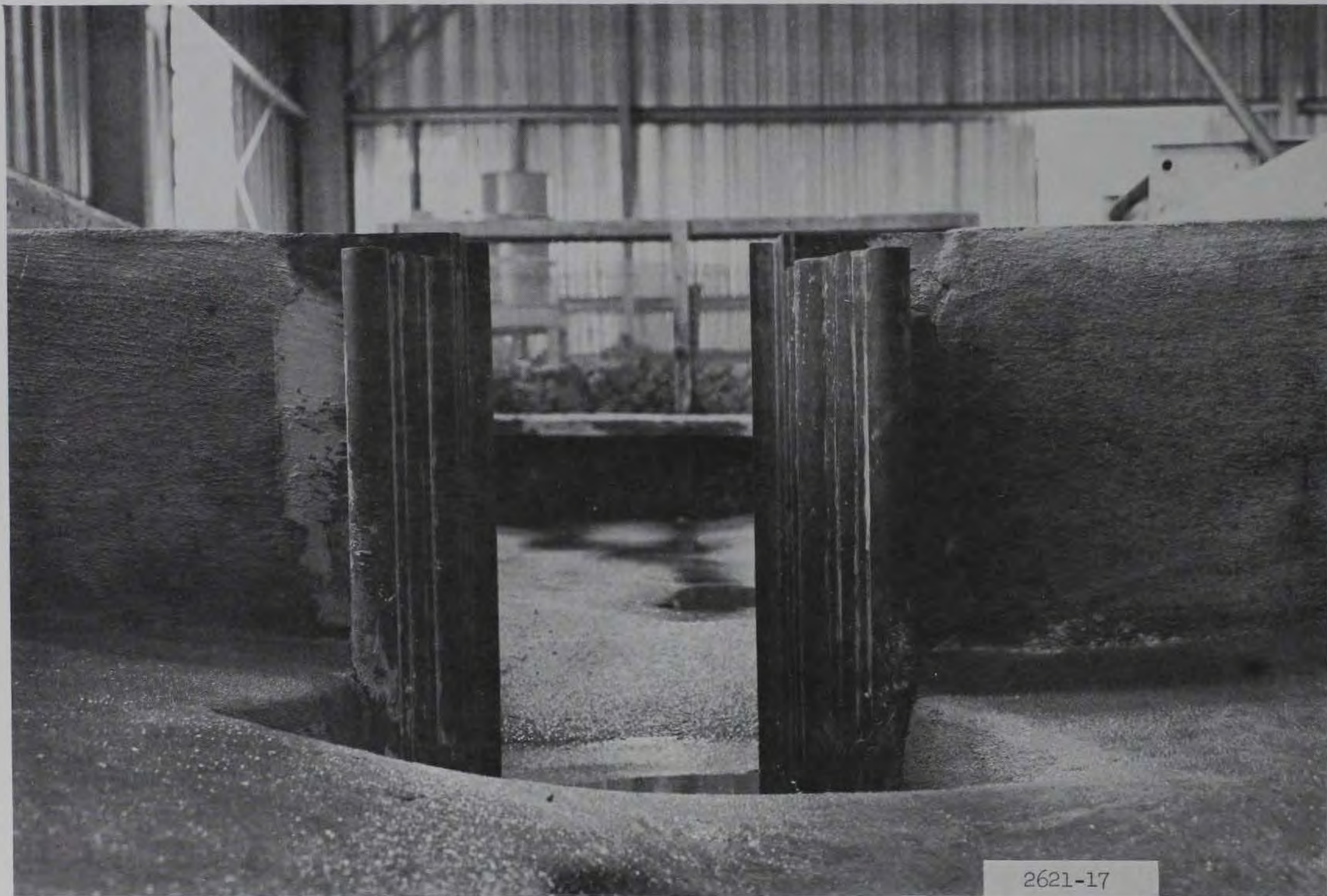
Photo B7. Alpha plan, distorted-scale model of the navigation structure, water-level view from the bay
