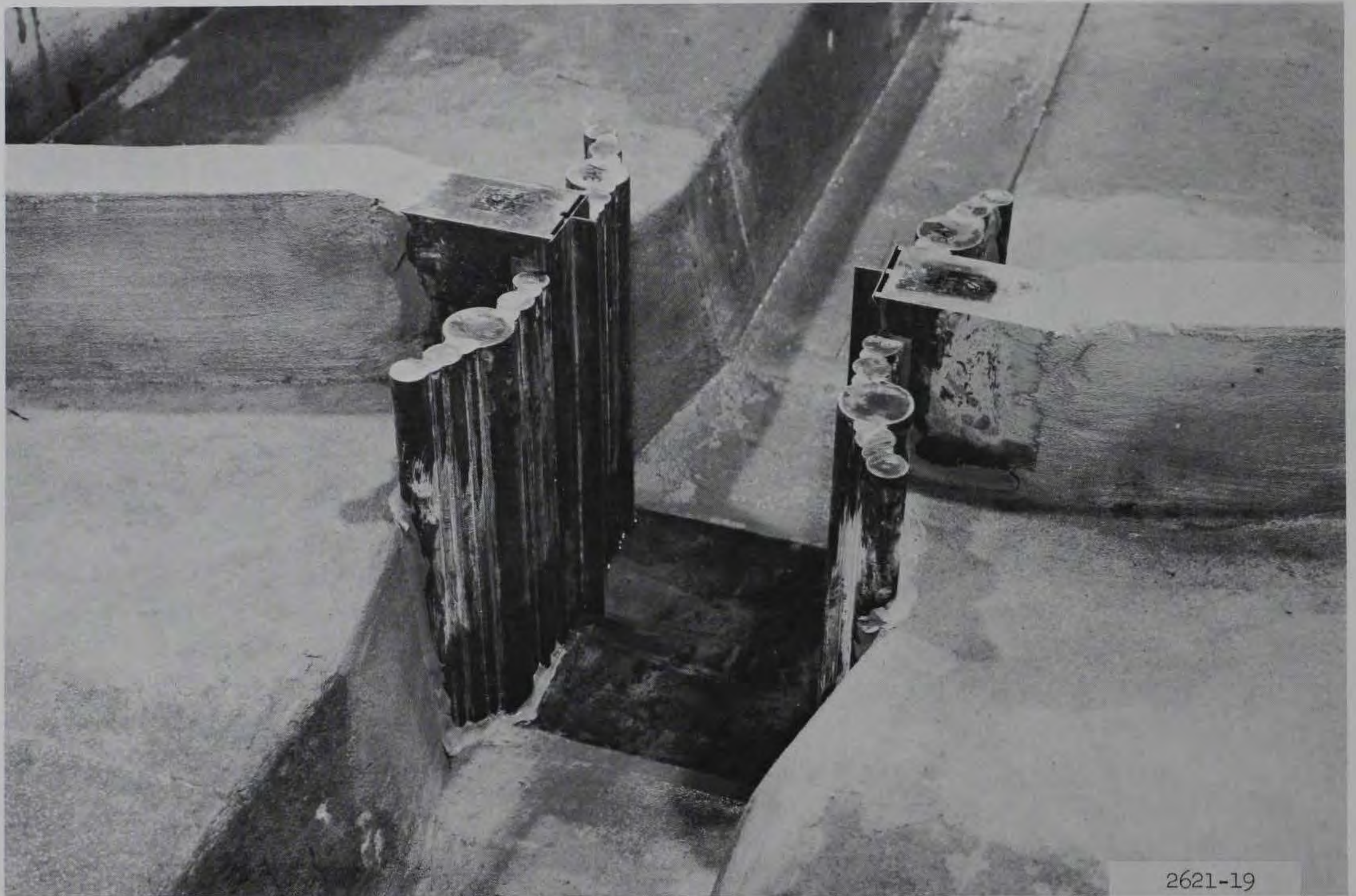
Photo B8. Gamma plan, distorted-scale model of the navigation structure, overhead view
