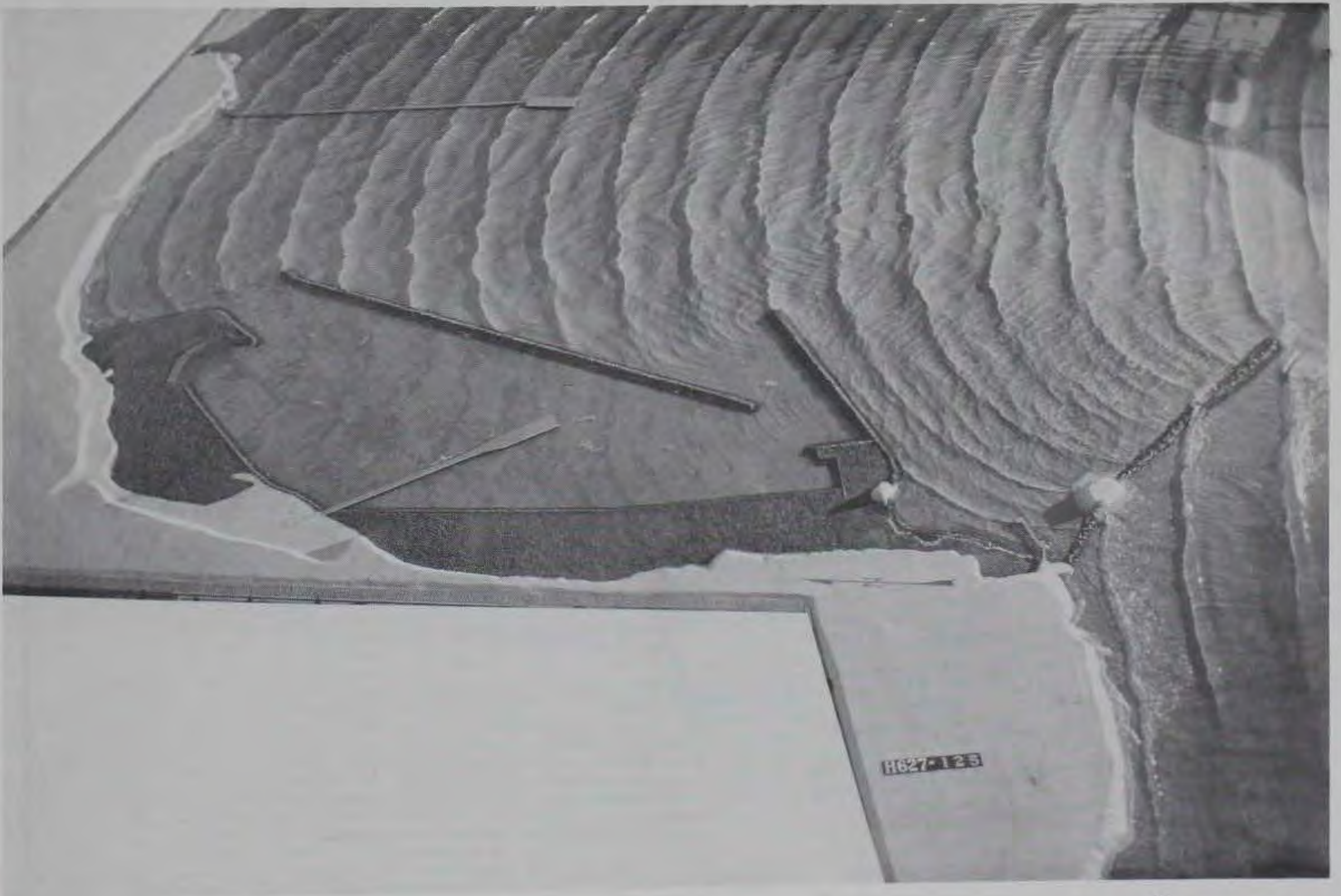
Photograph 14. Plan 12; 14-sec, 18-ft waves from south 16^{\circ} west
