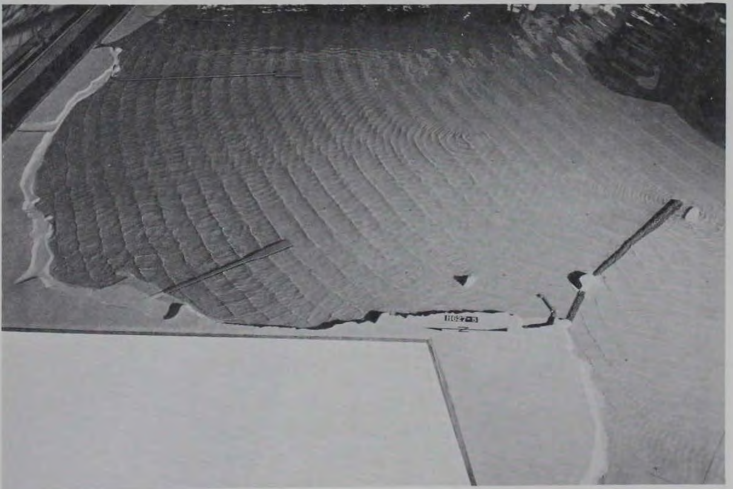
Photograph 2. Base test; 9-sec, 10-ft waves from south 25^{\circ} east
