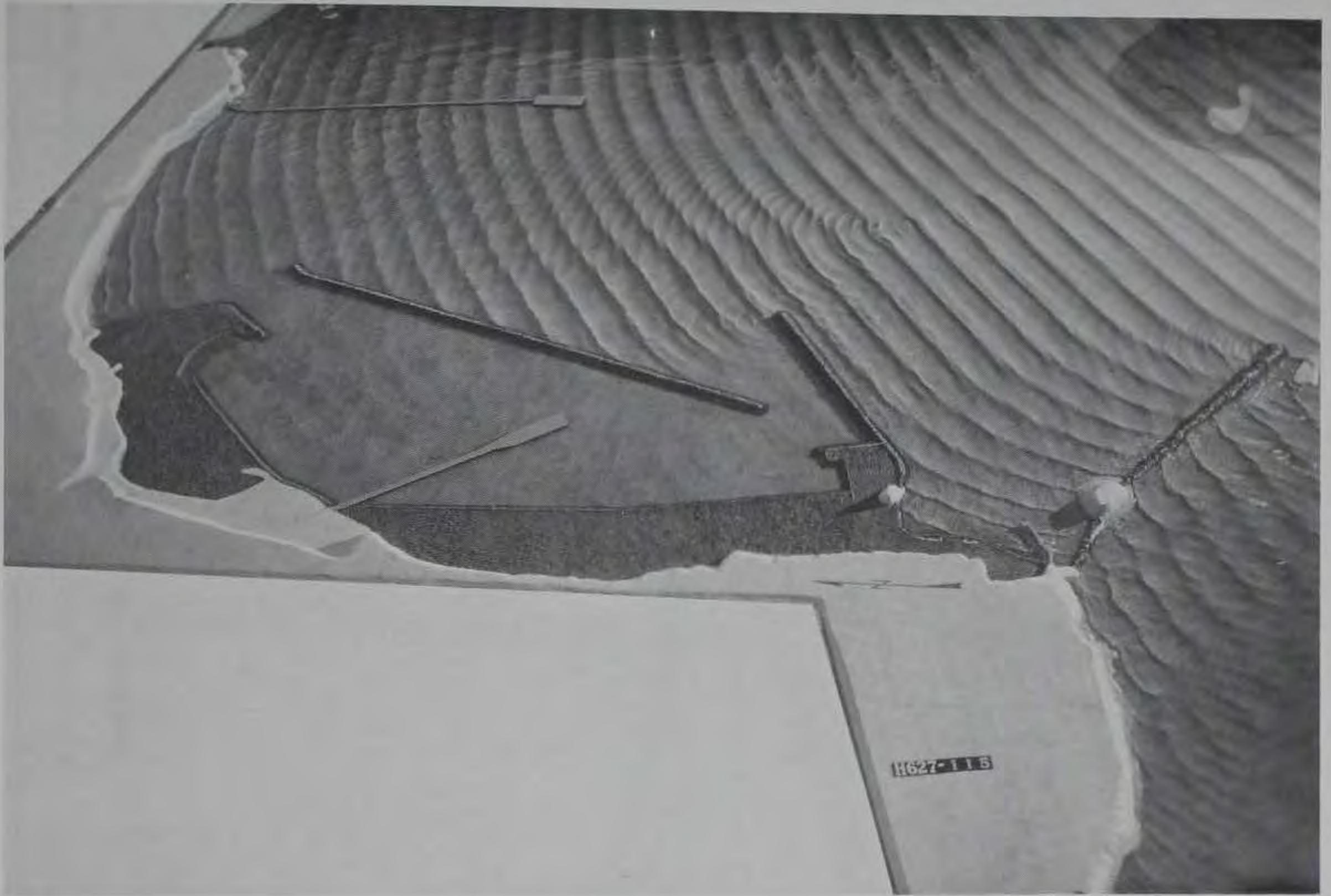
Photograph 13. Plan 12; 9-sec, 10-ft waves from south 25^{\circ} east
