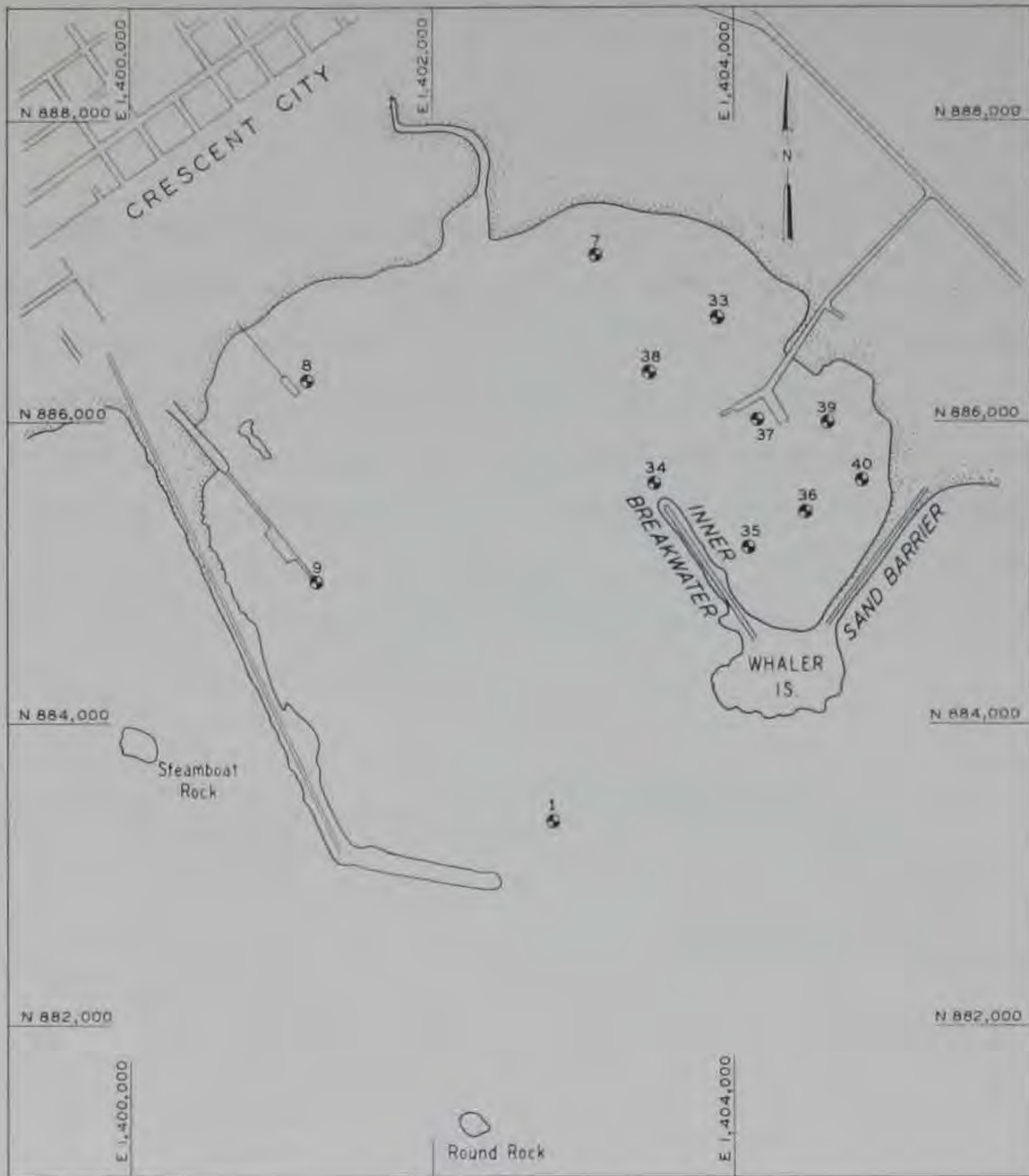
Fig. A1. Location of wave gages
