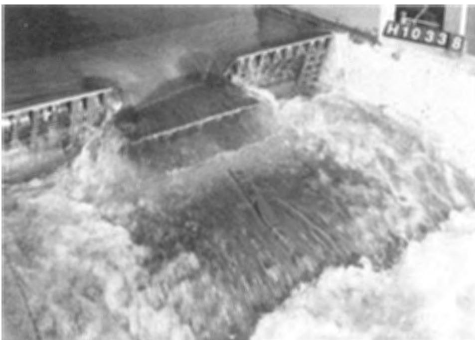
b. Pool el 118.2; center gate 60 deg; side gates 70 deg
