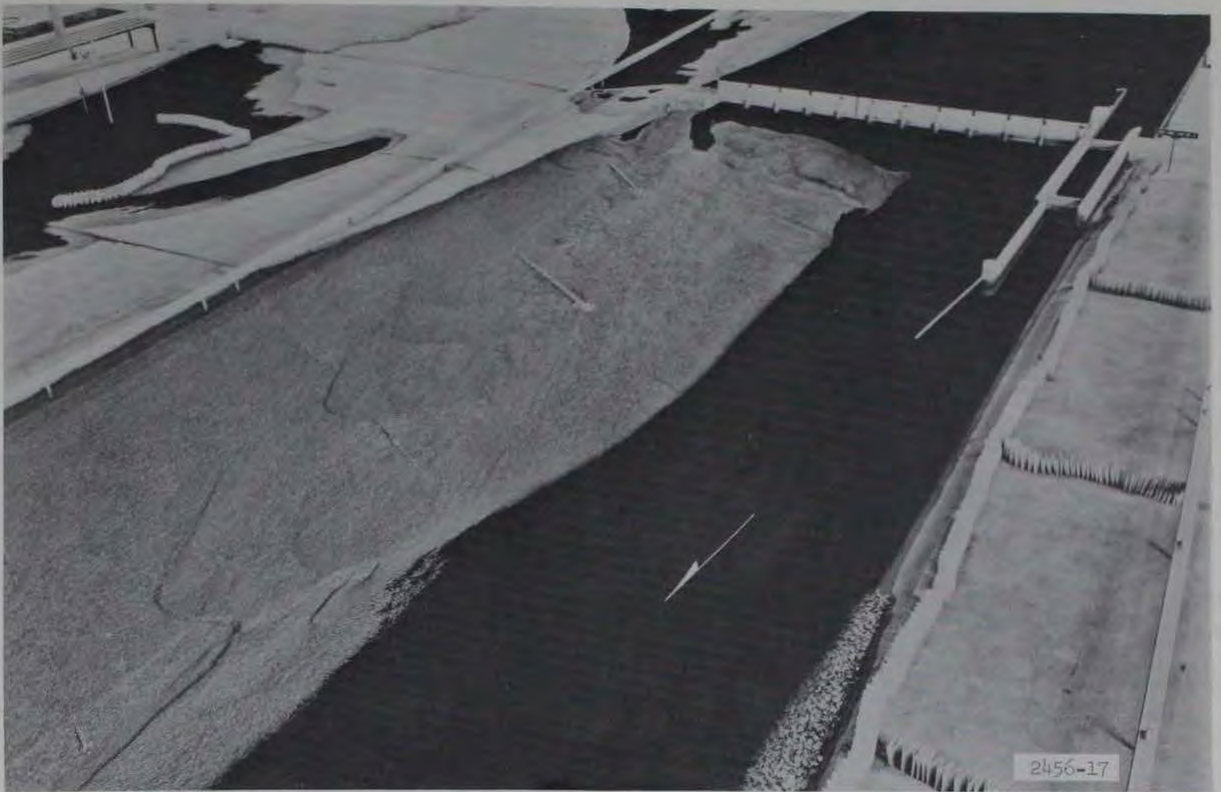
Photograph 5. Plan A-3, run 1, -1.0-ft stage. Bed configuration downstream of dam. Note bar in front of right bank dikes
