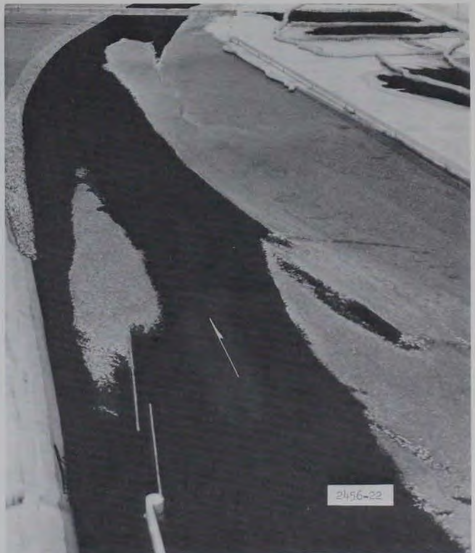
Photograph 5. Plan A-3, run 1, -1.0-ft stage. Bed configuration downstream of dam. Note bar in front of right bank dikes
