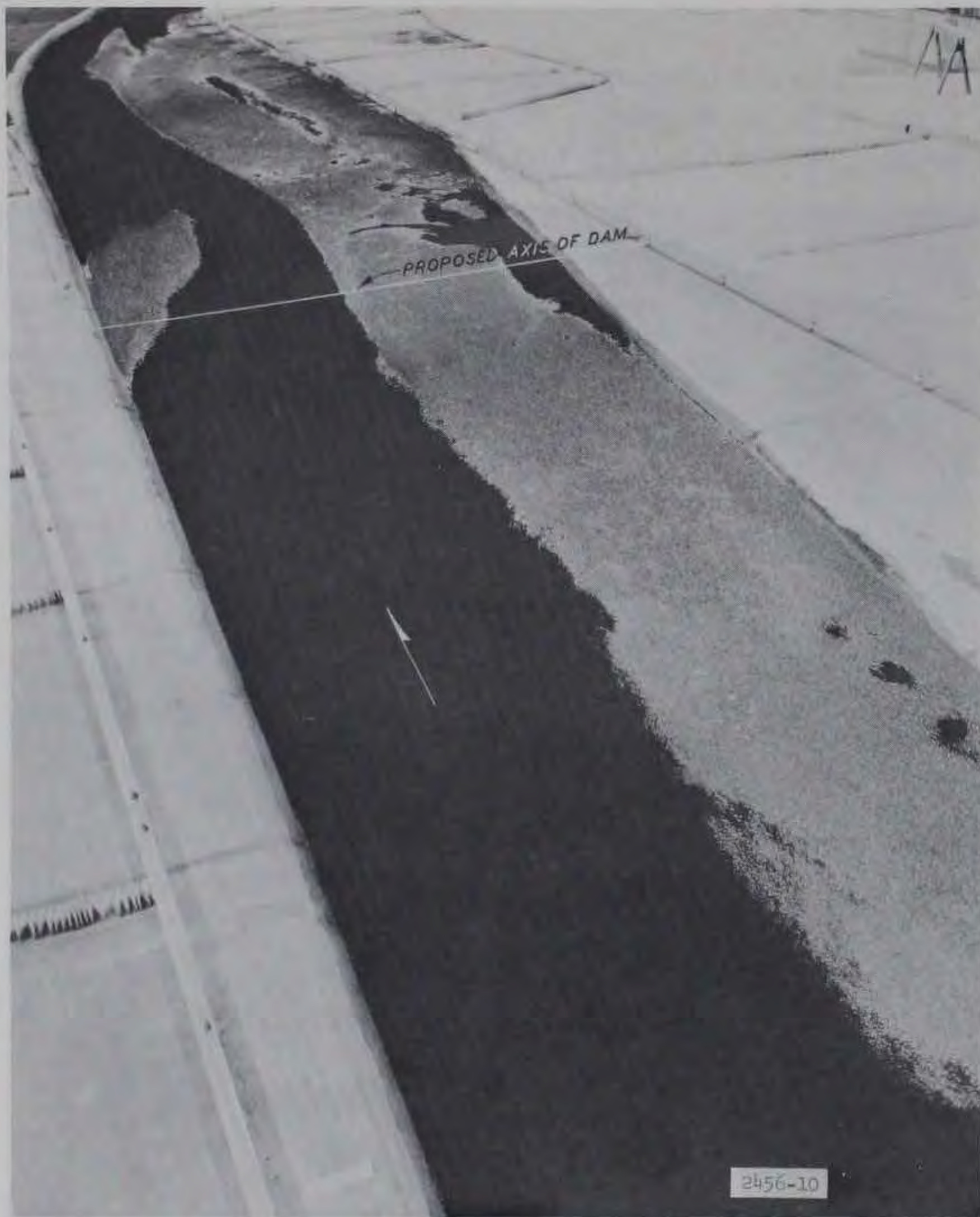
Photograph 1. Base test, run 1, 0-ft stage. View from about mile 73.0, showing bar formation along left bank near proposed damsite, indicating tendency for channel to meander
