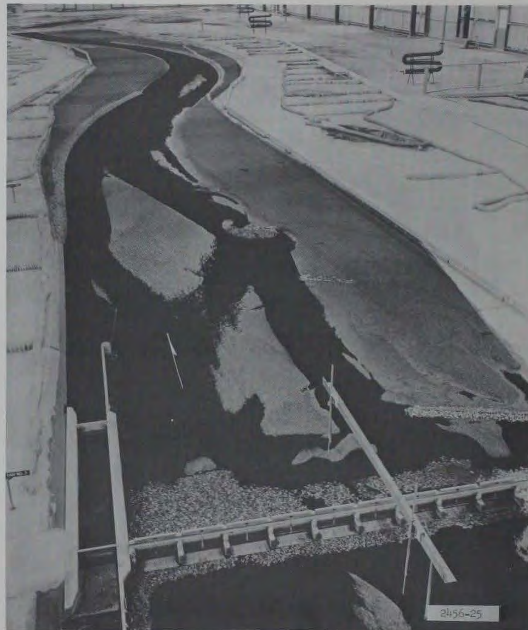
Photograph 8. Plan A-5, run 4, water-surface el 164.0. Note bar formation and division of channels below the dam
