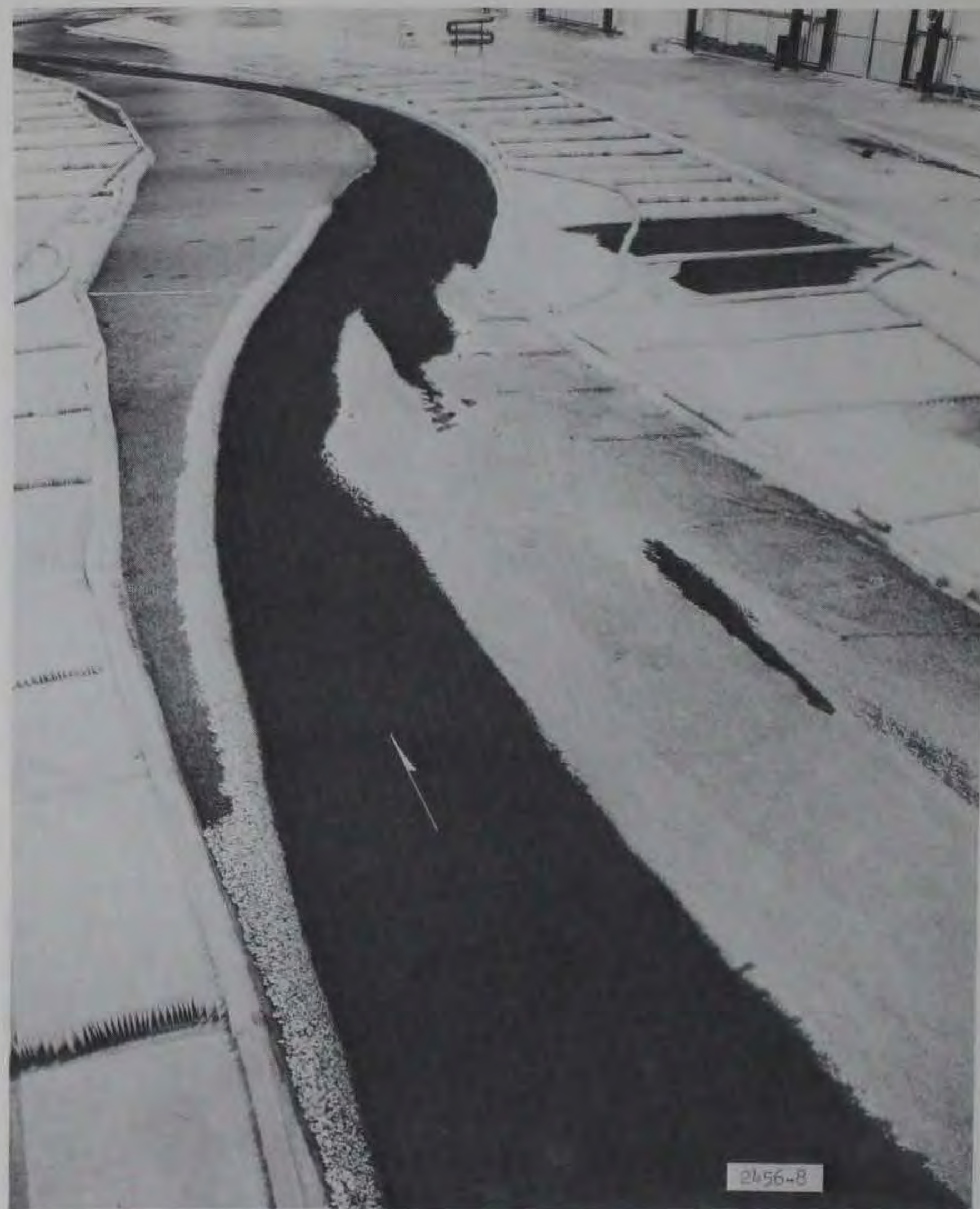
Photograph 2. Base test, run 1, 0-ft stage. View from about mile 72.2 showing channel along pile revetment downstream of proposed damsite
