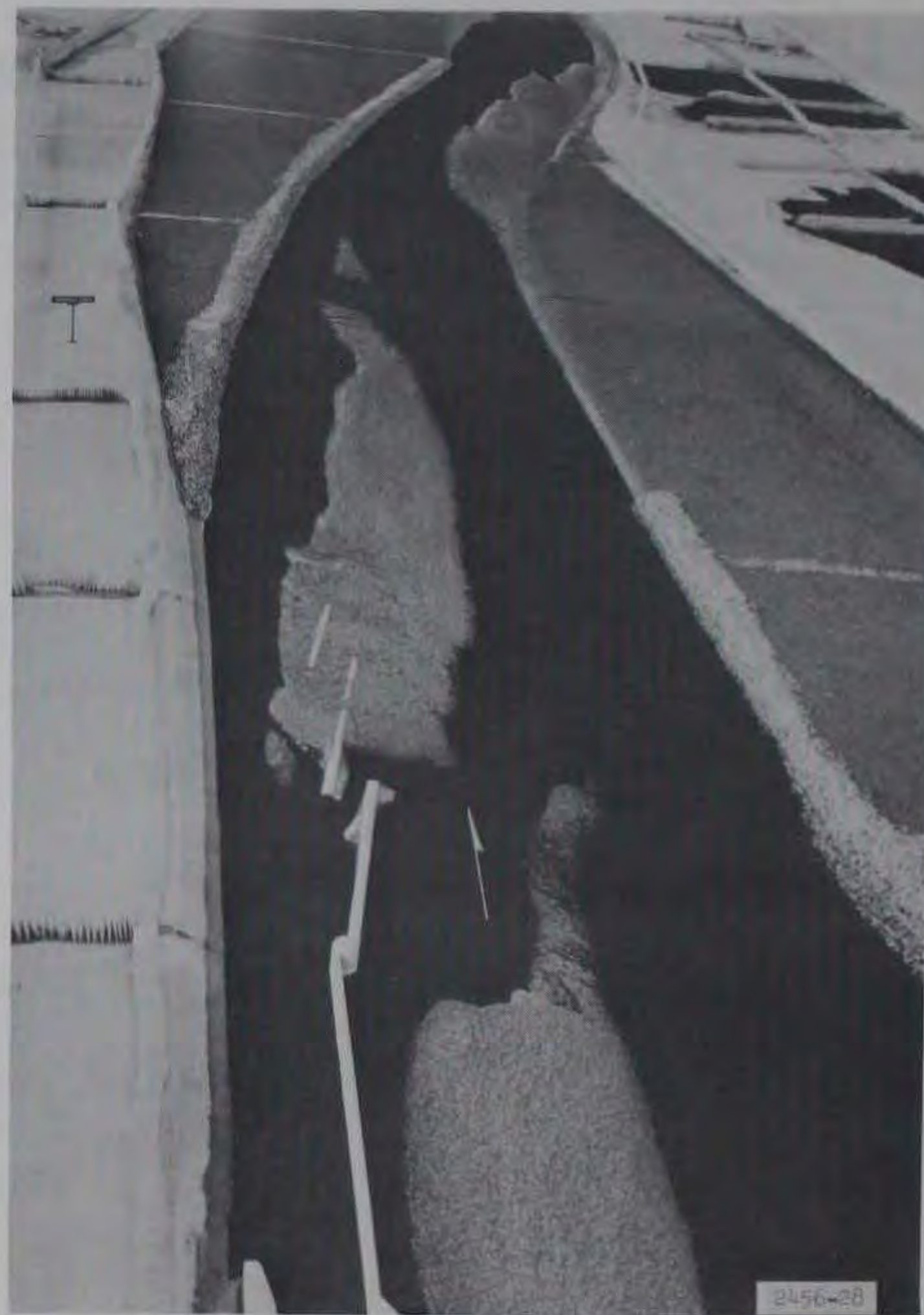
Photograph 10. Plan A-10, run 1, -1.0-ft stage. End of lower guard wall and wing dikes downstream. Note deposition over and downstream of lower two wing dikes and in lock approach channel
