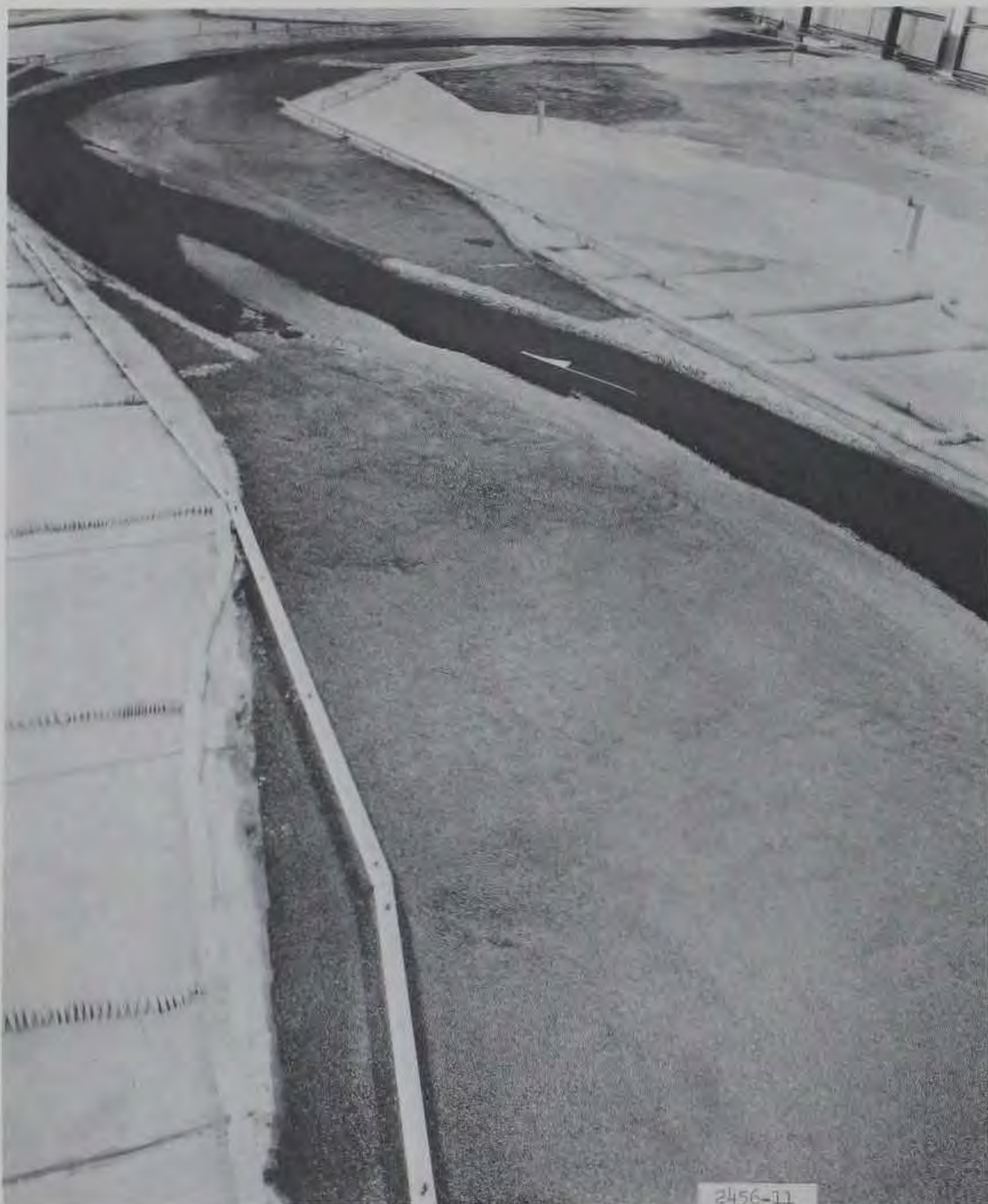
Photograph 3. Base test, run 1, 0-ft stage. View from about mile 69.4 showing crossing at mile 68.5 and channel into and through cutoff
