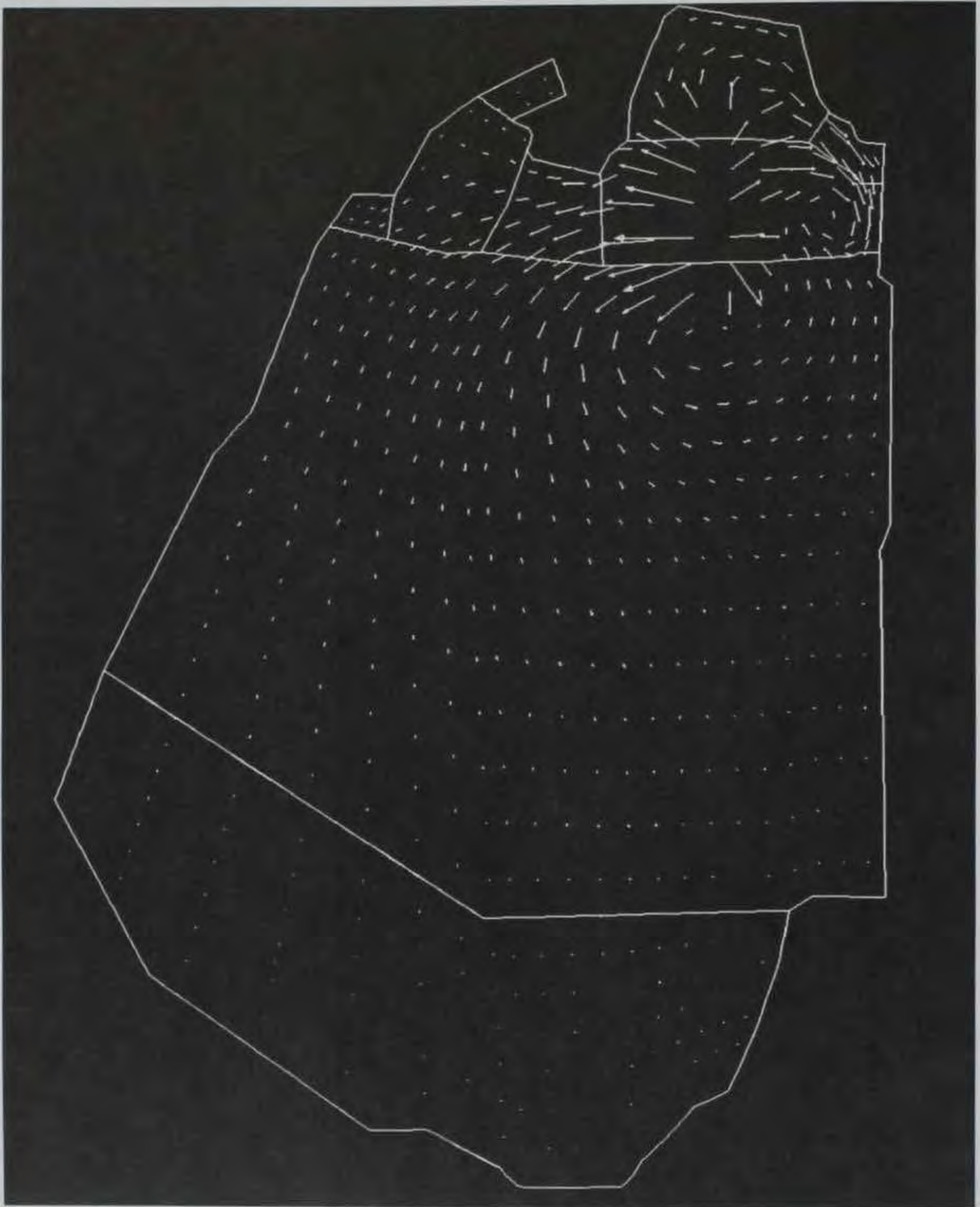
Figure 14. Surface velocities for cold reservoir with cold inflow
