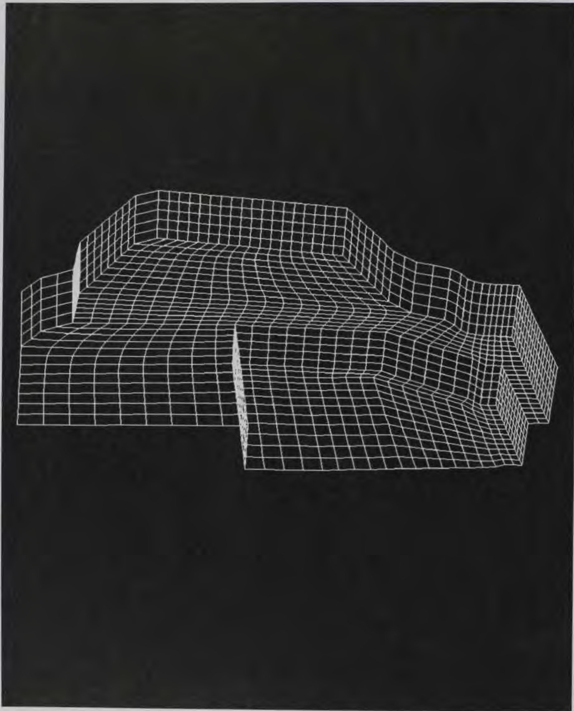
Figure 8. Cutaway of bottom and side grids in and around sump
