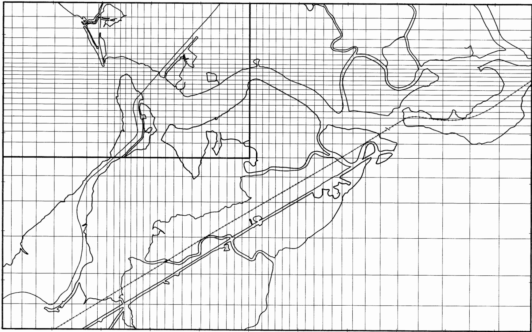
Figure 9. Sectional grid for The Rigolets computational model
