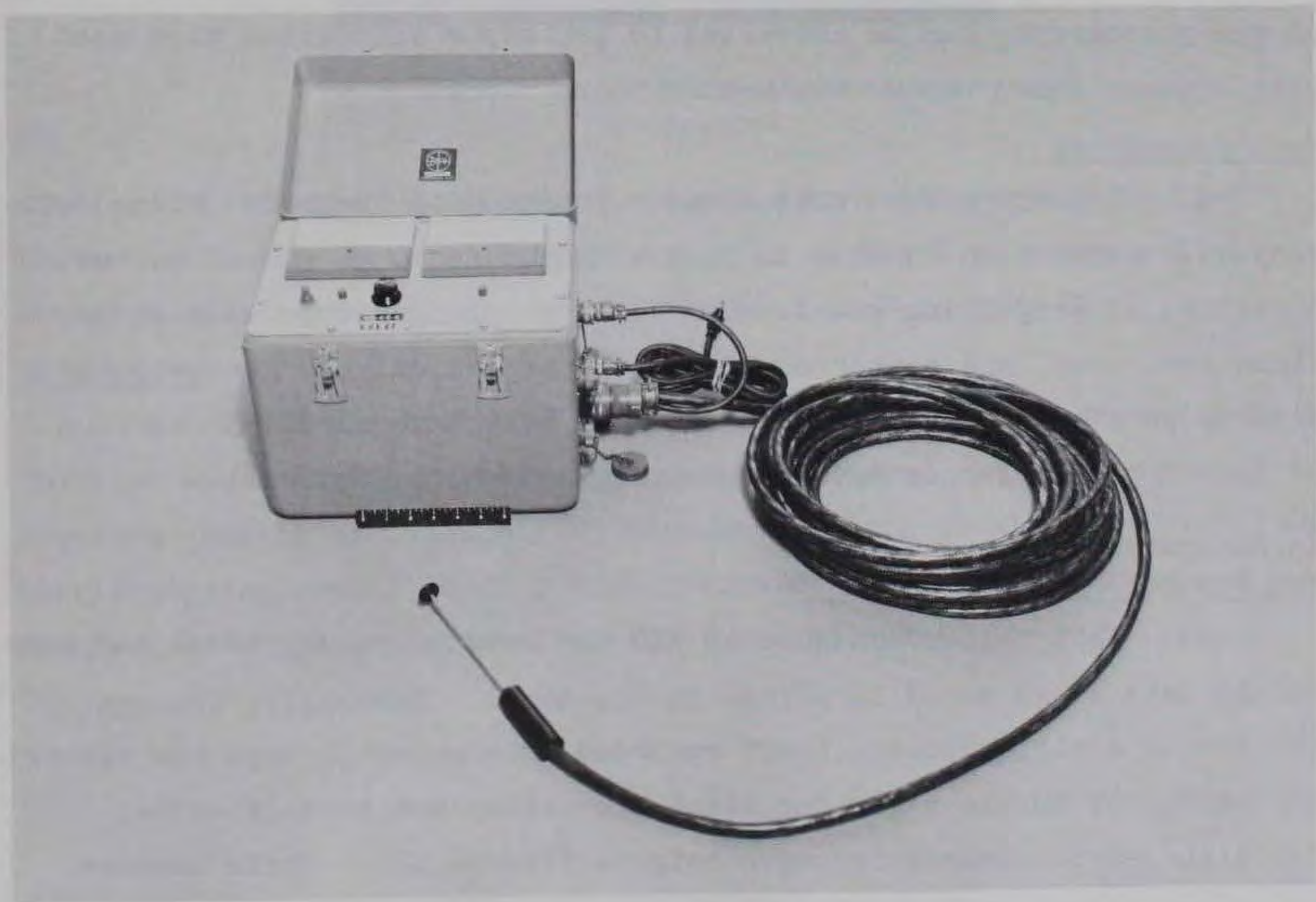
Figure 10. Electromagnetic current meter
