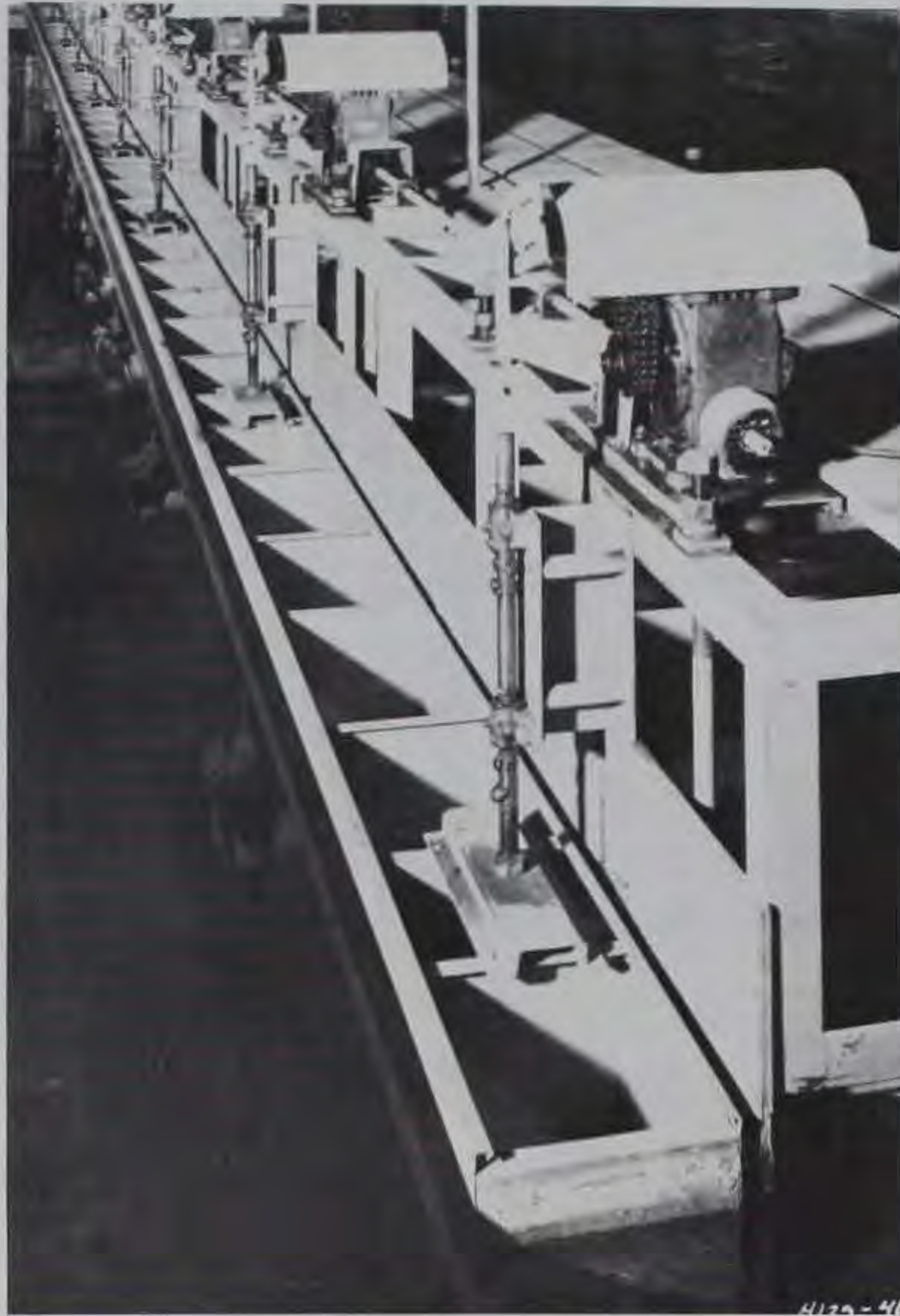
Figure 11. Vertical plunger wave generator
