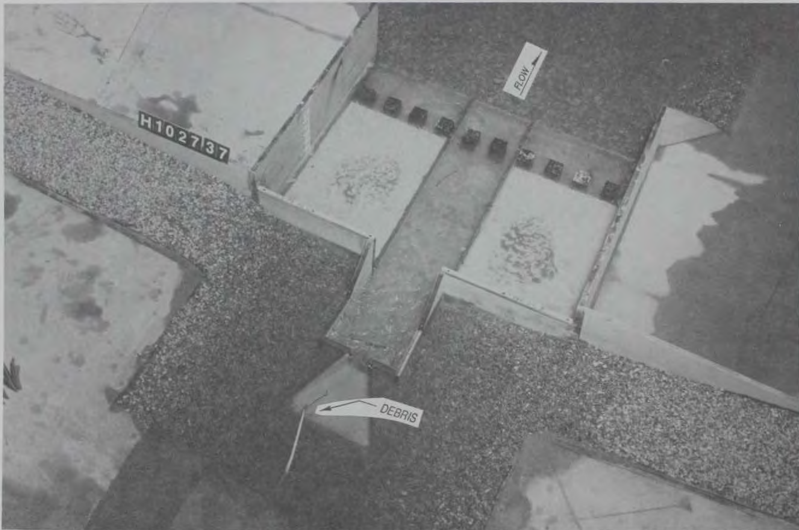
Photo 14. Type 2 debris deflectors, debris passage looking downstream, discharge 142 cu m/sec (5,000 cfs), tailwater el 741.44
