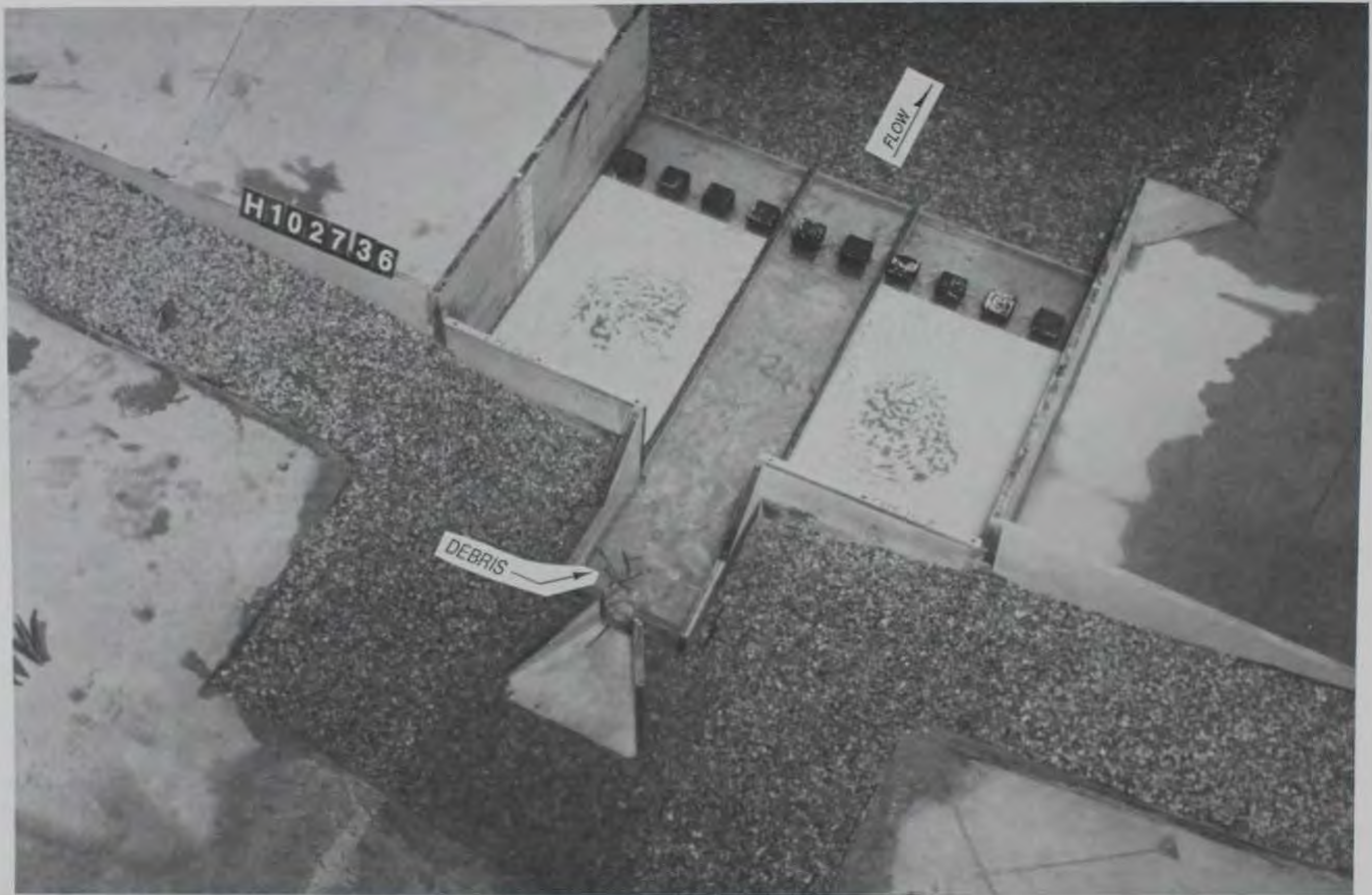
Photo 13. Type 2 debris deflectors, debris passage looking downstream, discharge 28 cu m/sec (1,000 cfs), tailwater el 735.54
