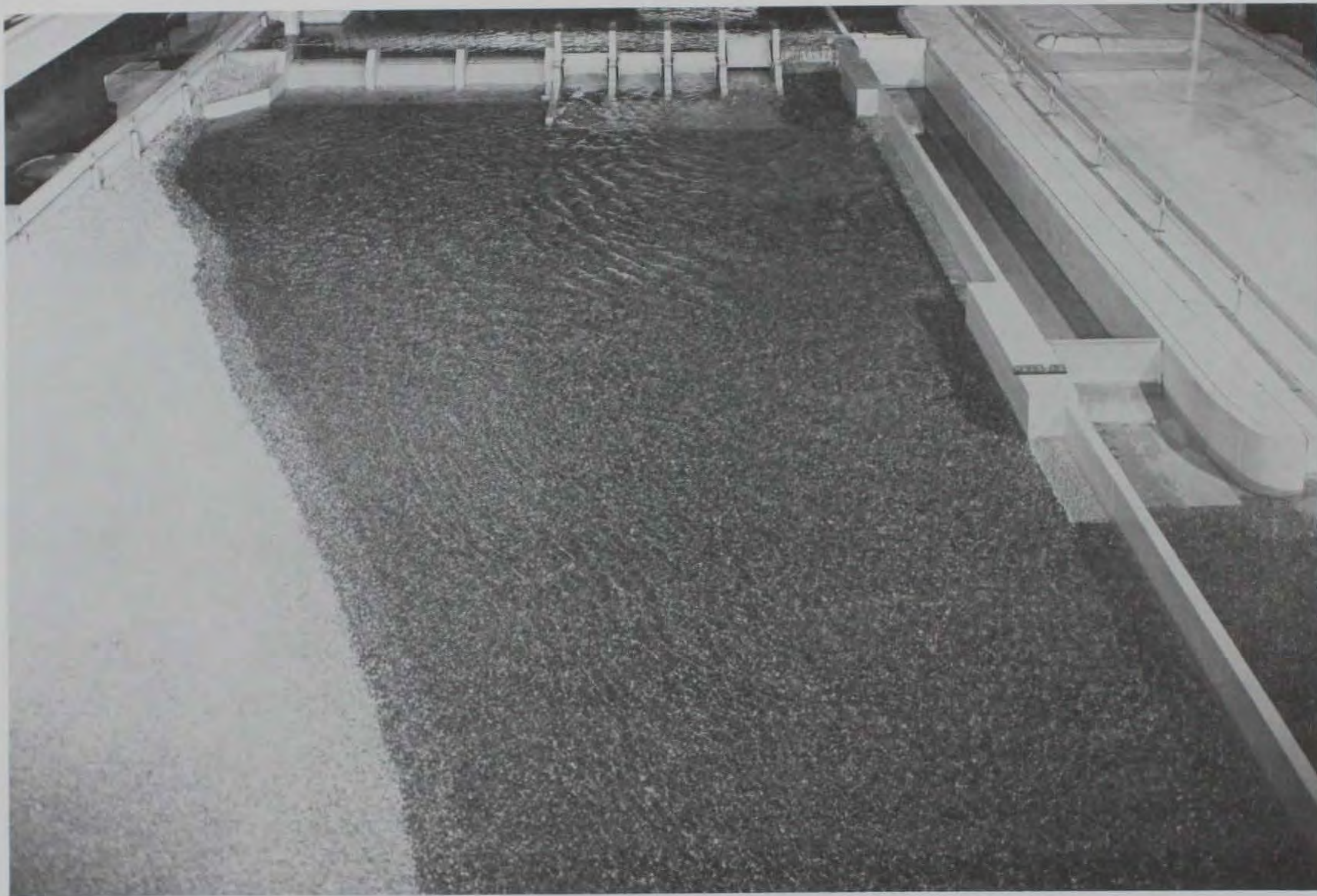
Photo 6. One tainter gate half open; pool el 122; tailwater el 95; looking upstream
