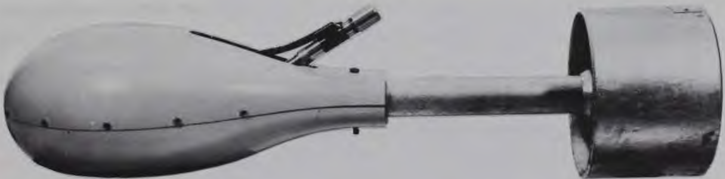
Fig. 14. Towed fish containing the four transducers in the array shown in fig. 13. The fish permits the transducers to be towed at greater depths, thus eliminating certain background noises and enabling the vessel to move at greater speeds
