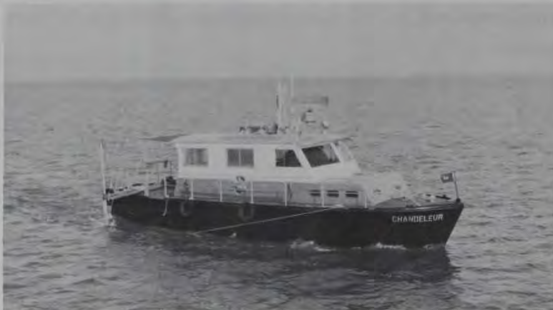
Fig. 30. Diesel-powered survey boat operated by the New Orleans District, Corps of Engineers. The vessel is approximately 50 ft long and has ample cabin space for the accommodation of all required surveying equipment
