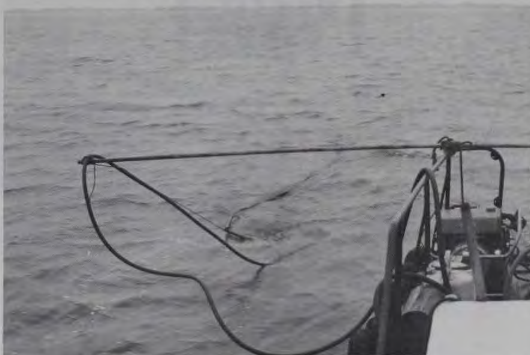
Fig. 17. Hydrophone array trailing survey boat on side opposite catamaran to avoid interference
