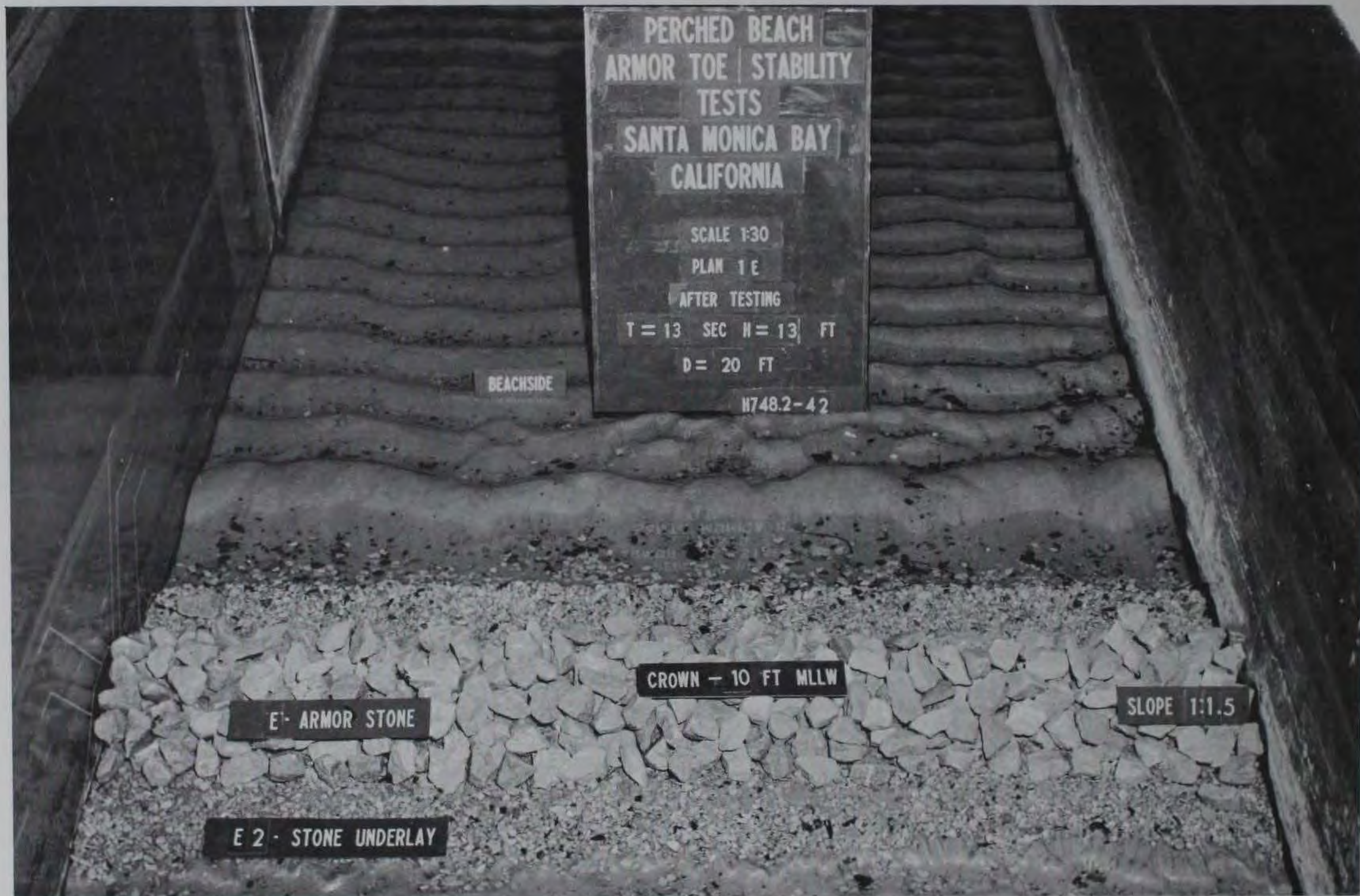
Photo 13. Plan T1E after attack by 11-sec, 11-ft; 17-sec, 8-ft; and 13-sec, 13-ft waves at 20-ft depth
