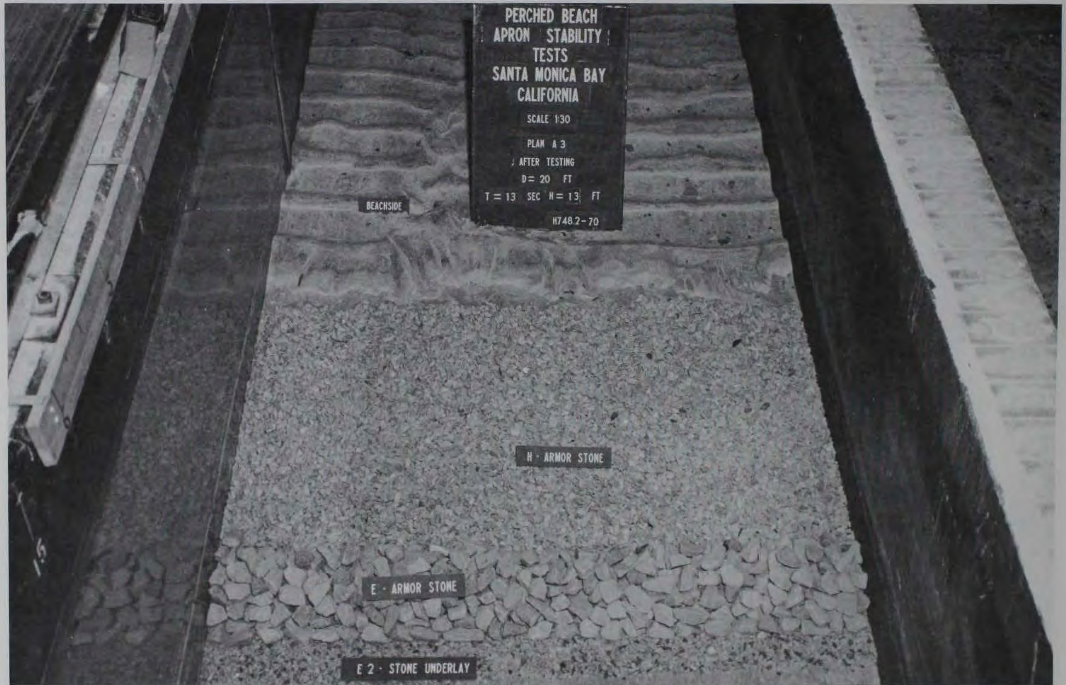
Photo 19. Plan A3 after attack of 11-sec, 11-ft; 17-sec, 8-ft; and 13-sec, 13-ft waves at 20-ft depth
