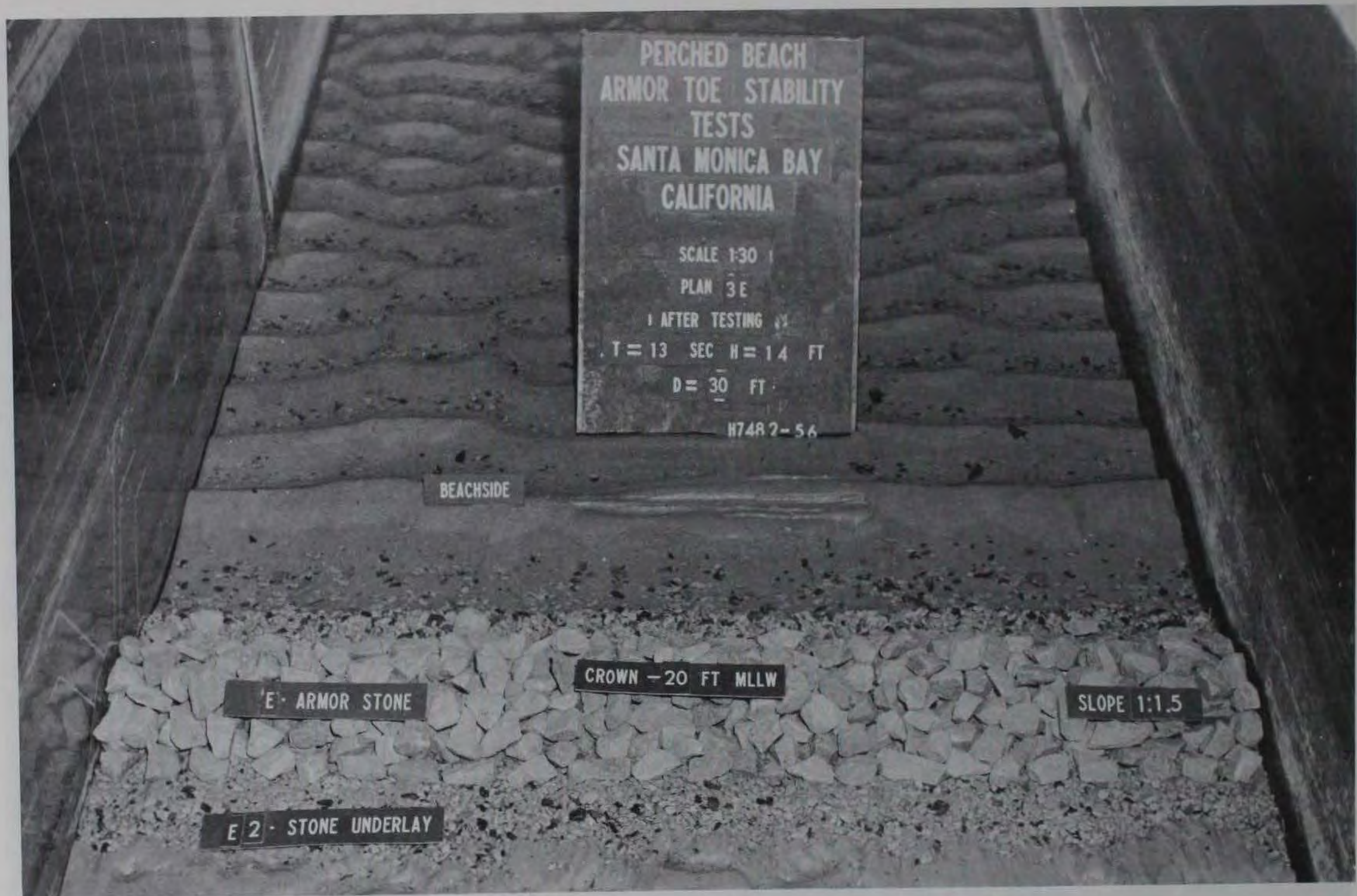
Photo 17. Plan T3E after attack by 11-sec, 13.5-ft; 17-sec, 12-ft; and 13-sec, 14-ft waves at 30-ft depth
