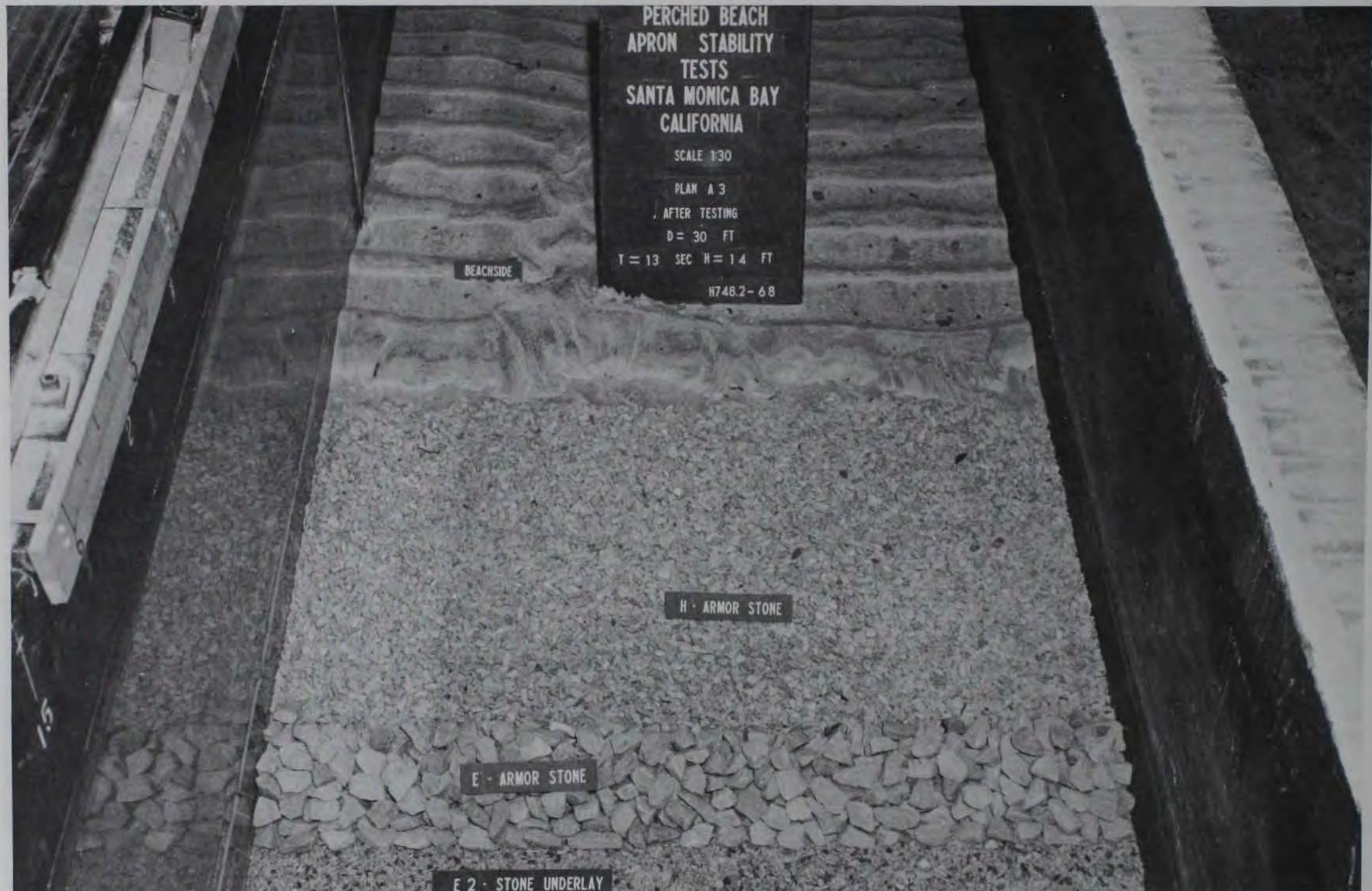
Photo 21. Plan A3 after attack of 11-sec, 13.5-ft; 17-sec, 12-ft; and 13-sec, 14-ft waves at 30-ft depth
