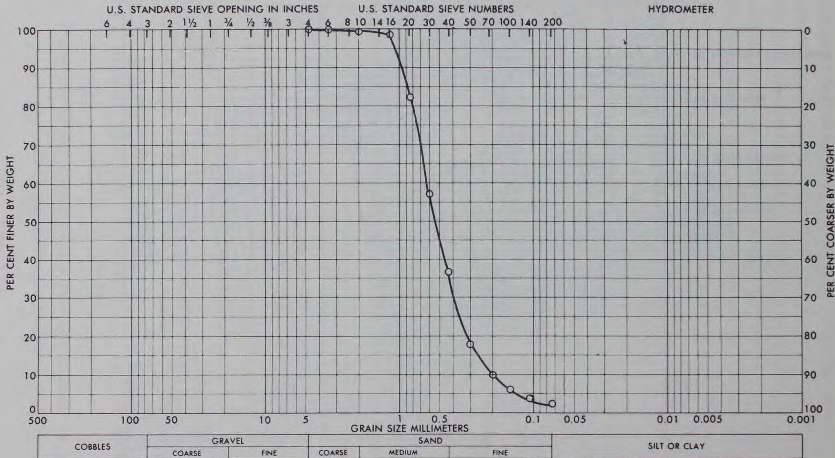
Fig. 8. Grain-size distribution for crushed coal used in movable-bed tests
