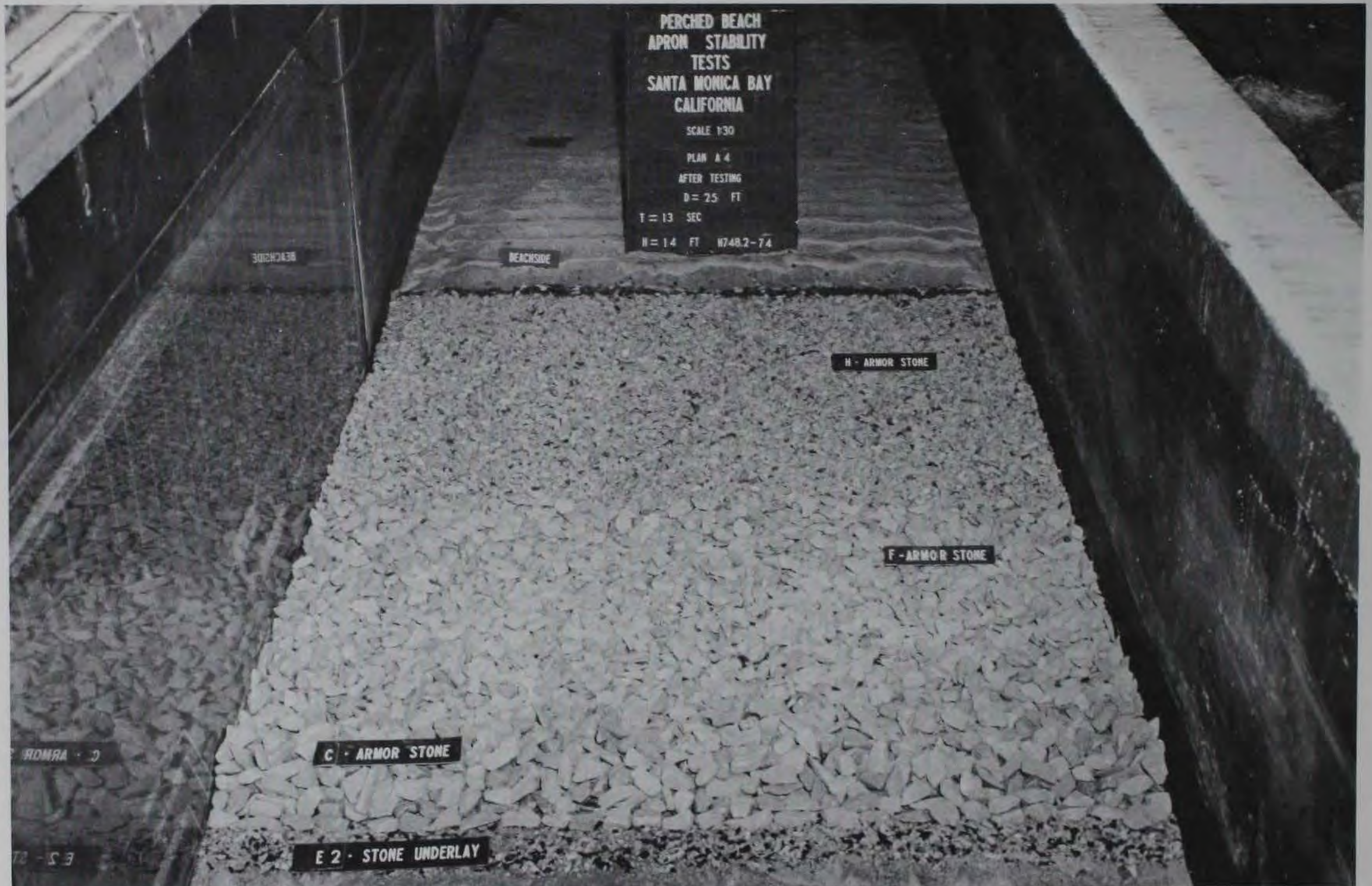
Photo 23. Plan A4 after attack of 11-sec, 13.5-ft; 17-sec, 12-ft; and 13-sec, 14-ft waves at 25-ft depth
