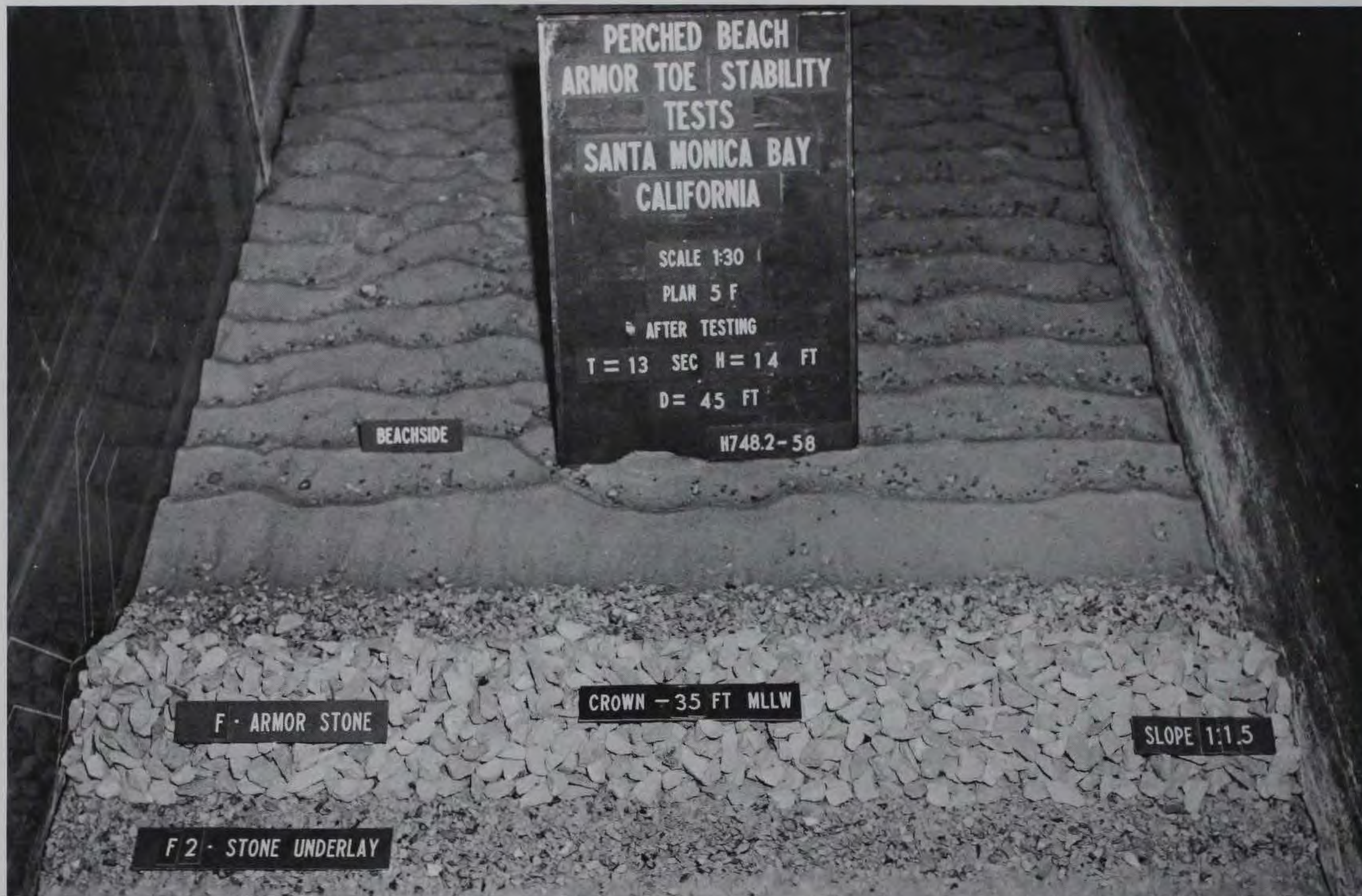
Photo 18. Plan T5F after attack by 11-sec, 13.5-ft; 17-sec, 12-ft; and 13-sec, 14-ft waves at 45-ft depth
