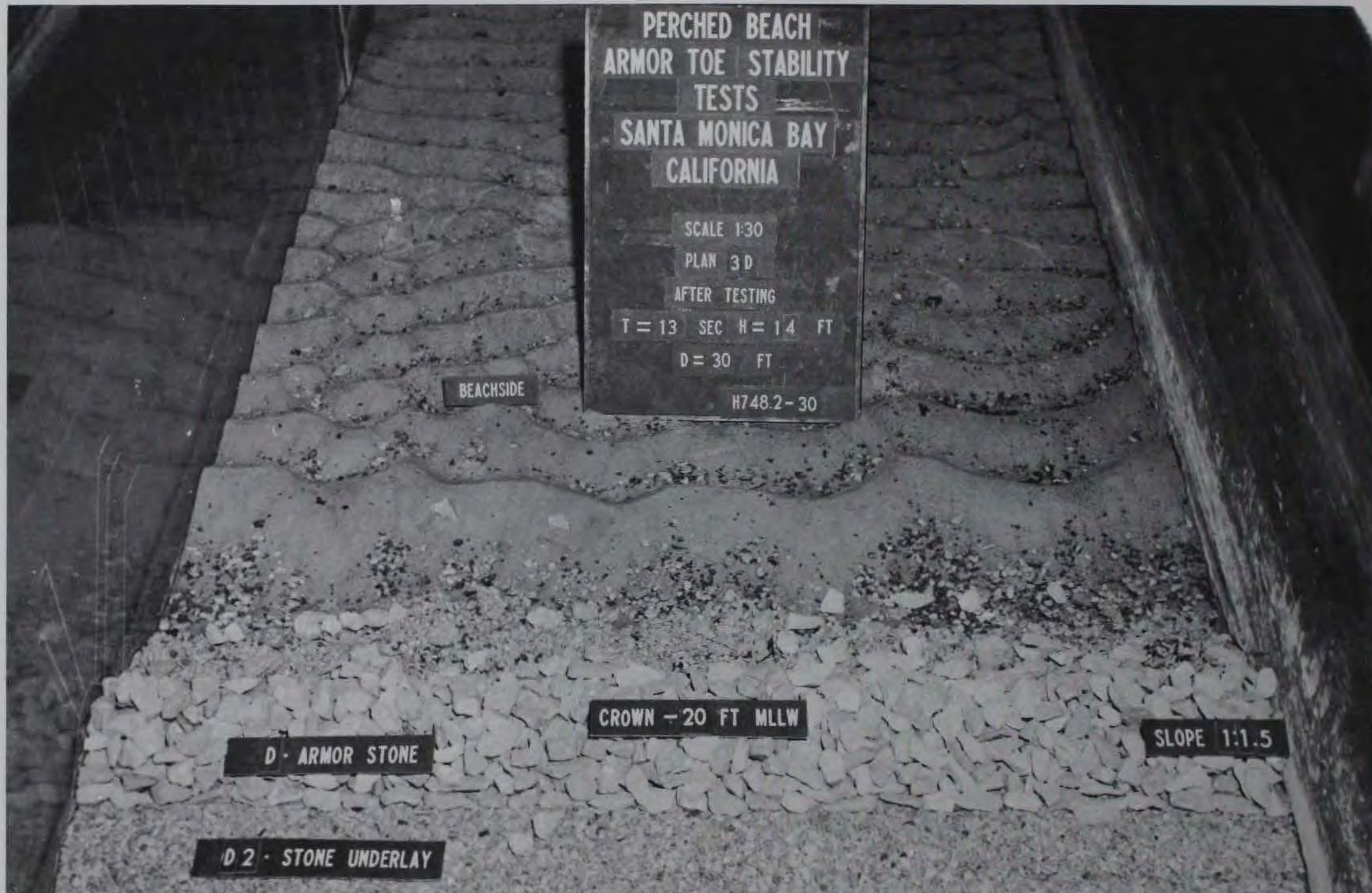
Photo 16. Plan T3D after attack by 11-sec, 13.5-ft; 17-sec, 12-ft; and 13-sec, 14-ft waves at 30-ft depth
