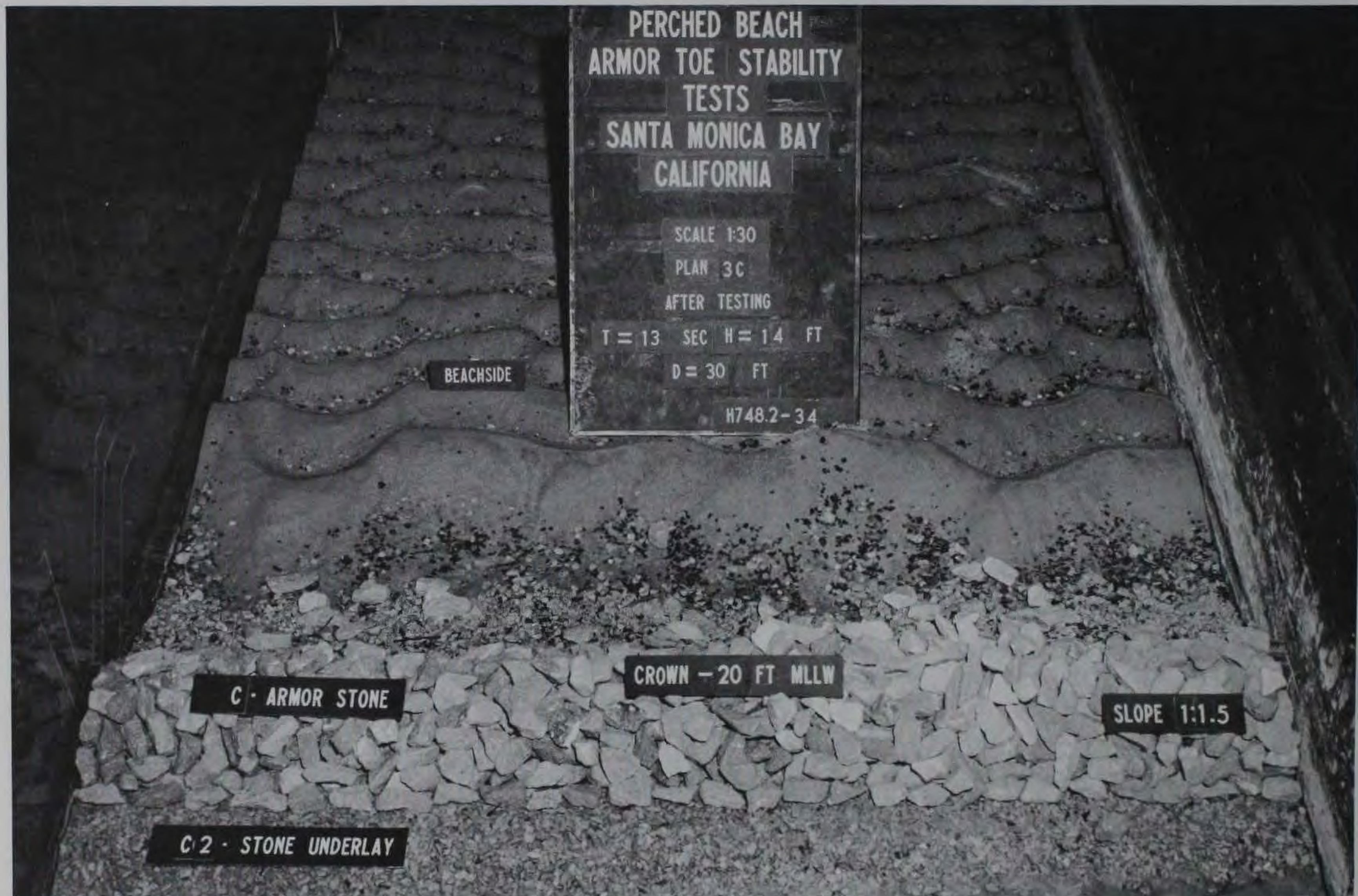
Photo 15. Plan T3C after attack by 11-sec, 13.5-ft; 17-sec, 12-ft; and 13-sec, 14-ft waves at 30-ft depth
