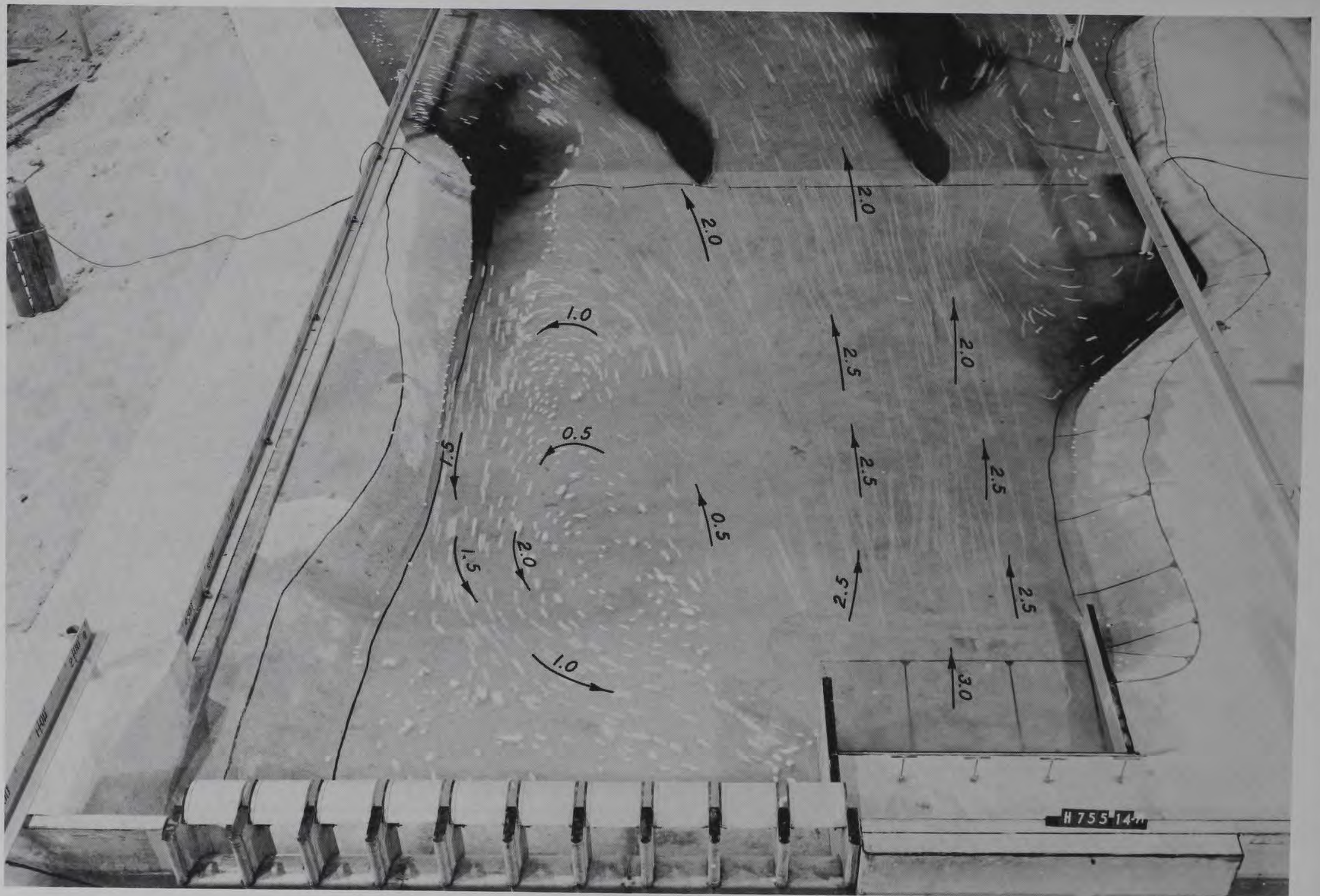
Photo 12. Flow conditions resulting from powerhouse release; discharge 28,000 cfs, tailwater el 345.0. Numbers denote bottom velocities in prototype feet per second
