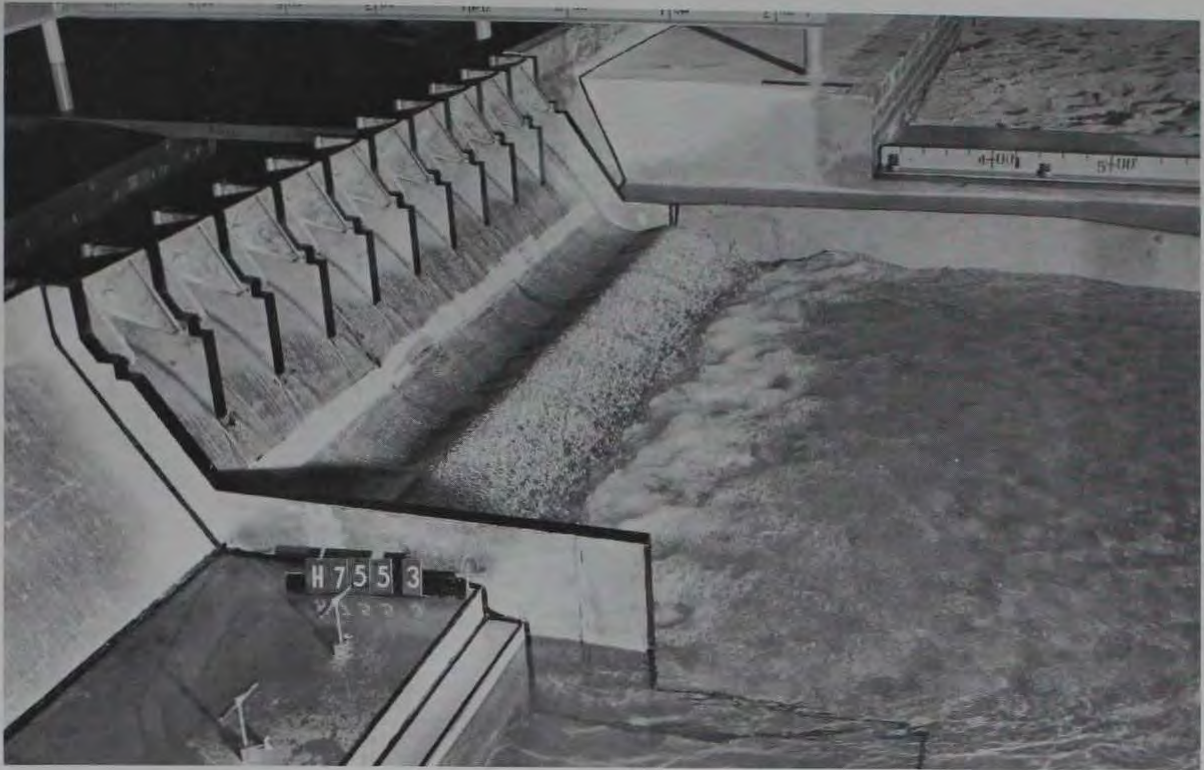
a. Nappe clinging to lip of flip bucket
