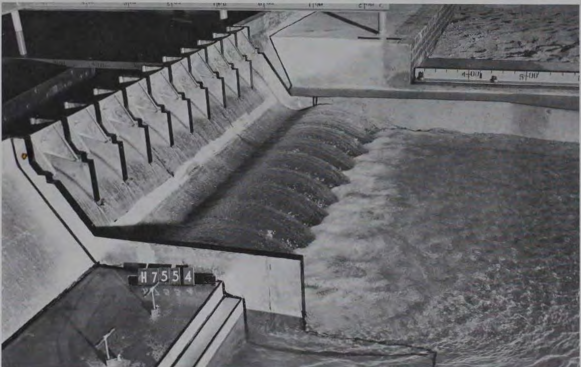
b. Nappe springing free from lip of flip bucket due to artificial venting
