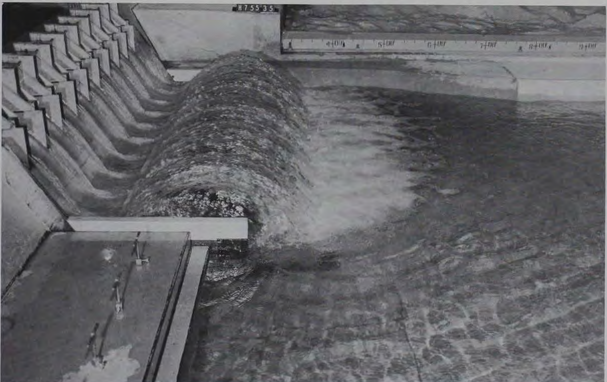
b. Discharge 100,000 cfs, pool el 482.0, tailwater el 335.0
