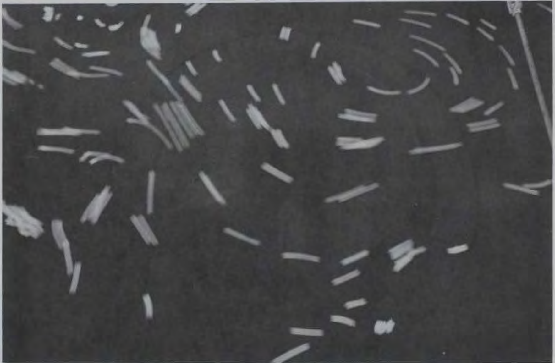
Photo 7. Flow conditions; conduit control; with cover plate; discharge 2,000 cfs, pool el -190.0
