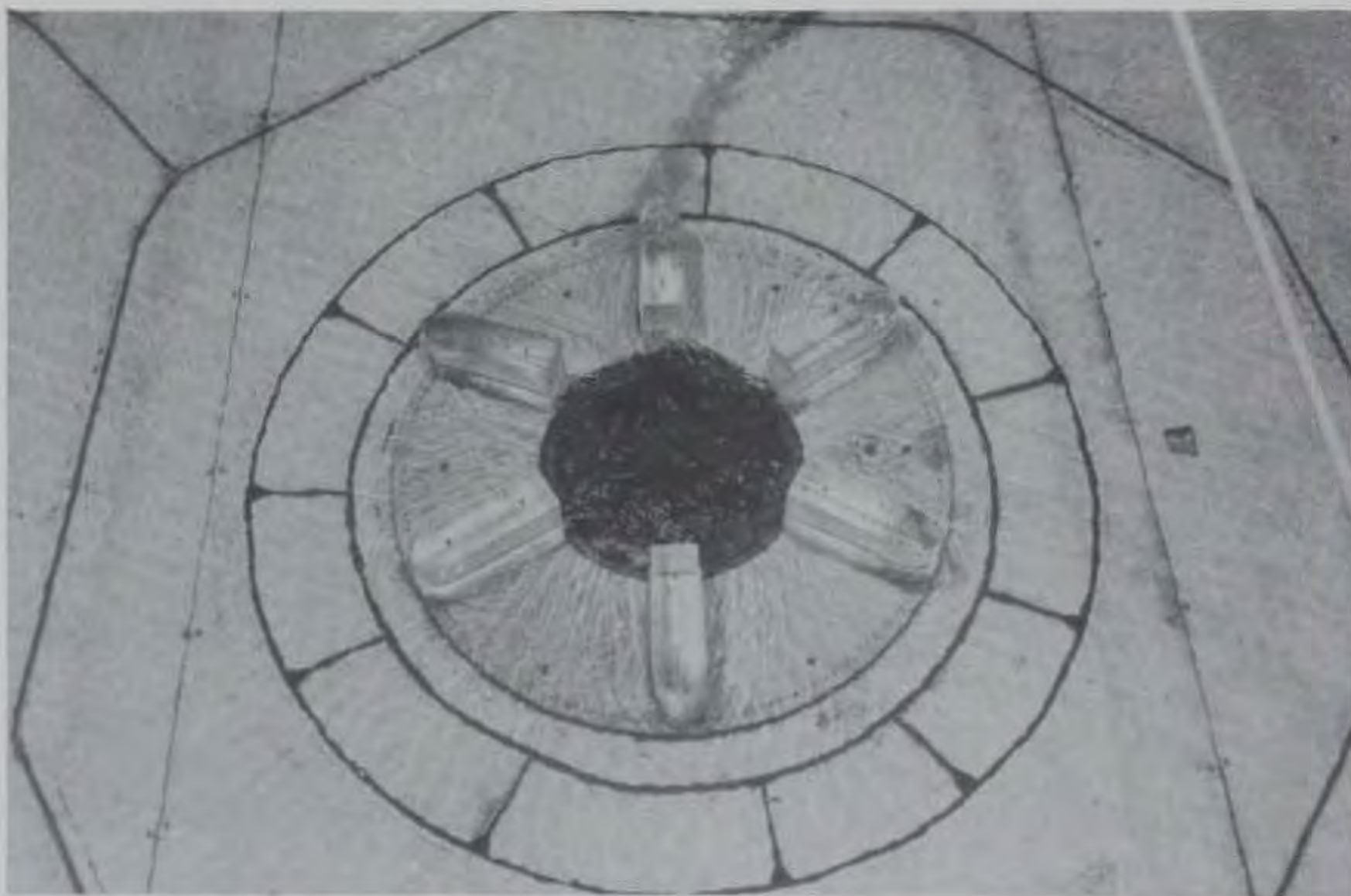
Photo 4. Flow conditions; transition from weir to conduit control; no cover plate; discharge 2,000 cfs, pool el -214.0
