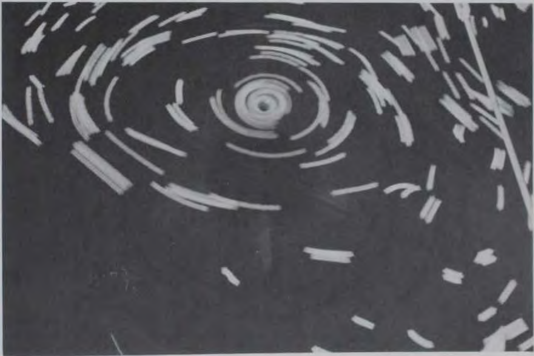
Photo 6. Flow conditions; conduit control; no cover plate; discharge 2,000 cfs, pool el -160.0
