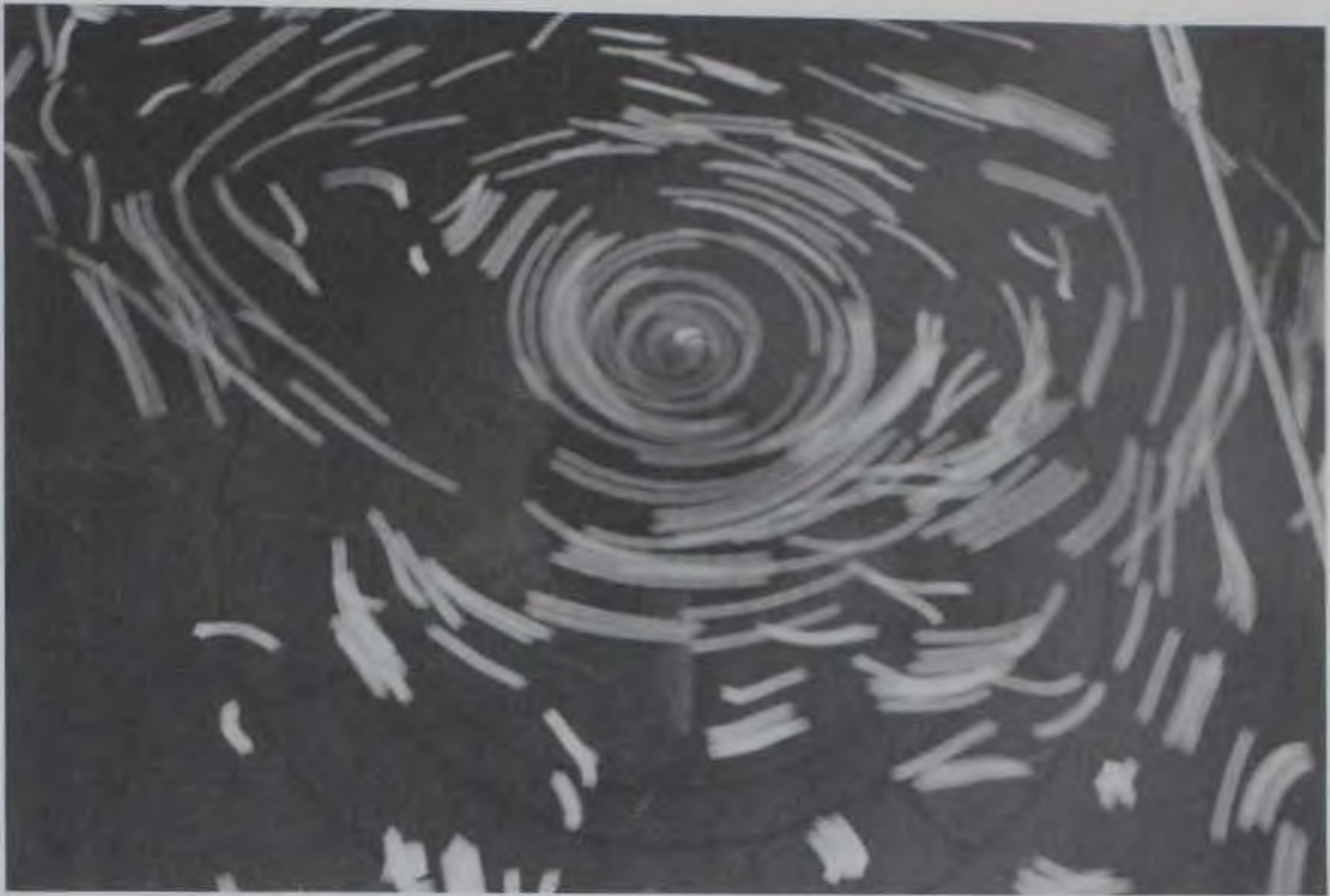
Photo 5. Flow conditions; conduit control; no cover plate; discharge 2,000 cfs, pool el -190.0
