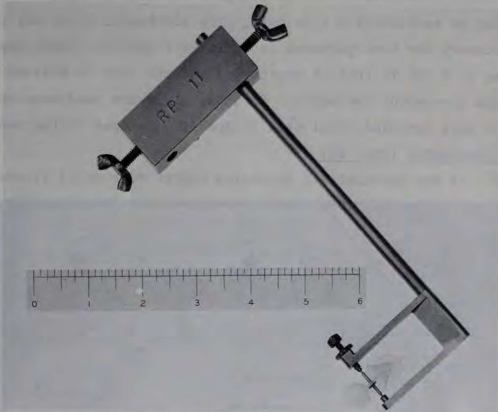
Fig. 10. Miniature Price-type current meter
