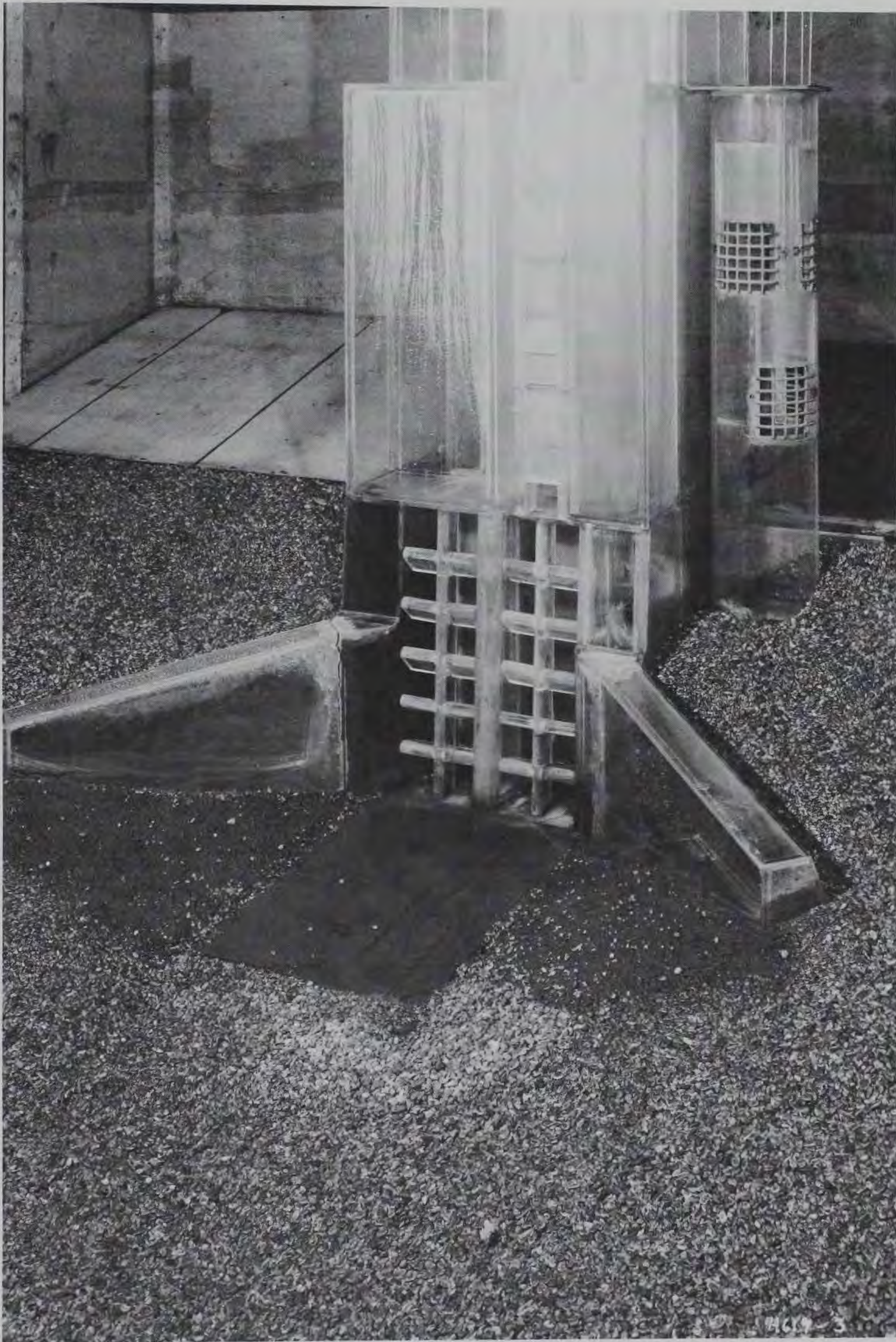
Figure 2. Intake structure with proposed selective withdrawal riser, 1:18-scale hydraulic model
