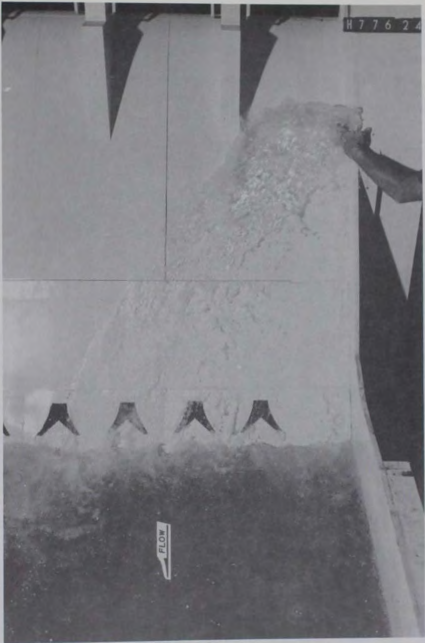
Photo 13. Sluice gate in modification 1 at 130-deg angle from downstream wall
