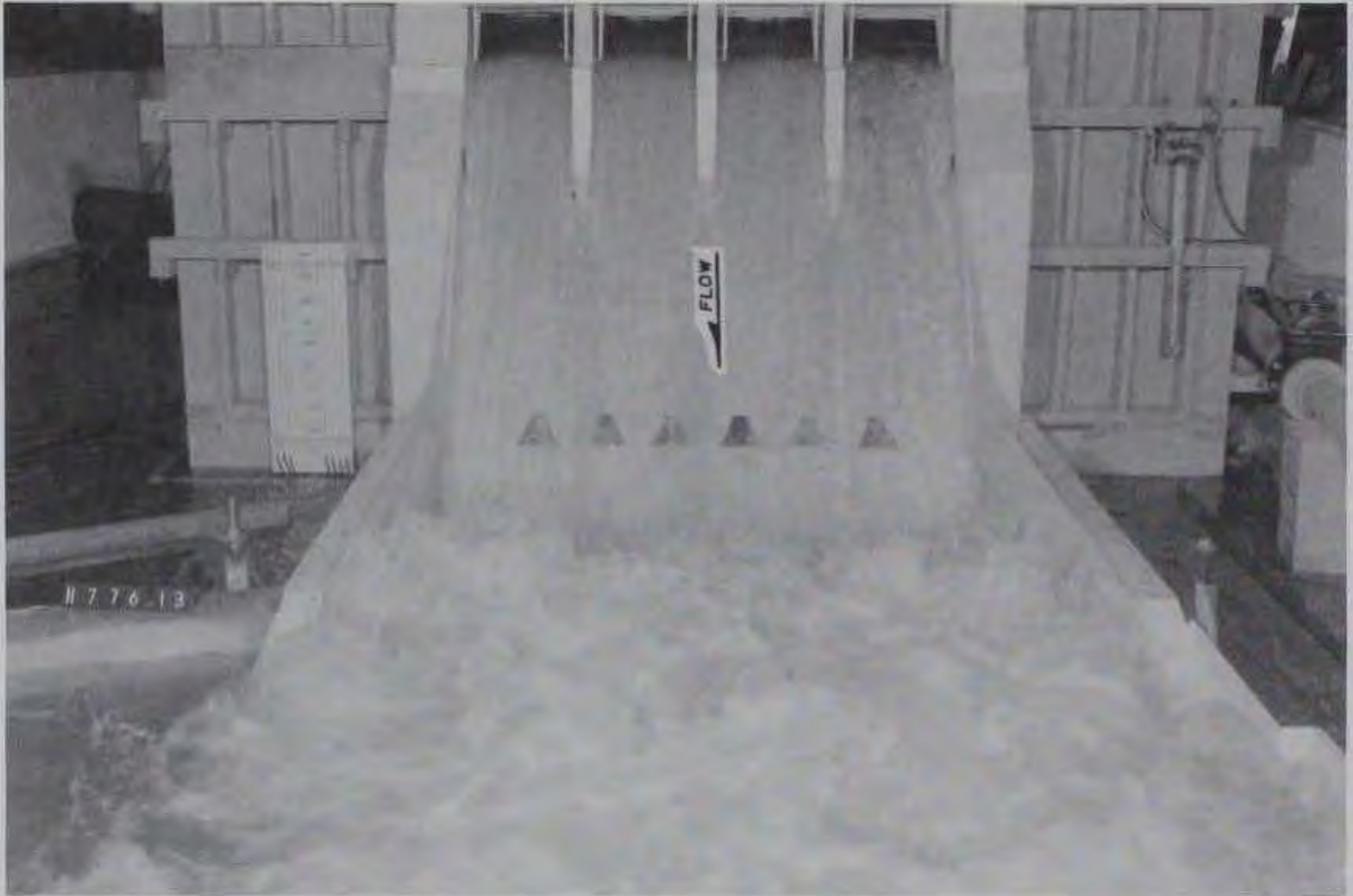
a. Discharge 114,000 cfs, tailwater el 1,266
