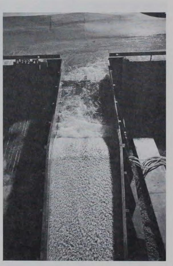
d. Discharge: North Gully 600 cfs Sandburg Creek 0 cfs
