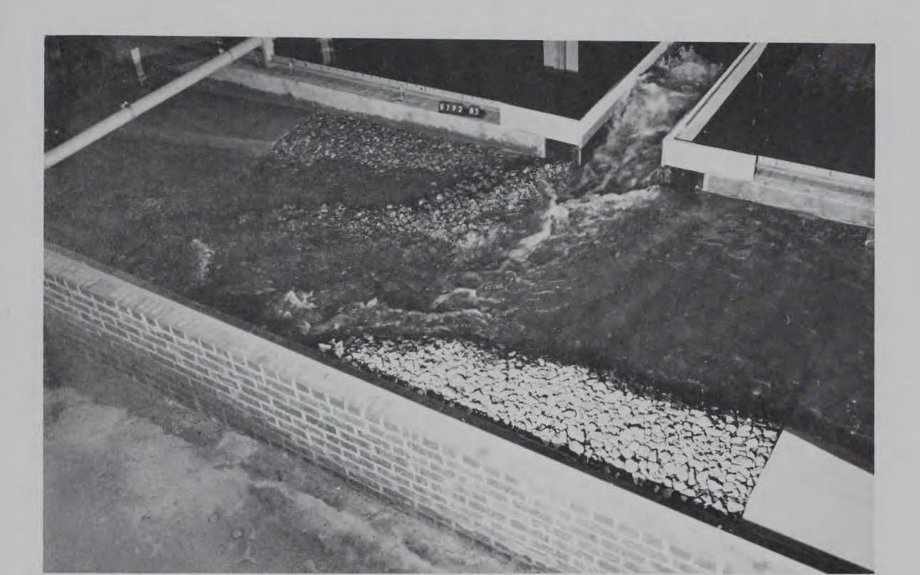
Photo 23. Flow conditions in and below the North Gully stilling basin (type 2 design) with 3900 cu yd of debris in and downstream of the basin. Discharge 3750 cfs North Gully and 0 cfs Sandburg Creek; tailwater el 314.0
