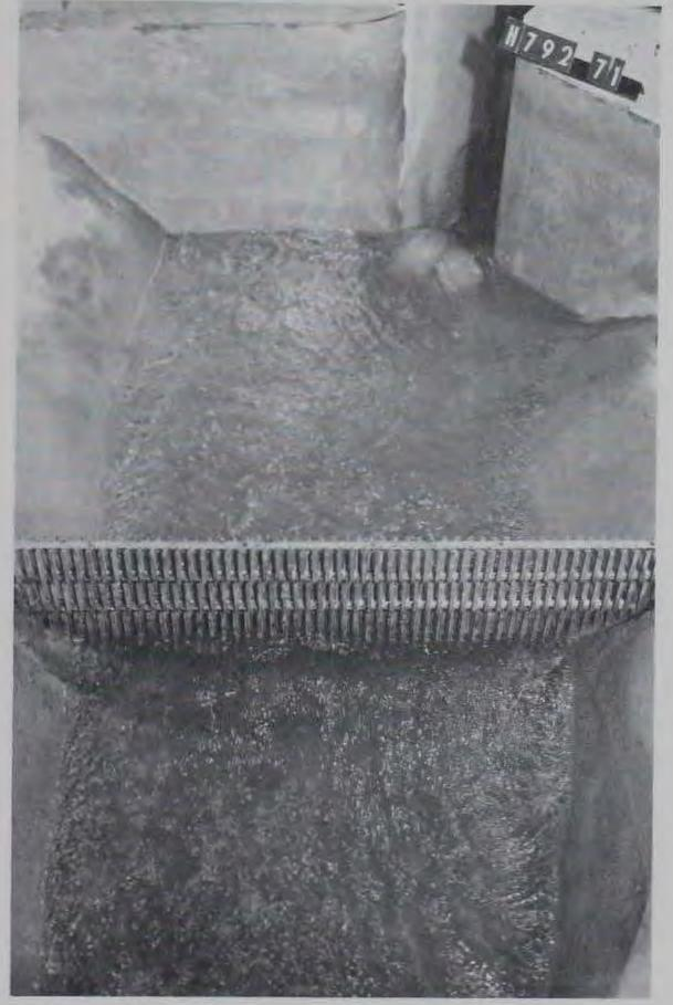
d. Discharge 1500 cfs; majority of flow along left bank of approach channel
