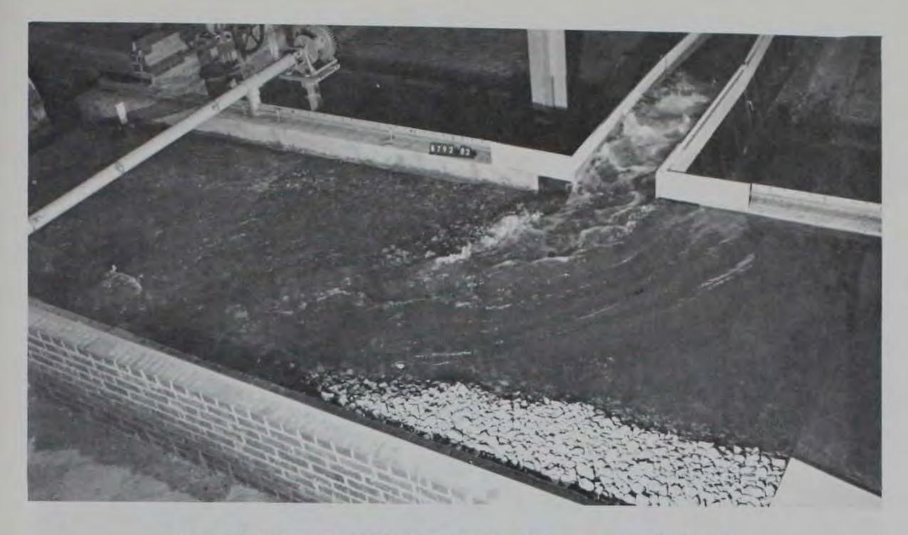
a. Discharge 3750 cfs North Gully and 9750 cfs Sandburg Creek; tailwater el 320.2
