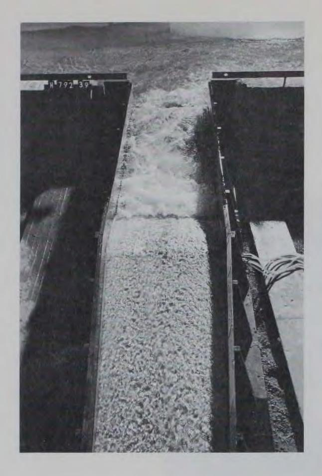
c. Discharge: North Gully 1500 cfs Sandburg Creek 0 cfs
