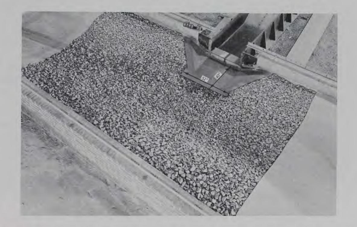
Photo 20. Results of scour test of 2-hr duration (model) with a paved section below the type 2 basin and riprap simulating prototype stone with an average weight of 360 lb (48-in.-thick layer). Discharge vared from 1500 to 3750 cfs in North Gully; no flow in Sandburg Creek. Also combined flows up to 15,000 cfs in North Gully and Sandburg Creek.
