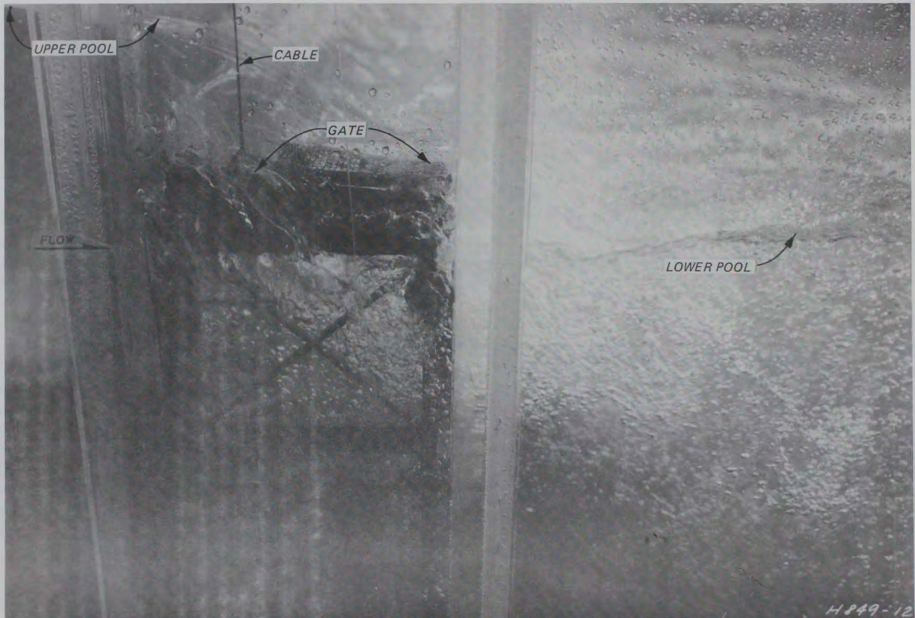
Photo 2. Unit discharge 64 cfs/ft, d_r = 9.0 ft, pool el 574 ft (NGVD), tailwater el 539 ft (NGVD)
