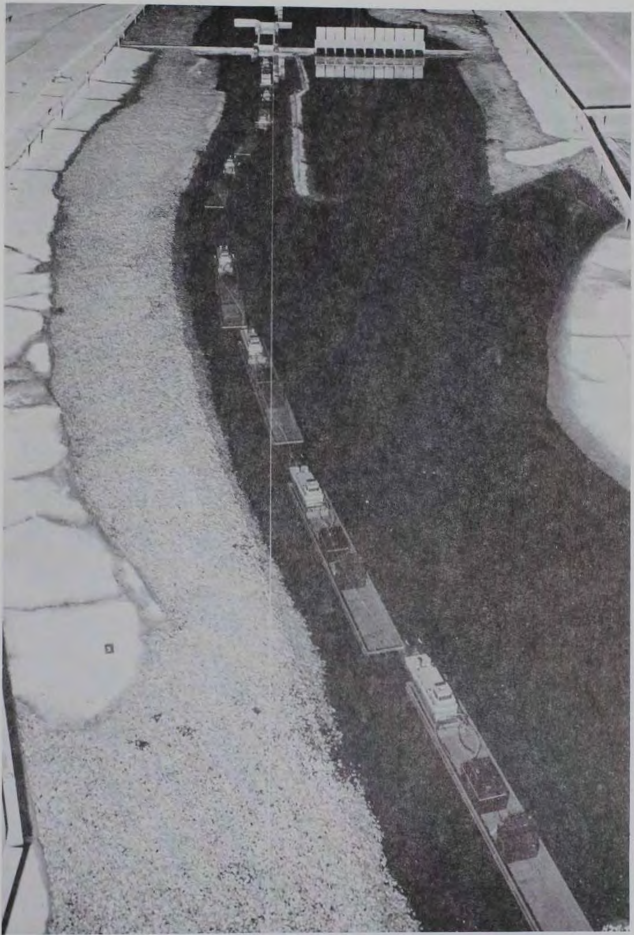
Photo 9. Plan B-34, upbound tow leaving the lock and canal; discharge 96,000 cfs, tailwater el 37.9 (normal)
