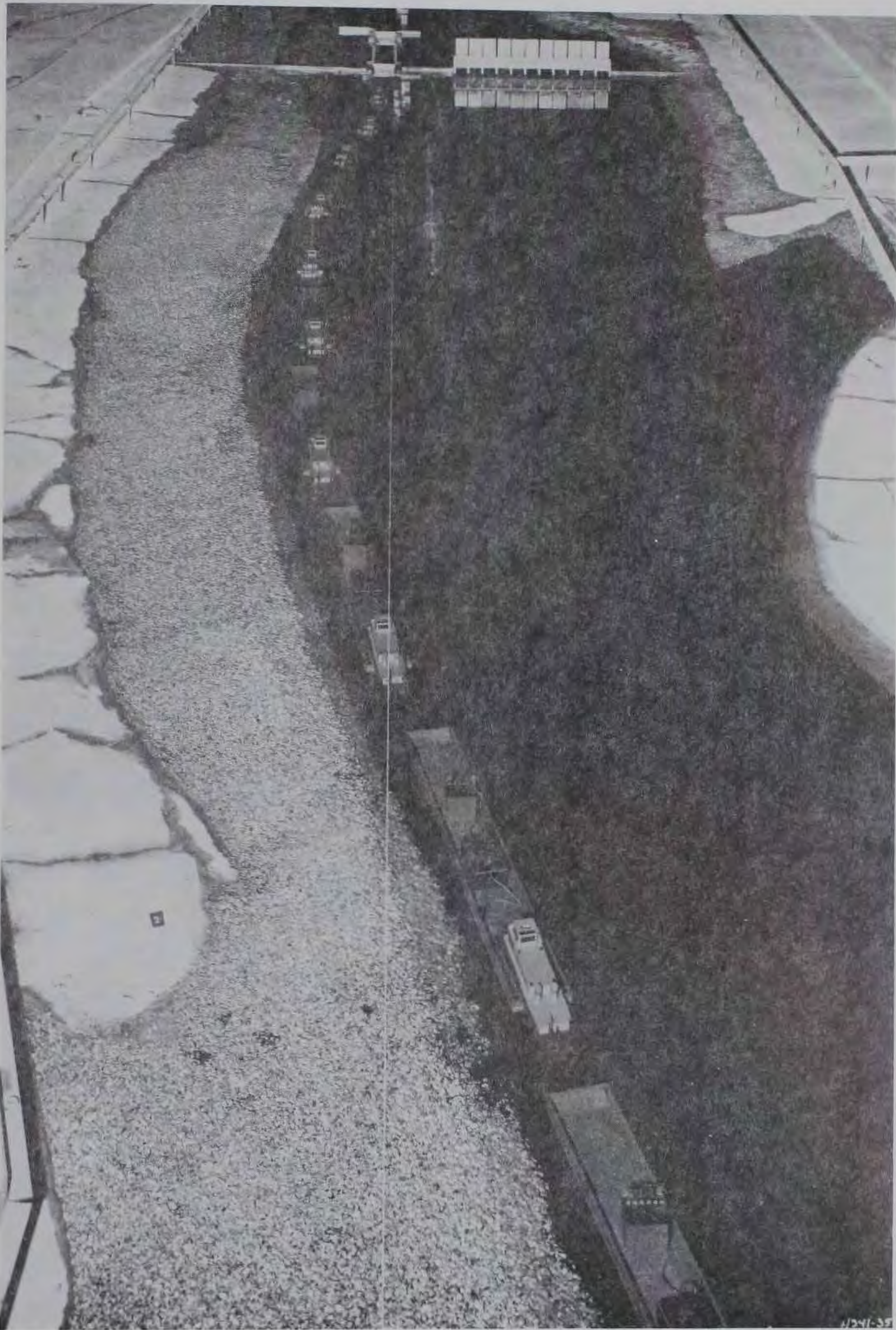
Photo 3. Plan B-34, downbound tow approaching the canal and lock from upstream; discharge 145,000 cfs, tailwater el 42.9 (minimum)
