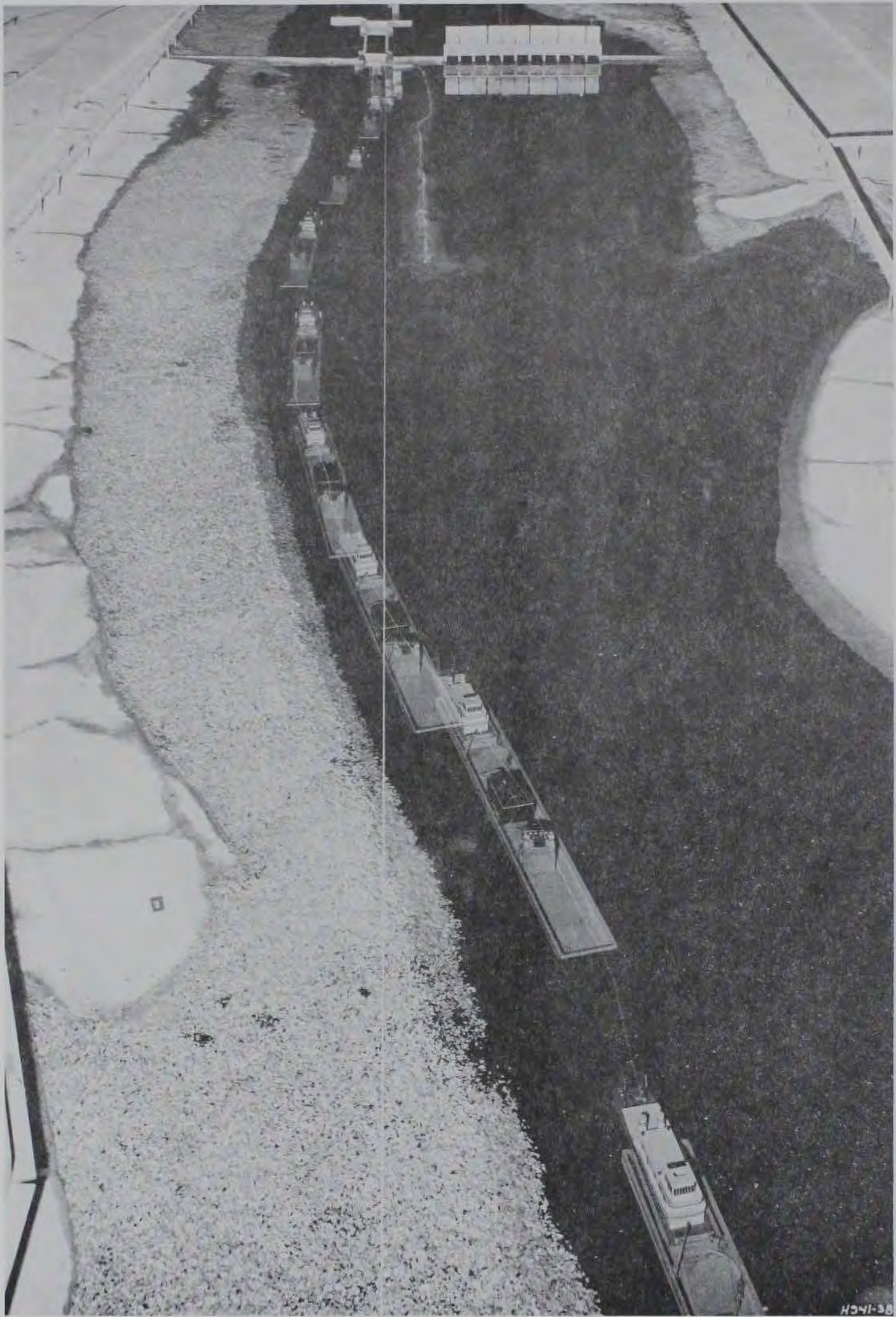
Photo 8. Plan B-34, upbound tow leaving the lock and canal; discharge 145,000 cfs, tailwater el 42.9 (minimum)
