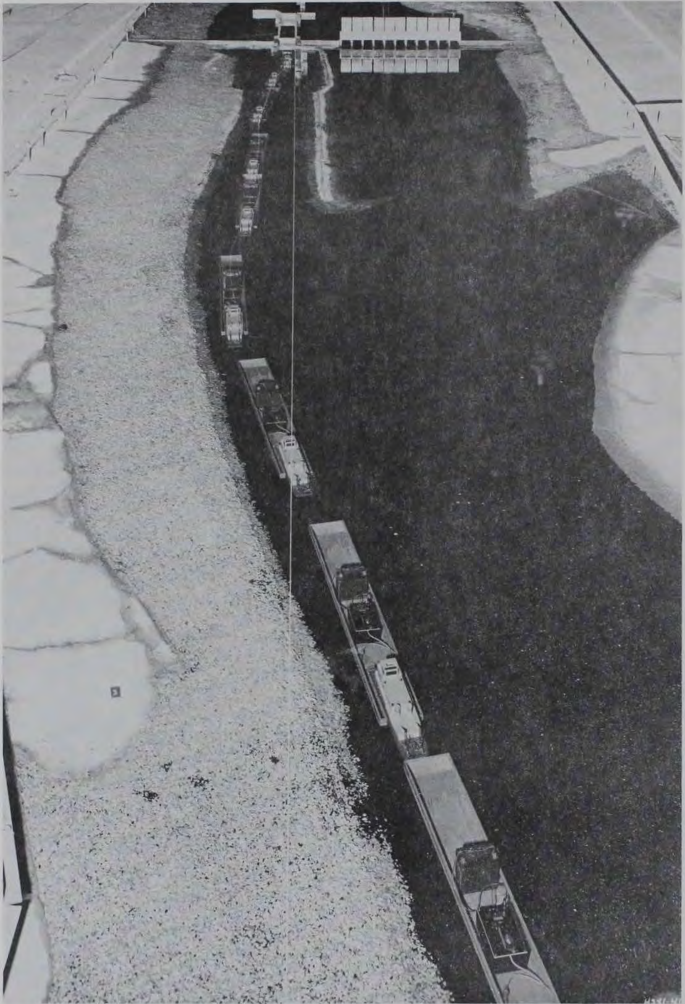
Photo 4. Plan B-34, downbound tow approaching the canal and lock from upstream; discharge 96,000 cfs, tailwater el 37.9 (normal)
