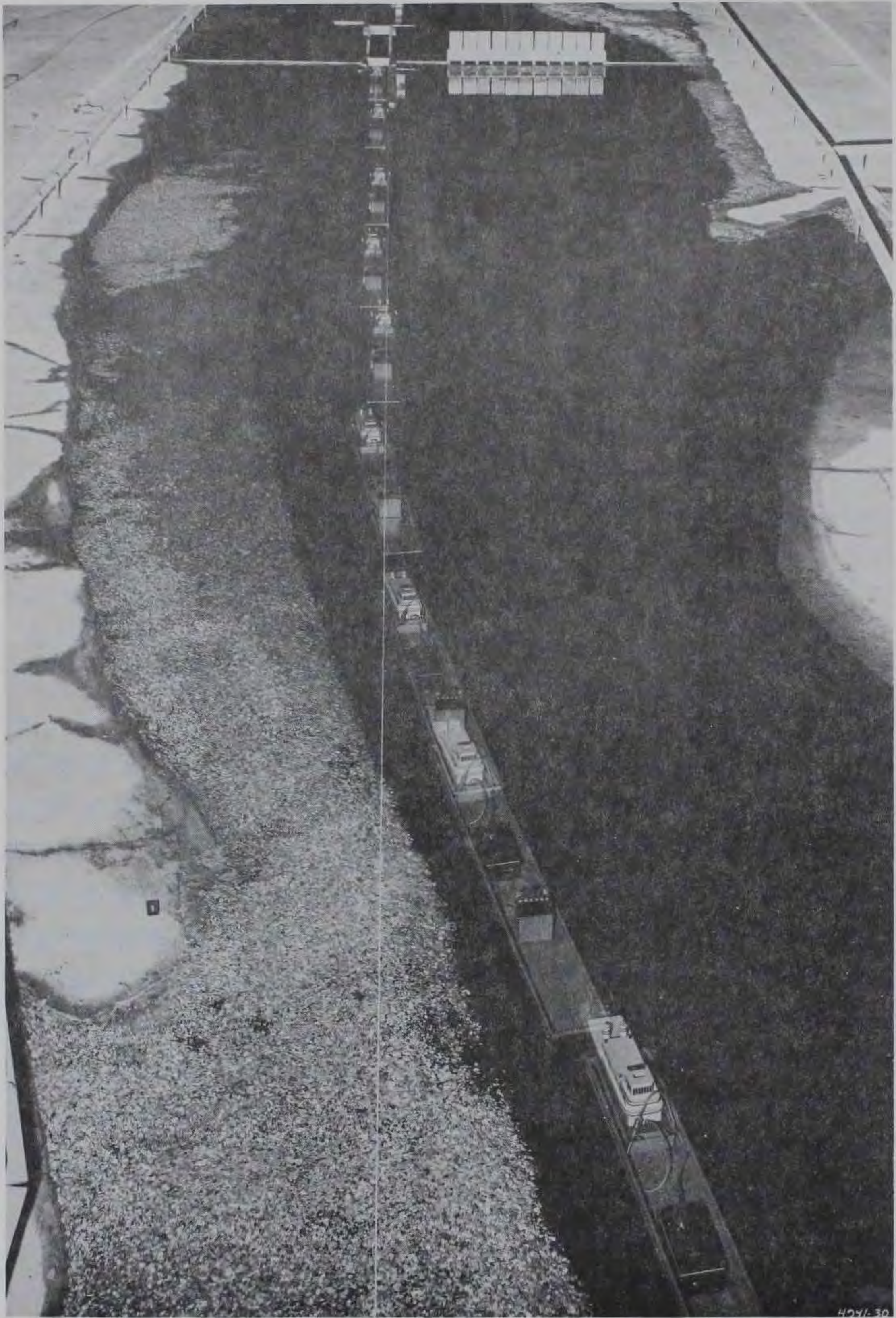
Photo 6. Plan B-34, upbound tow leaving the lock and canal; discharge 145,000 cfs, tailwater el 57.5 (normal)
