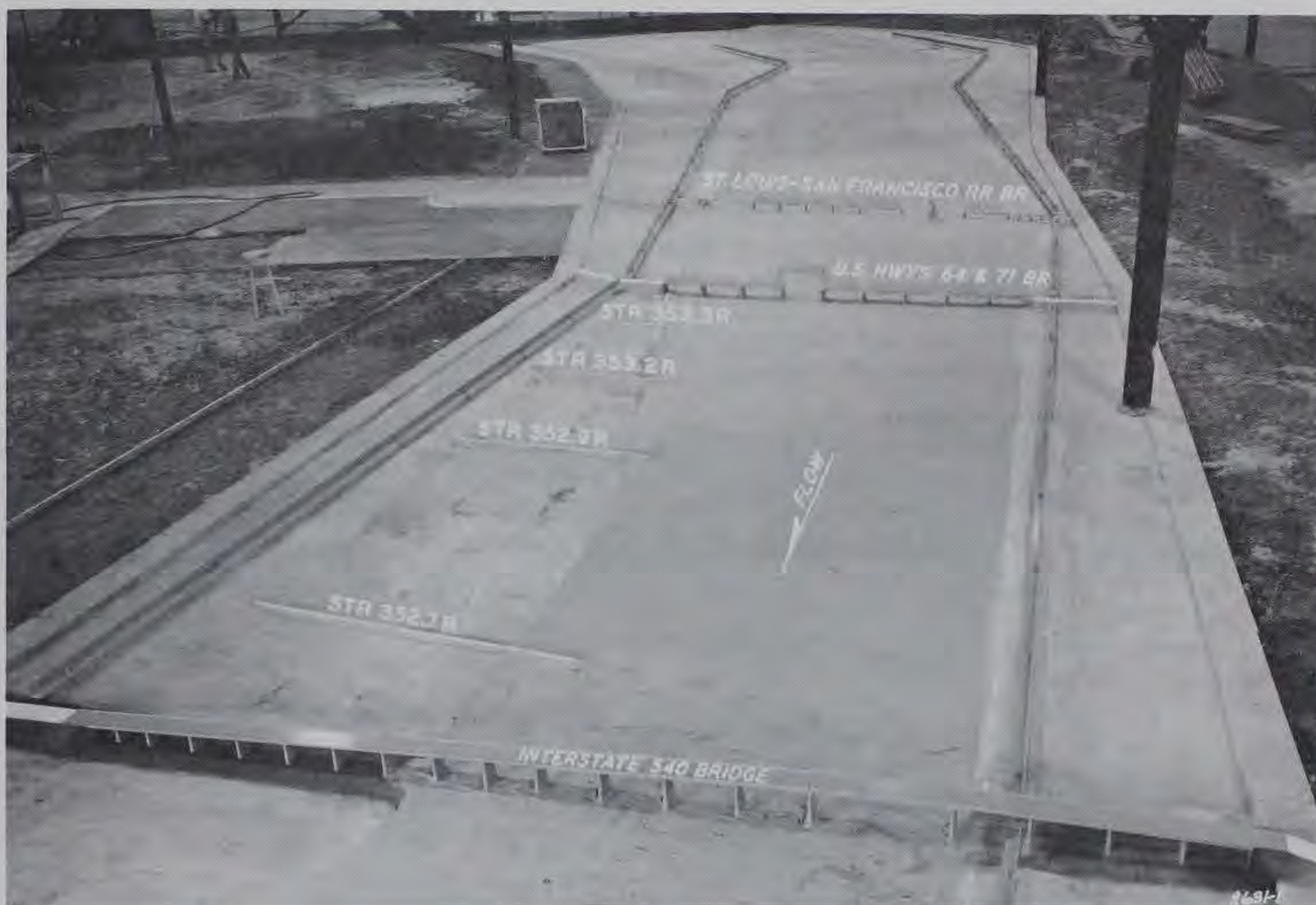
Fig. 2. General view of the model showing navigation spans of existing bridges and of the proposed I-540 bridge
