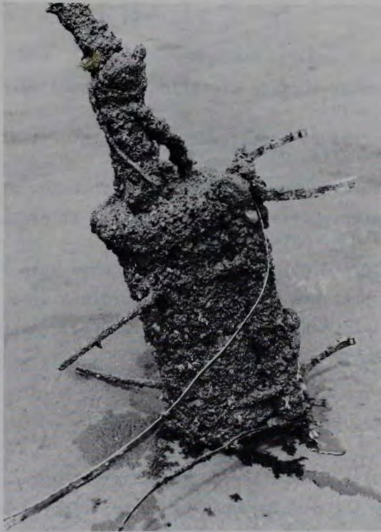
Figure 4. Typical marine growth on a transducer canister and cable after a few weeks submergence
