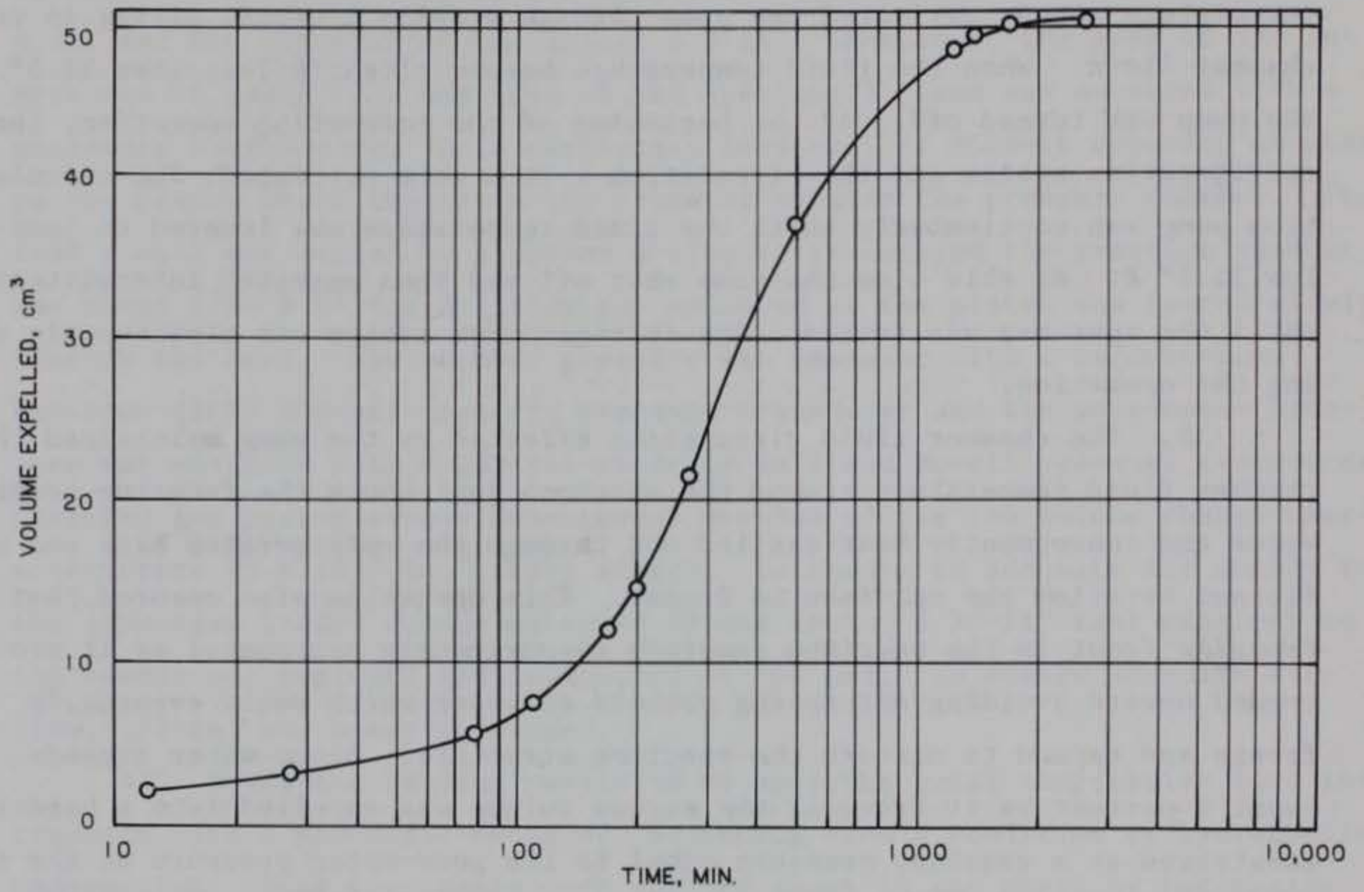
Figure 9. Water expelled versus time during specimen freezing
