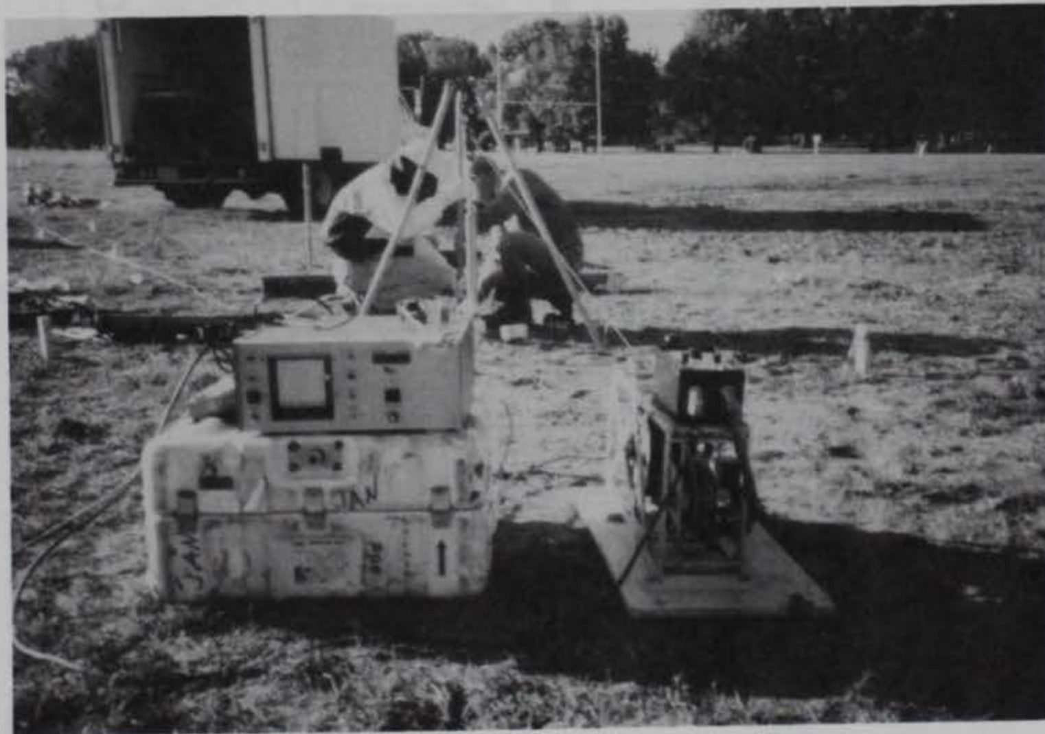
b. Surface control unit and winch
