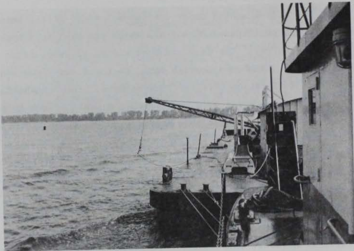
Figure 86. Towing configuration used for side-scanning sonar towfish during Middle Mississippi River acoustic survey, towfish approximately 5 ft below surface of water
