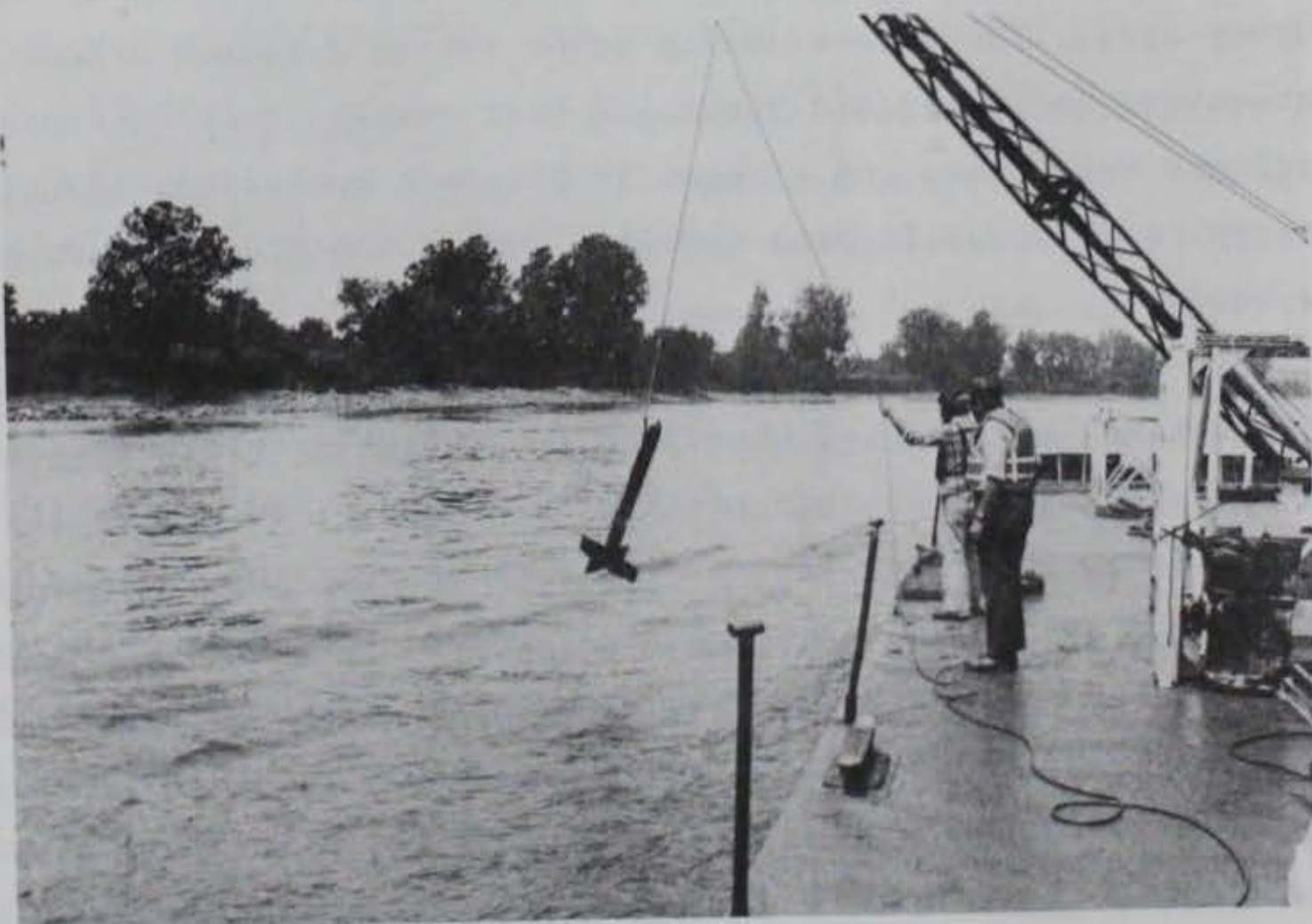
Figure 87. Retrieval of side-scanning sonar system towfish
