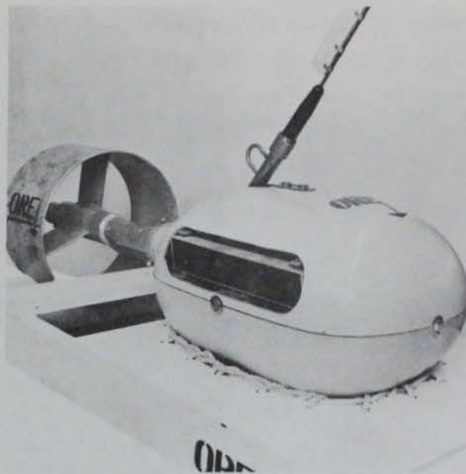
Figure 40. Towfish component of the ORE Model 1036 pinger subbottom profiling system (The source shown here has been modified to include side-scanning sonar transducers; courtesy of Ocean Research Equipment, Inc.)
