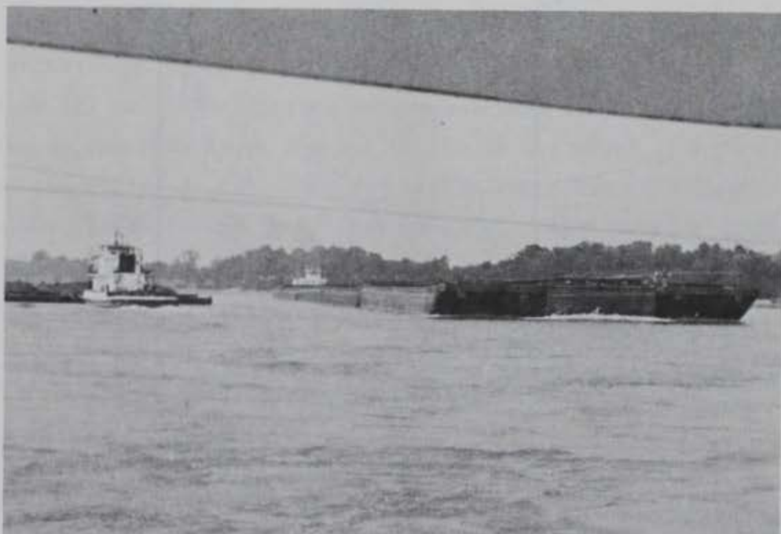
Figure 112. At some sites wave action generated by heavy commercial boat and barge traffic on the Ohio River has been identified as a mechanism for bank erosion
