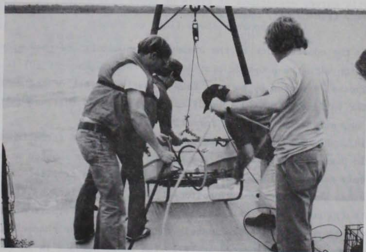
Figure 64. Survey personnel shown during deployment of the Uniboom profiling system's sound source from the stern of the survey boat; source weight, approximately 200 lb (from VED)
