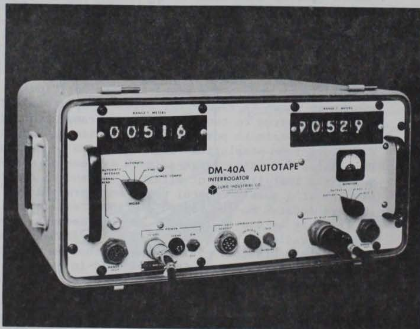
Figure 21. A two range configuration DMU (The unit provides visual readout of two ranges simultaneously one time per second; courtesy of Cubic Corporation.)
