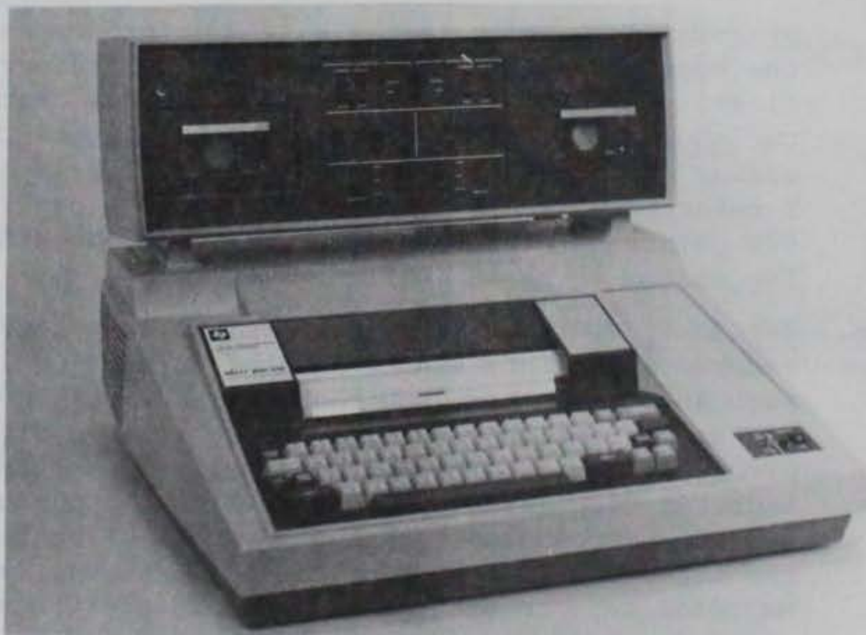
Figure 27. Texas Instruments Silent 700 data terminal and printer component of the WES Autocarta system
