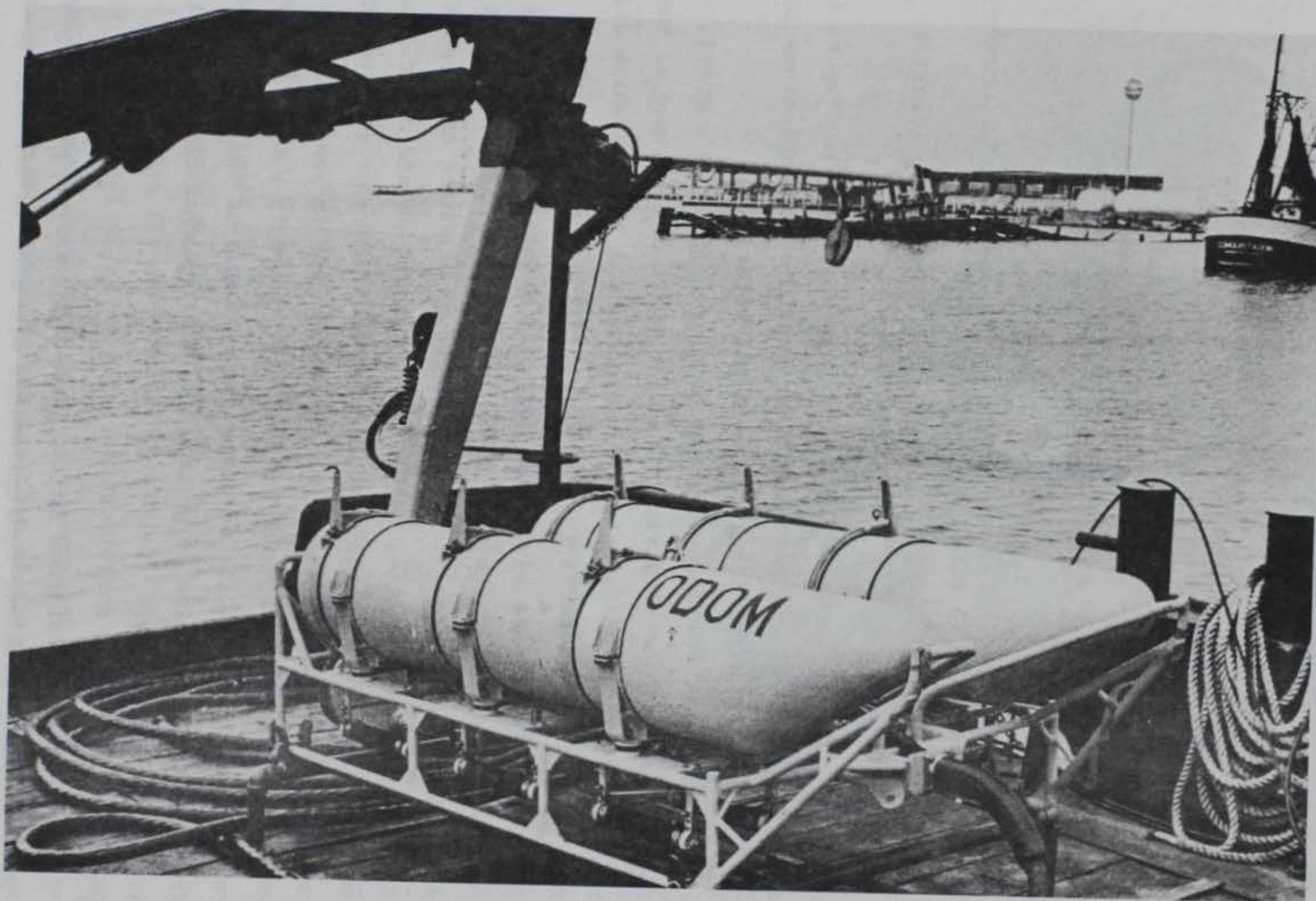
Figure 11. Thermodynamic source in a towing configuration utilizing multiple firing sleeves (courtesy of Odom Offshore Surveys, Inc.)
