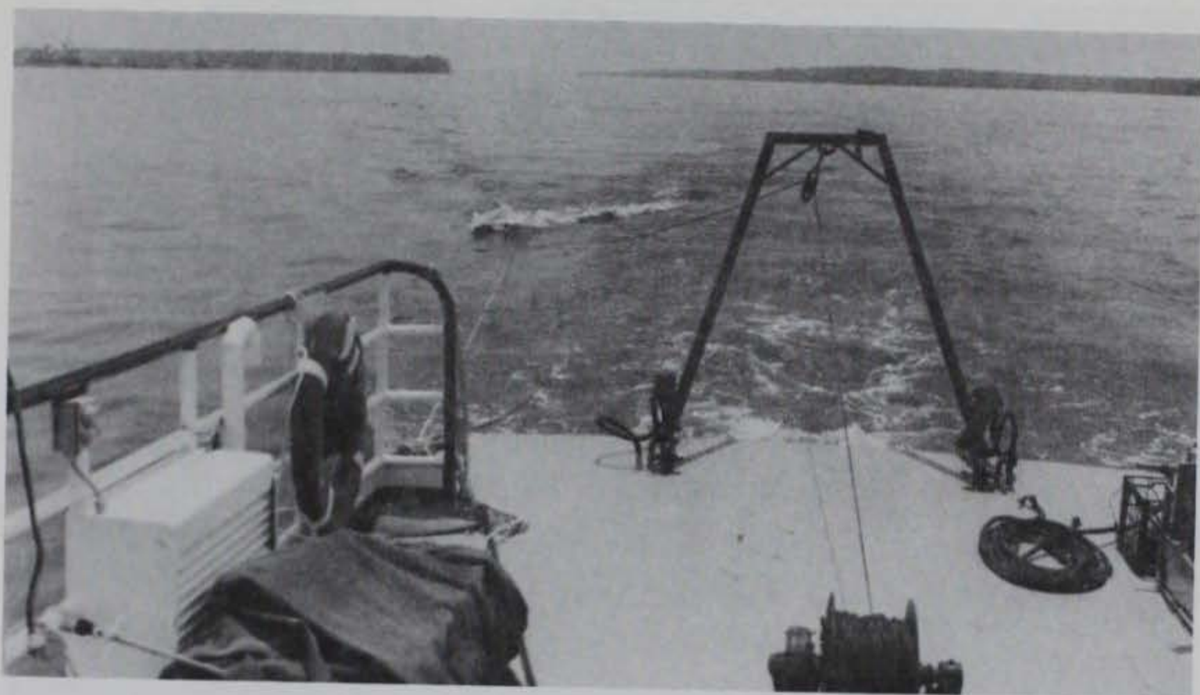
Figure 63. Towing arrangement used for Uniboom CSRP system at Diamond Point Cutoff and Arkansas City survey sites, Mississippi River (Sound source is visible at end of tow cable; steel cable and A-frame are used for deployment and retrieval; view is downstream at Diamond Point Cutoff survey area.)
