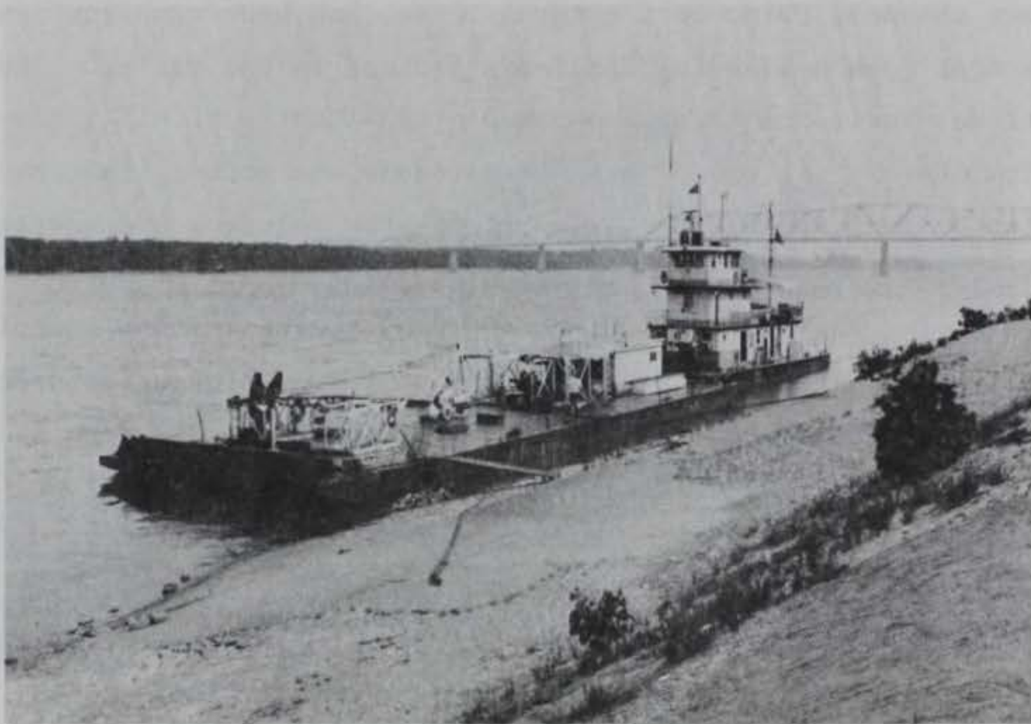
Figure 75. Barge and towboat configuration used as survey platform in support of Middle Mississippi River acoustic profiling survey, Cape Girardeau highway bridge in the background
