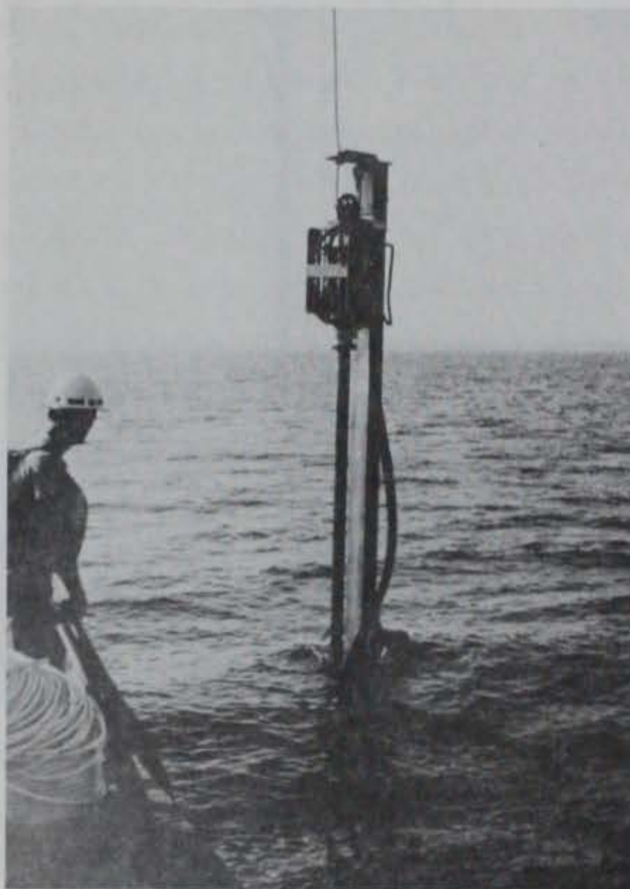
Figure 33. Vibratory sampler on the bottom and coring in Mississippi Sound (Water depth is approximately 10 ft)
