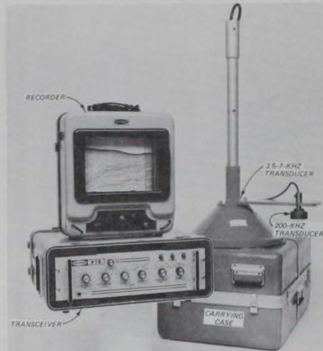
b. The Raytheon RTT-1000A-1 Portable Survey System, a small, compact pinger system designed for "over-the-side" towing configuration (The system operates at either 3.5 or 7 kHz for sub-bottom profiling. A small, 200-kHz transducer may be attached for acquisition of high resolution bathymetry. Courtesy of Raytheon Company.)
