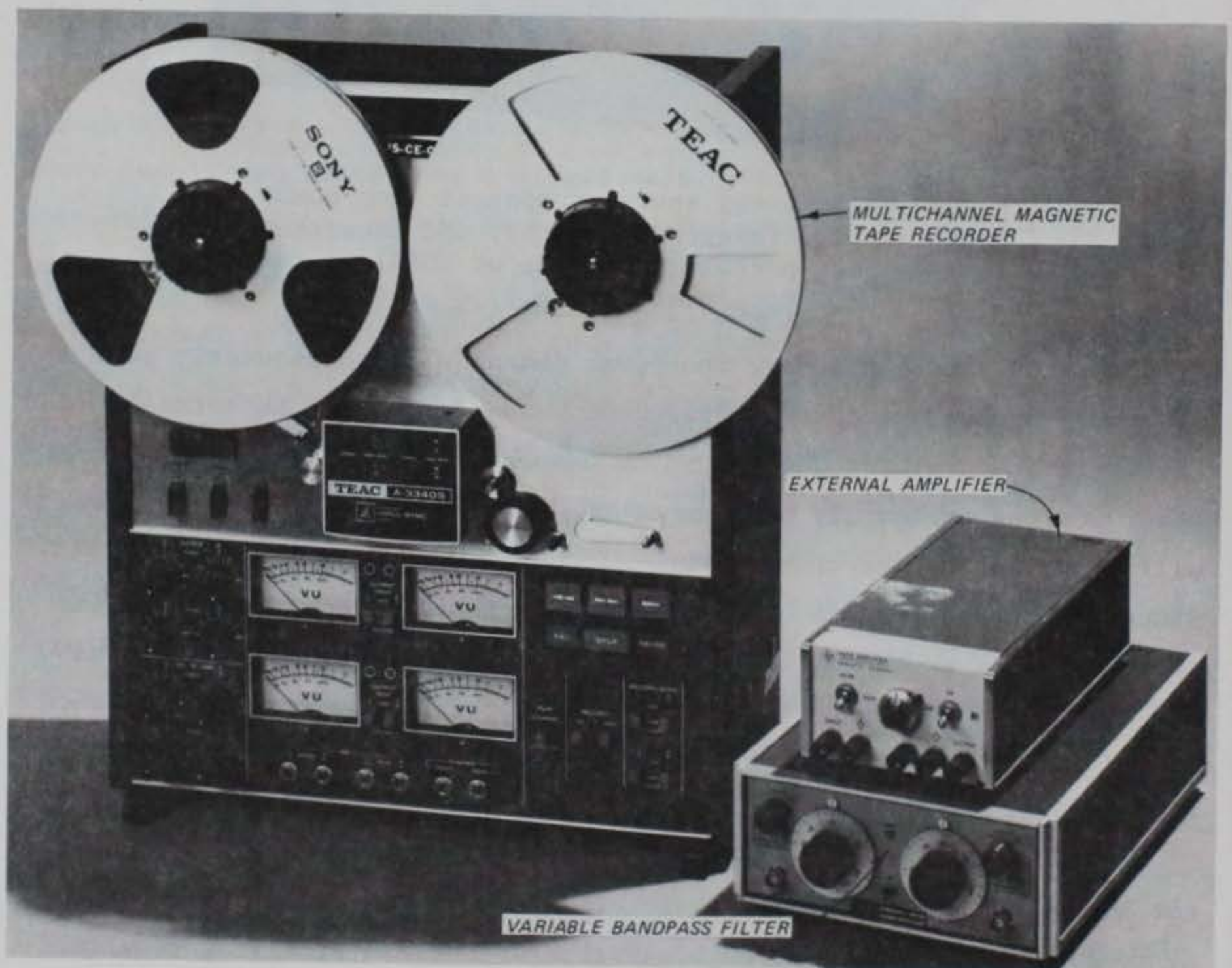
Figure 16. Signal processing components commonly utilized with small acoustic profiling systems
